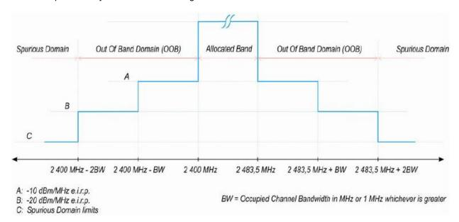
NOTE: Within the 2 400 MHz to 2 483.5 MHz band, the Out-of-band emissions are fulfilled by compliance with the Occupied Channel Bandwidth requirement in clause 4.3.2.7.
