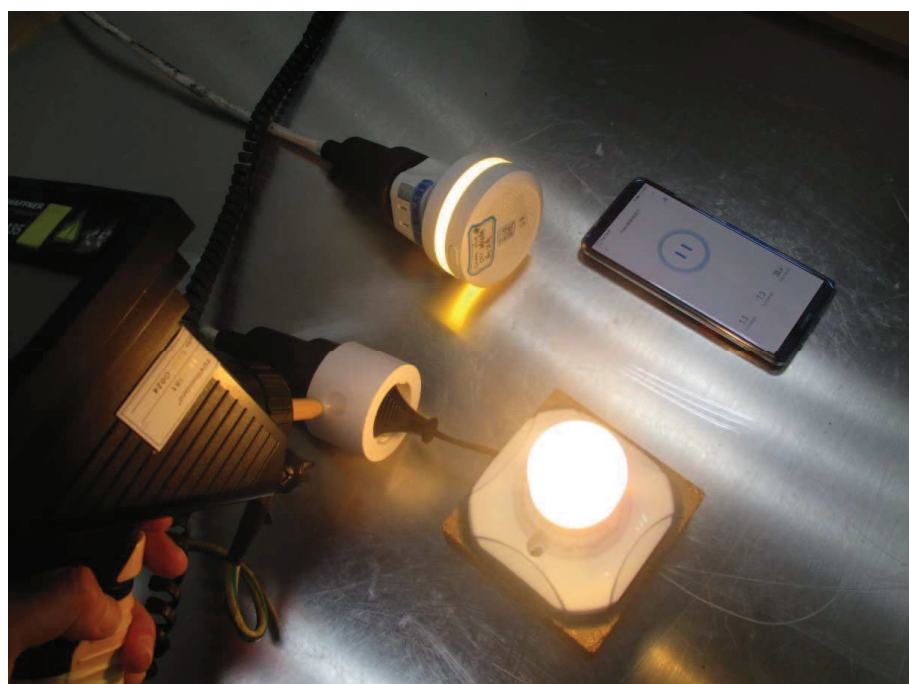
Photograph 2: Set-up for immunity test of electrostatic discharge
