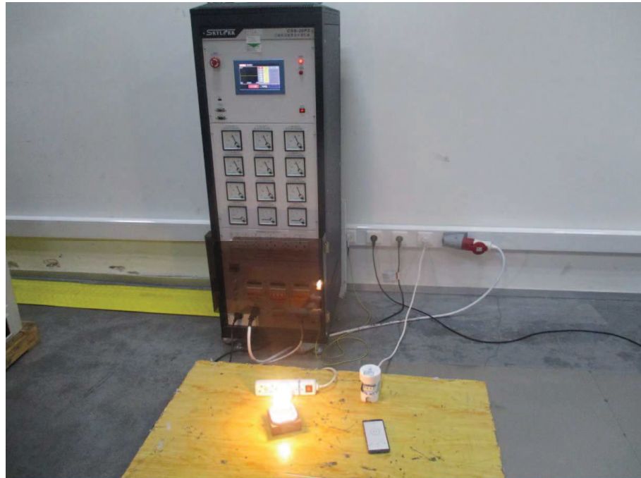
Photograph 6: Set-up for immunity test of voltage dips and short interruptions
