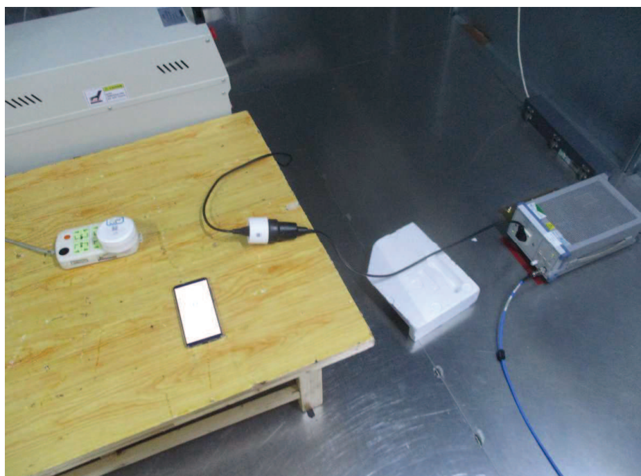
Photograph 2: Set-up for immunity test of electrostatic discharge
