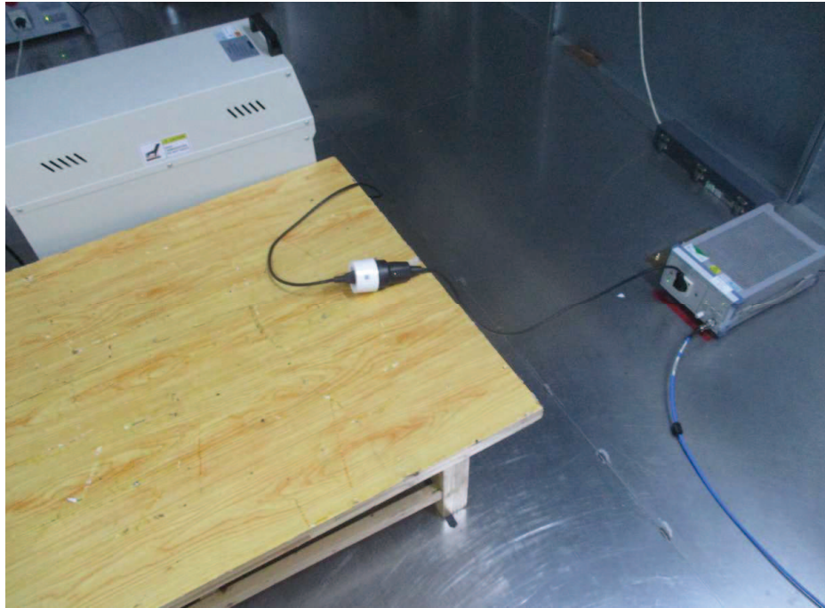
Photograph 1: Set-up for disturbance voltage measurement
