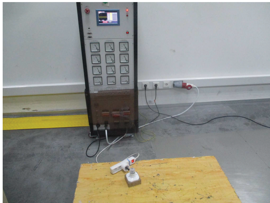
Photograph 7: Set-up for voltage dips and interruptions immunity test
