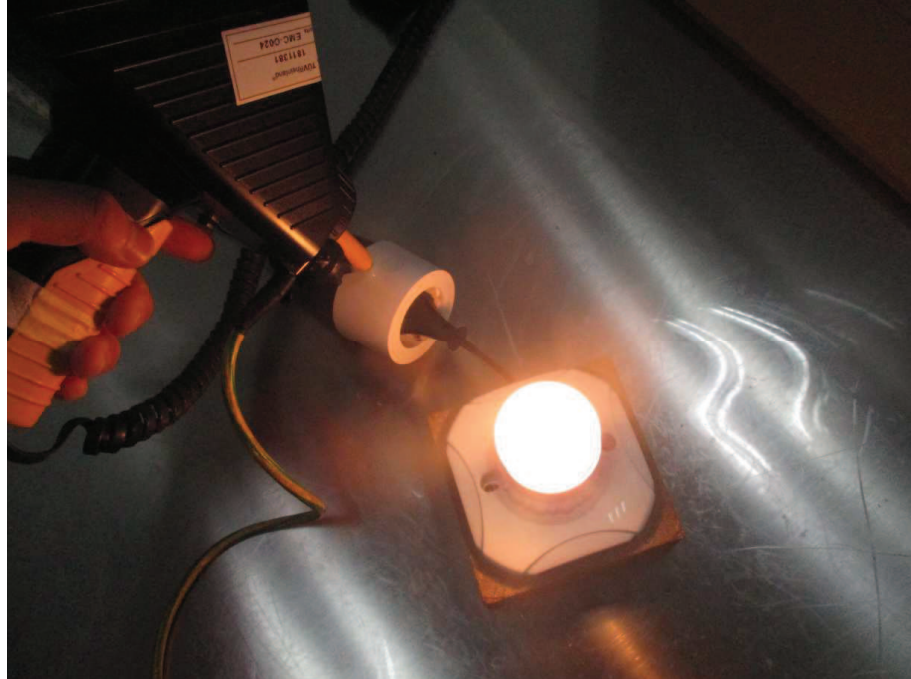
Photograph 3: Set-up for electrostatic discharge immunity test
