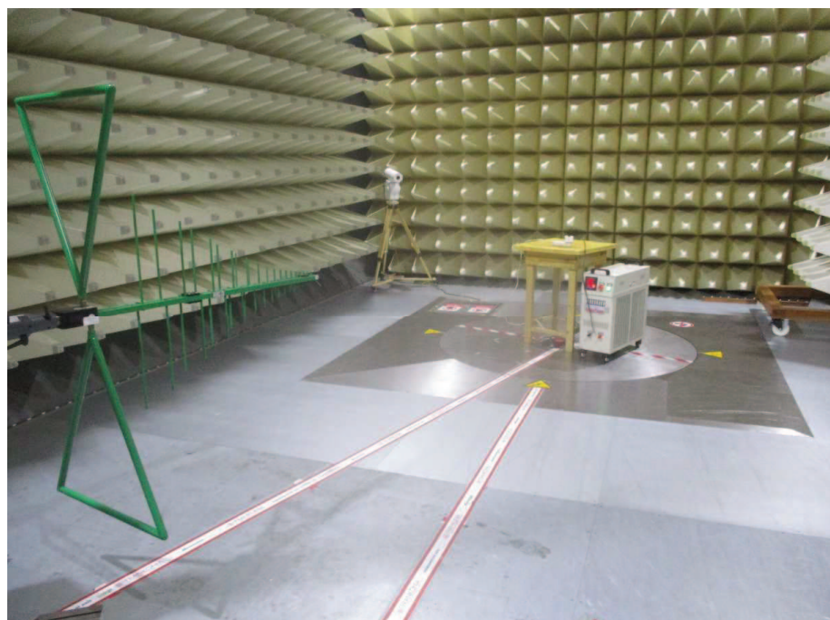
Photograph 2: Set-up for measurement of radiated emissions
