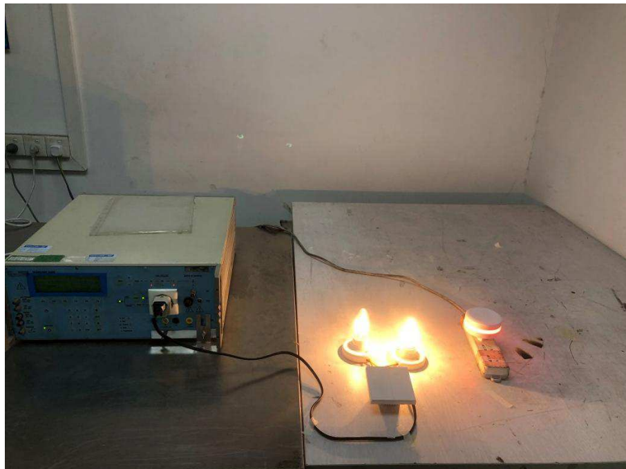
Photograph 11: Set-up for Voltage dips
