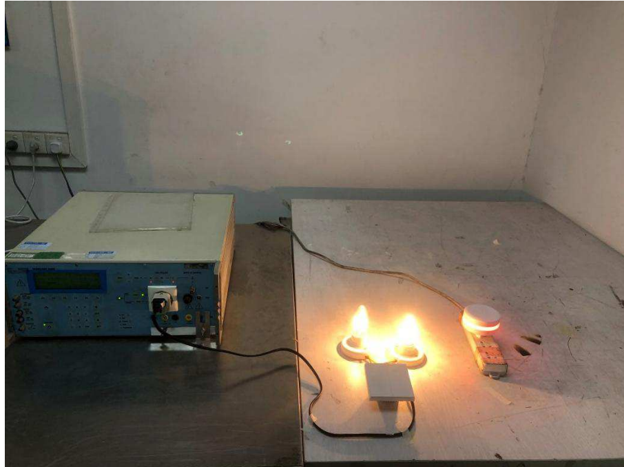
Photograph 10: Set-up for Surge
