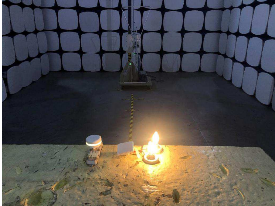
Photograph 5: Set-up for Radiated Emission
