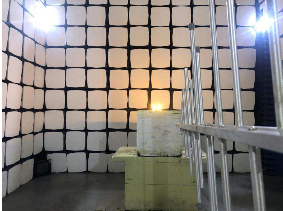
Photograph 2: Set-up for Transmitter & Receiver Spurious Emissions
