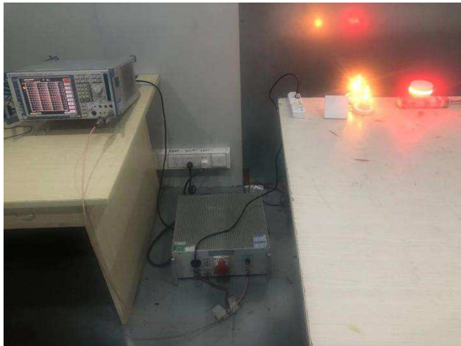
Photograph 4: Set-up for Conducted Emission
