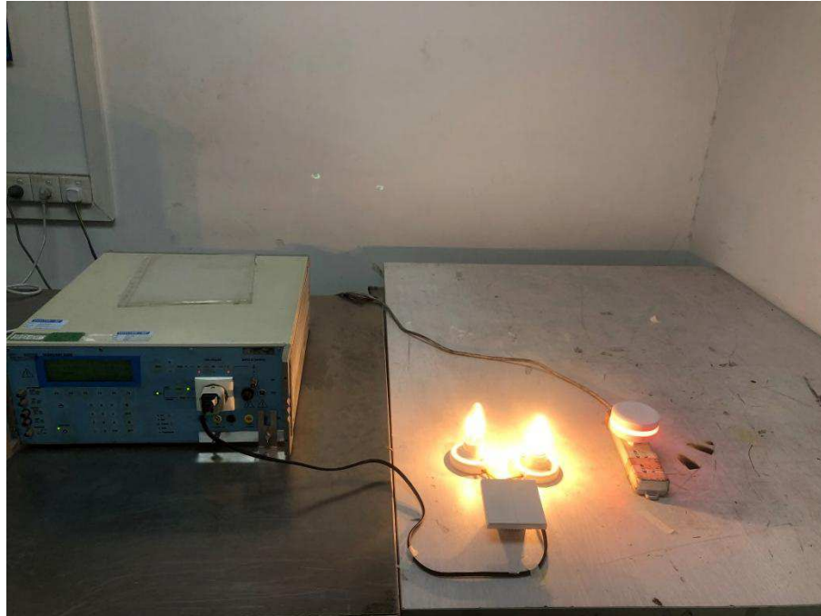
Photograph 10: Set-up for Surge
