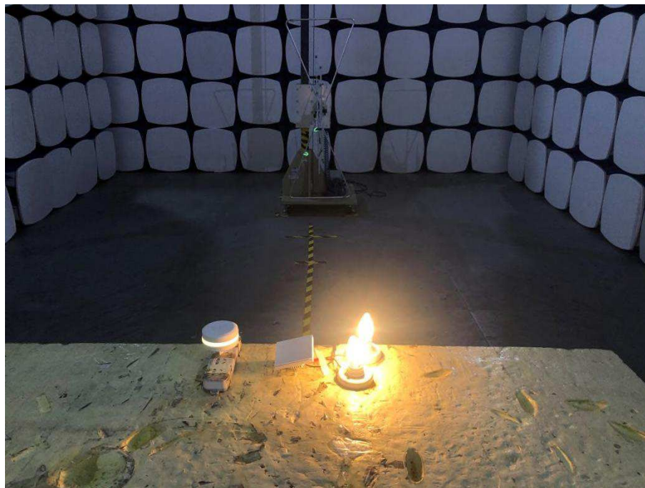
Photograph 5: Set-up for Radiated Emission
