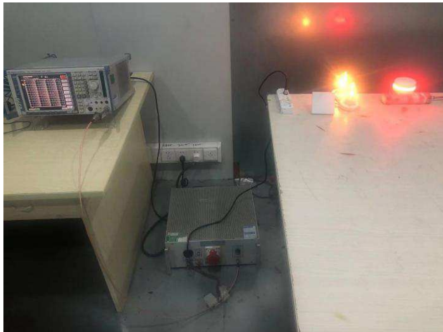
Photograph 4: Set-up for Conducted Emission
