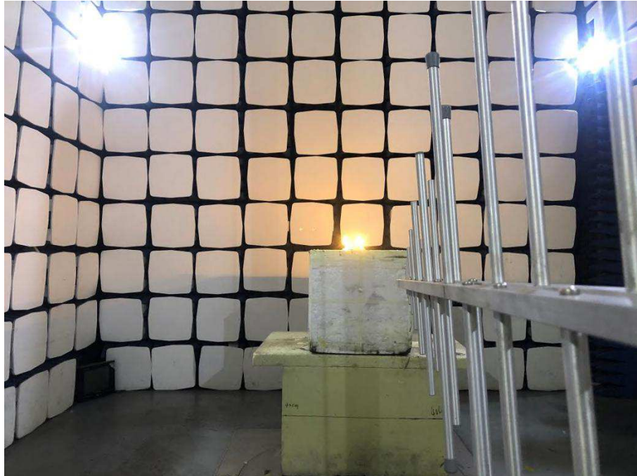
Photograph 2: Set-up for Transmitter & Receiver Spurious Emissions
