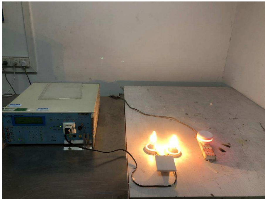
Photograph 11: Set-up for Voltage dips
