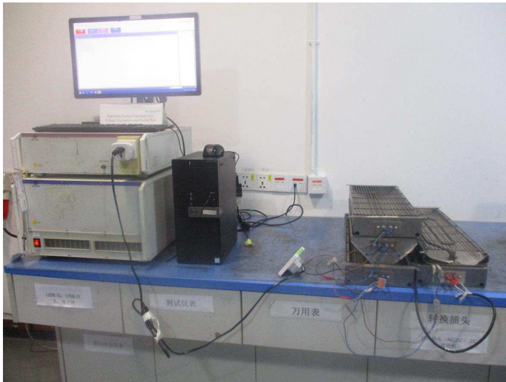
Photograph 1: Set-up for Harmonic Current Emission on AC Mains
