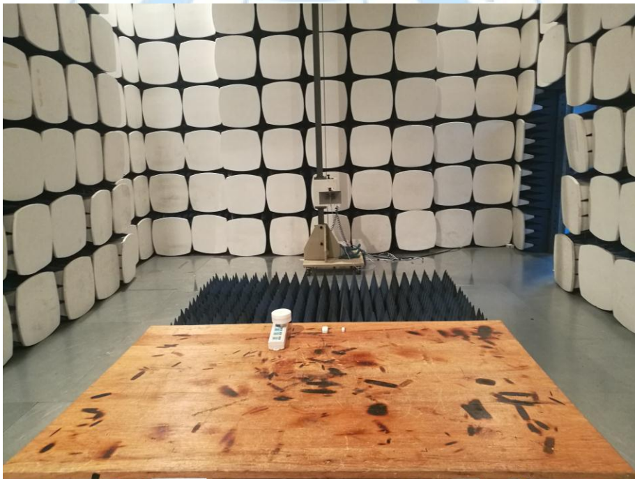
Radiated Measurement (1000~6000MHz)
