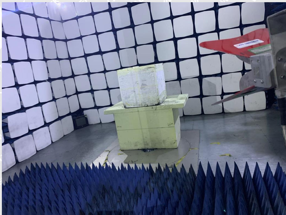
Spurious Emission Test Setup (Above 1GHz)
