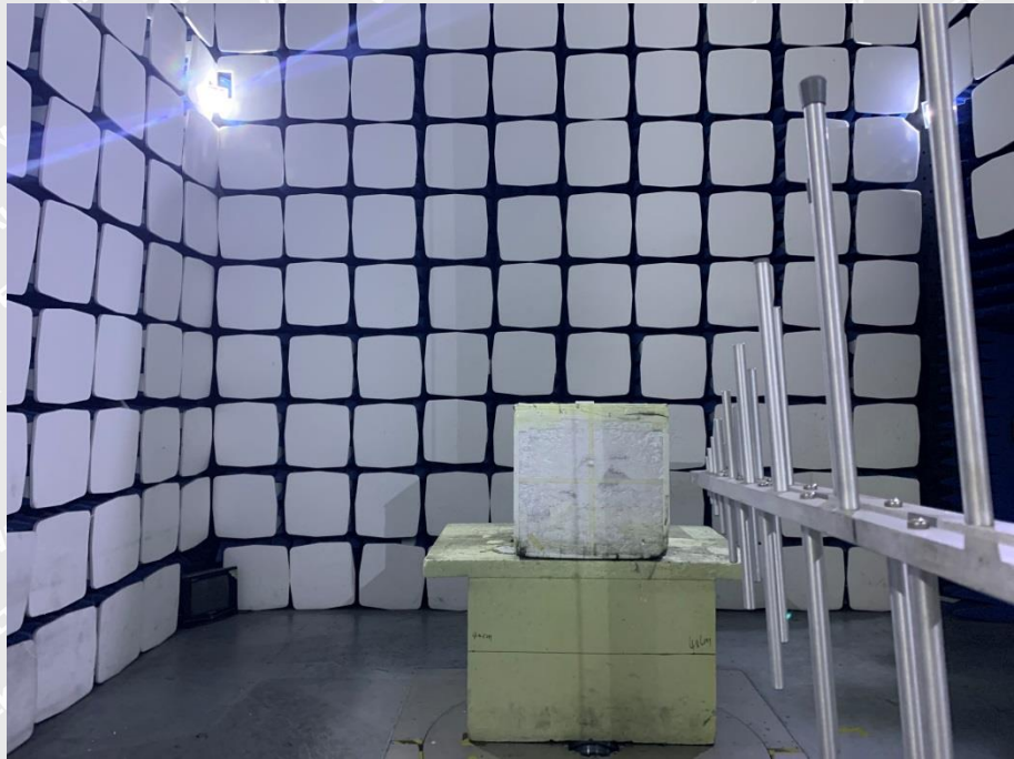
Spurious Emission Test Setup (Below 1GHz)
