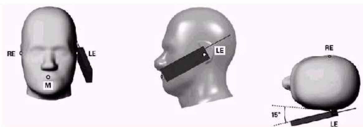
Figure 6.3.1 – Tilt position of the wireless device on the left side of SAM
