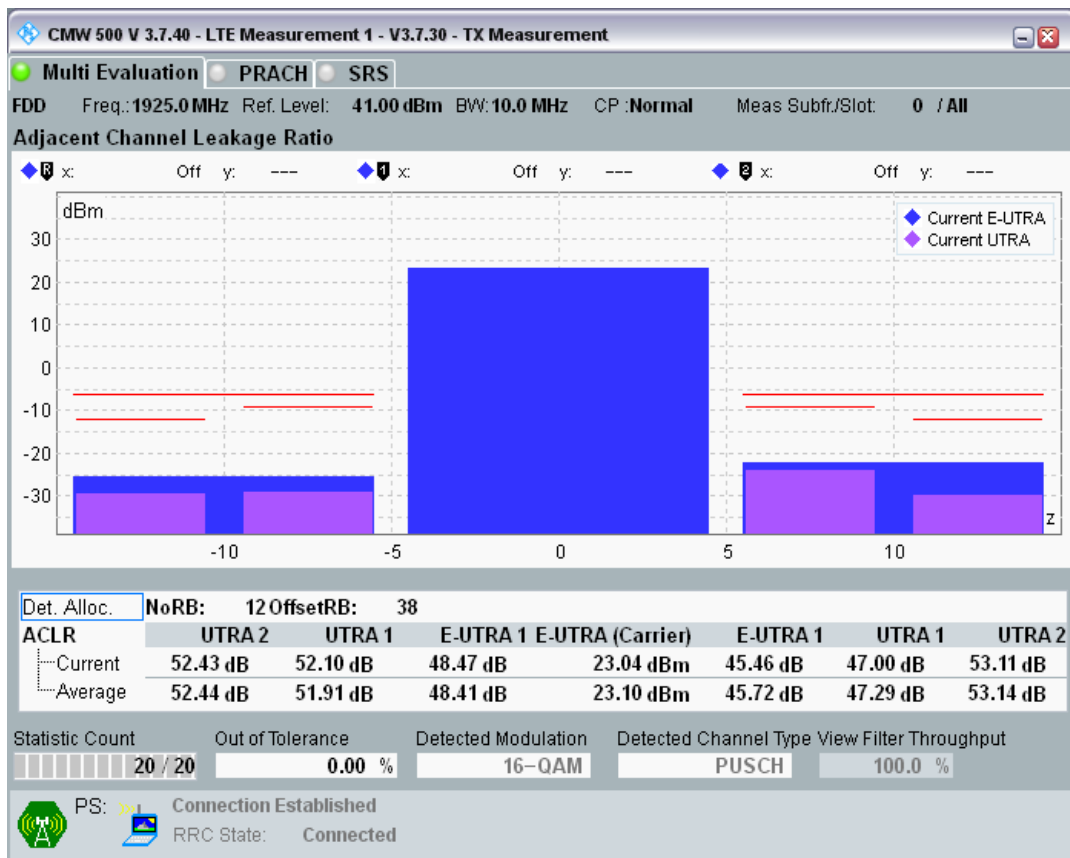
Band1 QAM16 BW=10MHz Channel=18050 RB Size=50 Position=#0
