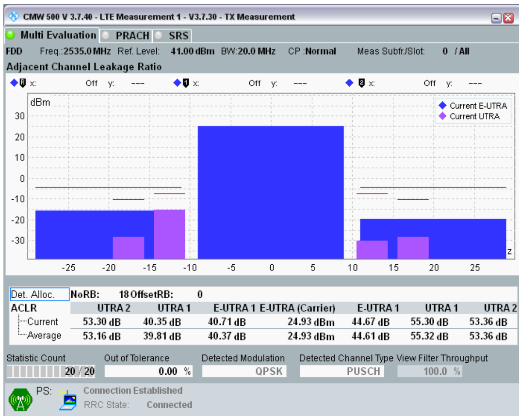
Band7 QPSK BW=20MHz Channel=21100 RB Size=18 Position=#Max
