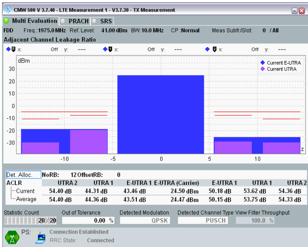
Band1 QPSK BW=10MHz Channel=18550 RB Size=12 Position=#Max
