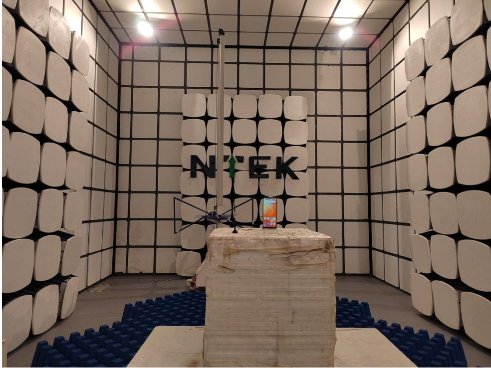
Radiated Spurious Emission Test
