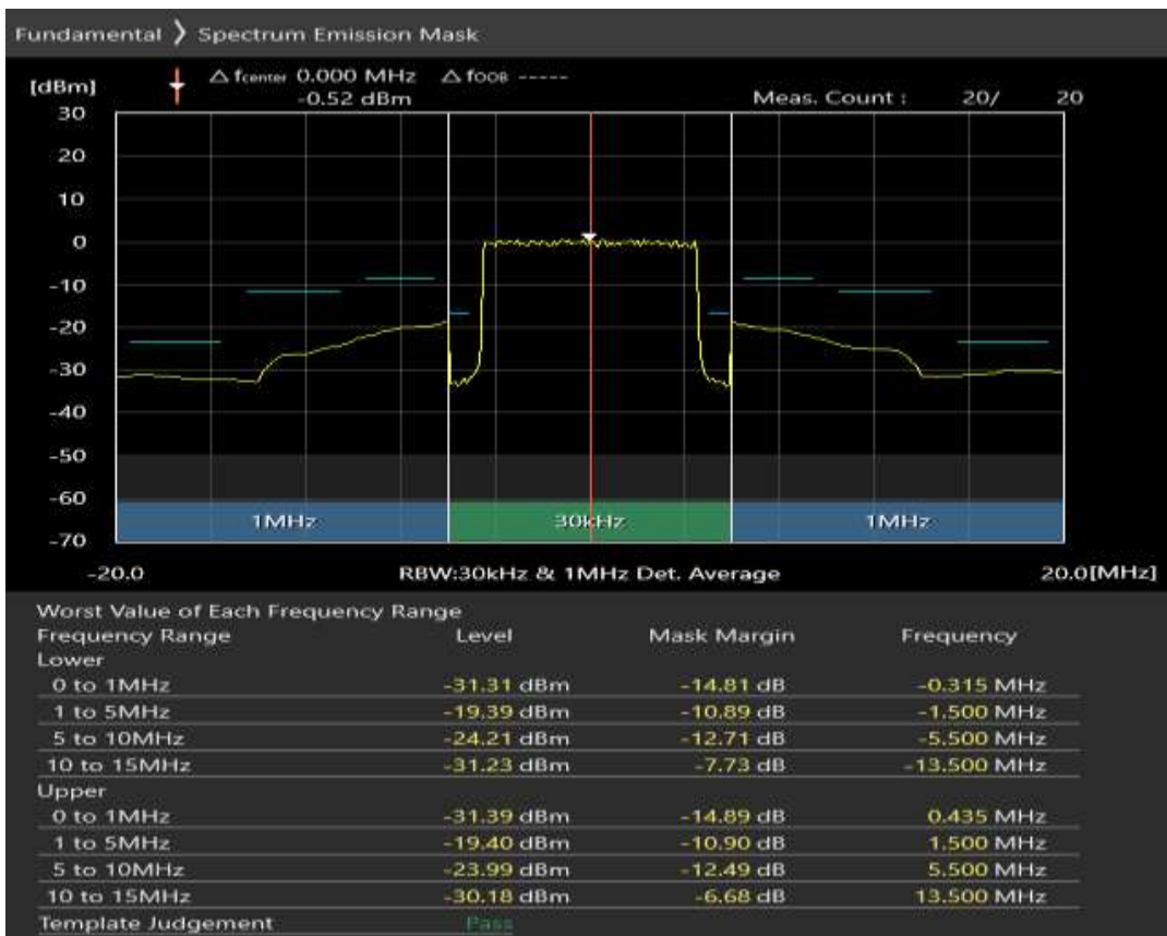
Band40 QAM16 BW=10MHz Channel=39150 RB Size=12 Position=#0
