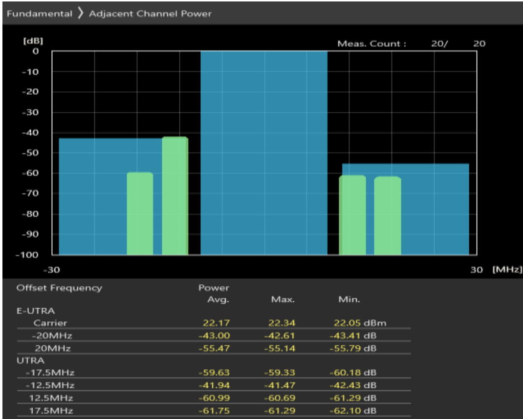
Band1 QAM16 BW=20MHz Channel=18100 RB Size=18 Position=#Max
