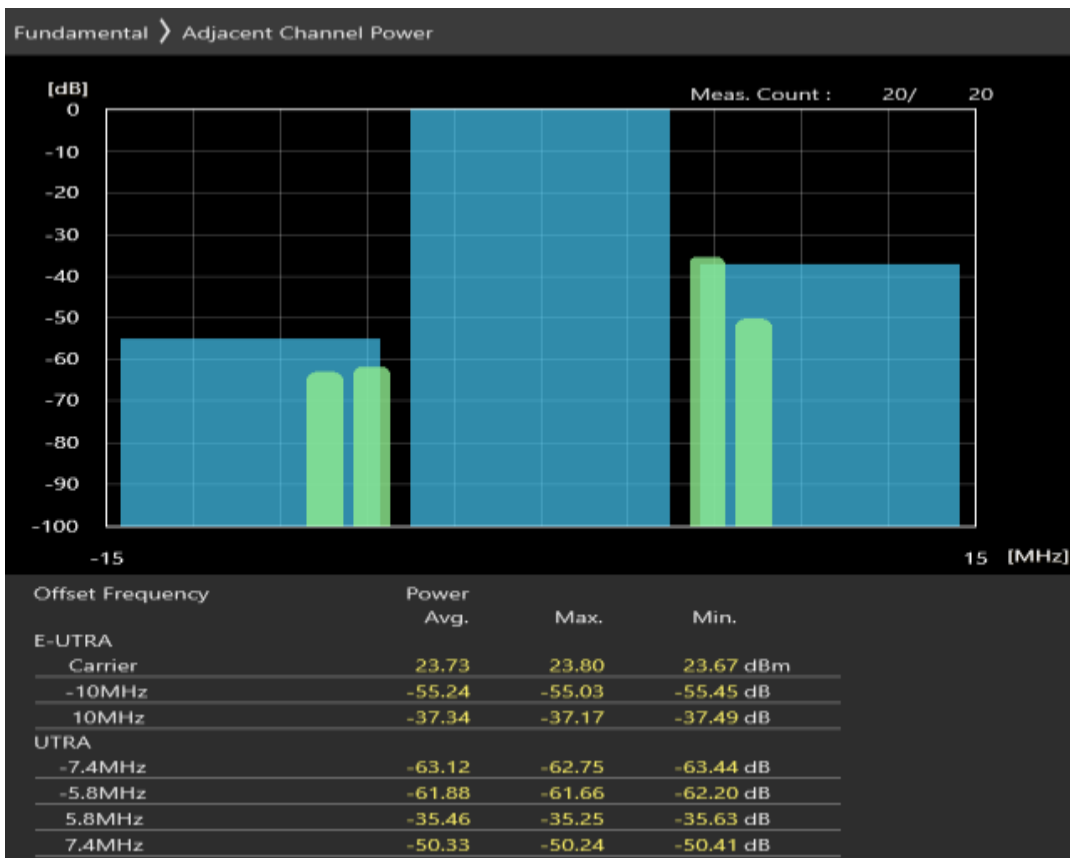
Band40 QAM16 BW=10MHz Channel=39600 RB Size=50 Position=#0
