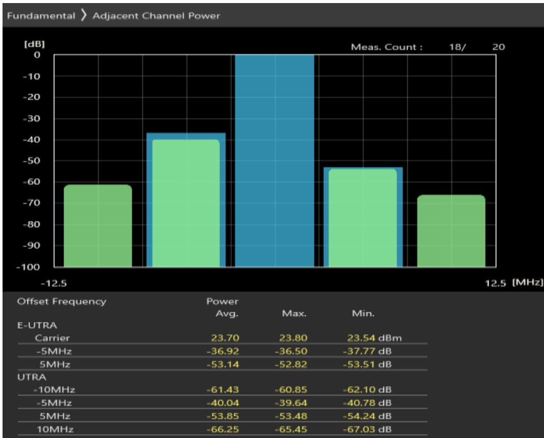
Band7 QAM16 BW=5MHz Channel=21100 RB Size=8 Position=#Max
