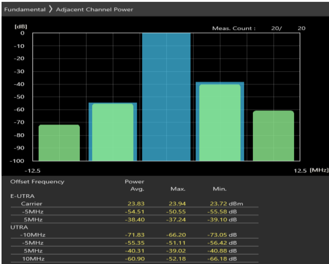
Band8 QPSK BW=5MHz Channel=21625 RB Size=25 Position=#0
