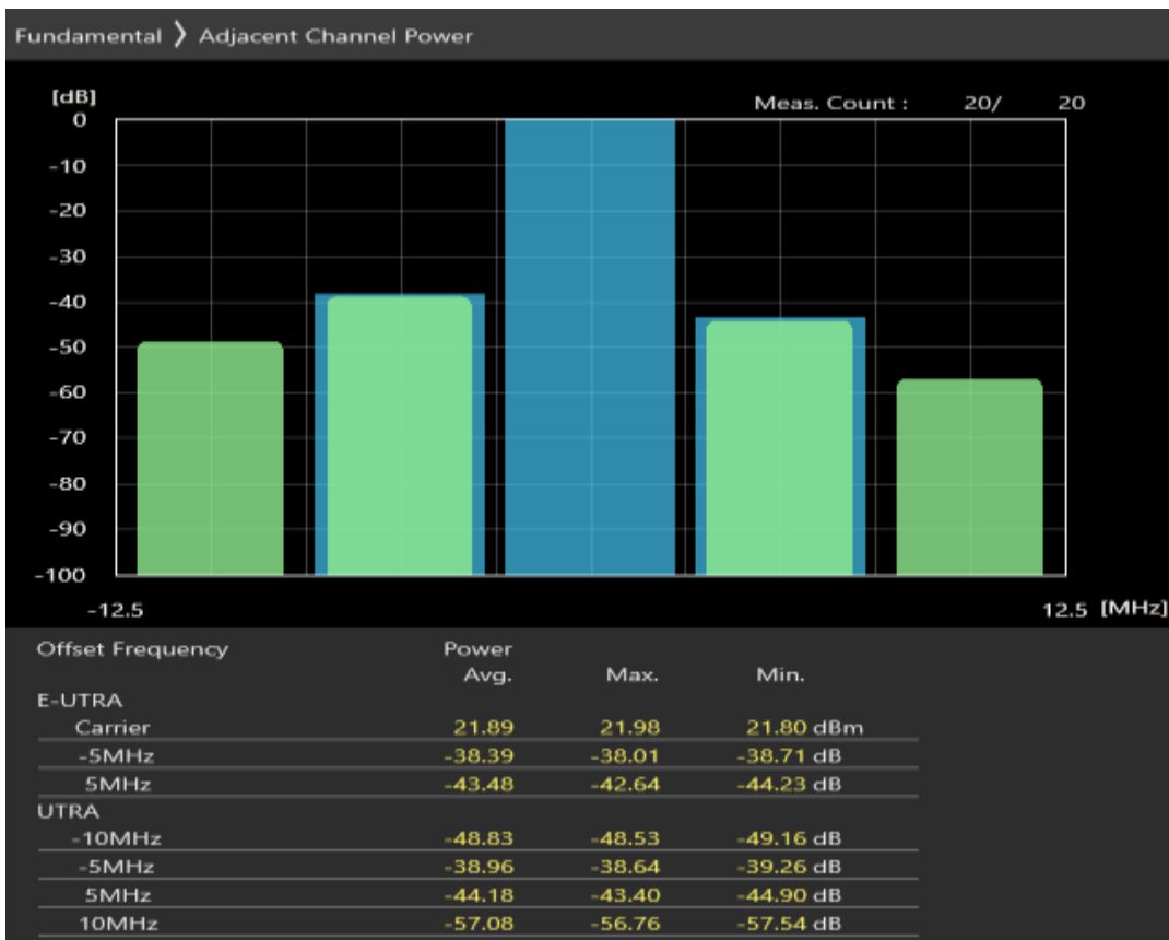
Band20 QAM16 BW=5MHz Channel=24425 RB Size=8 Position=#0
