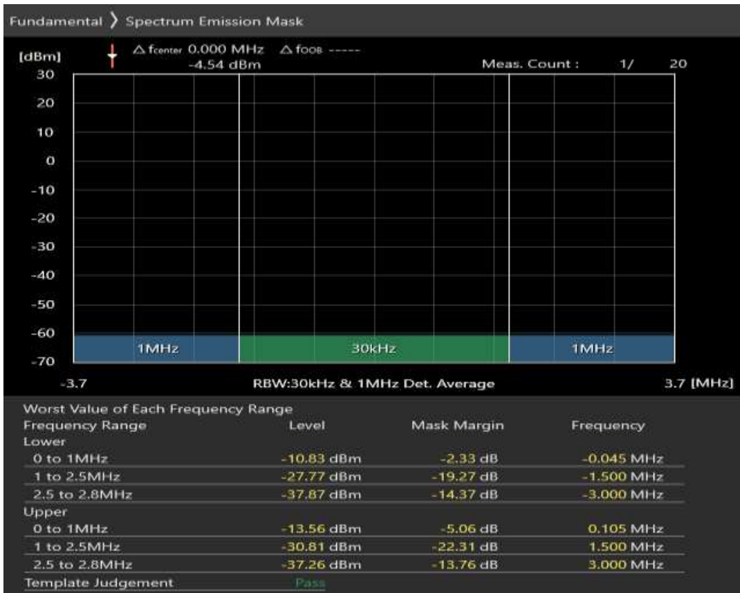
Band8 QPSK BW=1.4MHz Channel=21457 RB Size=5 Position=#Max
