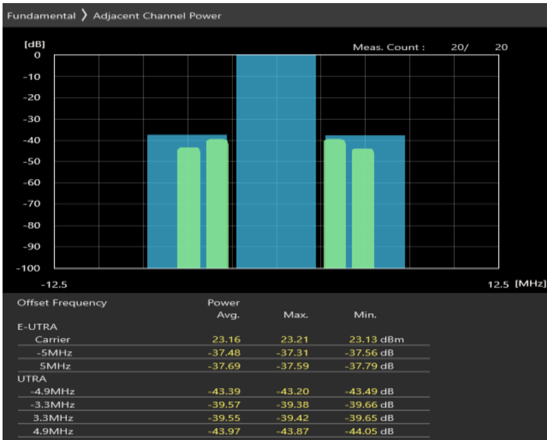
Band38 QPSK BW=5MHz Channel=38000 RB Size=8 Position=#0
