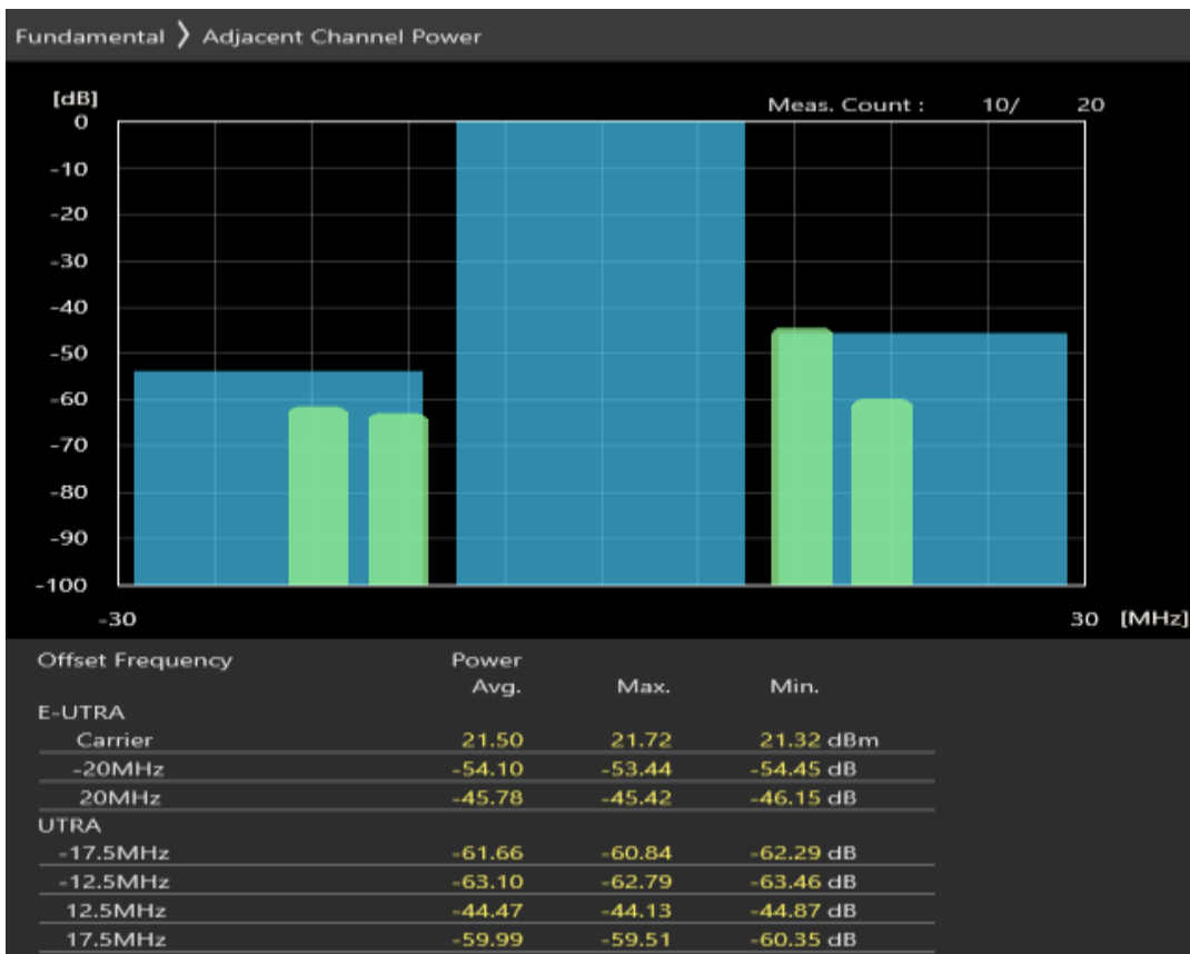
Band3 QAM16 BW=20MHz Channel=19300 RB Size=100 Position=#0
