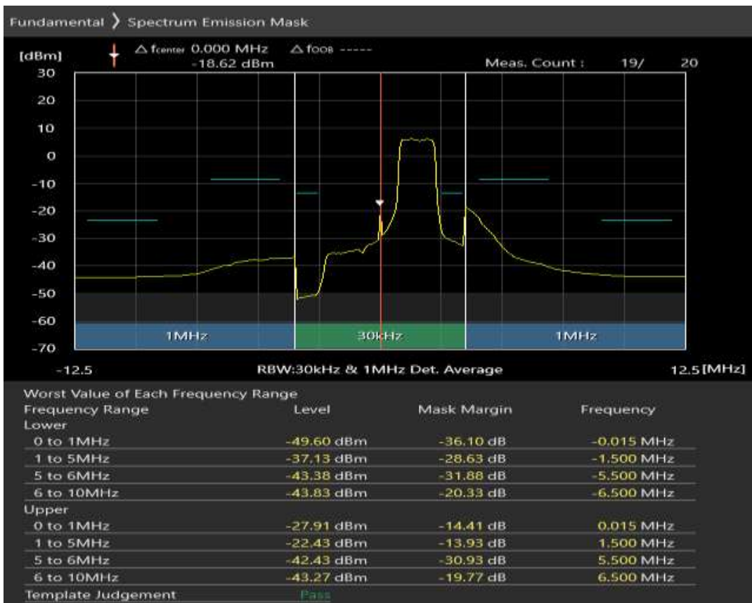
Band1 QAM16 BW=5MHz Channel=18300 RB Size=25 Position=#0
