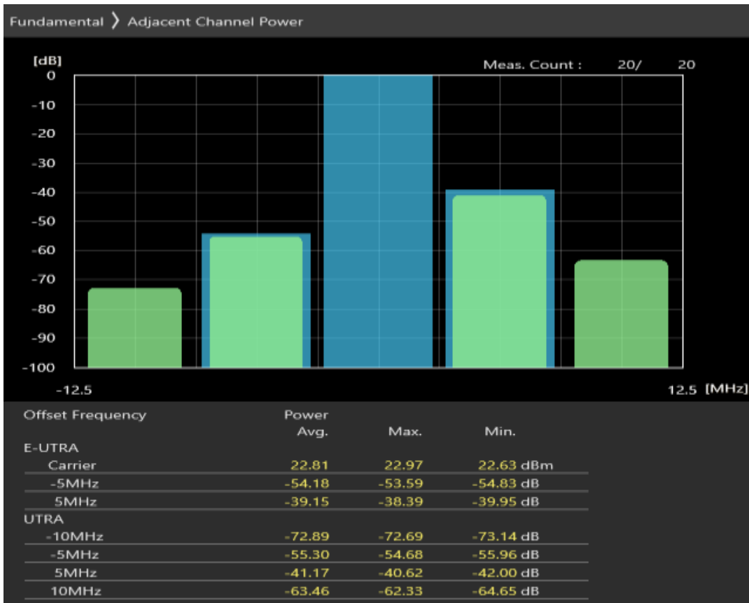
Band28 QPSK BW=5MHz Channel=27235 RB Size=25 Position=#0
