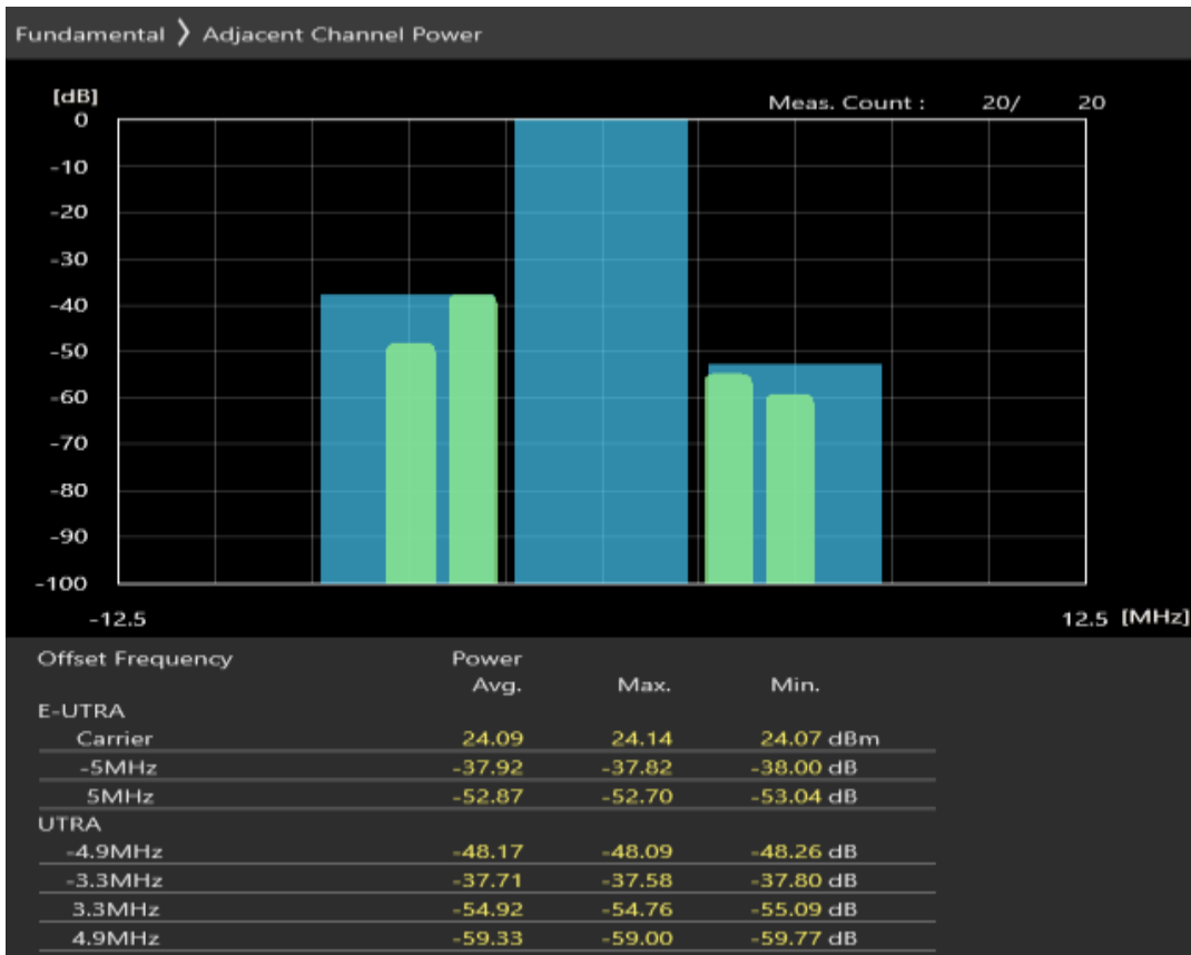
Band40 QPSK BW=5MHz Channel=38675 RB Size=8 Position=#Max
