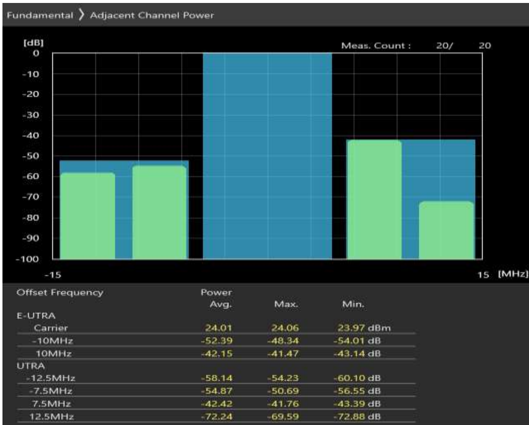
Band8 QPSK BW=10MHz Channel=21750 RB Size=50 Position=#0
