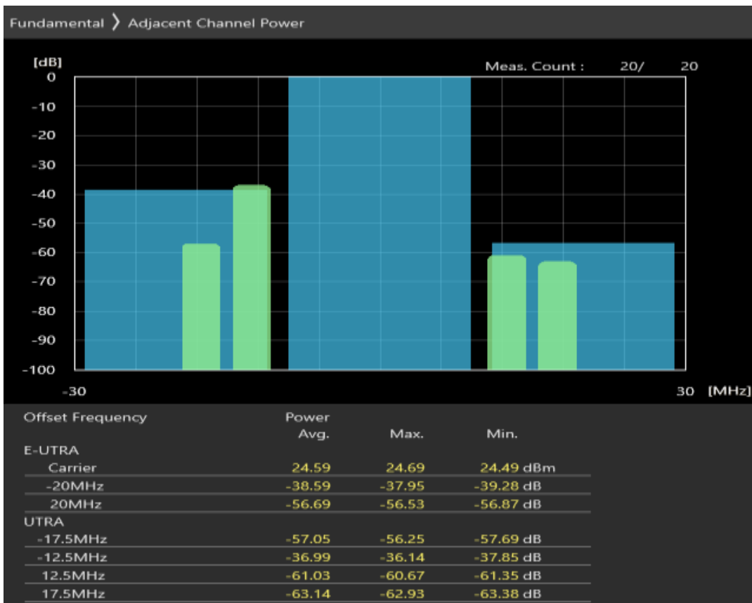
Band1 QPSK BW=20MHz Channel=18100 RB Size=18 Position=#Max
