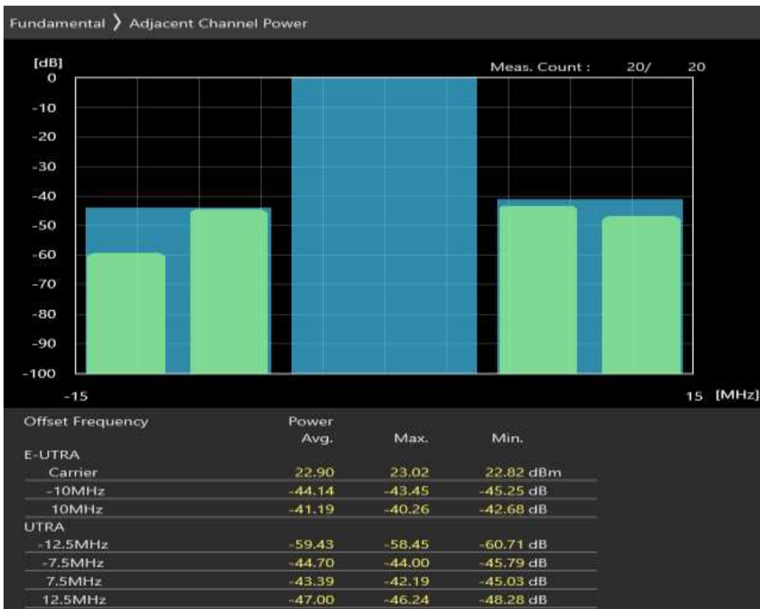
Band8 QPSK BW=10MHz Channel=21625 RB Size=12 Position=#0
