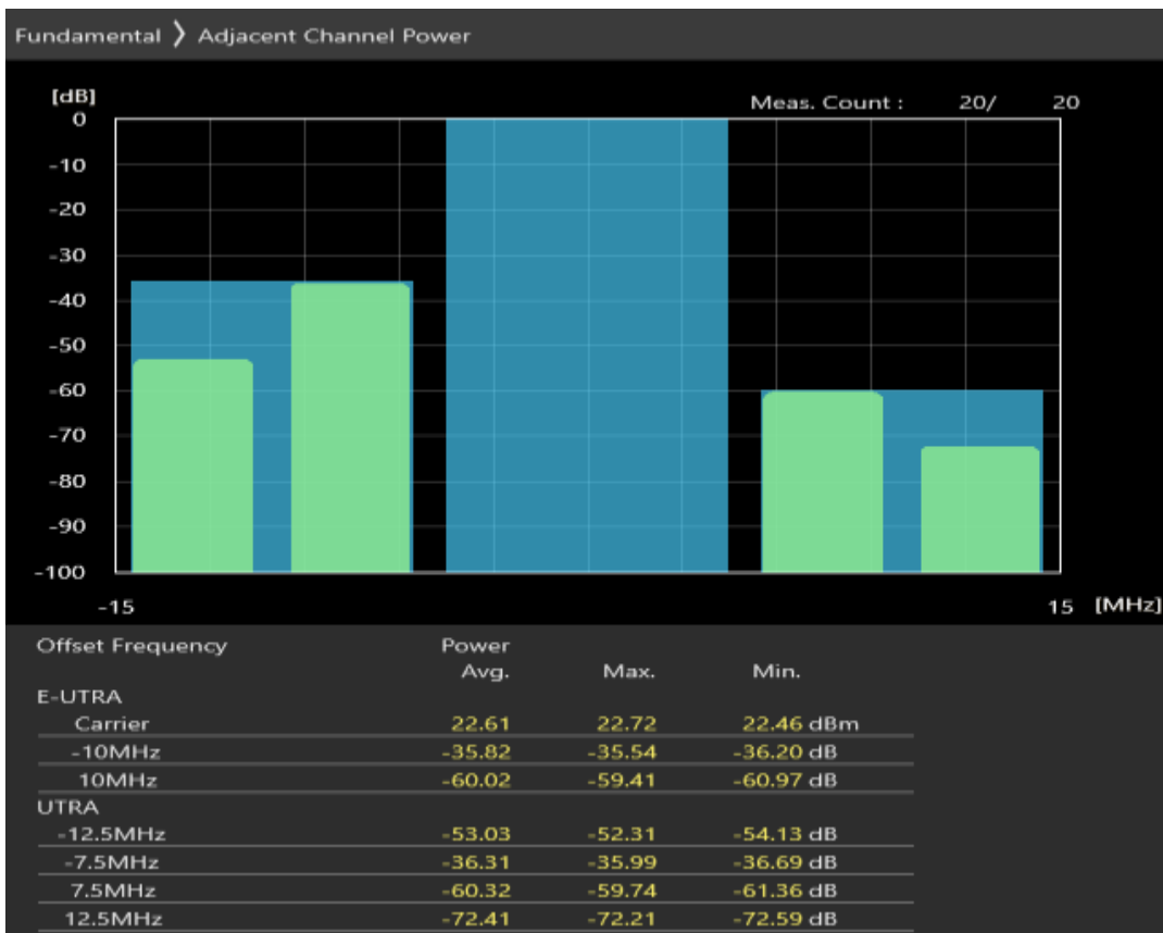
Band28 QPSK BW=10MHz Channel=27610 RB Size=12 Position=#Max
