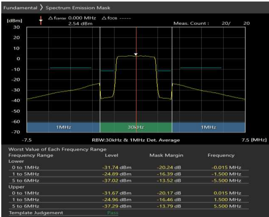
Band28 QPSK BW=3MHz Channel=27495 RB Size=4 Position=#0
