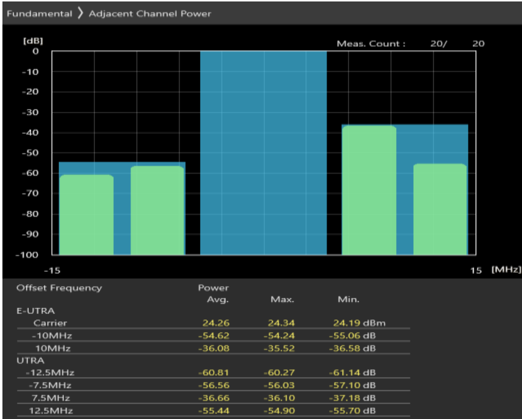
Band7 QPSK BW=10MHz Channel=21400 RB Size=50 Position=#0
