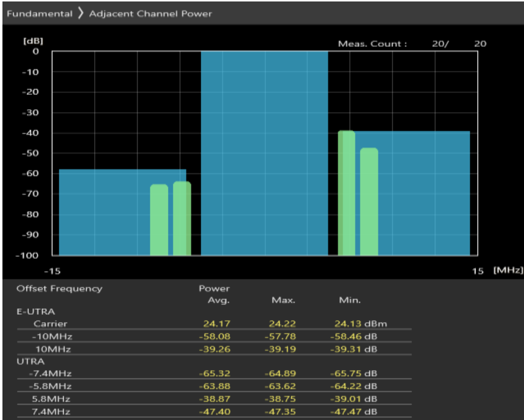
Band40 QPSK BW=10MHz Channel=38700 RB Size=50 Position=#0
