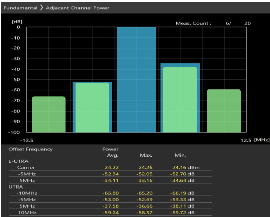
Band7 QPSK BW=5MHz Channel=21425 RB Size=25 Position=#0
