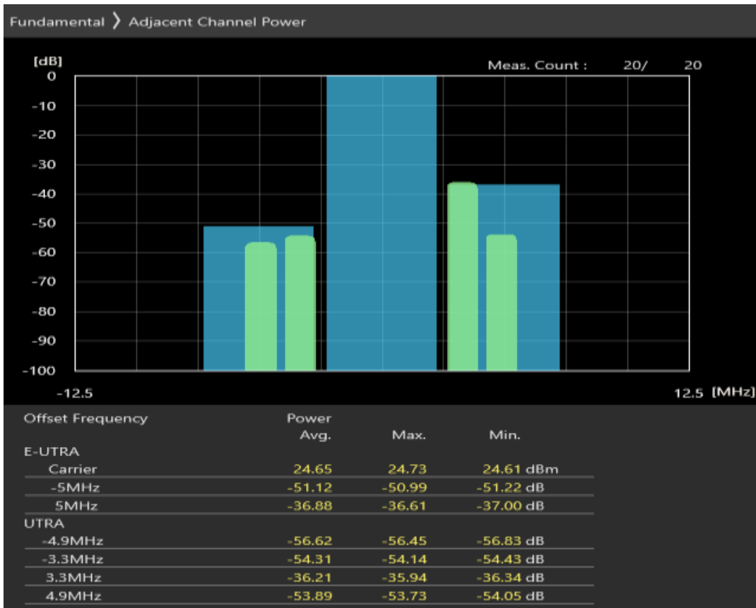
Band38 QPSK BW=5MHz Channel=37775 RB Size=25 Position=#0
