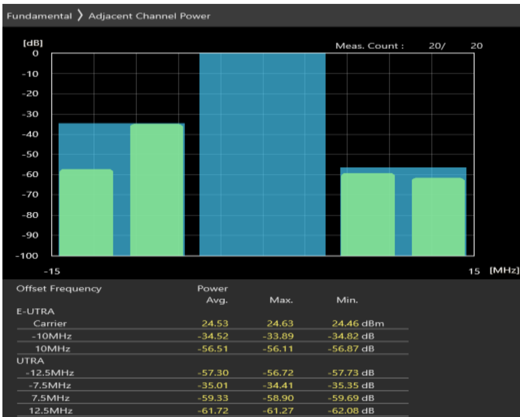
Band20 QPSK BW=10MHz Channel=24300 RB Size=12 Position=#Max
