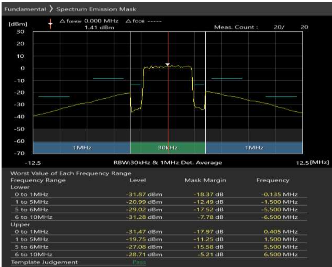
Band40 QPSK BW=5MHz Channel=39150 RB Size=8 Position=#0
