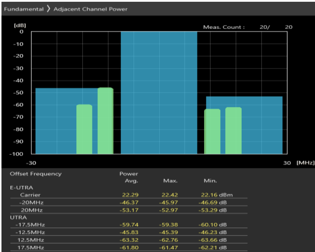
Band3 QPSK BW=20MHz Channel=19300 RB Size=18 Position=#Max
