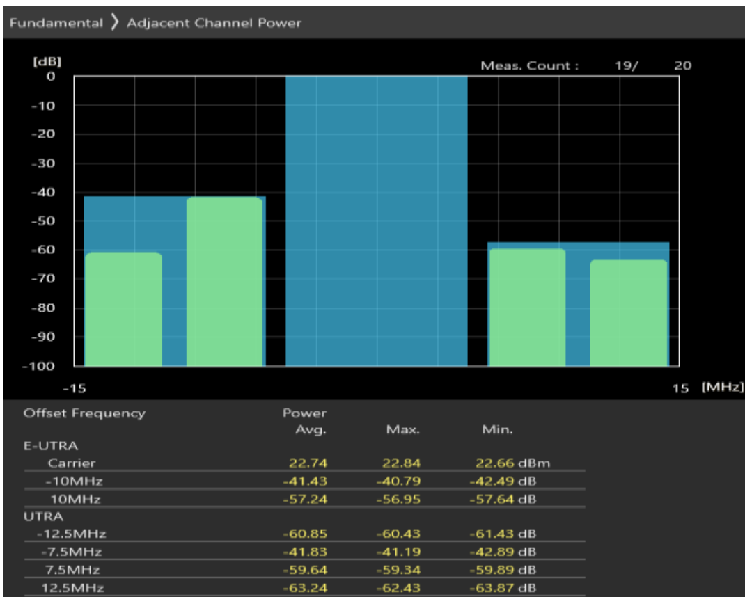
Band8 QAM16 BW=10MHz Channel=21625 RB Size=12 Position=#Max
