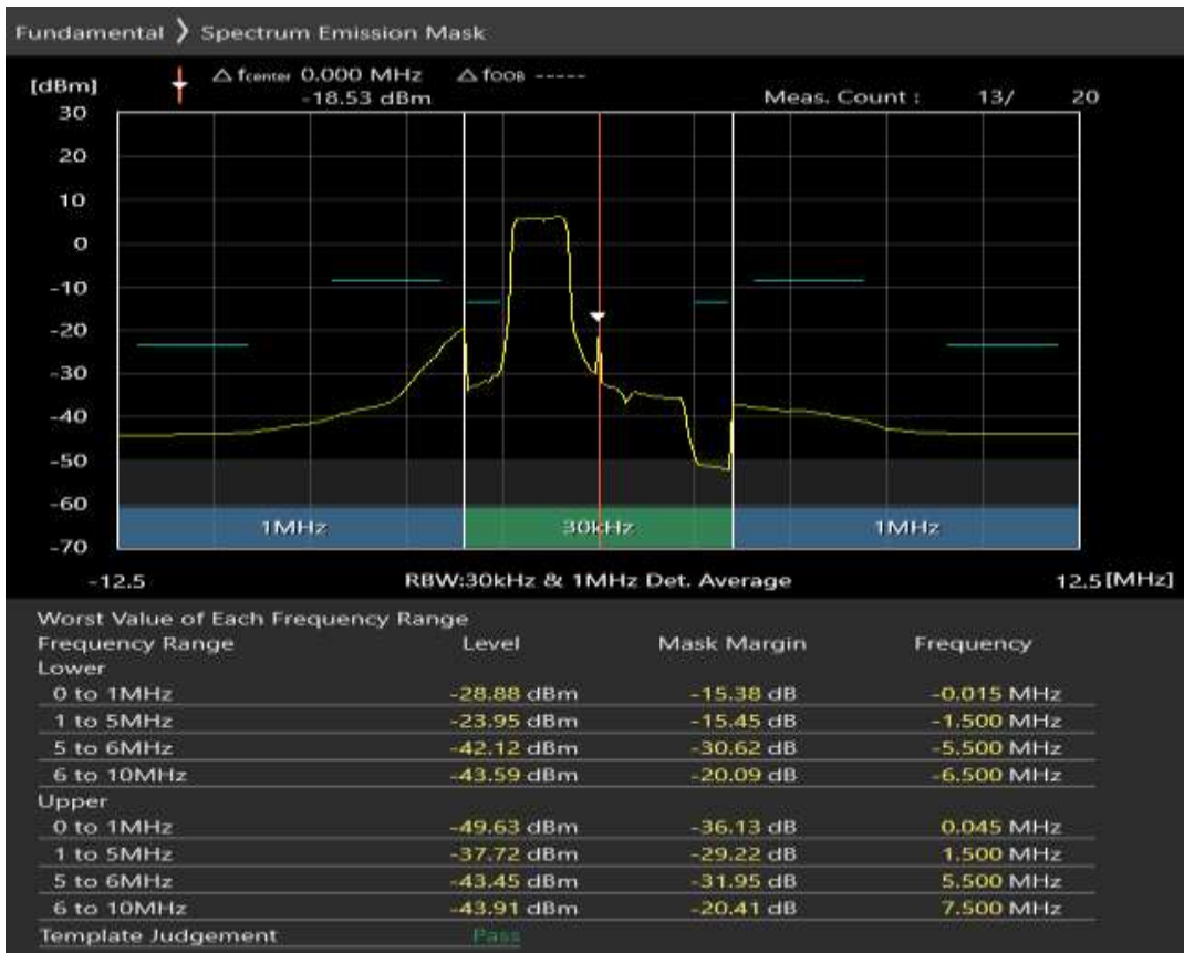
Band1 QAM16 BW=5MHz Channel=18025 RB Size=8 Position=#Max
