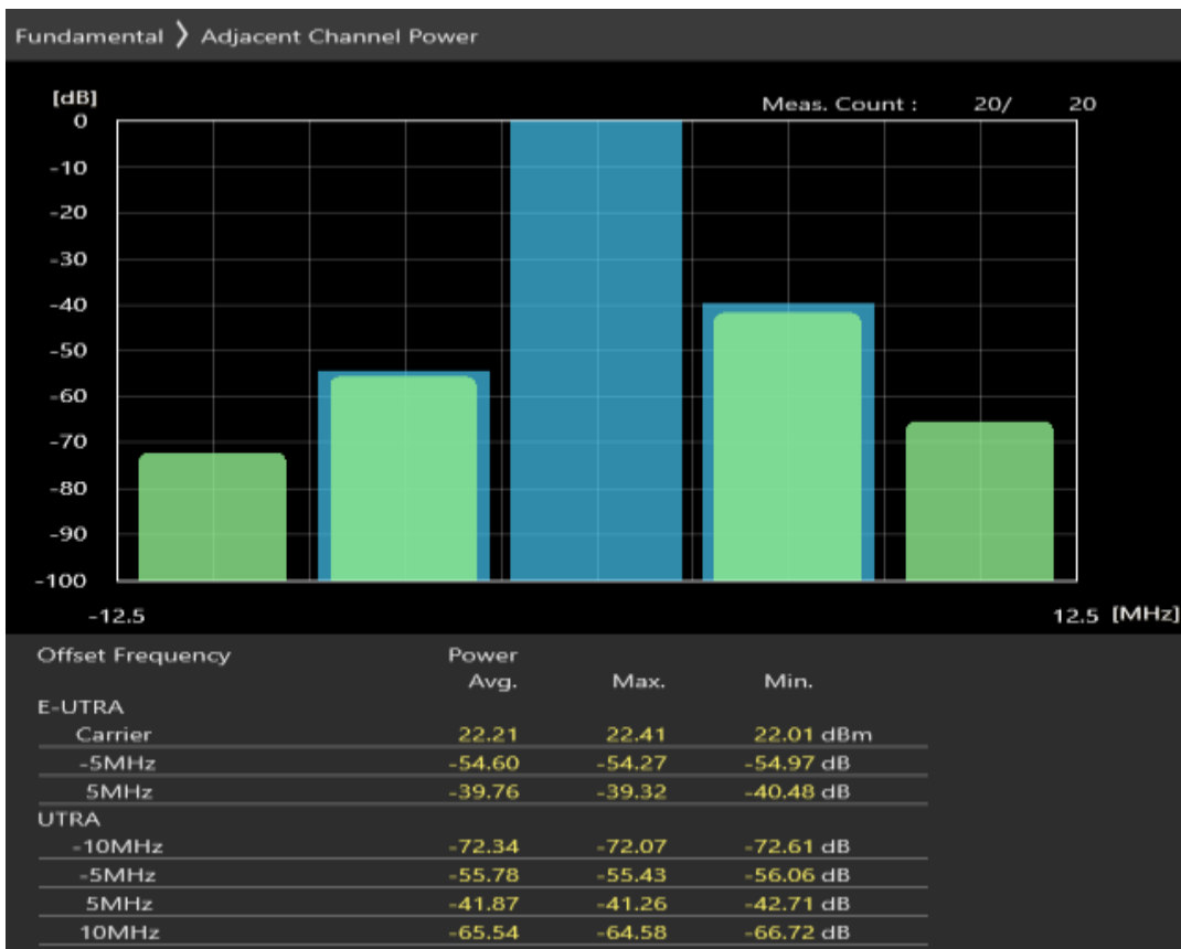
Band28 QAM16 BW=5MHz Channel=27235 RB Size=25 Position=#0
