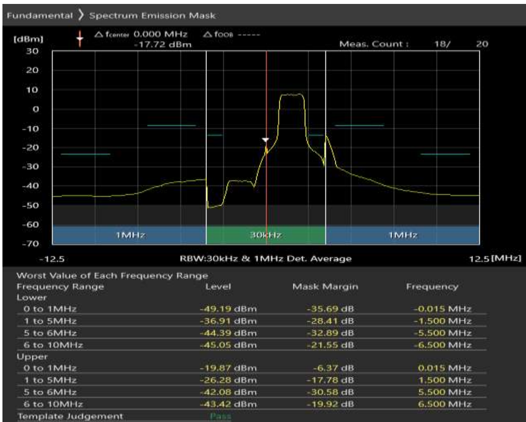
Band8 QAM16 BW=5MHz Channel=21475 RB Size=25 Position=#0
