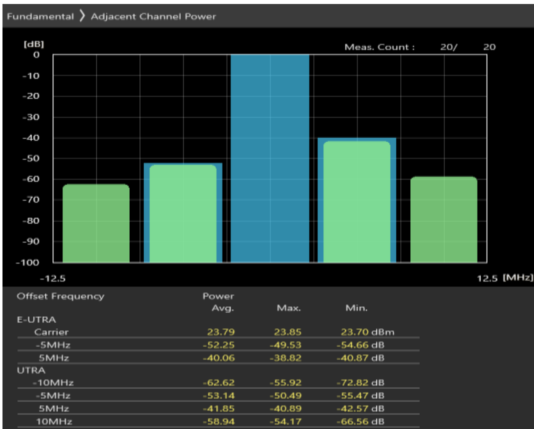
Band8 QPSK BW=5MHz Channel=21775 RB Size=25 Position=#0
