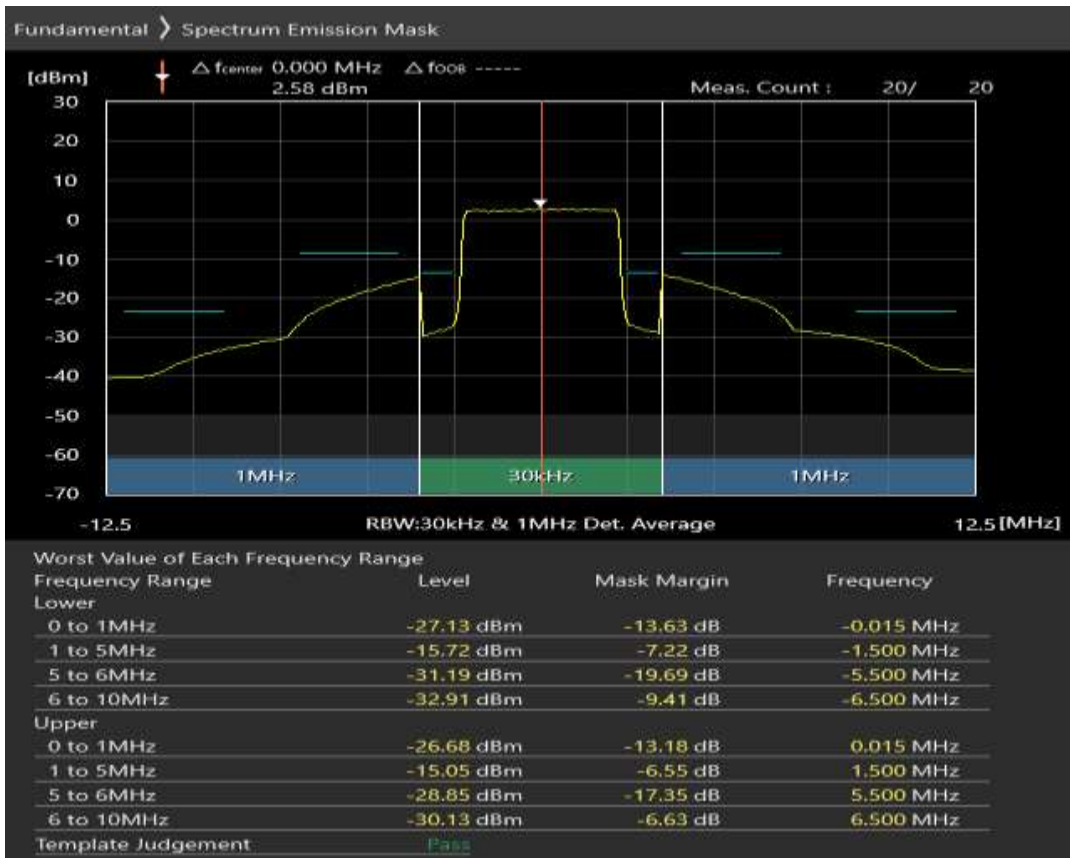
Band7 QAM16 BW=5MHz Channel=20775 RB Size=8 Position=#0
