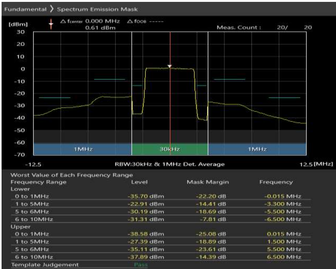
Band20 QAM16 BW=5MHz Channel=24425 RB Size=8 Position=#0
