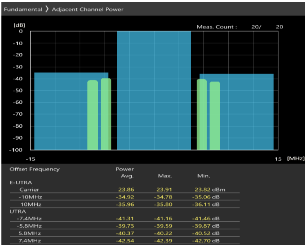
Band38 QAM16 BW=10MHz Channel=38000 RB Size=12 Position=#0
