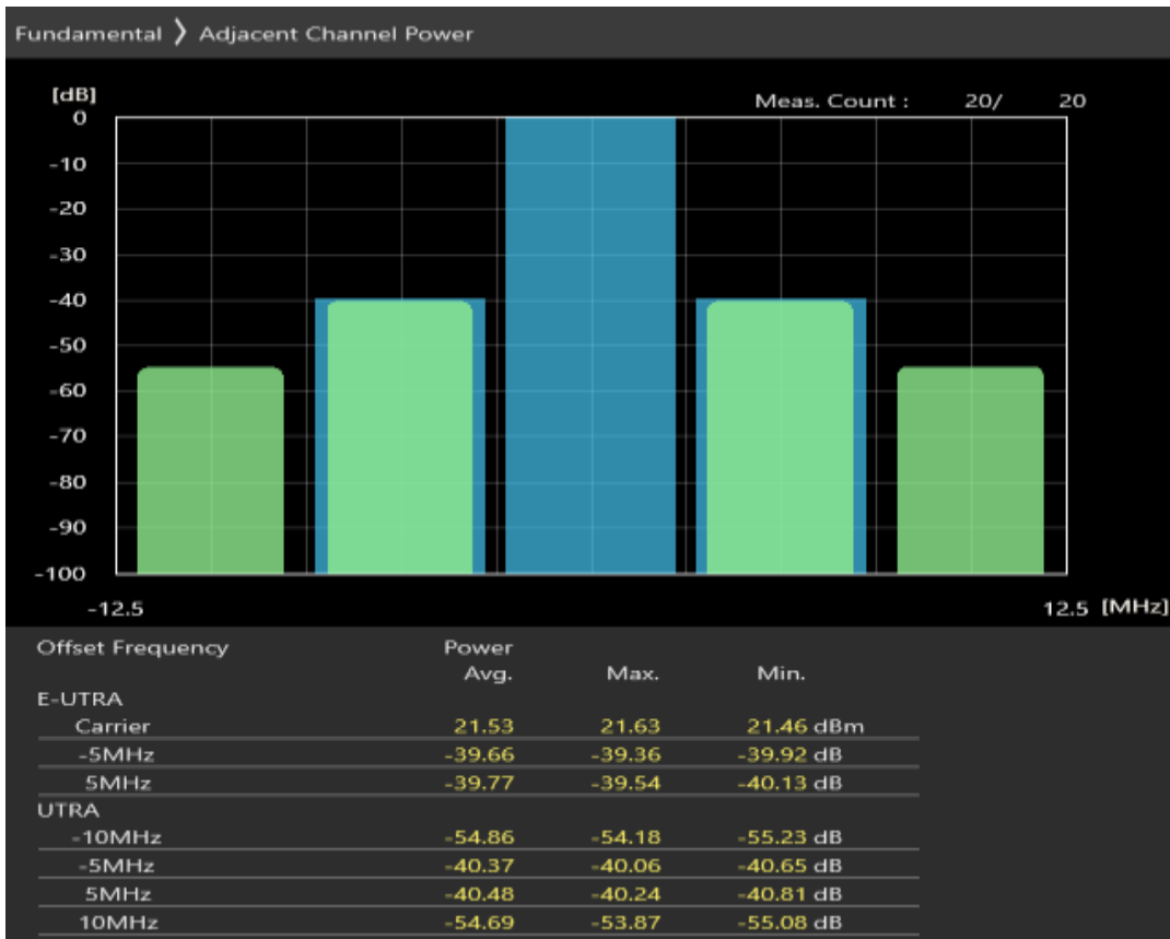
Band1 QPSK BW=5MHz Channel=18300 RB Size=8 Position=#0
