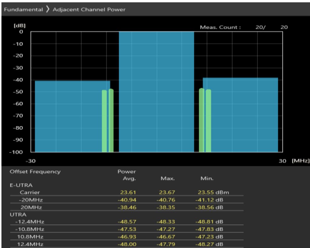
Band40 QAM16 BW=20MHz Channel=38750 RB Size=18 Position=#0
