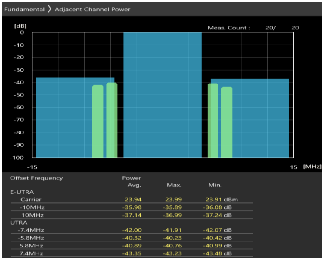
Band38 QAM16 BW=10MHz Channel=37800 RB Size=12 Position=#0
