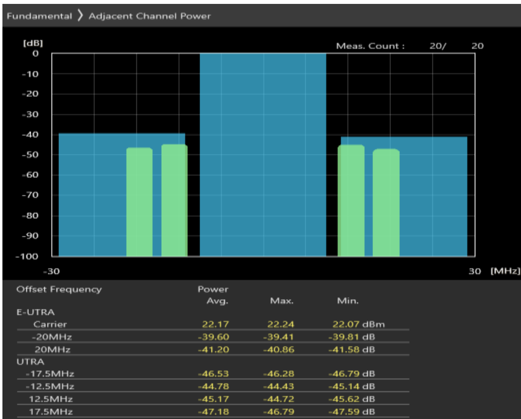
Band1 QAM16 BW=20MHz Channel=18500 RB Size=18 Position=#0
