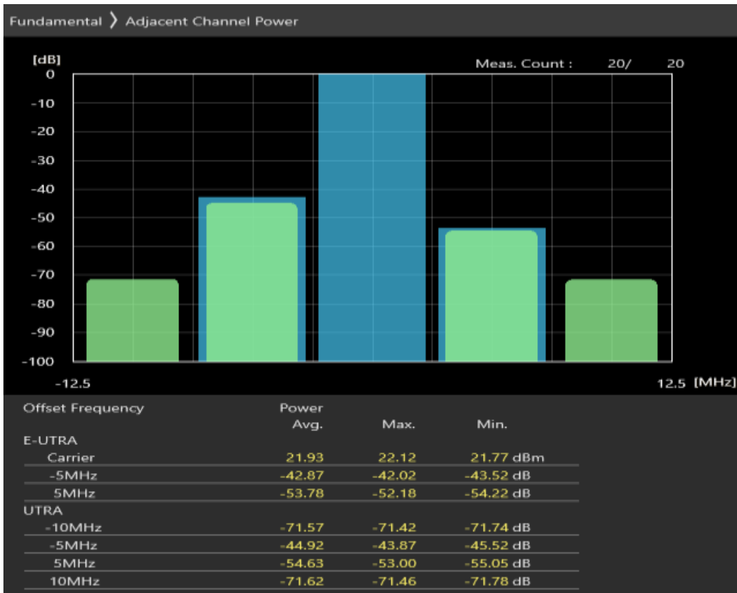
Band28 QAM16 BW=5MHz Channel=27235 RB Size=8 Position=#Max
