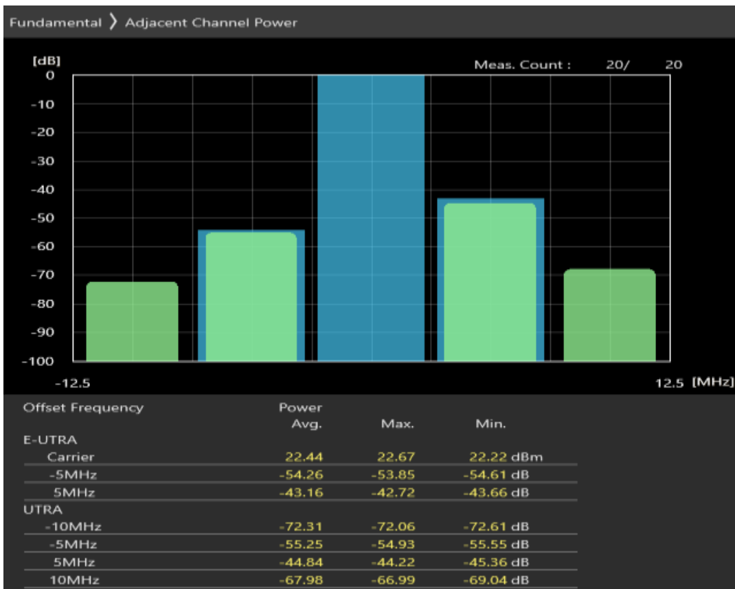
Band28 QAM16 BW=5MHz Channel=27385 RB Size=25 Position=#0
