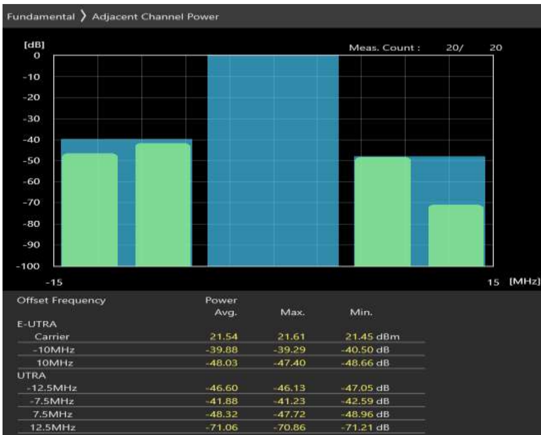
Band28 QAM16 BW=10MHz Channel=27610 RB Size=12 Position=#0
