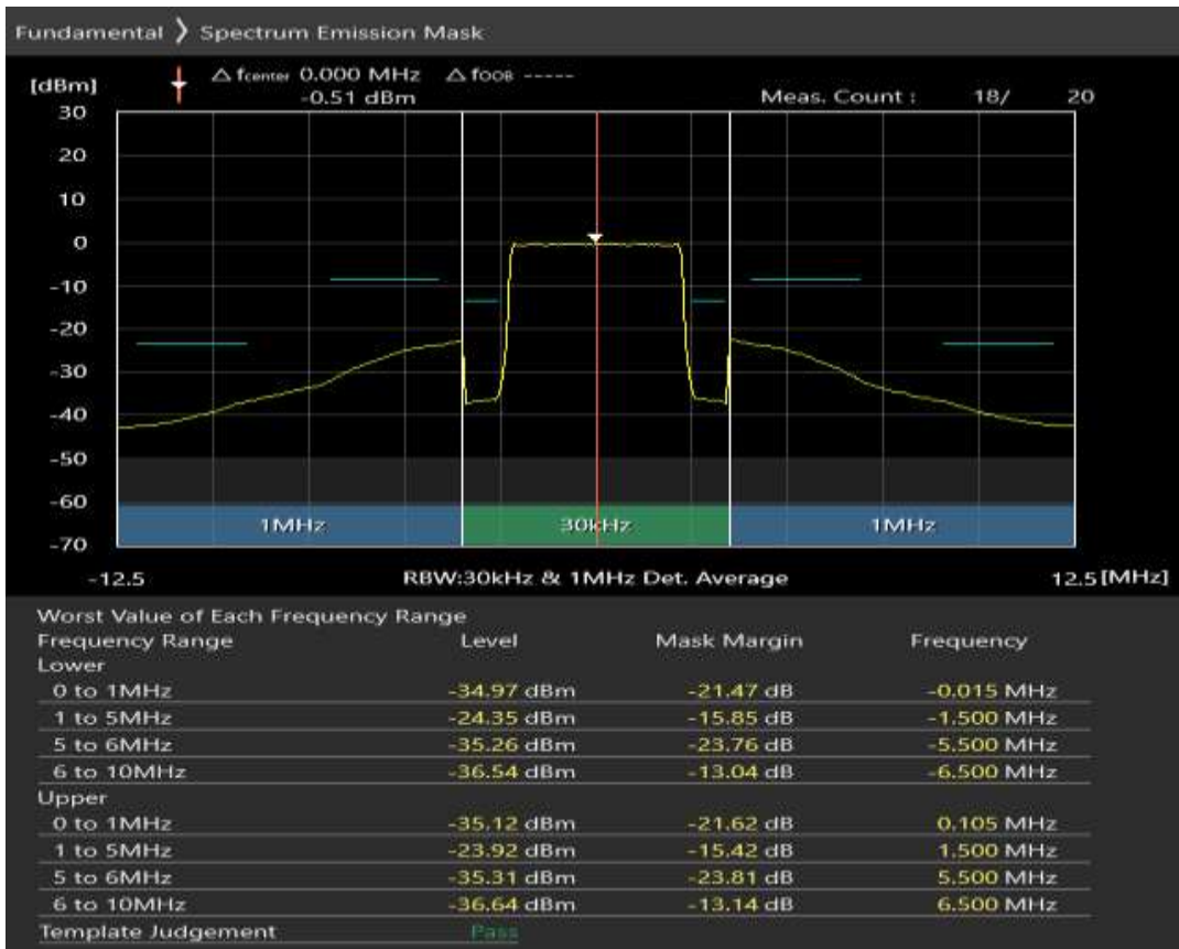
Band3 QPSK BW=5MHz Channel=19575 RB Size=8 Position=#0
