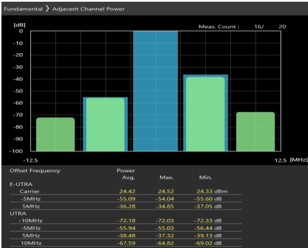
Band1 QPSK BW=5MHz Channel=18575 RB Size=25 Position=#0
