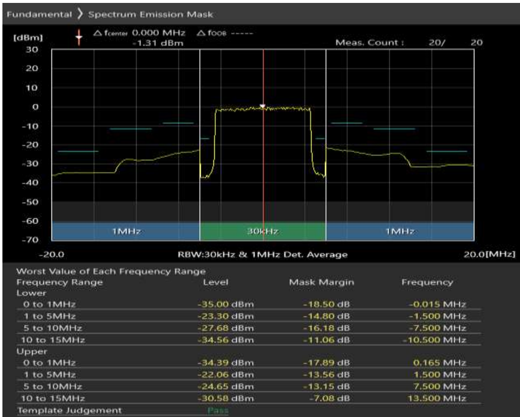
Band40 QAM16 BW=10MHz Channel=38700 RB Size=12 Position=#0
