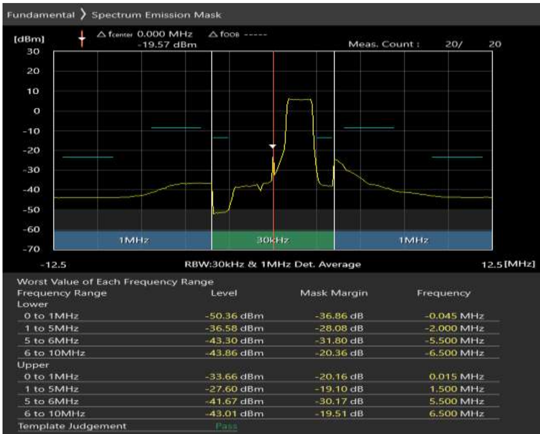
Band3 QPSK BW=5MHz Channel=19225 RB Size=25 Position=#0
