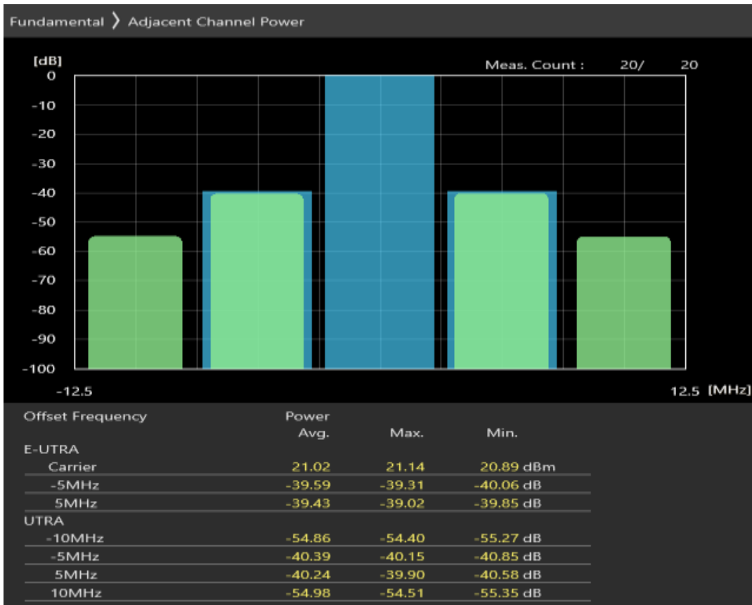
Band3 QPSK BW=5MHz Channel=19575 RB Size=8 Position=#0
