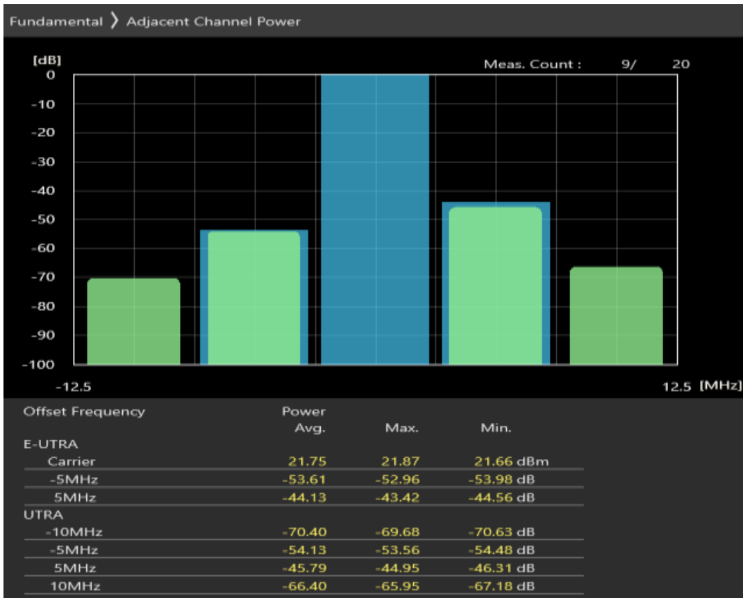
Band3 QPSK BW=5MHz Channel=19925 RB Size=25 Position=#0
