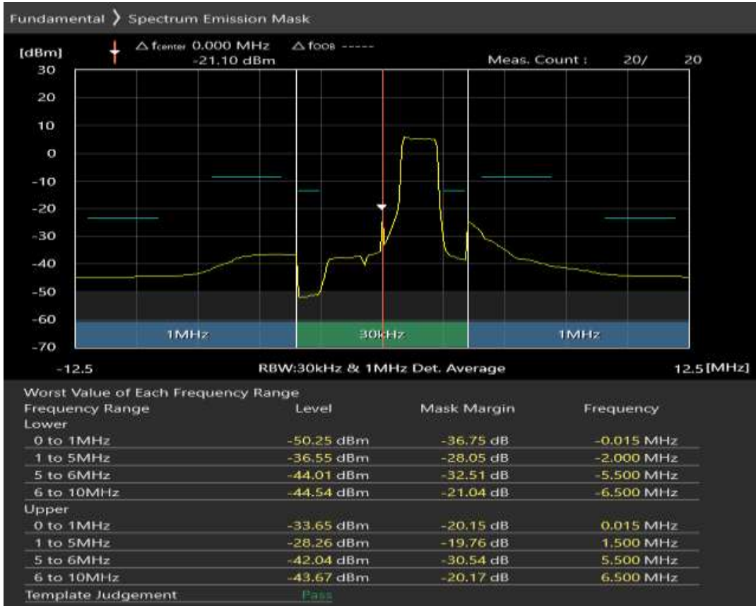
Band3 QPSK BW=5MHz Channel=19925 RB Size=25 Position=#0
