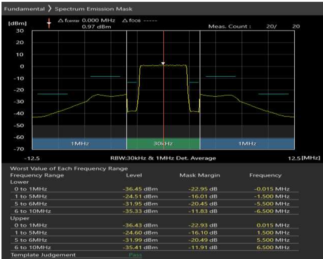
Band1 QAM16 BW=5MHz Channel=18025 RB Size=8 Position=#0
