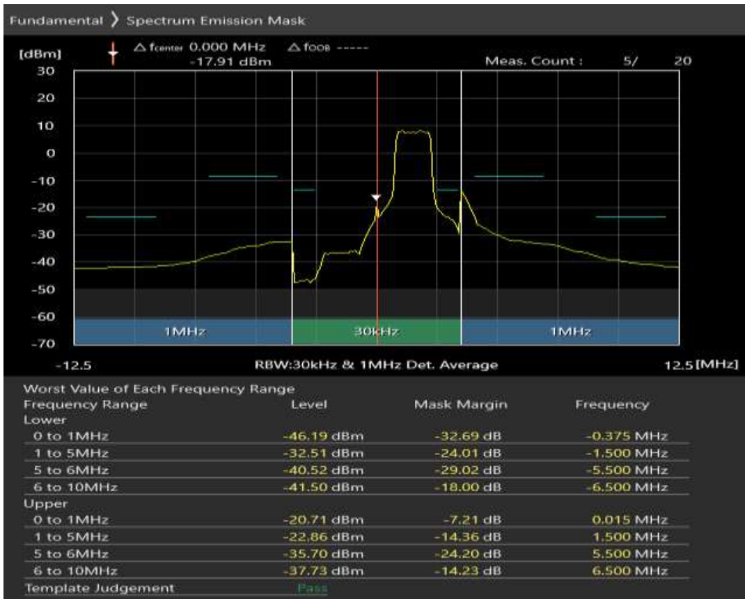
Band7 QPSK BW=5MHz Channel=21425 RB Size=25 Position=#0
