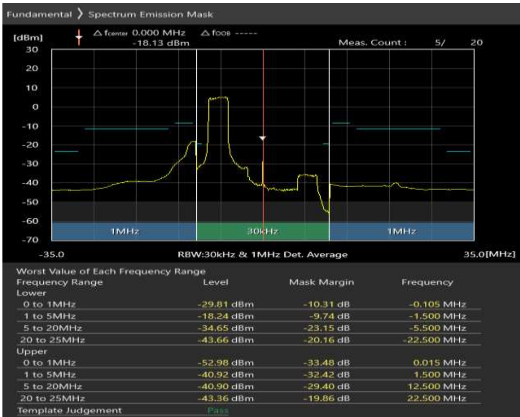
Band1 QPSK BW=20MHz Channel=18500 RB Size=18 Position=#Max
