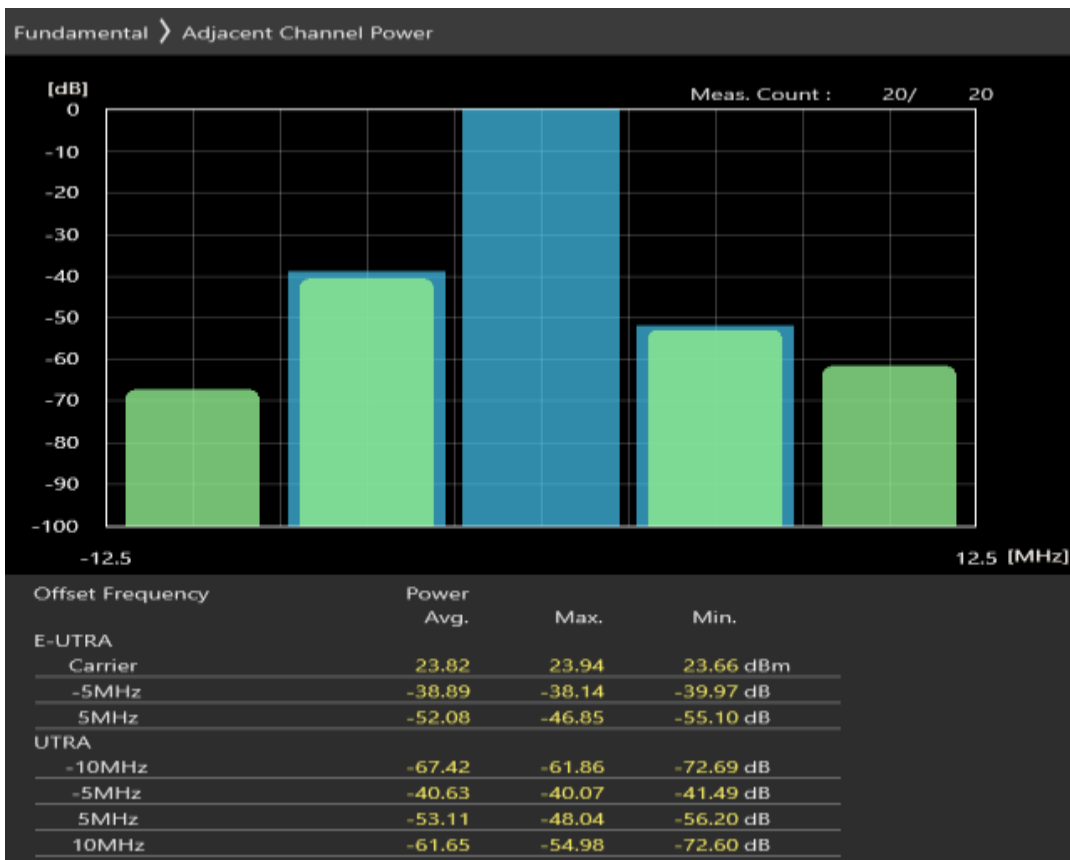
Band8 QPSK BW=5MHz Channel=21475 RB Size=8 Position=#Max
