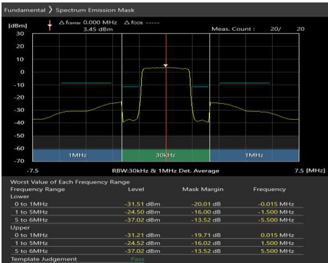
Band28 QAM16 BW=3MHz Channel=27360 RB Size=4 Position=#0
