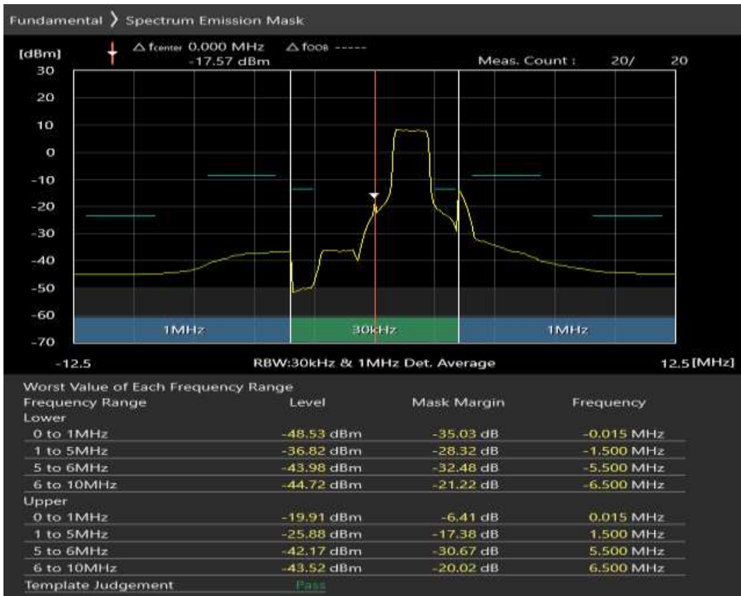
Band8 QPSK BW=5MHz Channel=21625 RB Size=25 Position=#0
