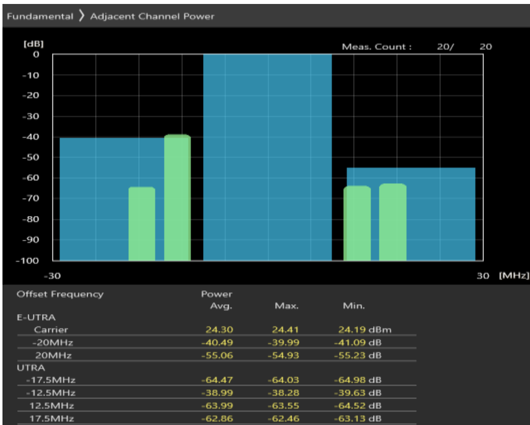
Band20 QPSK BW=20MHz Channel=24250 RB Size=18 Position=#Max
