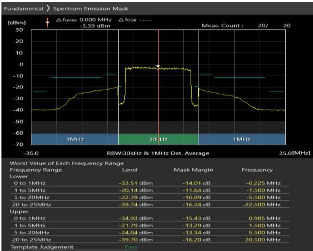
Band38 QAM16 BW=20MHz Channel=37850 RB Size=18 Position=#0
