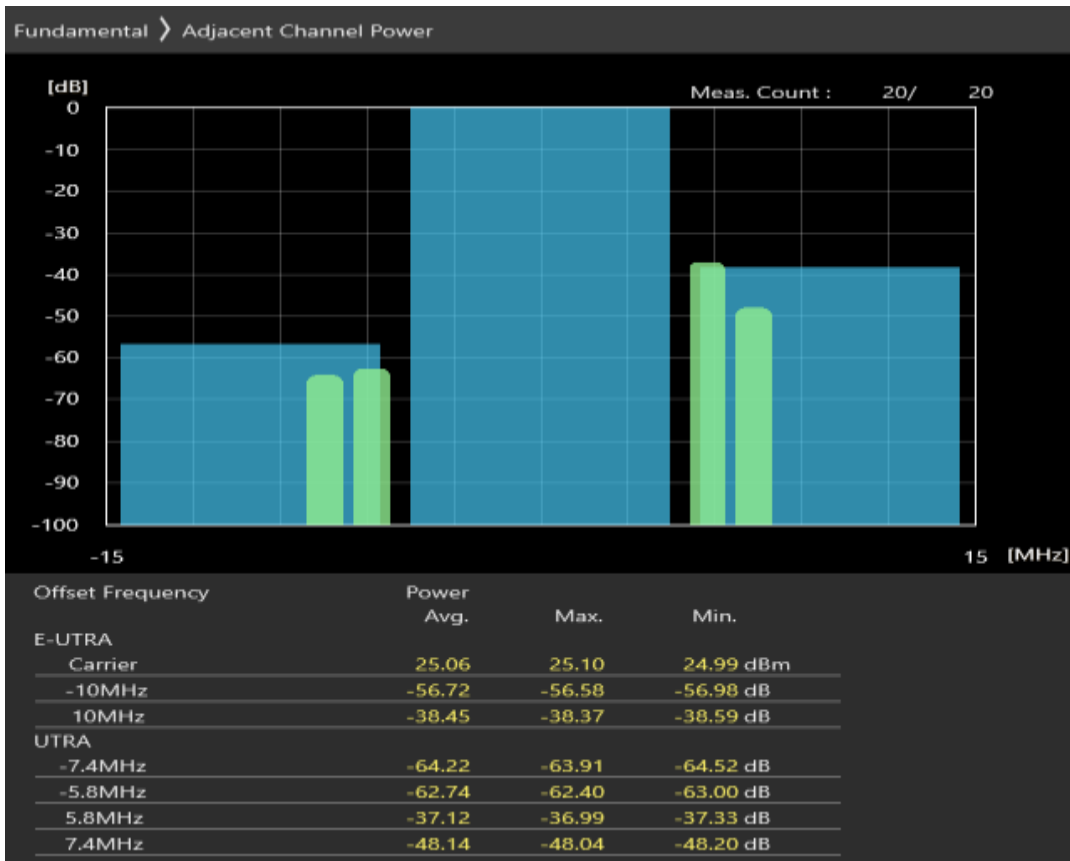
Band40 QPSK BW=10MHz Channel=39150 RB Size=50 Position=#0
