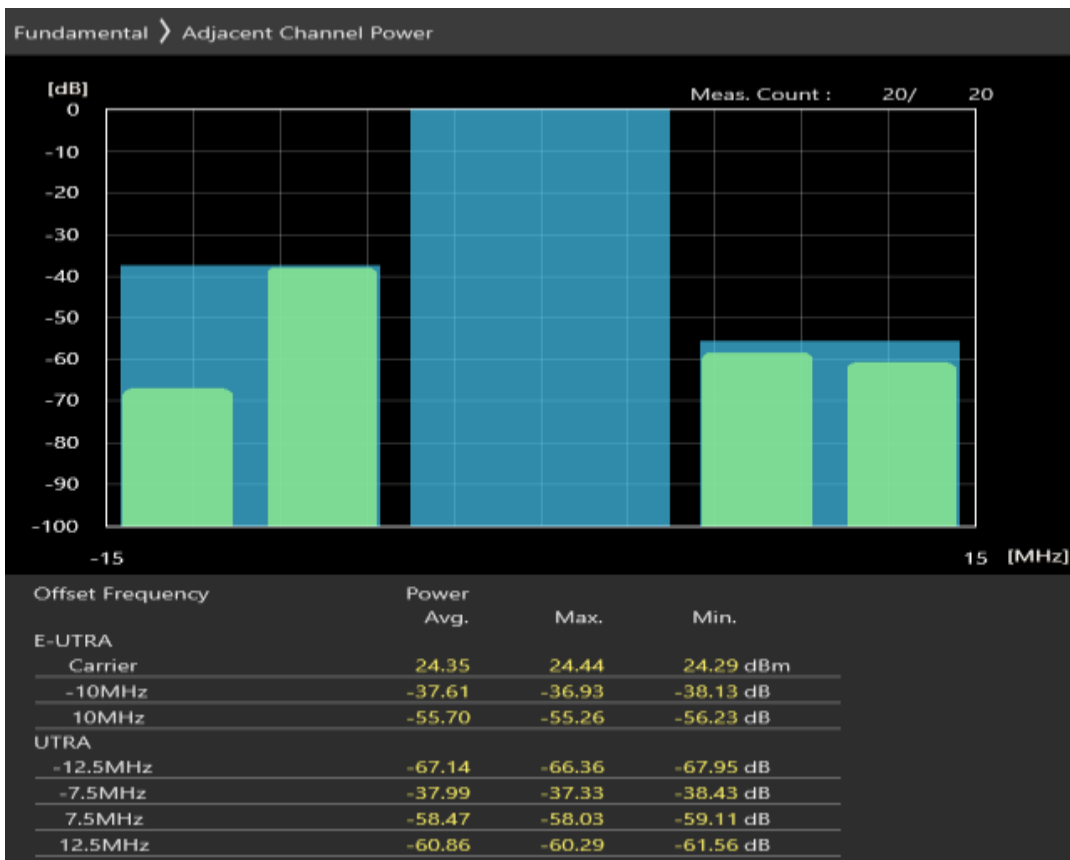
Band20 QPSK BW=10MHz Channel=24200 RB Size=12 Position=#Max
