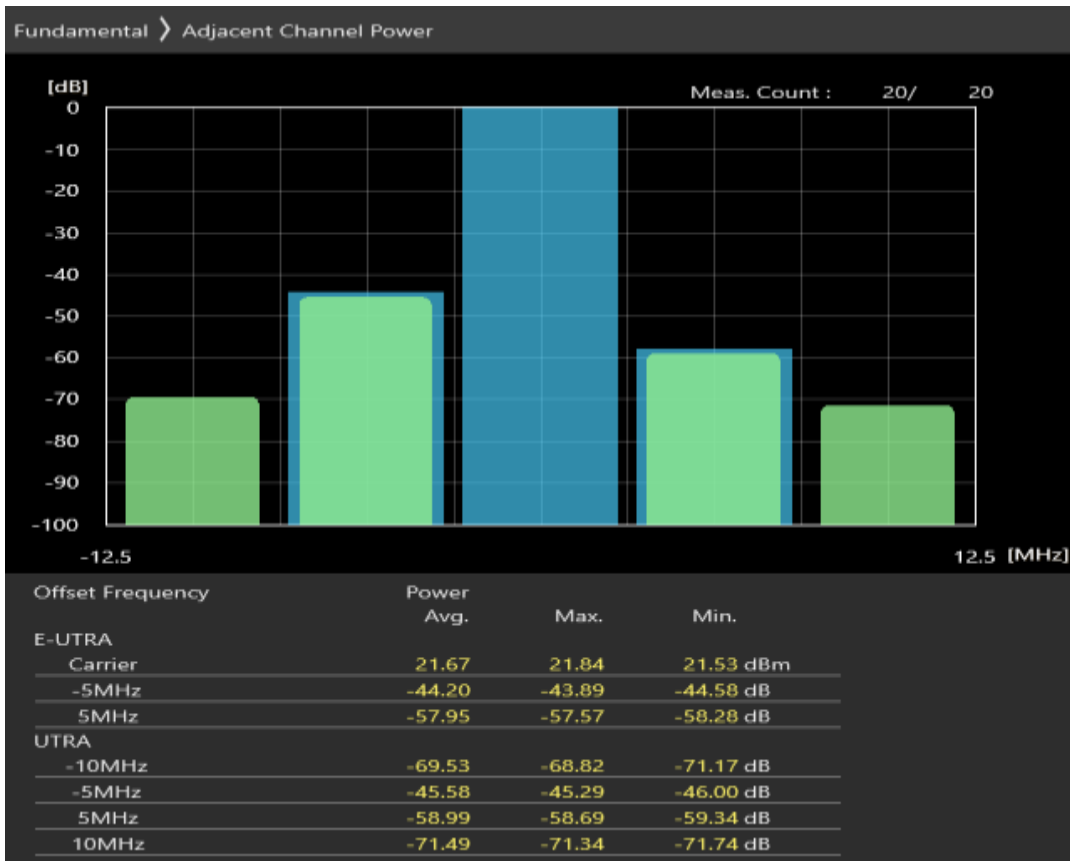
Band28 QAM16 BW=5MHz Channel=27635 RB Size=8 Position=#Max
