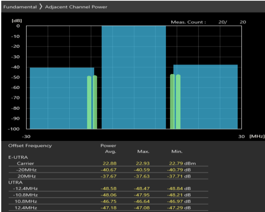
Band40 QPSK BW=20MHz Channel=39150 RB Size=18 Position=#0
