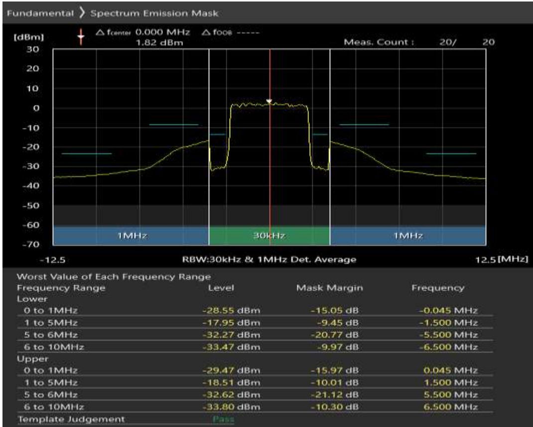
Band38 QPSK BW=5MHz Channel=38225 RB Size=8 Position=#0
