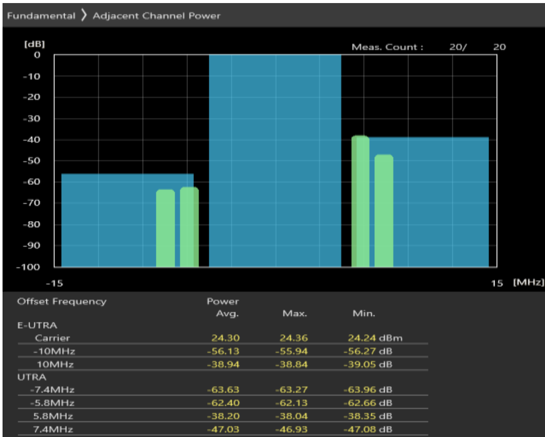
Band40 QAM16 BW=10MHz Channel=39150 RB Size=50 Position=#0
