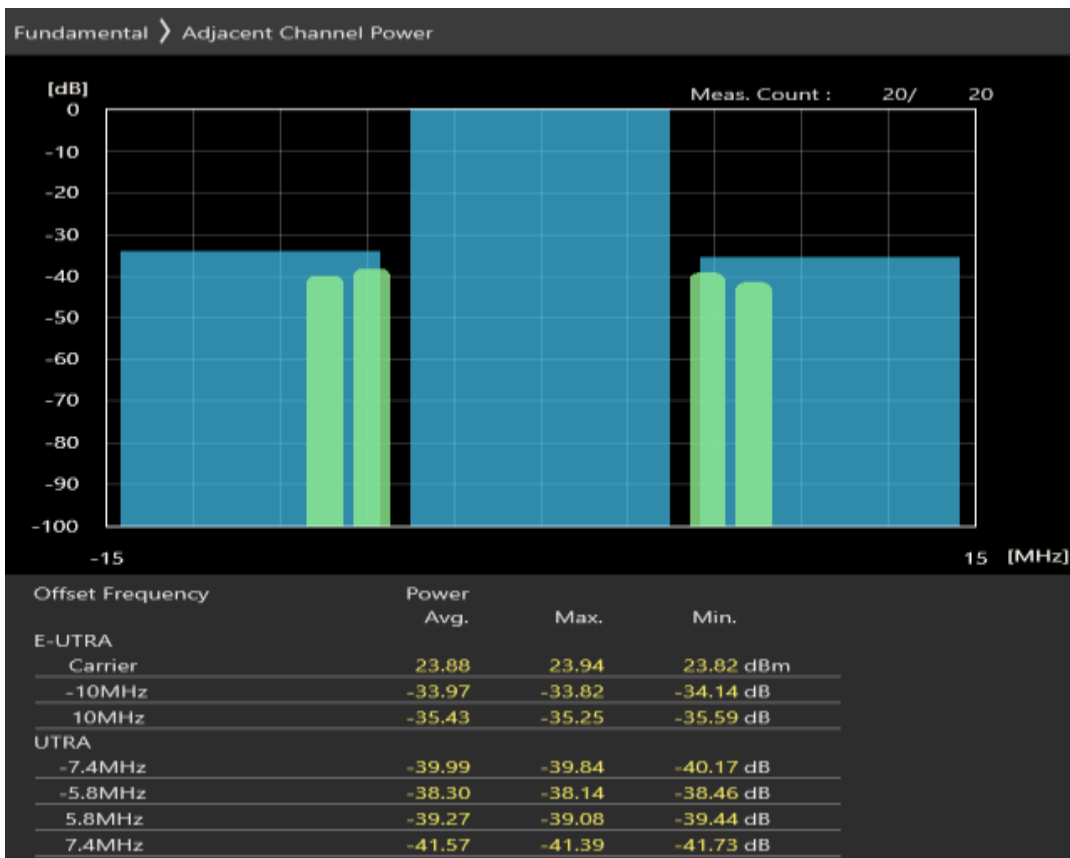
Band40 QAM16 BW=10MHz Channel=39600 RB Size=12 Position=#0
