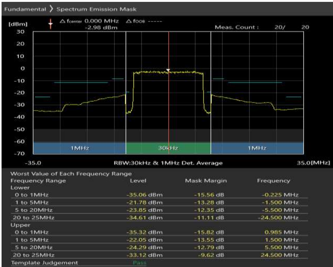
Band40 QAM16 BW=20MHz Channel=39150 RB Size=18 Position=#0
