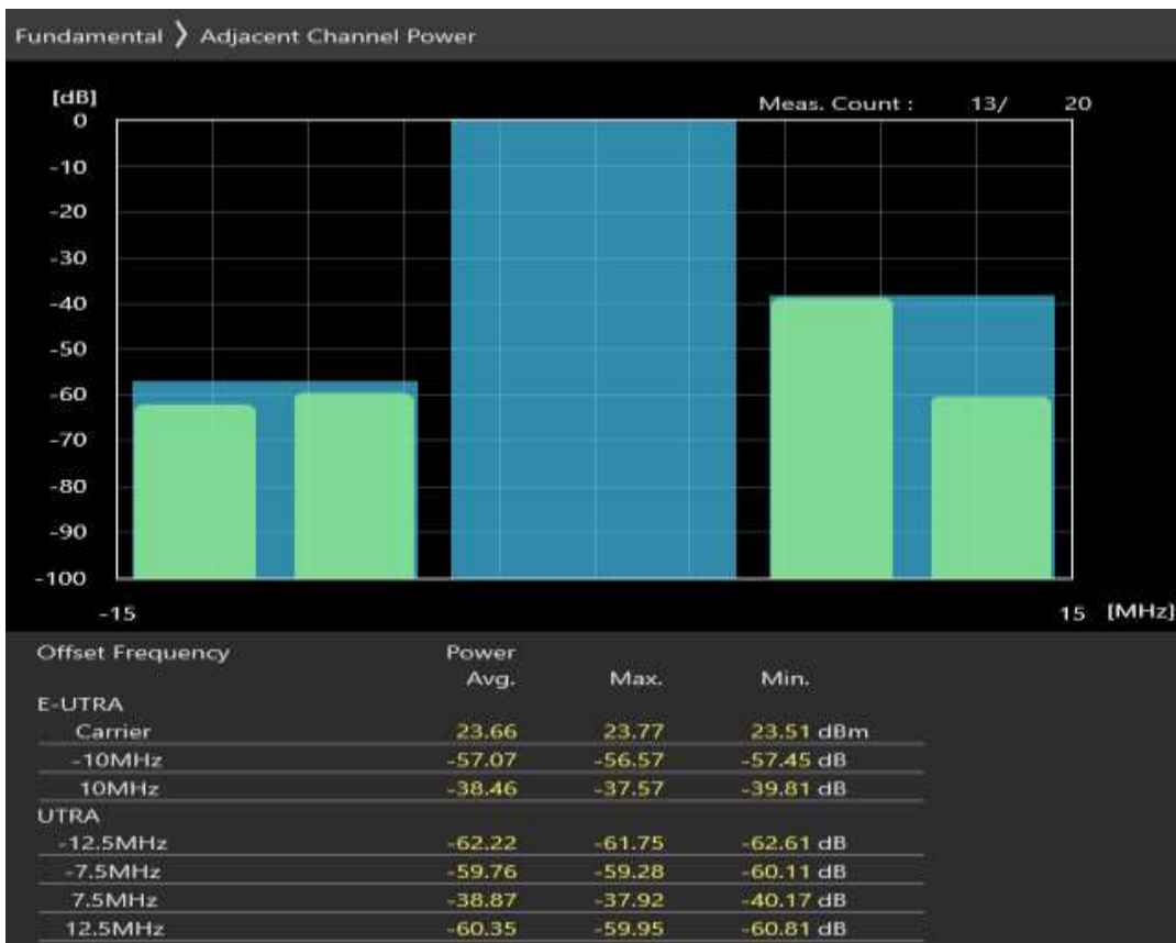
Band1 QAM16 BW=10MHz Channel=18550 RB Size=50 Position=#0
