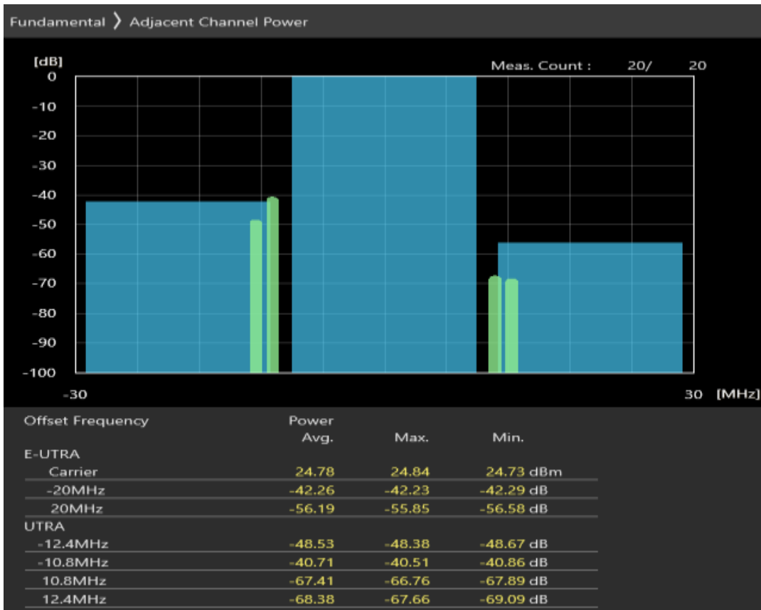
Band40 QPSK BW=20MHz Channel=39150 RB Size=18 Position=#Max
