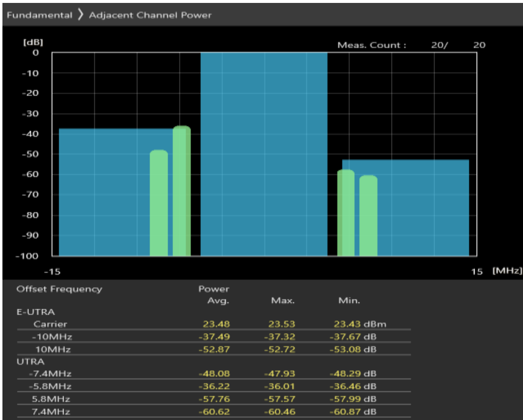
Band38 QAM16 BW=10MHz Channel=38200 RB Size=12 Position=#Max
