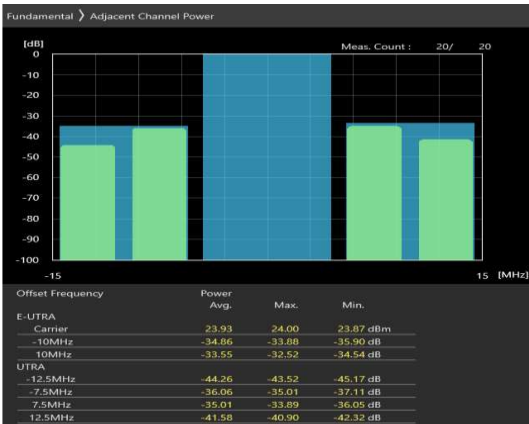
Band7 QAM16 BW=10MHz Channel=20800 RB Size=12 Position=#0
