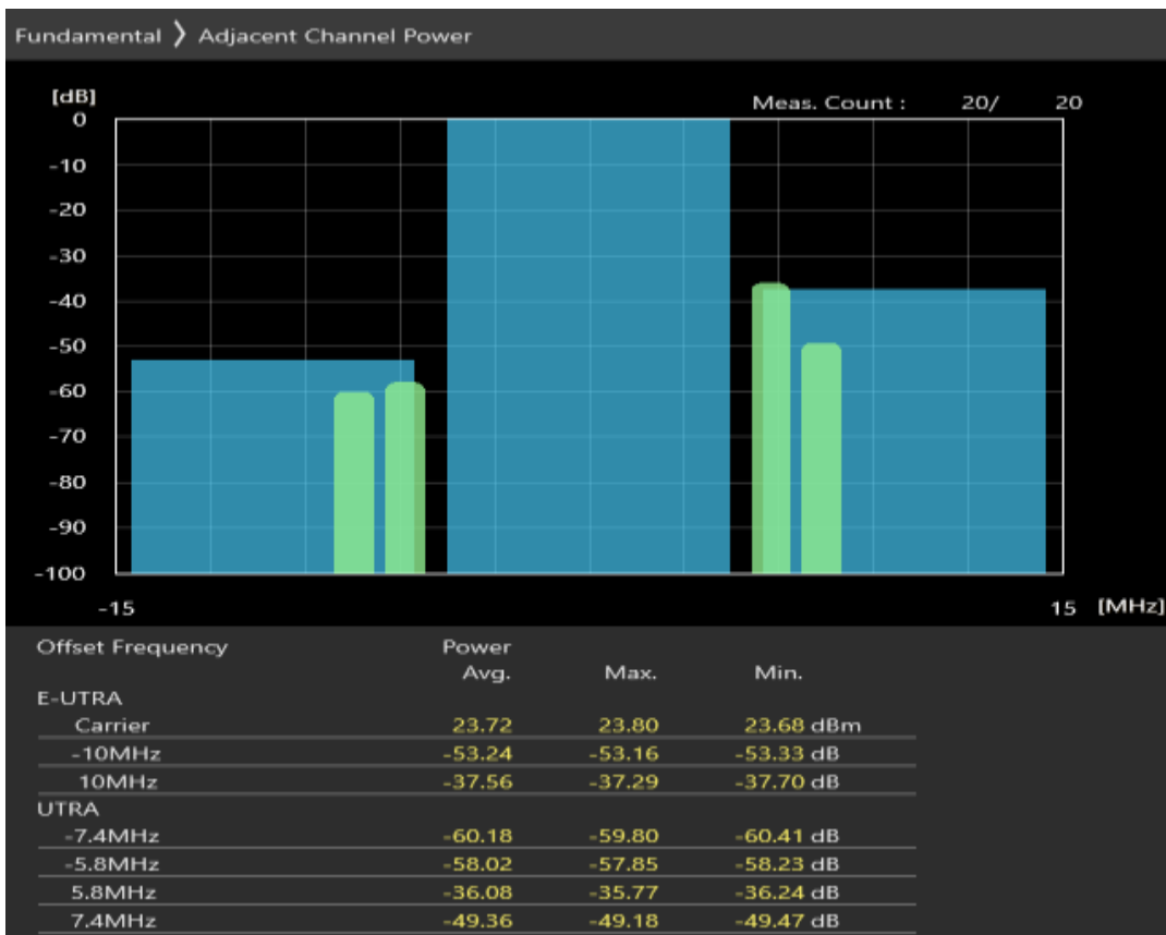
Band38 QAM16 BW=10MHz Channel=38000 RB Size=50 Position=#0
