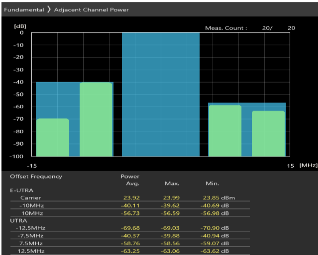
Band8 QPSK BW=10MHz Channel=21500 RB Size=12 Position=#Max
