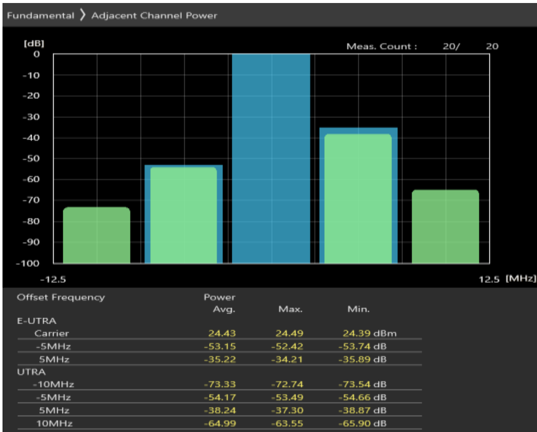
Band20 QPSK BW=5MHz Channel=24300 RB Size=25 Position=#0
