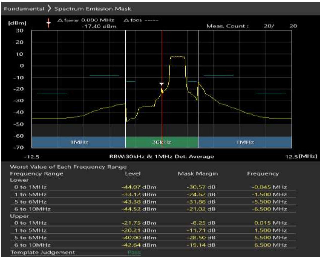
Band20 QPSK BW=5MHz Channel=24425 RB Size=25 Position=#0
