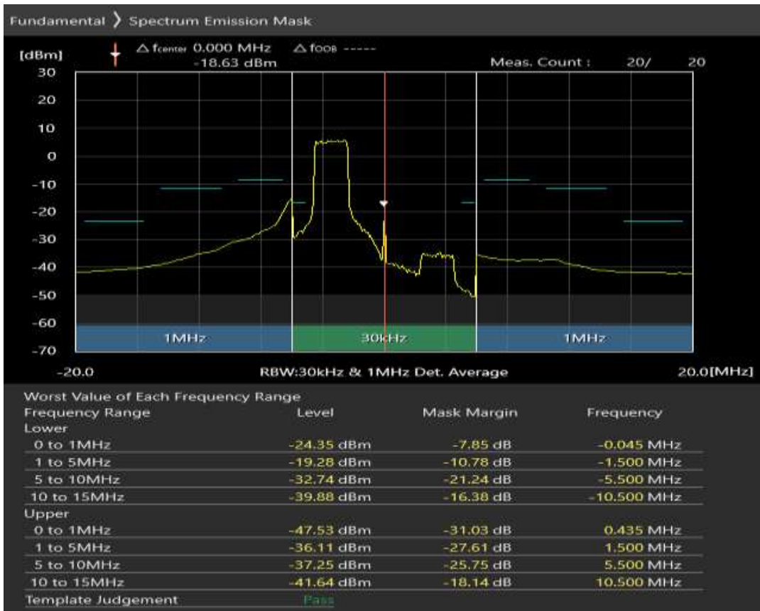
Band38 QAM16 BW=10MHz Channel=38200 RB Size=12 Position=#Max
