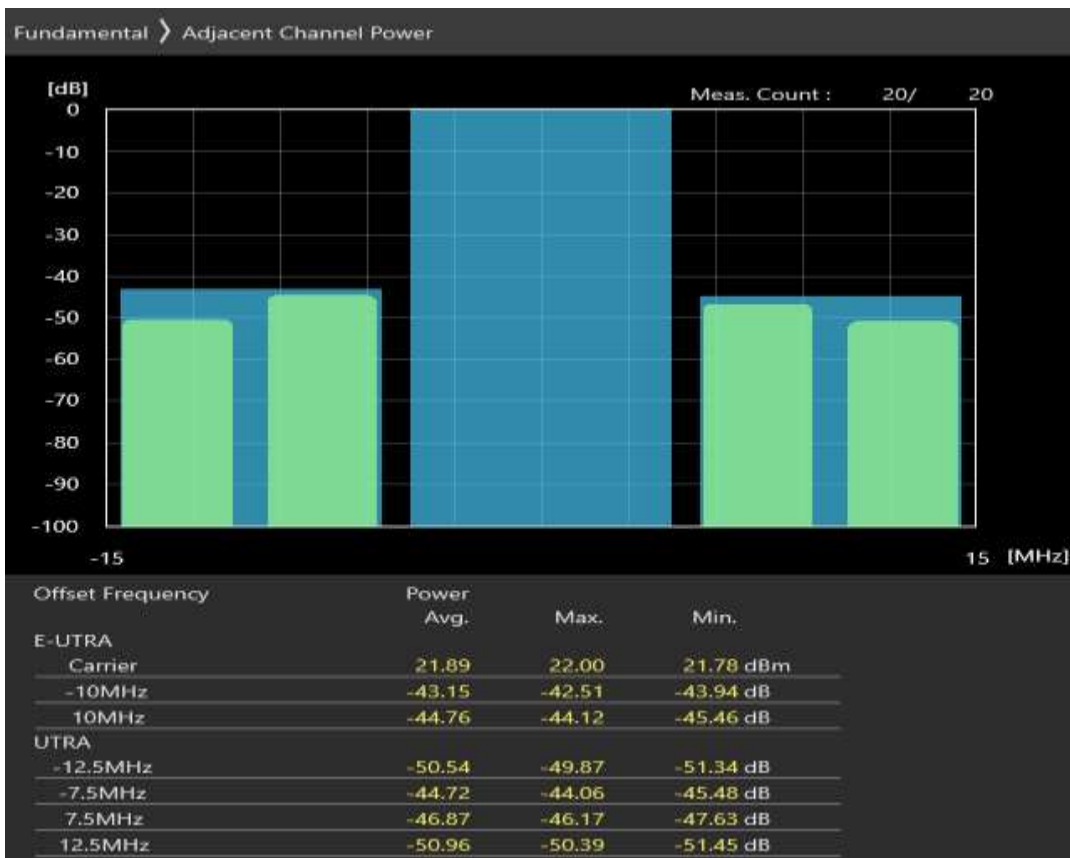
Band8 QAM16 BW=10MHz Channel=21750 RB Size=12 Position=#0
