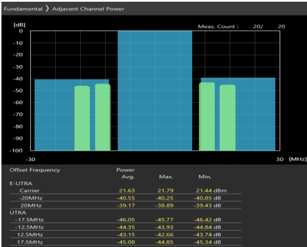
Band1 QPSK BW=20MHz Channel=18300 RB Size=18 Position=#0
