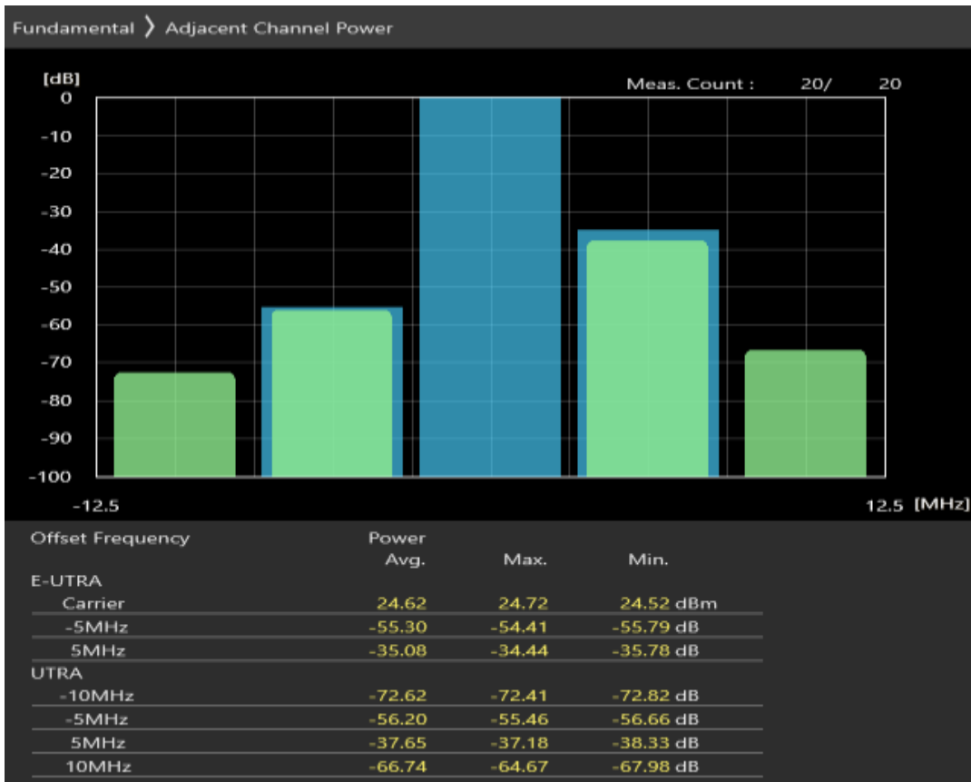
Band1 QPSK BW=5MHz Channel=18025 RB Size=25 Position=#0
