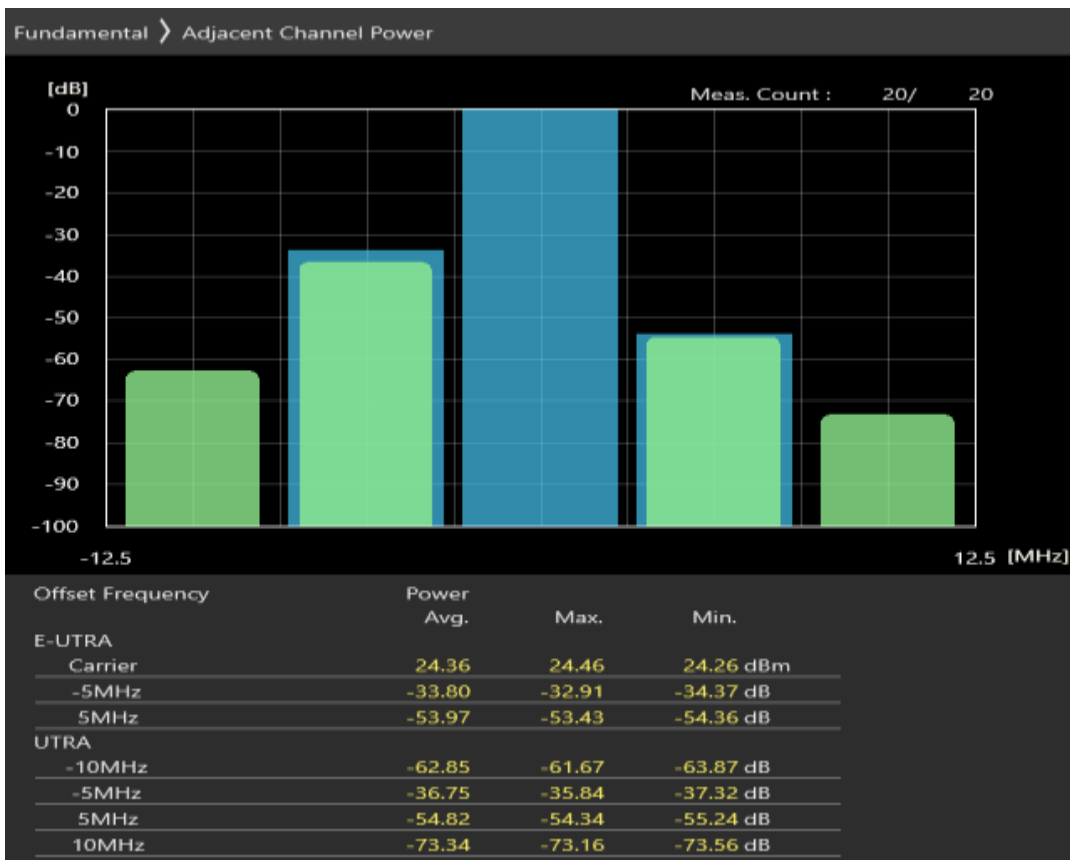
Band20 QPSK BW=5MHz Channel=24425 RB Size=8 Position=#Max
