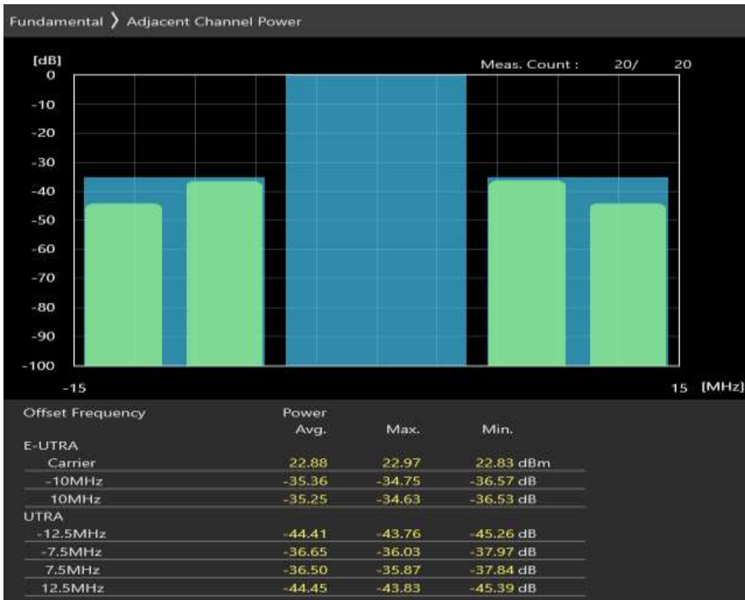
Band7 QPSK BW=20MHz Channel=20850 RB Size=18 Position=#0
