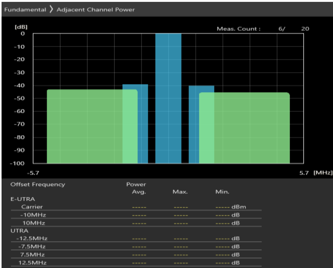
Band8 QPSK BW=1.4MHz Channel=21457 RB Size=5 Position=#Max
