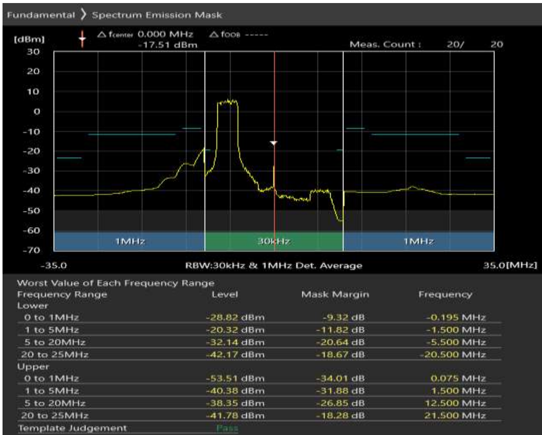
Band40 QPSK BW=20MHz Channel=39150 RB Size=18 Position=#Max
