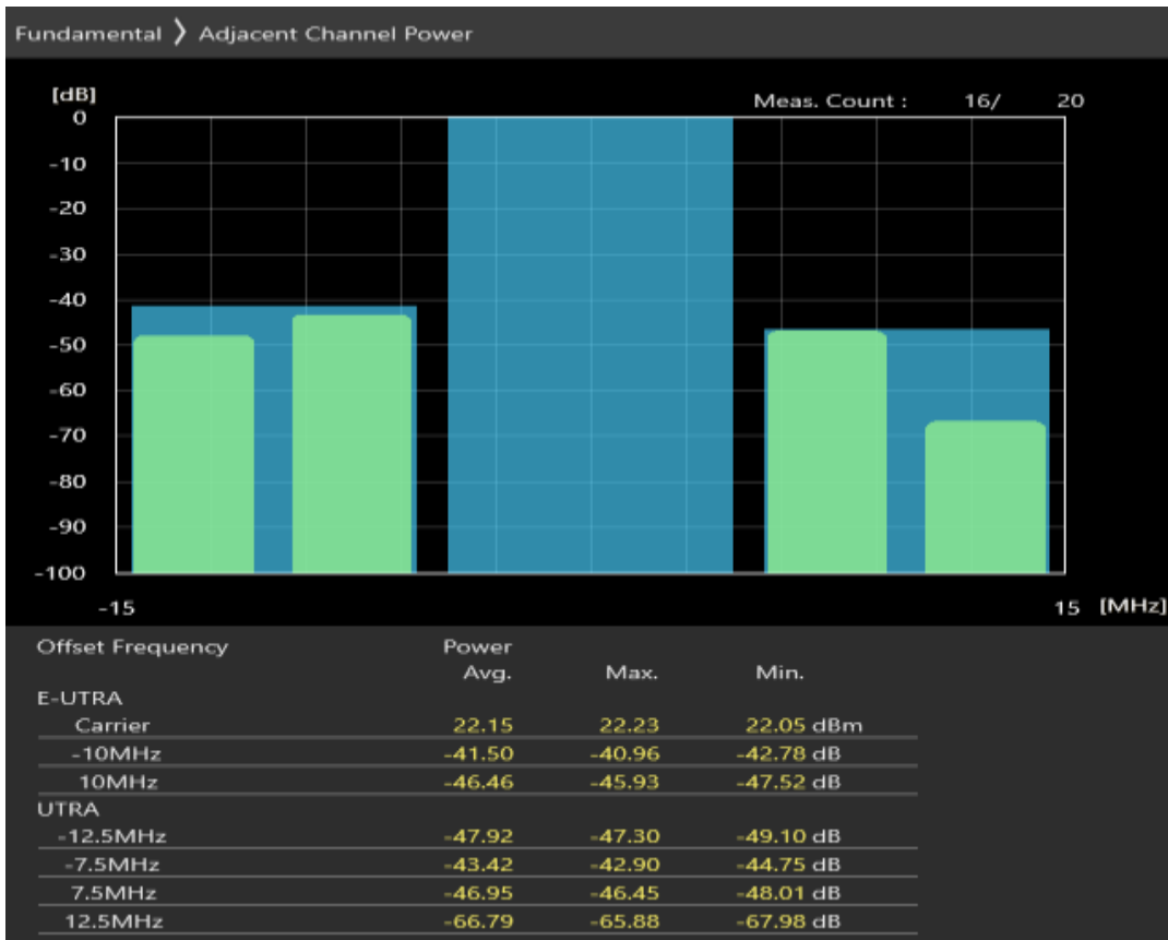
Band8 QAM16 BW=5MHz Channel=21475 RB Size=25 Position=#0
