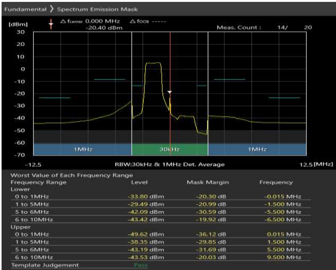
Band3 QAM16 BW=5MHz Channel=19575 RB Size=8 Position=#Max
