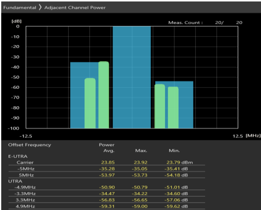
Band40 QAM16 BW=5MHz Channel=39625 RB Size=8 Position=#Max
