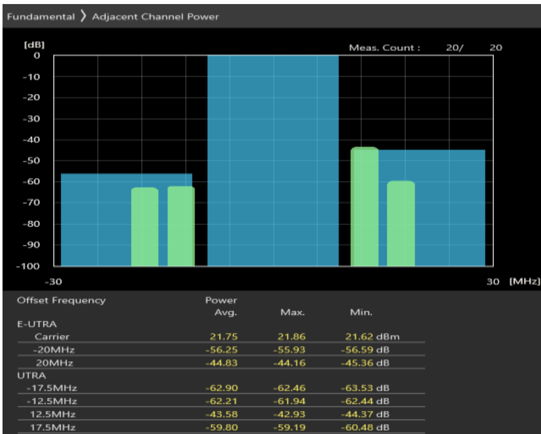
Band20 QAM16 BW=20MHz Channel=24350 RB Size=100 Position=#
