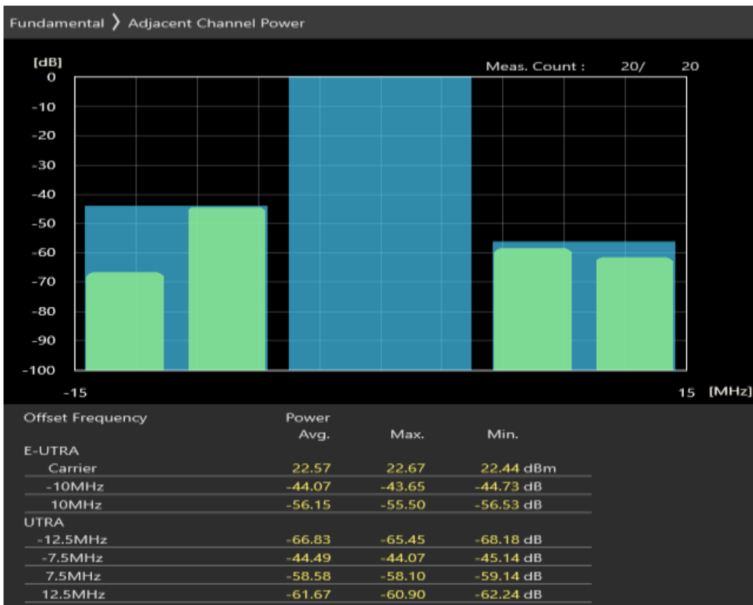
Band28 QPSK BW=10MHz Channel=27260 RB Size=12 Position=#Max
