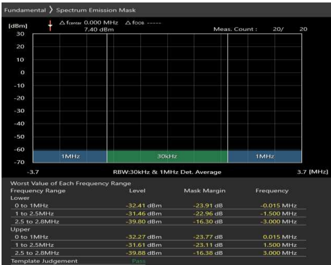
Band3 QAM16 BW=1.4MHz Channel=19575 RB Size=5 Position=#0
