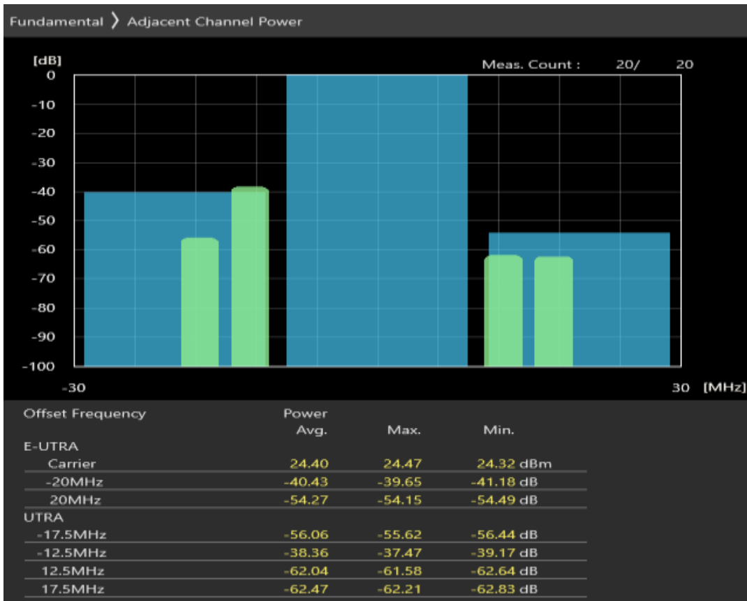
Band7 QPSK BW=20MHz Channel=21100 RB Size=100 Position=#0
