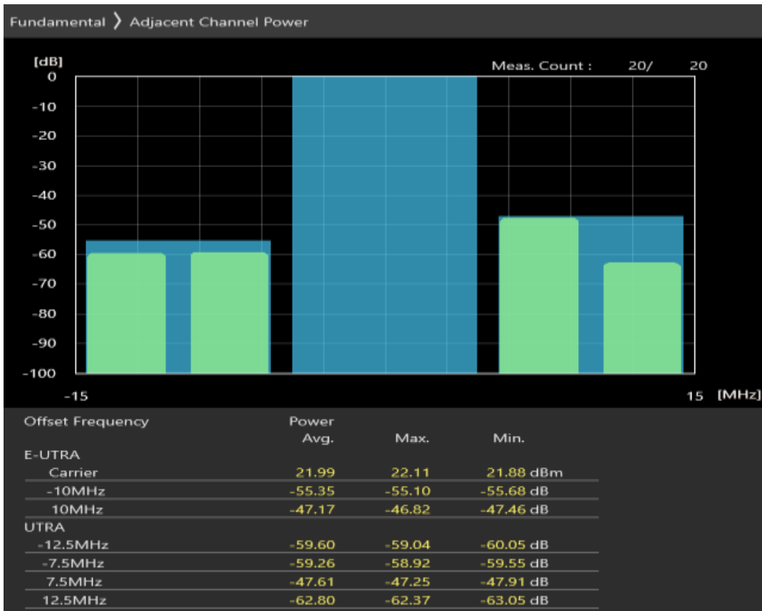
Band3 QPSK BW=10MHz Channel=19575 RB Size=50 Position=#0
