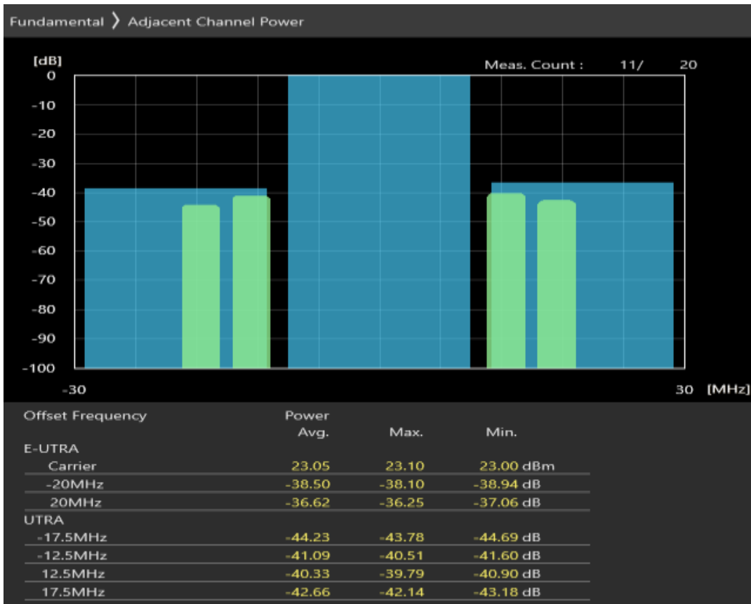
Band7 QPSK BW=20MHz Channel=21100 RB Size=18 Position=#0
