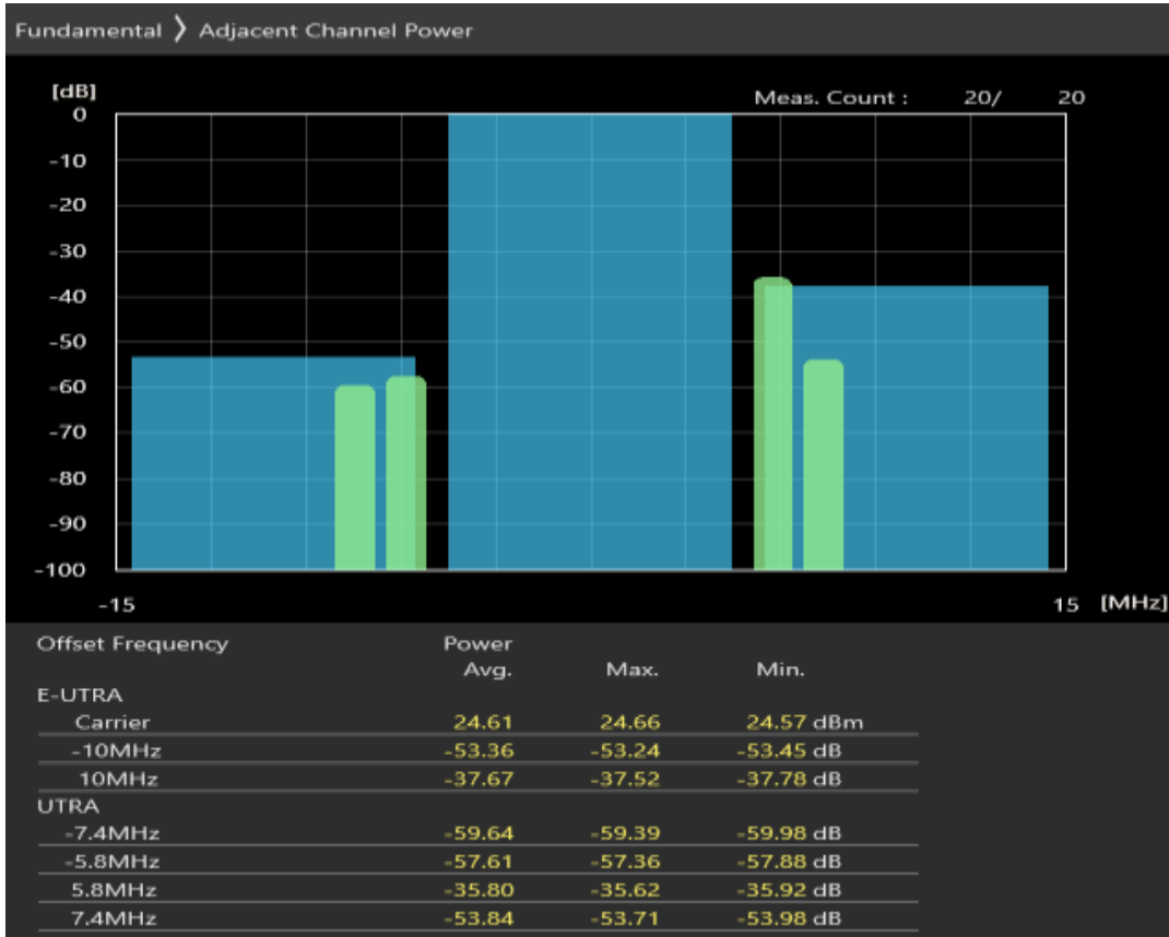
Band38 QPSK BW=10MHz Channel=37800 RB Size=50 Position=#0
