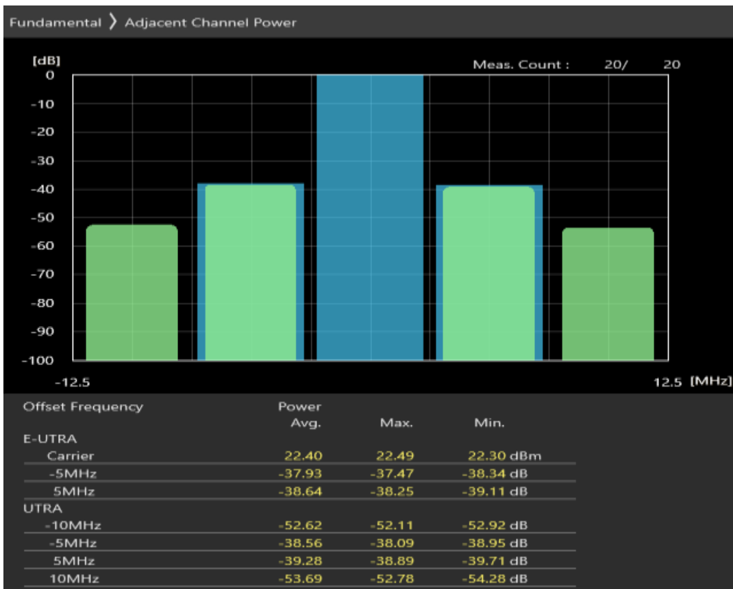
Band1 QAM16 BW=5MHz Channel=18300 RB Size=8 Position=#0
