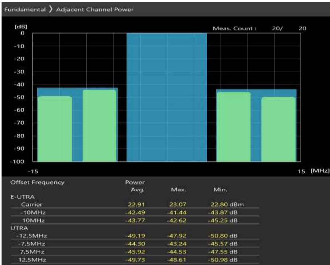
Band8 QPSK BW=10MHz Channel=21750 RB Size=12 Position=#0
