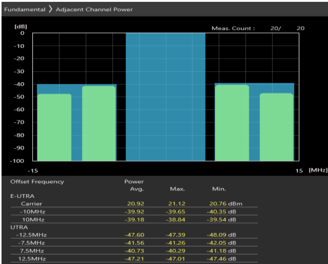
Band3 QPSK BW=10MHz Channel=19575 RB Size=12 Position=#0
