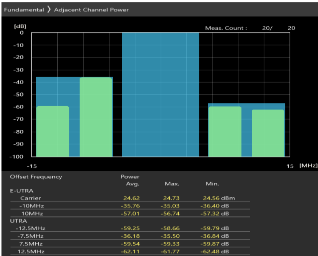
Band1 QPSK BW=10MHz Channel=18050 RB Size=12 Position=#Max
