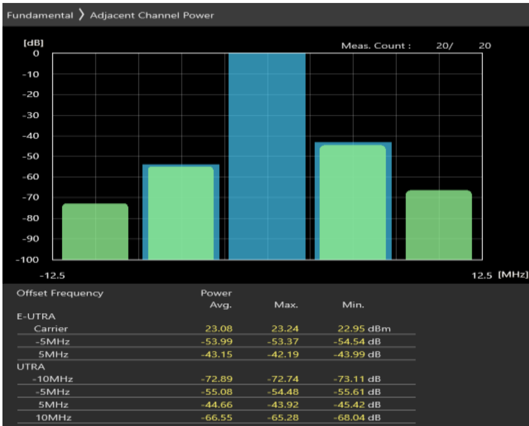
Band28 QPSK BW=5MHz Channel=27385 RB Size=25 Position=#0
