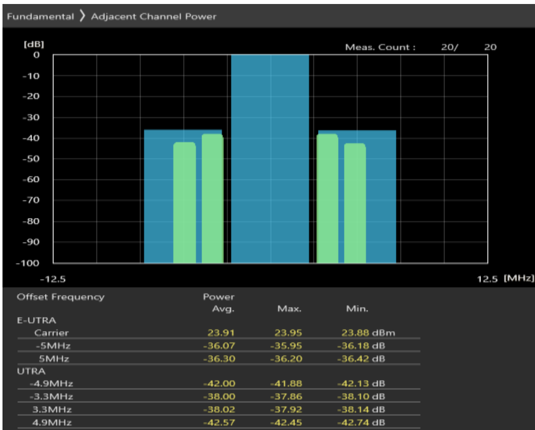
Band38 QAM16 BW=5MHz Channel=37775 RB Size=8 Position=#0
