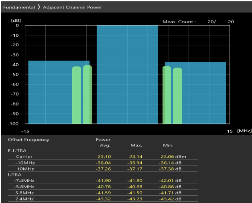
Band38 QPSK BW=10MHz Channel=38200 RB Size=12 Position=#0
