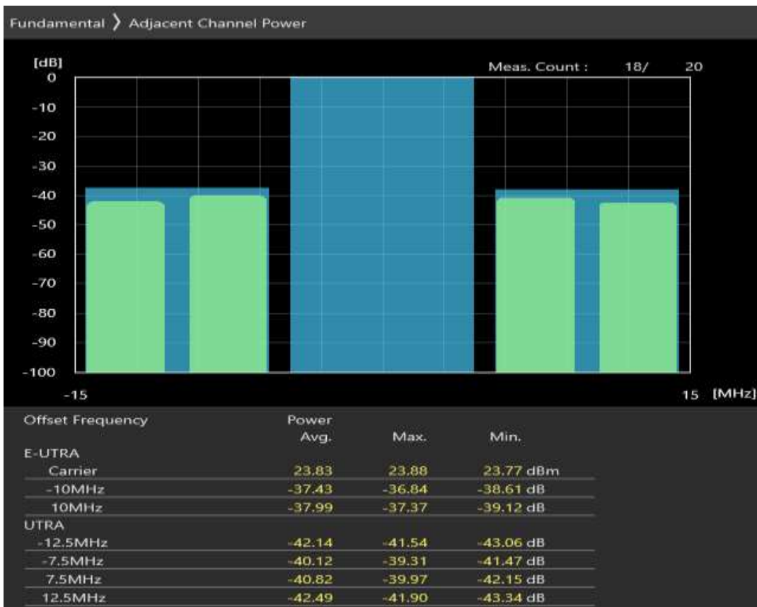
Band1 QAM16 BW=10MHz Channel=18550 RB Size=12 Position=#0
