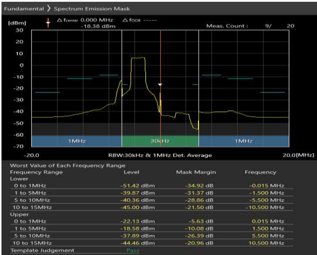
Band8 QPSK BW=10MHz Channel=21625 RB Size=50 Position=#0
