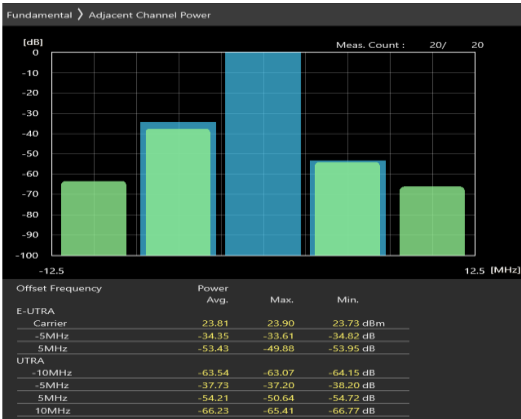
Band7 QAM16 BW=5MHz Channel=20775 RB Size=8 Position=#Max
