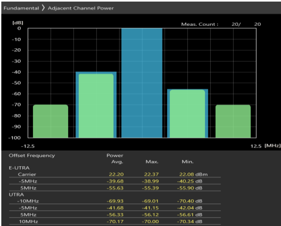
Band1 QAM16 BW=5MHz Channel=18025 RB Size=8 Position=#Max
