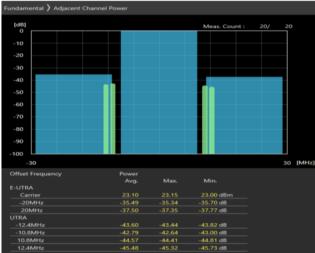
Band38 QPSK BW=20MHz Channel=38150 RB Size=18 Position=#0
