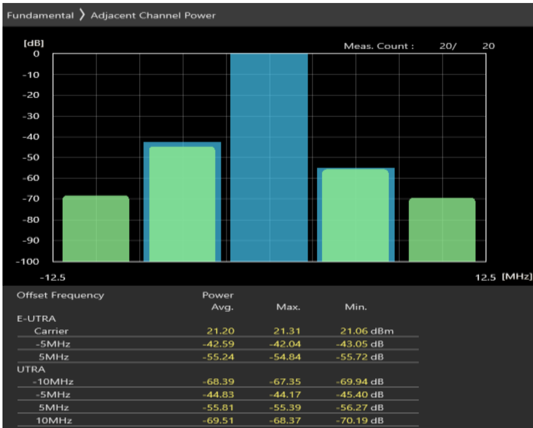
Band3 QAM16 BW=5MHz Channel=19925 RB Size=8 Position=#Max
