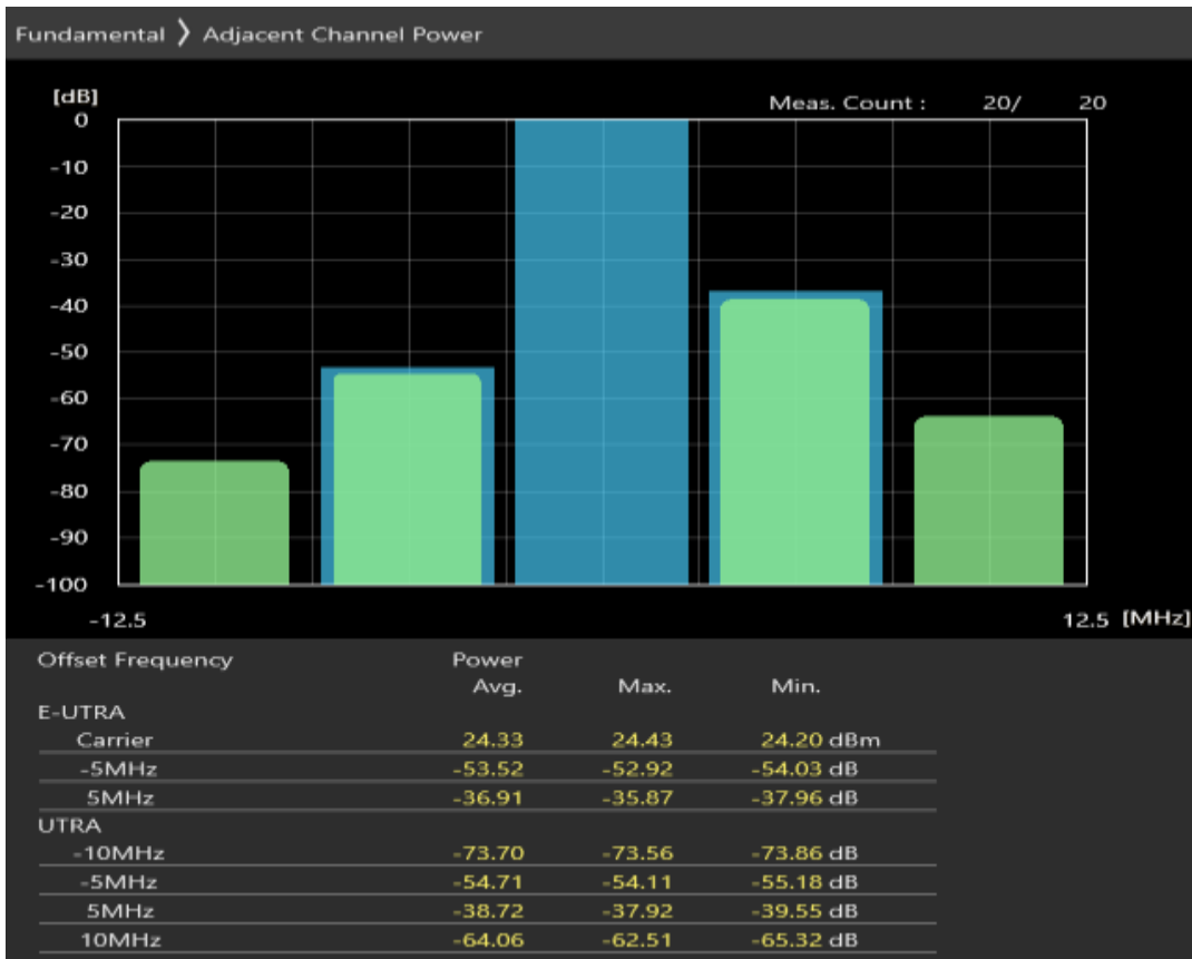
Band20 QPSK BW=5MHz Channel=24175 RB Size=25 Position=#0
