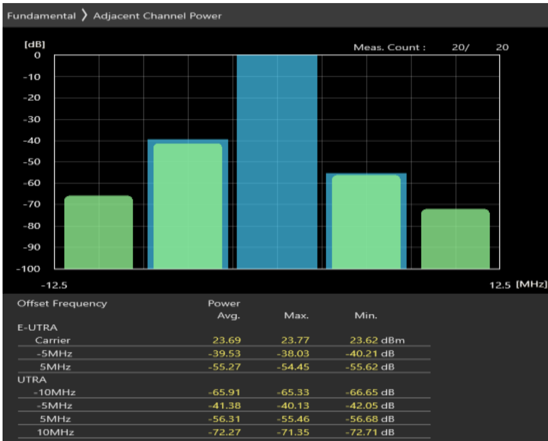
Band8 QPSK BW=5MHz Channel=21625 RB Size=8 Position=#Max
