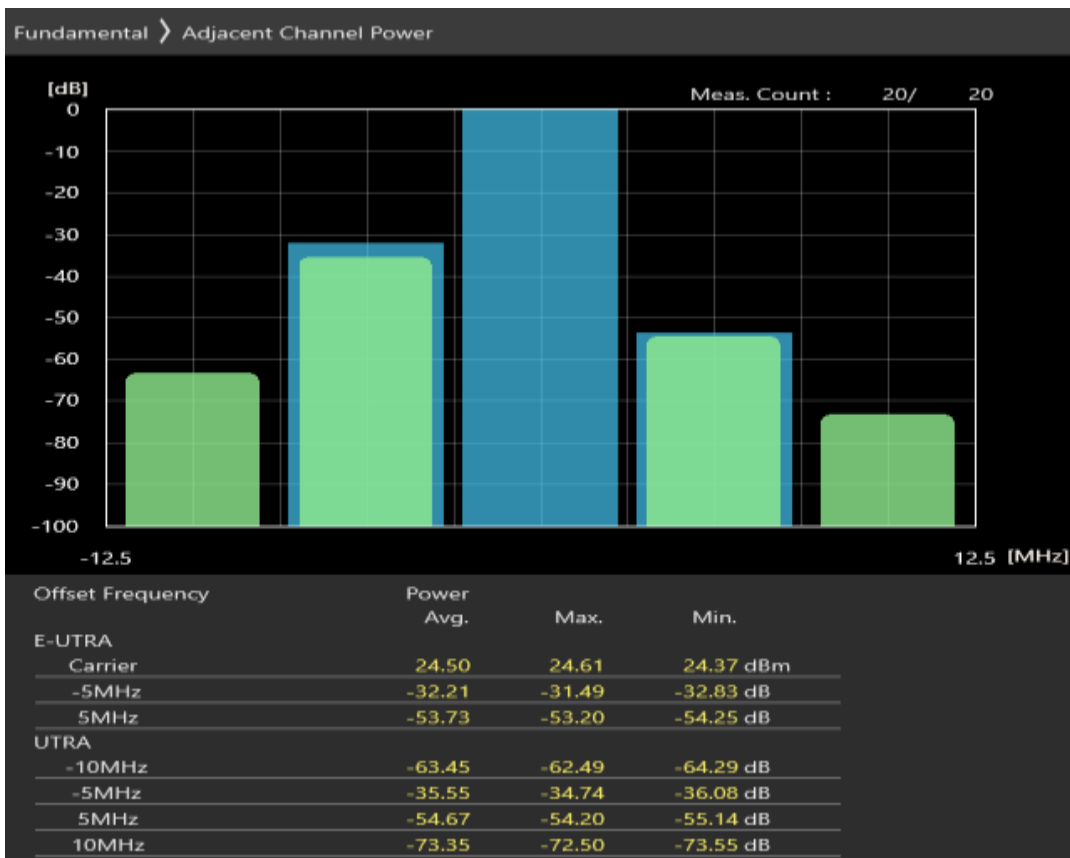
Band20 QPSK BW=5MHz Channel=24300 RB Size=8 Position=#Max
