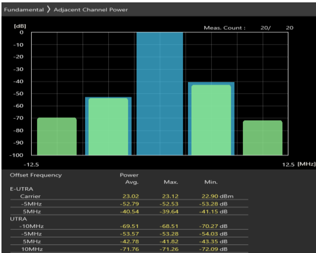
Band8 QPSK BW=1.4MHz Channel=21457 RB Size=5 Position=#0
