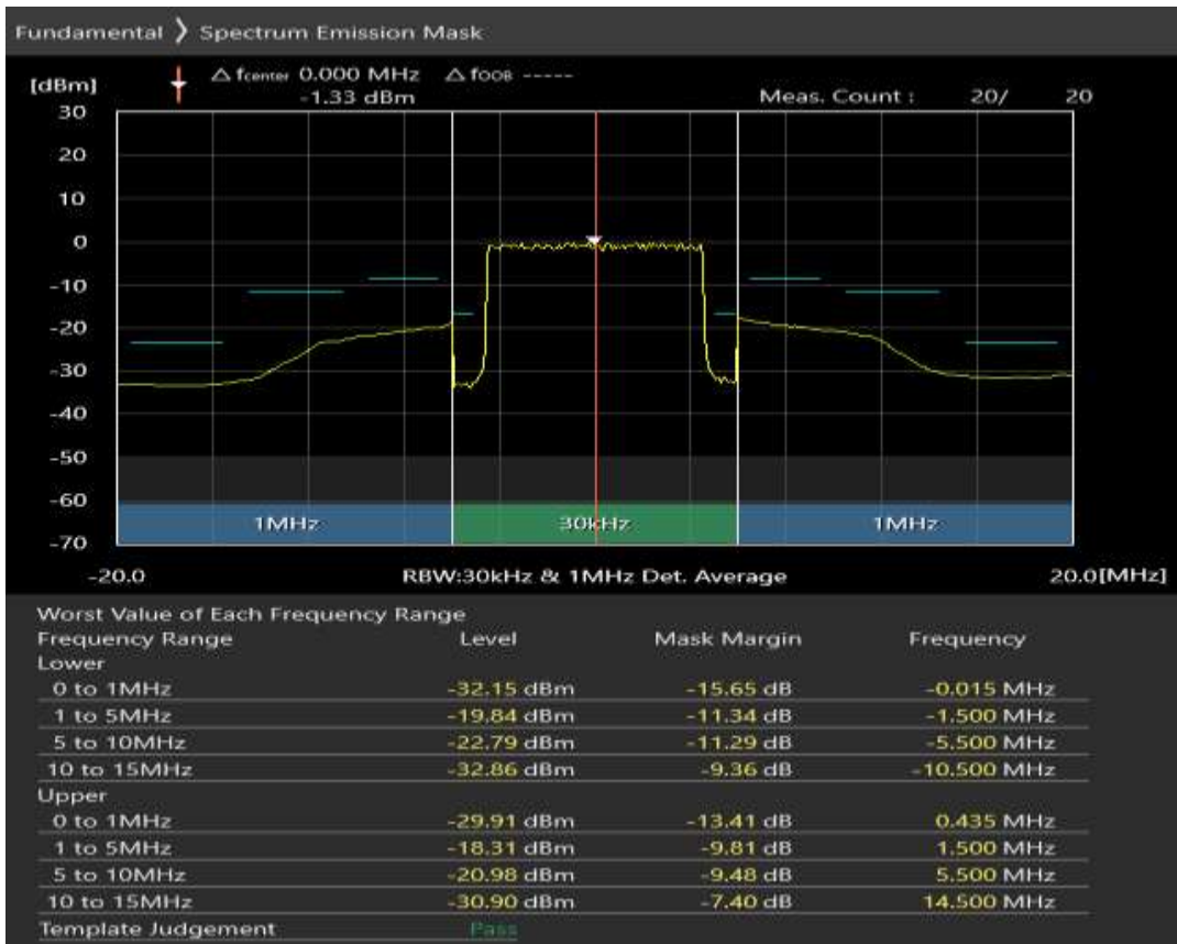
Band38 QAM16 BW=10MHz Channel=38200 RB Size=12 Position=#0
