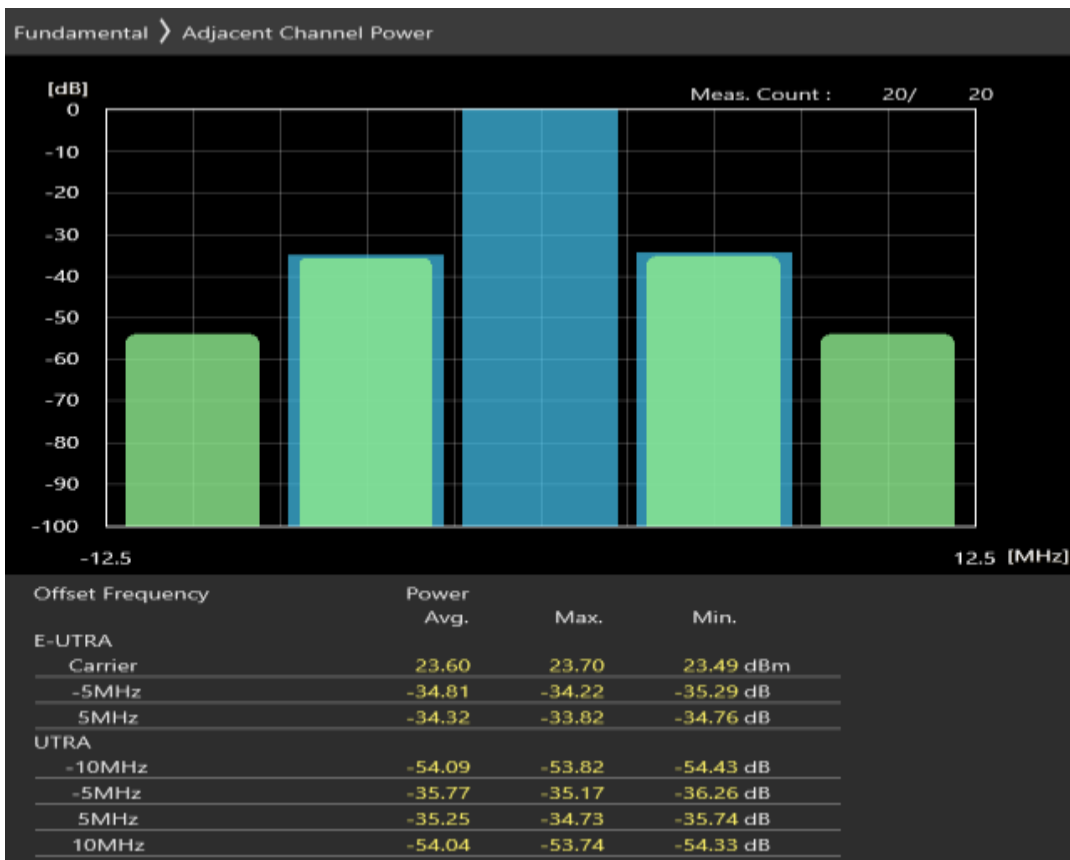
Band7 QAM16 BW=5MHz Channel=21425 RB Size=8 Position=#0
