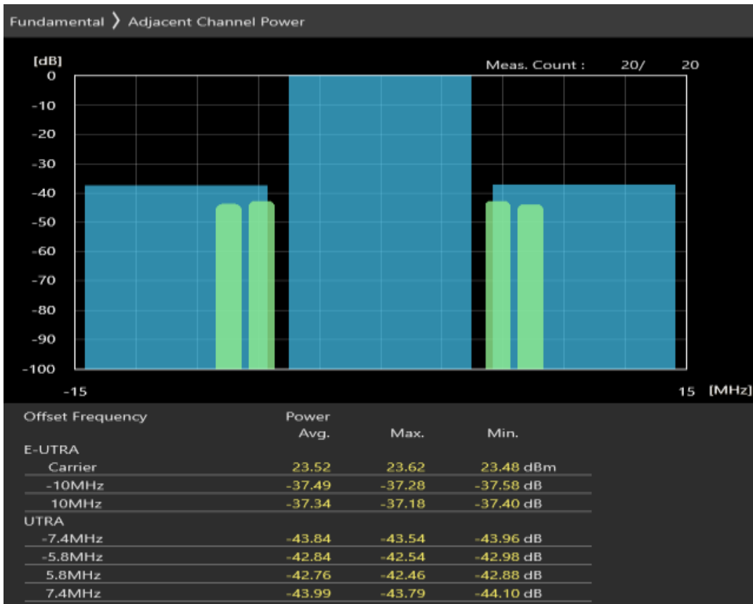
Band40 QPSK BW=10MHz Channel=39600 RB Size=12 Position=#0
