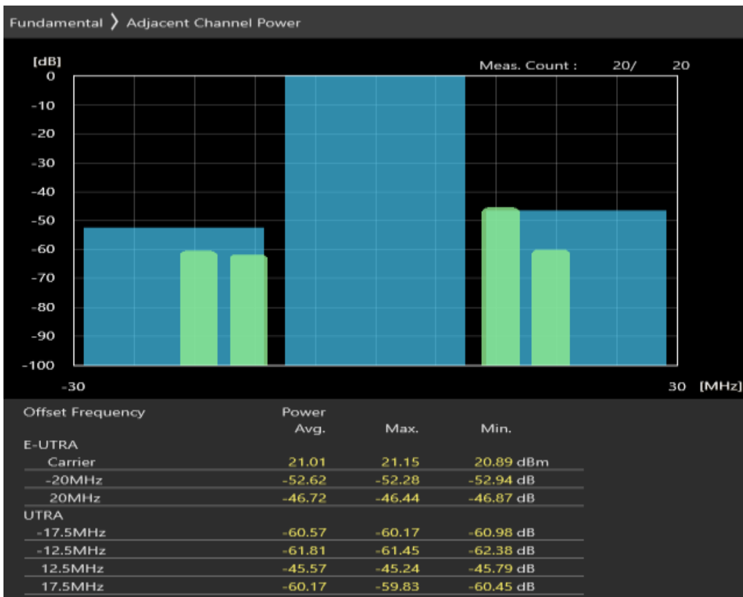
Band3 QAM16 BW=20MHz Channel=19850 RB Size=100 Position=#0
