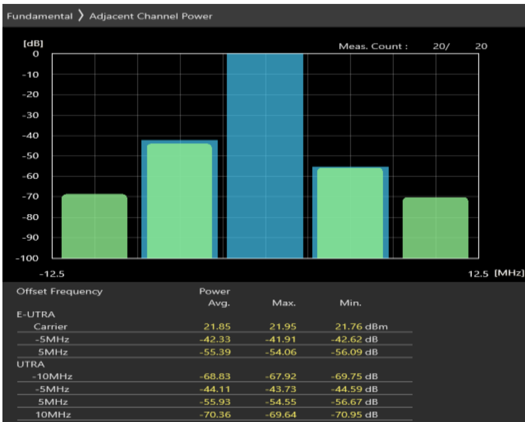
Band3 QPSK BW=5MHz Channel=19925 RB Size=8 Position=#Max
