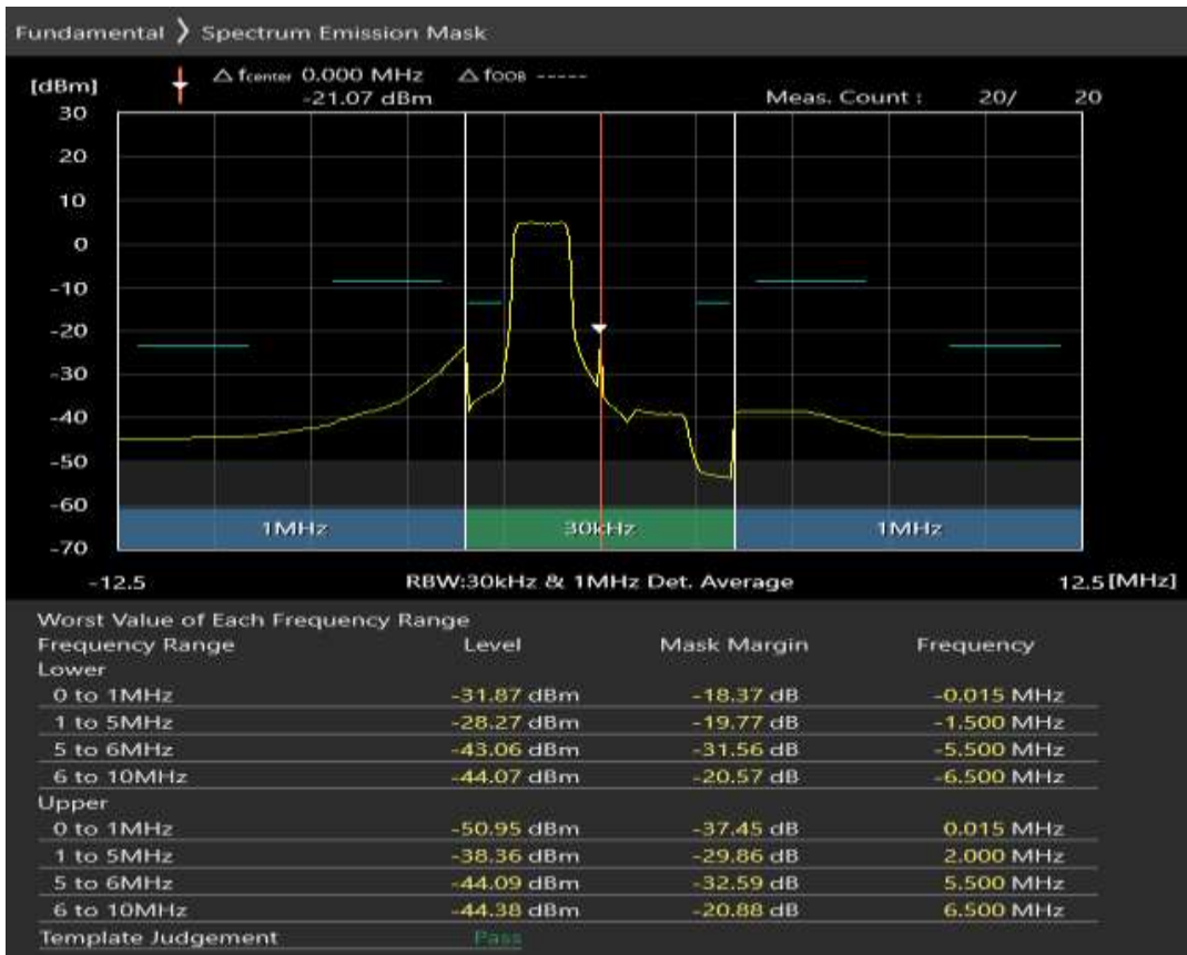
Band3 QAM16 BW=5MHz Channel=19925 RB Size=8 Position=#Max
