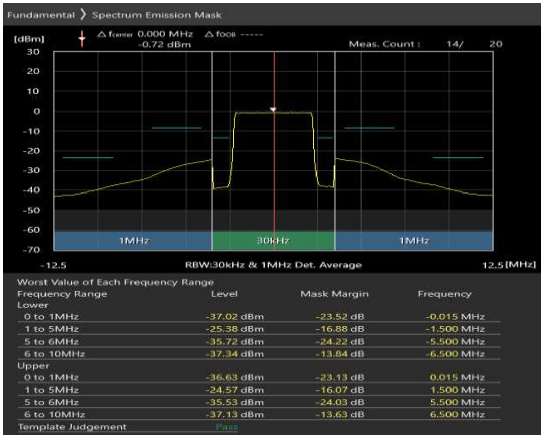
Band3 QPSK BW=5MHz Channel=19925 RB Size=8 Position=#0
