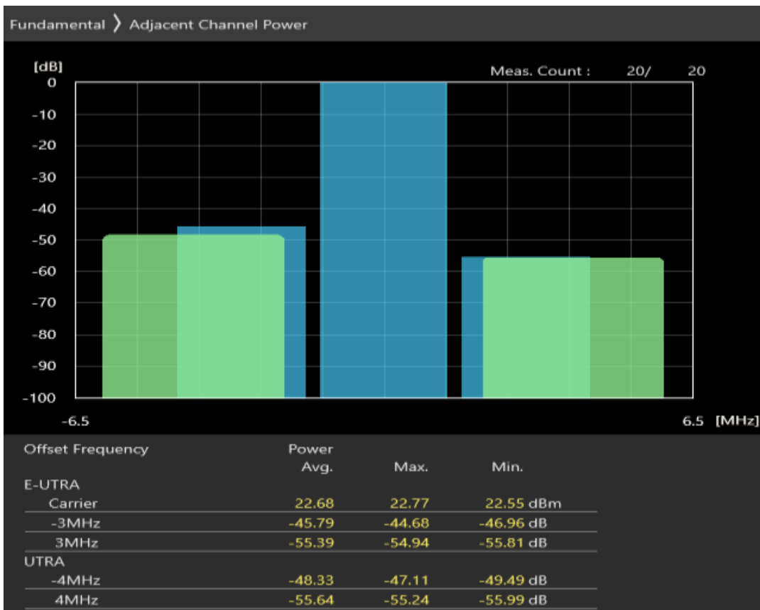
Band28 QPSK BW=3MHz Channel=27495 RB Size=4 Position=#Max
