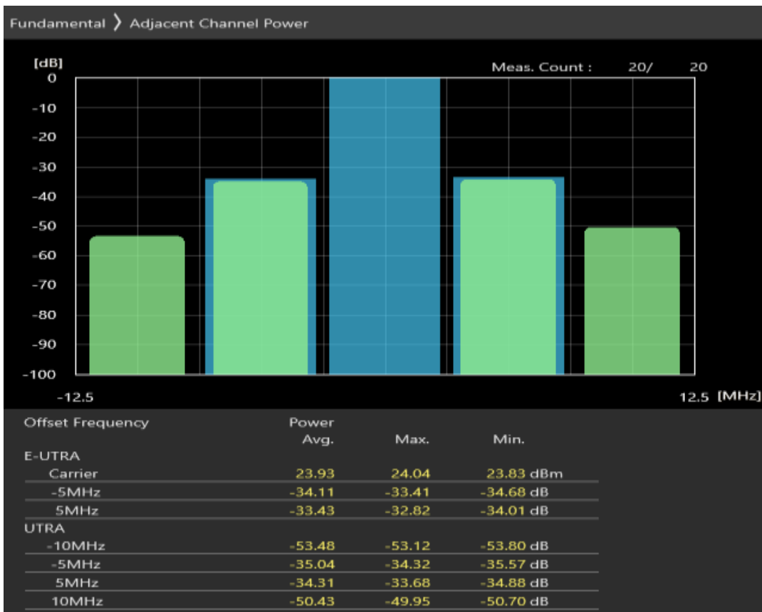
Band7 QAM16 BW=5MHz Channel=20775 RB Size=8 Position=#0
