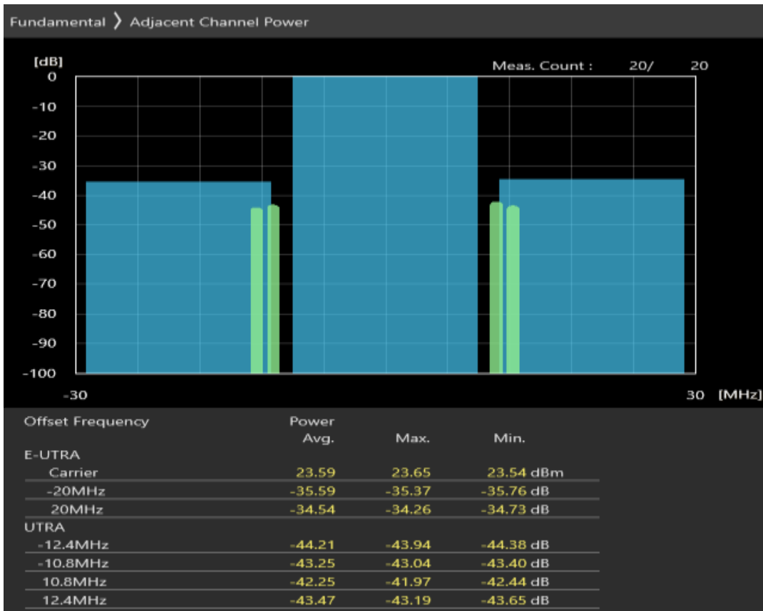
Band38 QAM16 BW=20MHz Channel=38150 RB Size=18 Position=#0
