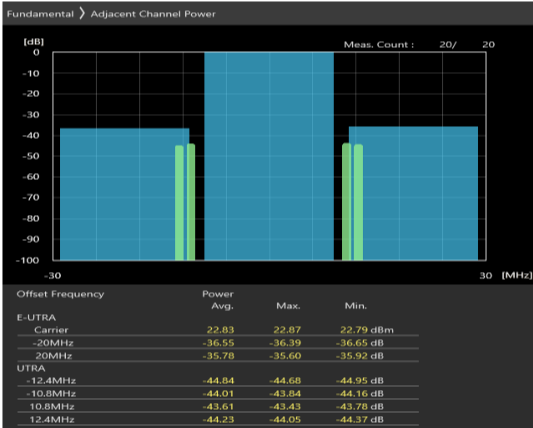
Band40 QPSK BW=5MHz Channel=38675 RB Size=8 Position=#0
