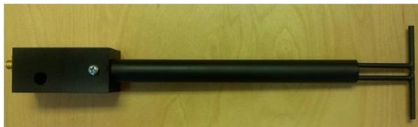
Figure 1 – MVG COMOSAR Validation Dipole
