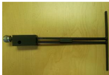
Figure 1 – MVG COMOSAR Validation Dipole
