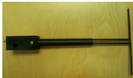
Figure 1 – MVG COMOSAR Validation Dipole
