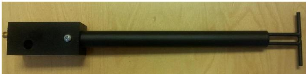
Figure 1 – MVG COMOSAR Validation Dipole
