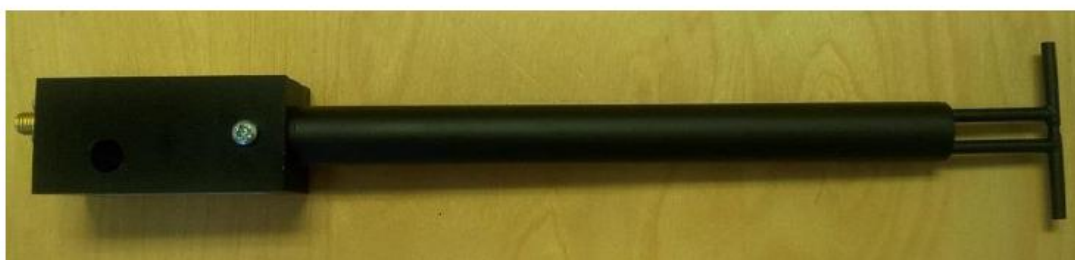
Figure 1 – MVG COMOSAR Validation Dipole
