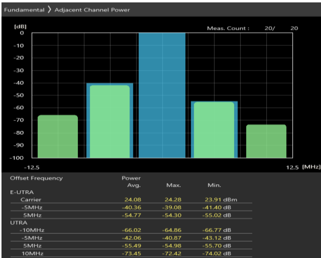
Band28 QPSK BW=5MHz Channel=27385 RB Size=8 Position=#Max
