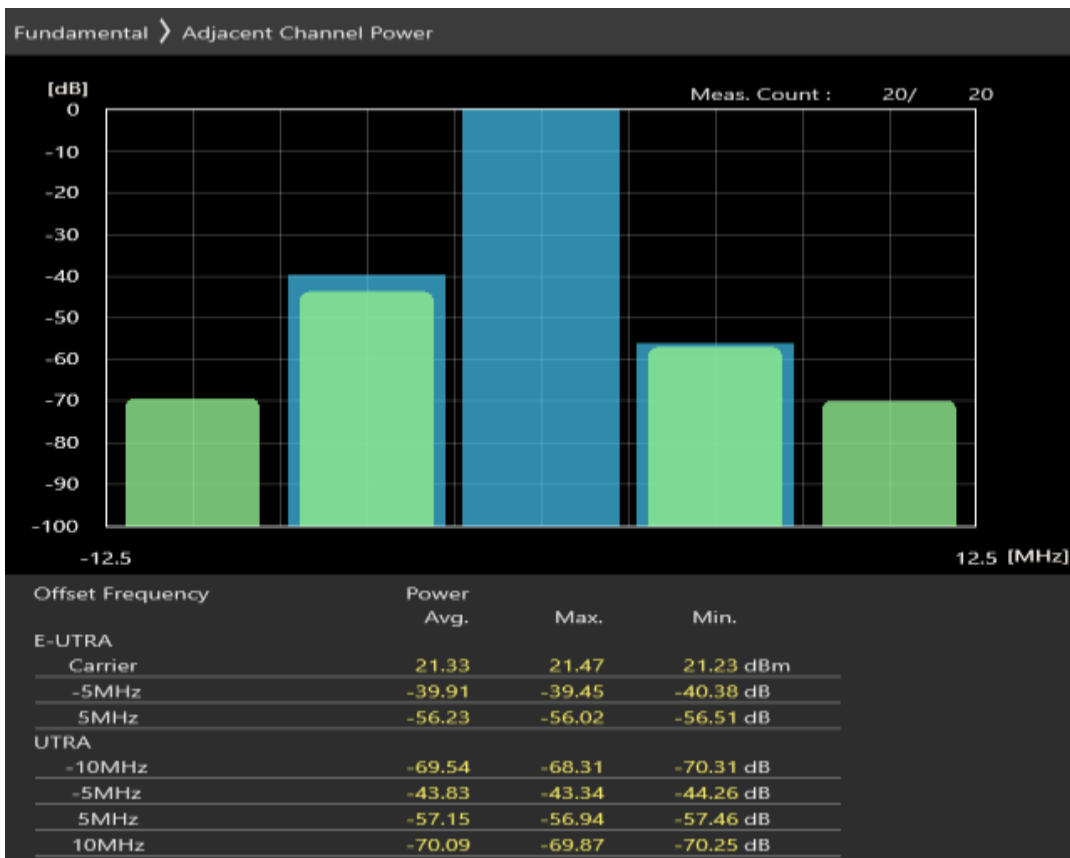
Band8 QAM16 BW=5MHz Channel=21625 RB Size=8 Position=#Max
