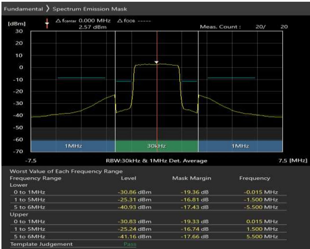
Band28 16QAM BW=3MHz Channel=27360 RB Size=4 Position=#0
