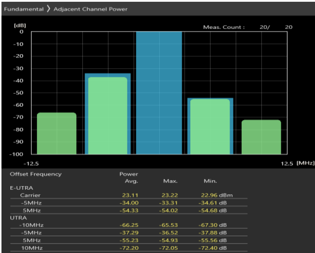
Band20 16QAM BW=5MHz Channel=24425 RB Size=8 Position=#Max
