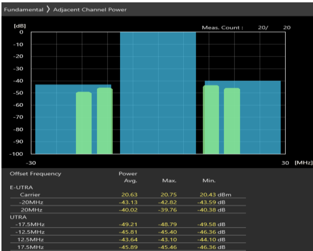
Band3 16QAM BW=20MHz Channel=19300 RB Size=18 Position=#0
