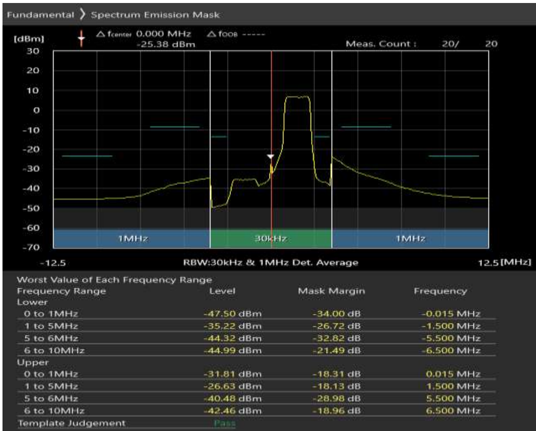
Band20 16QAM BW=5MHz Channel=24175 RB Size=25 Position=#0
