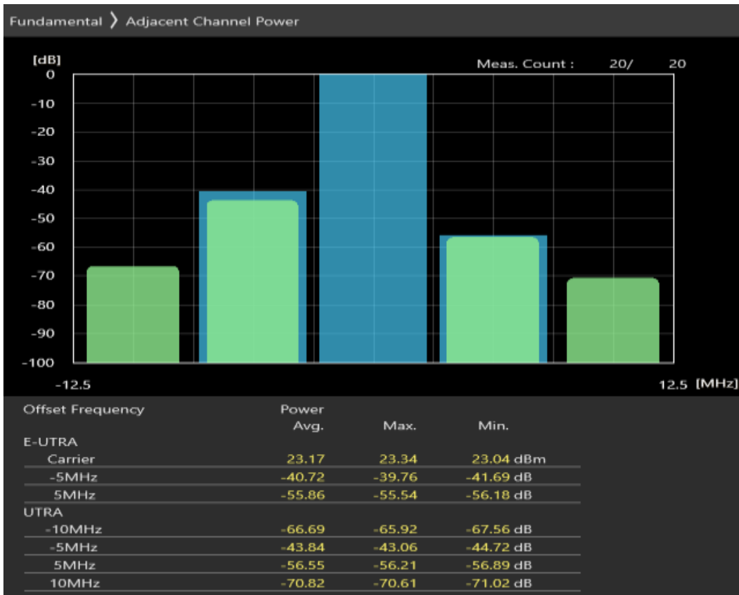
Band1 16QAM BW=5MHz Channel=18575 RB Size=8 Position=#Max
