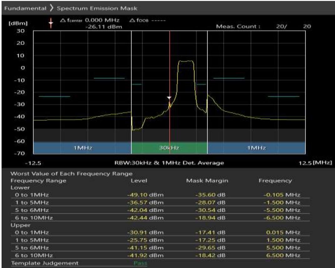
Band40 16QAM BW=5MHz Channel=38675 RB Size=25 Position=#0
