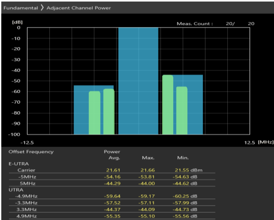
Band40 16QAM BW=5MHz Channel=39625 RB Size=25 Position=#0
