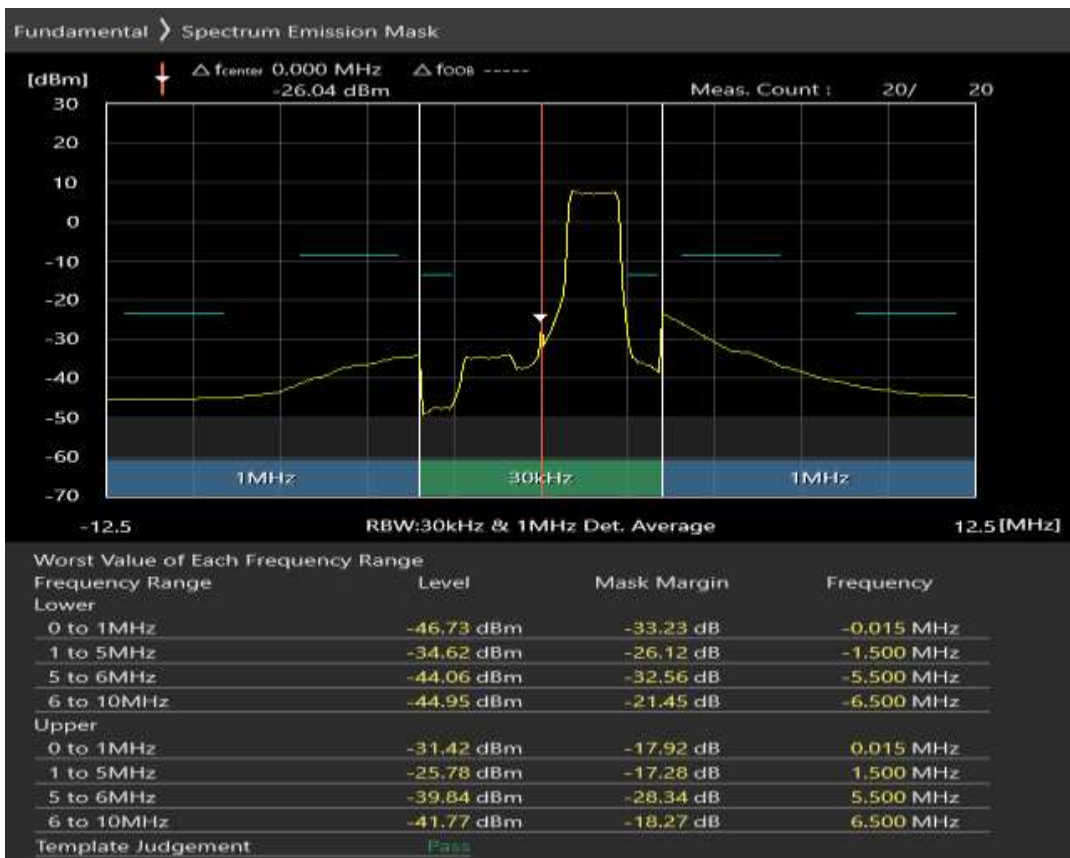
Band20 QPSK BW=5MHz Channel=24175 RB Size=25 Position=#0
