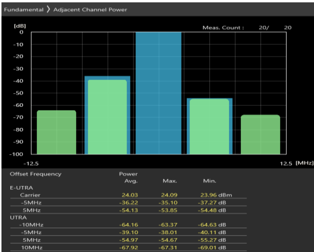
Band7 QPSK BW=5MHz Channel=21425 RB Size=8 Position=#Max
