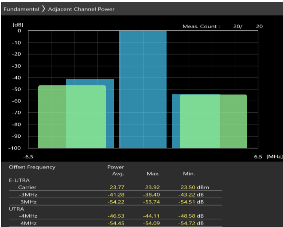
Band28 QPSK BW=3MHz Channel=27360 RB Size=4 Position=#Max
