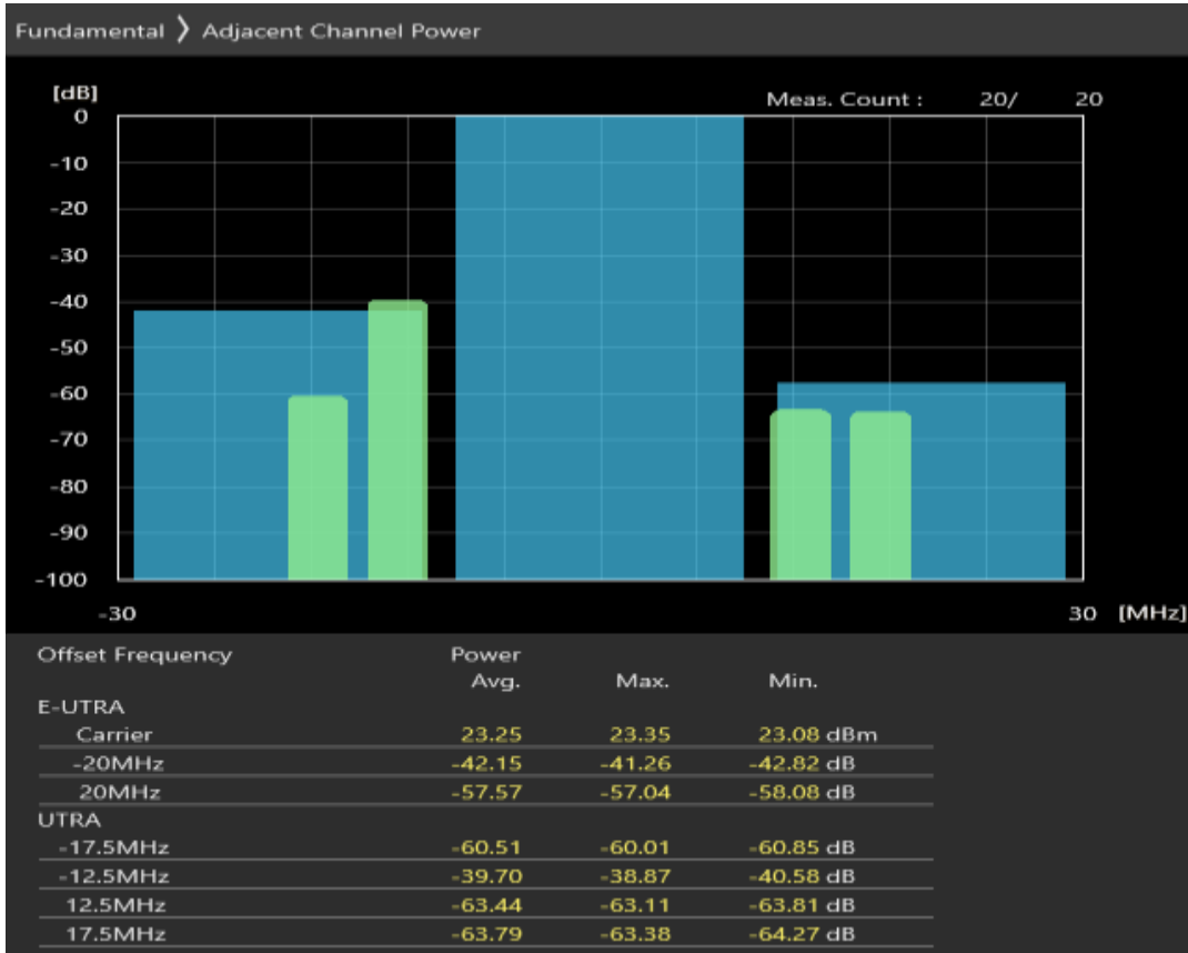
Band1 16QAM BW=20MHz Channel=18300 RB Size=18 Position=#Max
