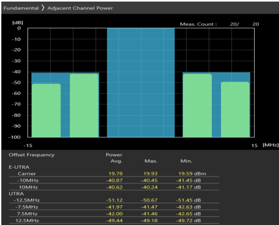
Band3 QPSK BW=10MHz Channel=19575 RB Size=12 Position=#0
