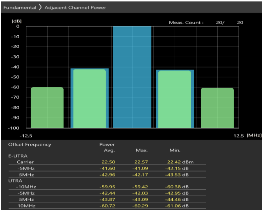
Band1 QPSK BW=5MHz Channel=18575 RB Size=8 Position=#0
