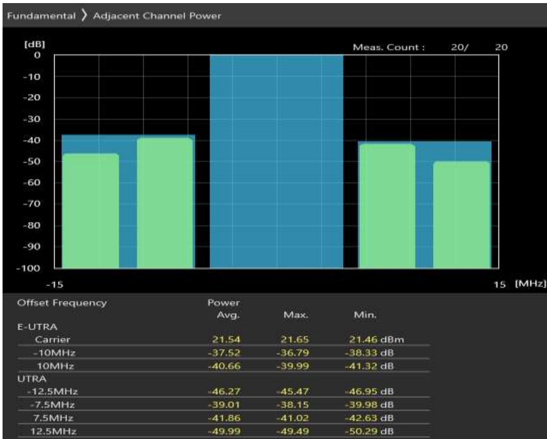
Band8 QPSK BW=10MHz Channel=21750 RB Size=12 Position=#0
