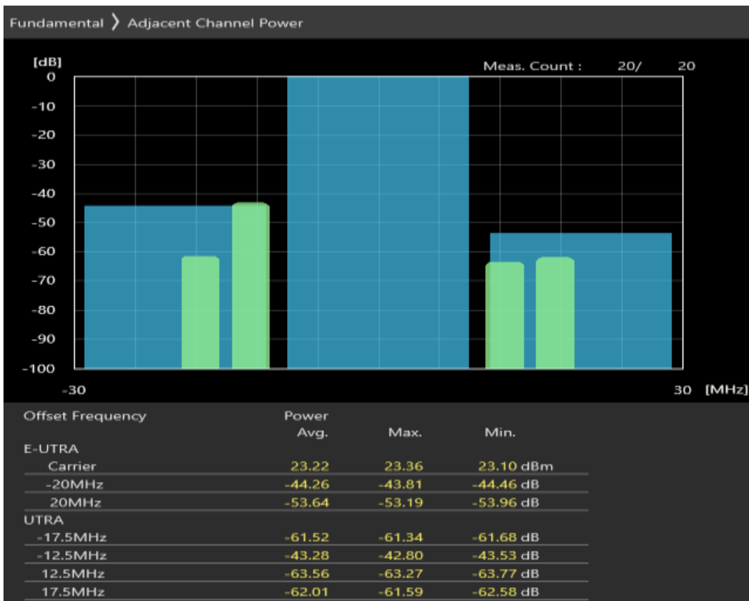
Band3 QPSK BW=20MHz Channel=19575 RB Size=18 Position=#Max
