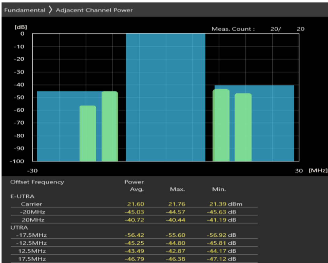
Band28 16QAM BW=20MHz Channel=27310 RB Size=18 Position=#0
