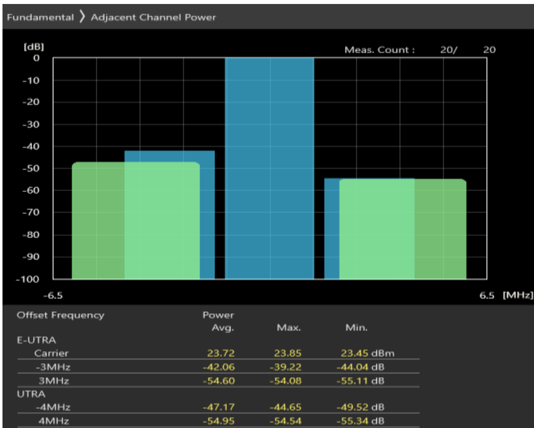
Band28 QPSK BW=3MHz Channel=27495 RB Size=4 Position=#Max
