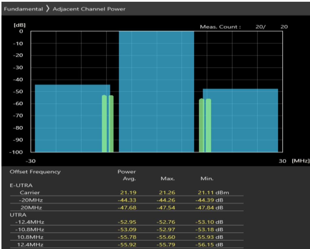
Band7 QPSK BW=5MHz Channel=20775 RB Size=8 Position=#0
