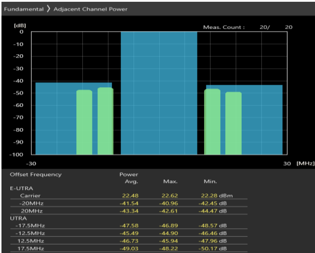
Band8 QAM16 BW=1.4MHz Channel=21457 RB Size=5 Position=#0
