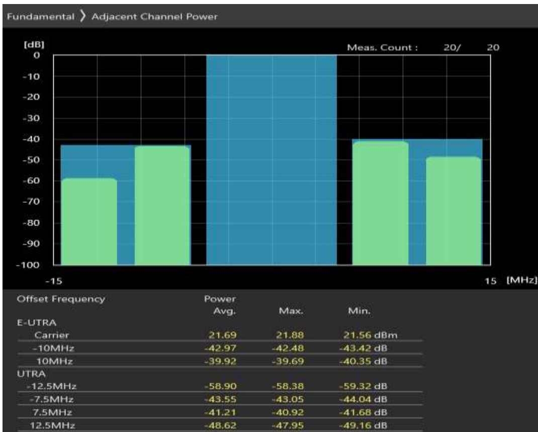
Band28 16QAM BW=10MHz Channel=27260 RB Size=12 Position=#0
