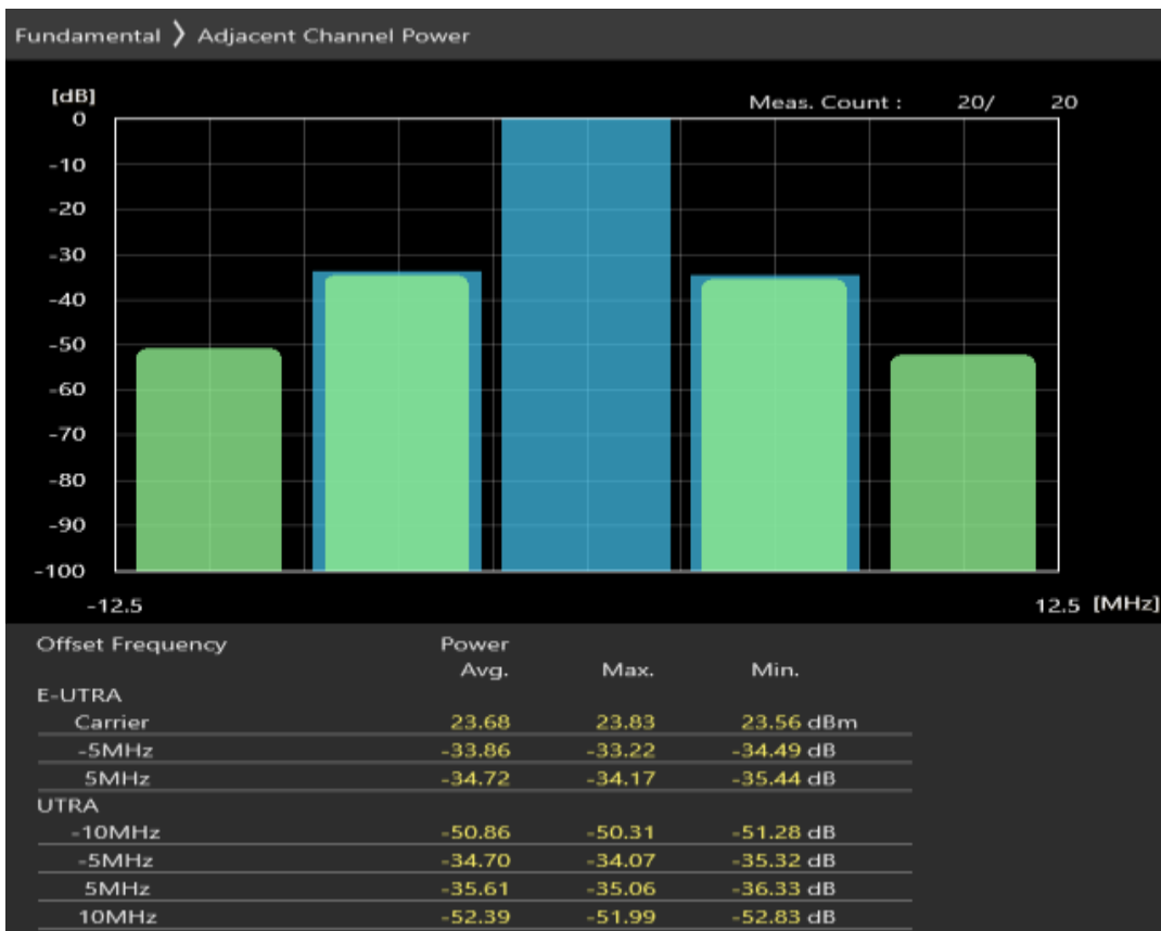
Band7 16QAM BW=5MHz Channel=21100 RB Size=8 Position=#0
