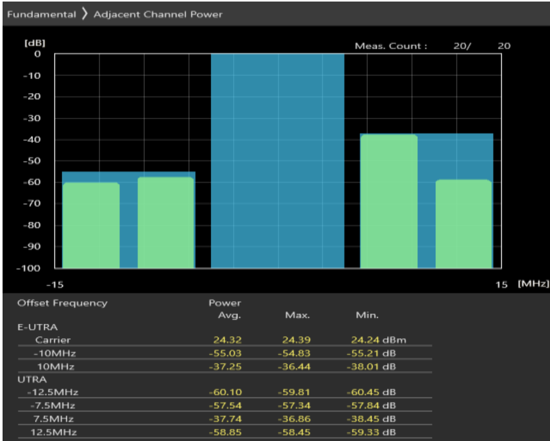
Band7 QPSK BW=10MHz Channel=21100 RB Size=50 Position=#0
