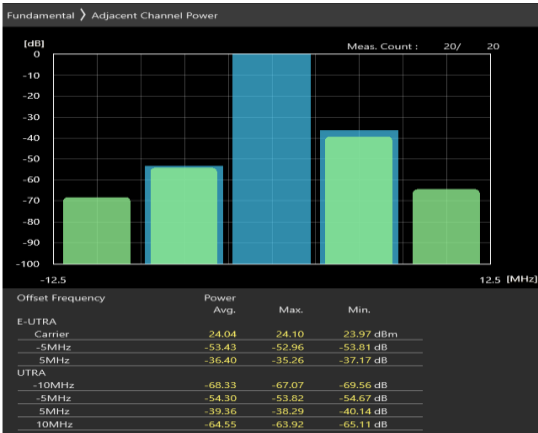
Band7 QPSK BW=5MHz Channel=21425 RB Size=25 Position=#0
