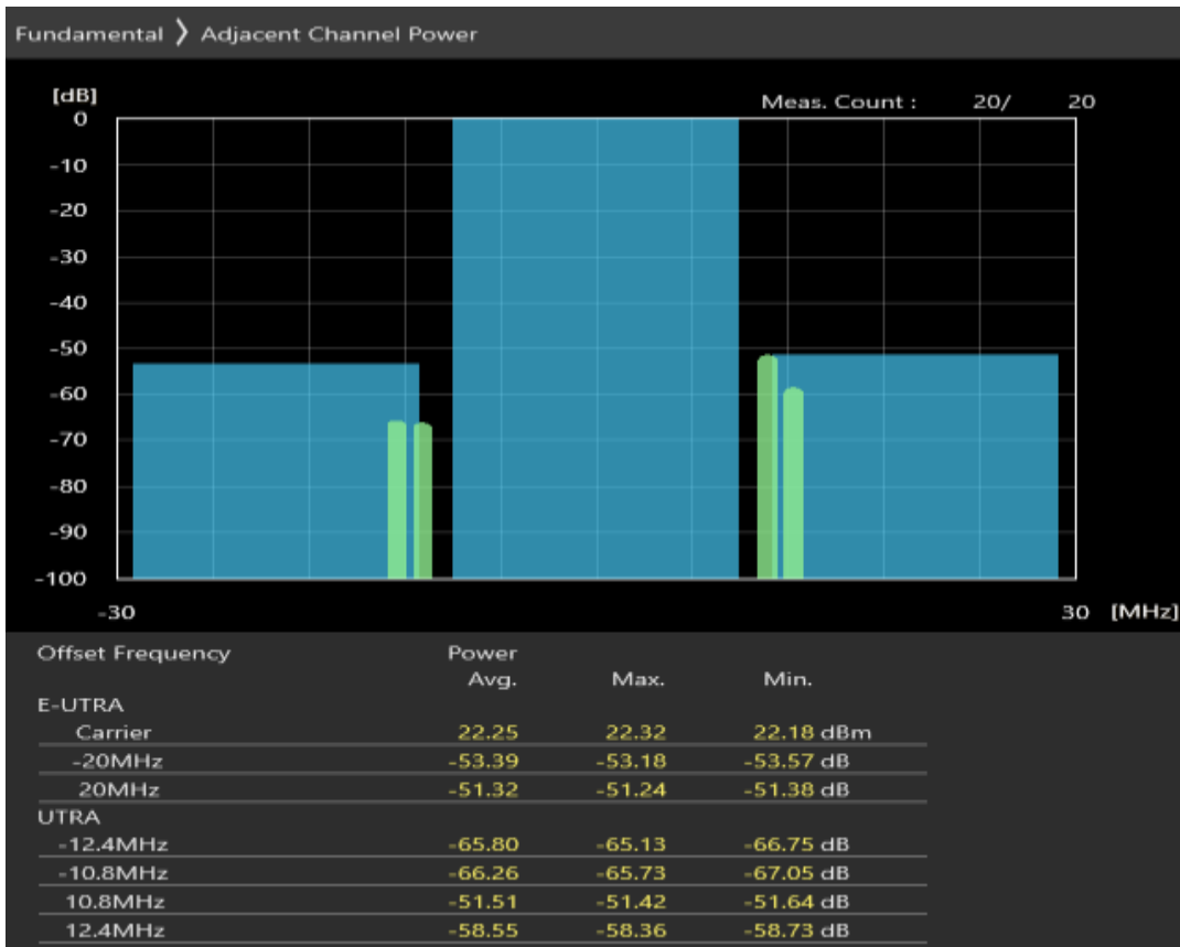
Band40 QPSK BW=20MHz Channel=38750 RB Size=100 Position=#0
