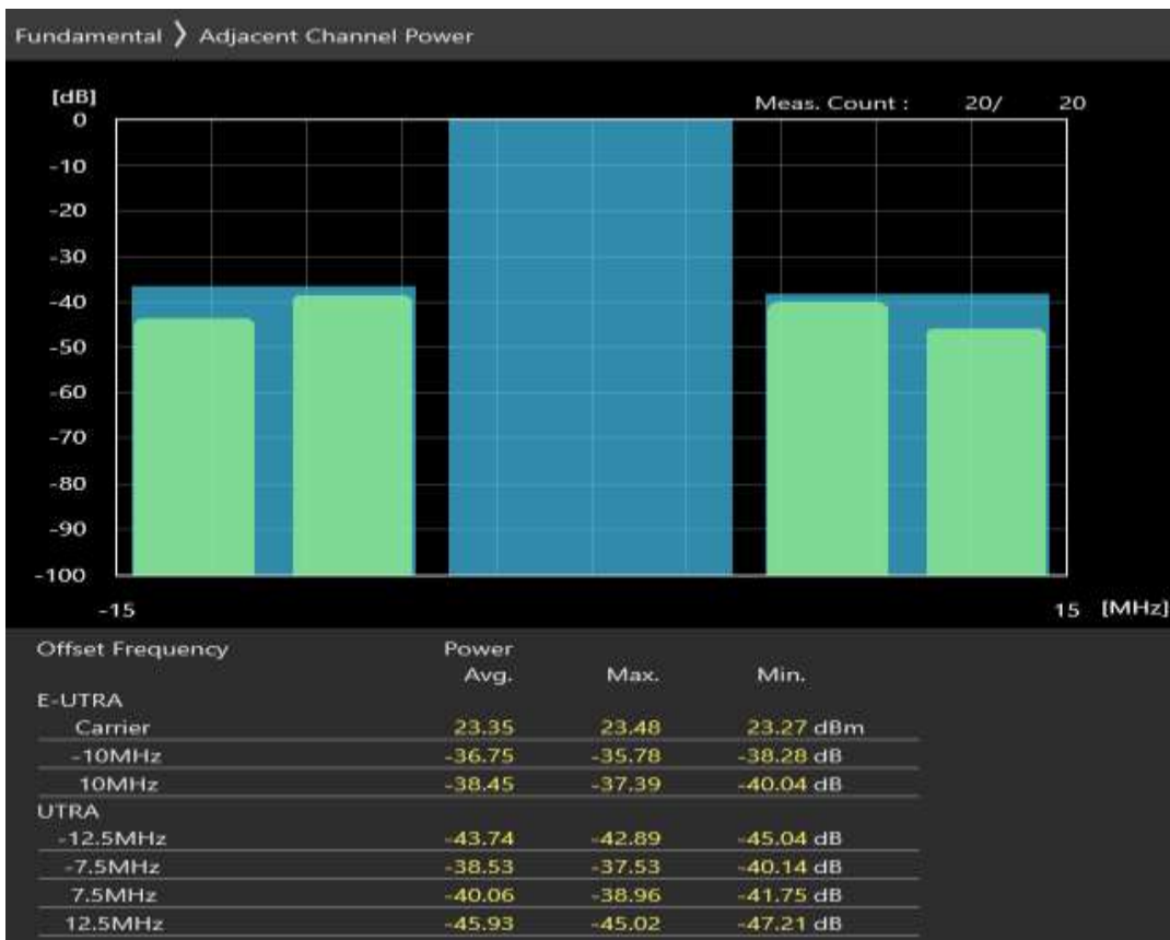
Band7 16QAM BW=10MHz Channel=21400 RB Size=12 Position=#0
