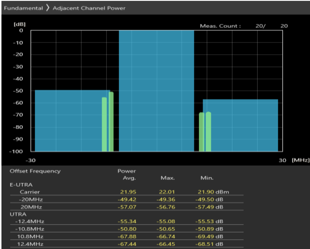
Band40 16QAM BW=20MHz Channel=39550 RB Size=18 Position=#Max
