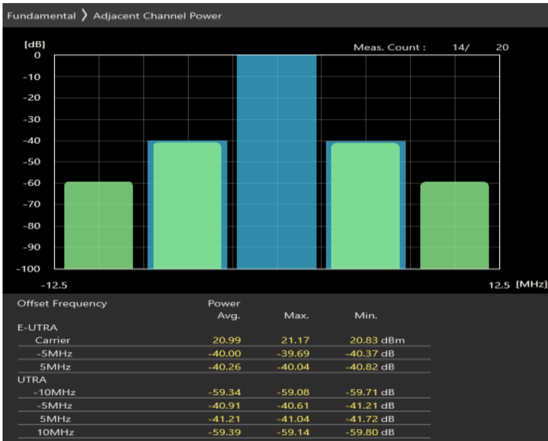
Band28 QPSK BW=5MHz Channel=27635 RB Size=8 Position=#0
