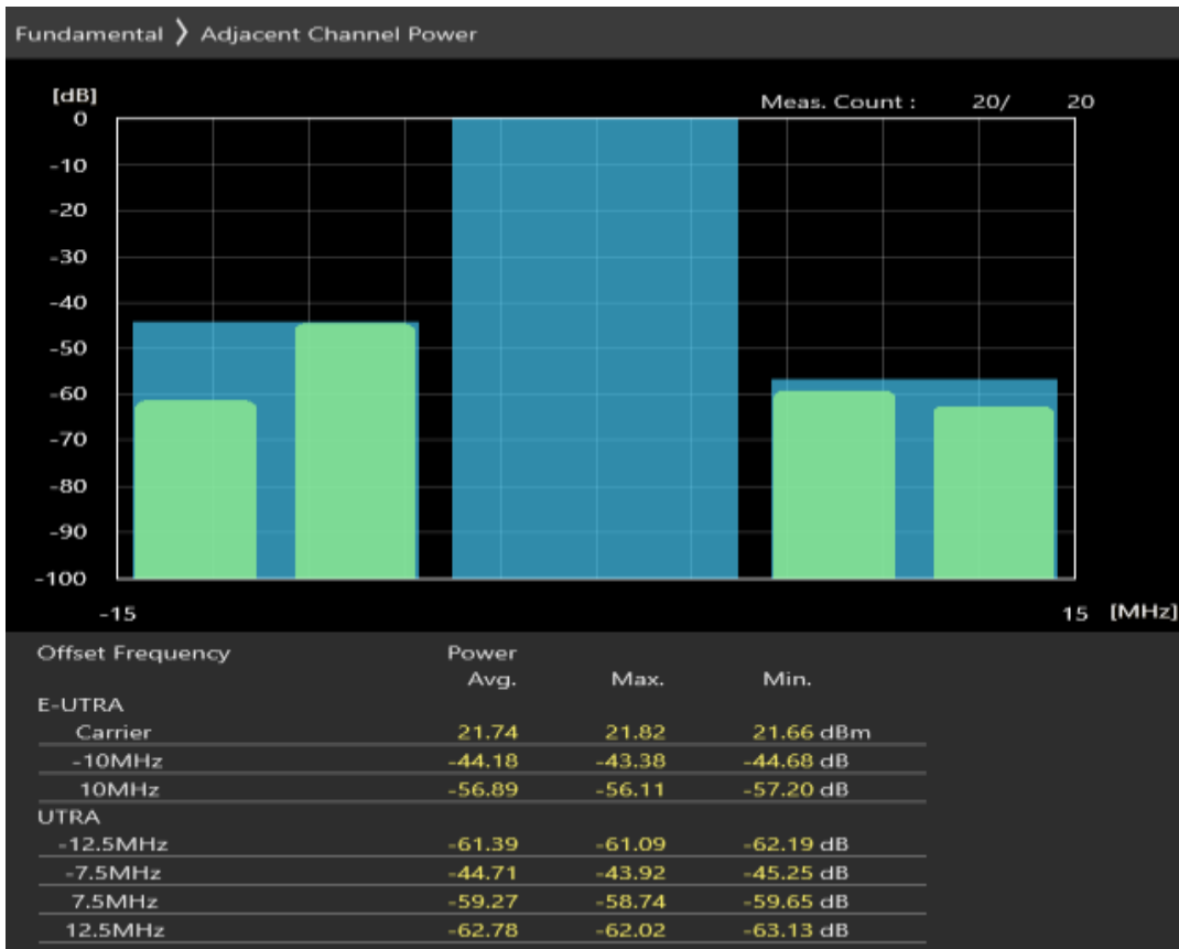
Band28 16QAM BW=10MHz Channel=27410 RB Size=12 Position=#Max
