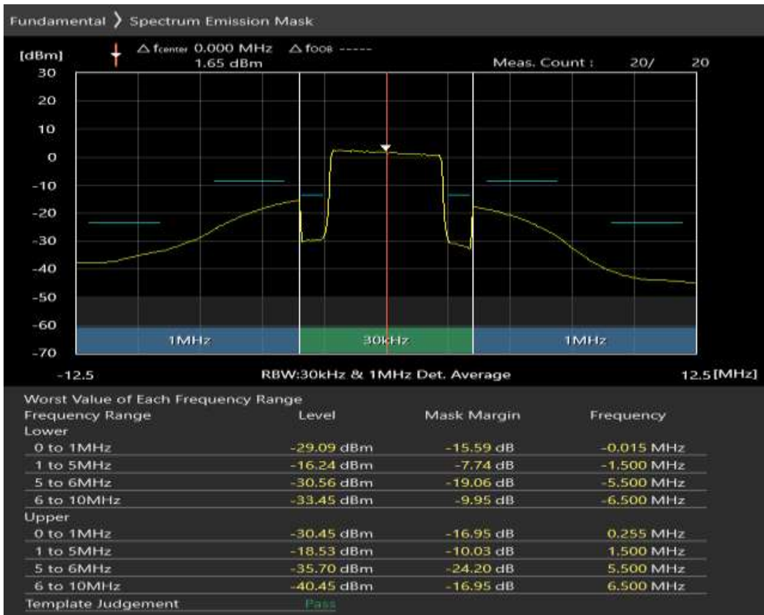
Band20 16QAM BW=5MHz Channel=24425 RB Size=8 Position=#0
