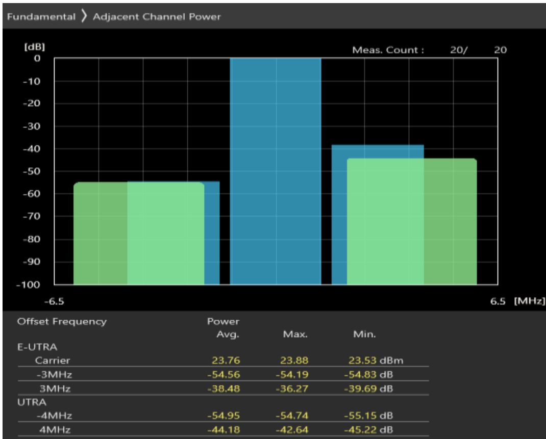
Band28 QPSK BW=3MHz Channel=27225 RB Size=15 Position=#0
