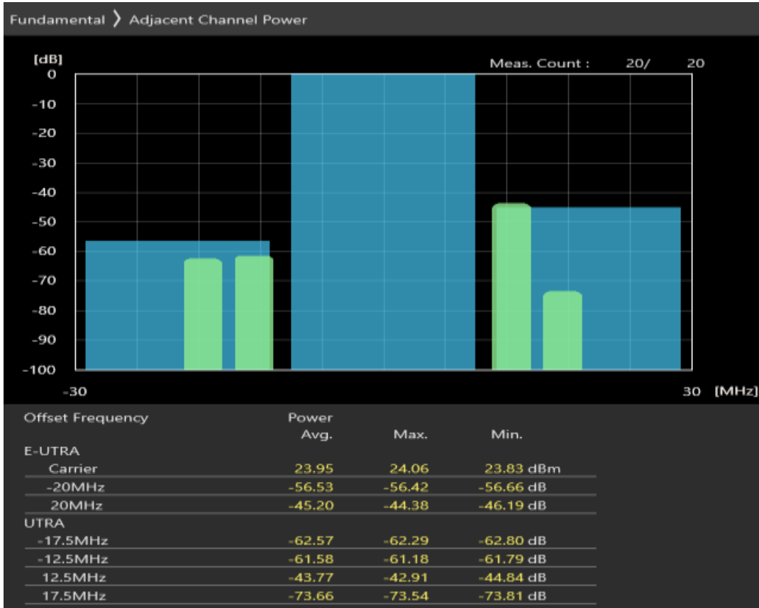
Band28 QPSK BW=20MHz Channel=27560 RB Size=100 Position=#0
