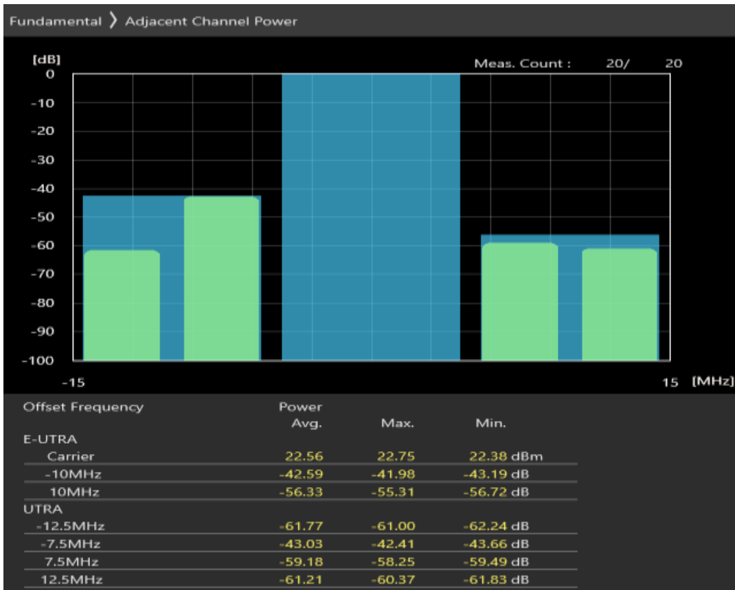
Band3 16QAM BW=10MHz Channel=19575 RB Size=12 Position=#Max
