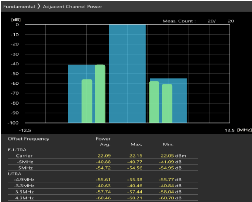
Band40 16QAM BW=5MHz Channel=38675 RB Size=8 Position=#Max
