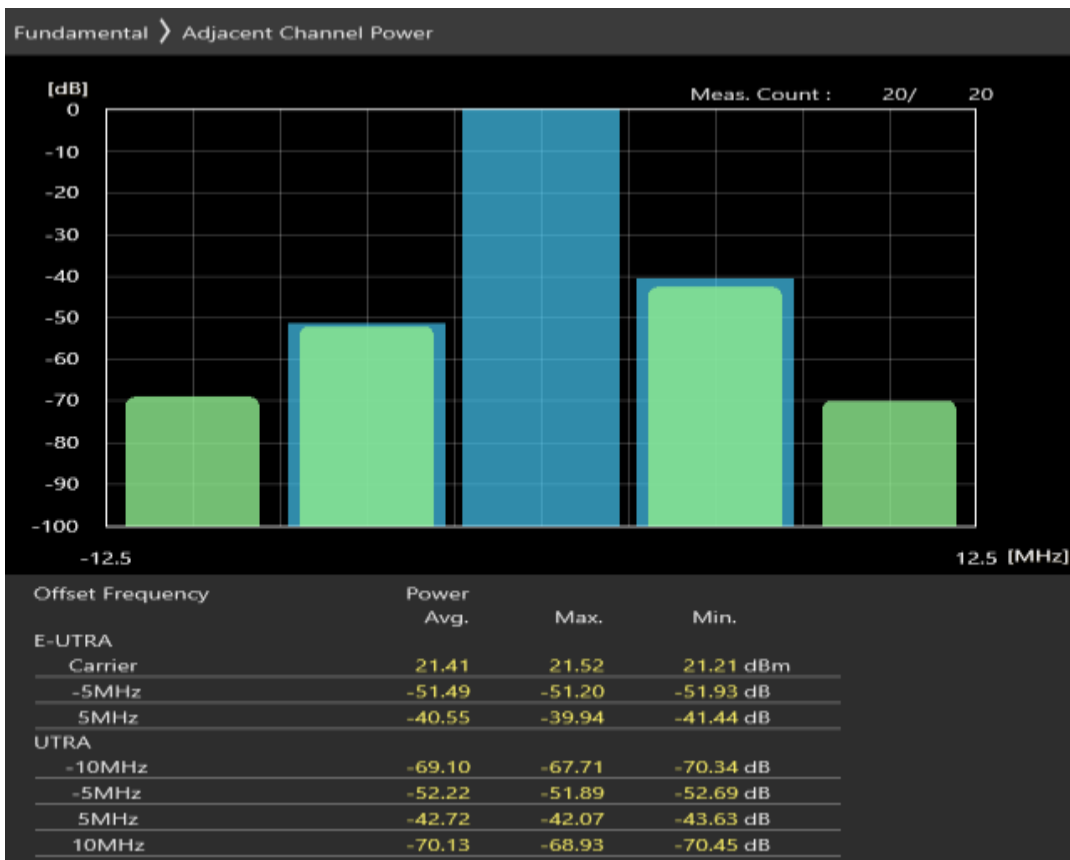
Band8 QPSK BW=1.4MHz Channel=21457 RB Size=5 Position=#0
