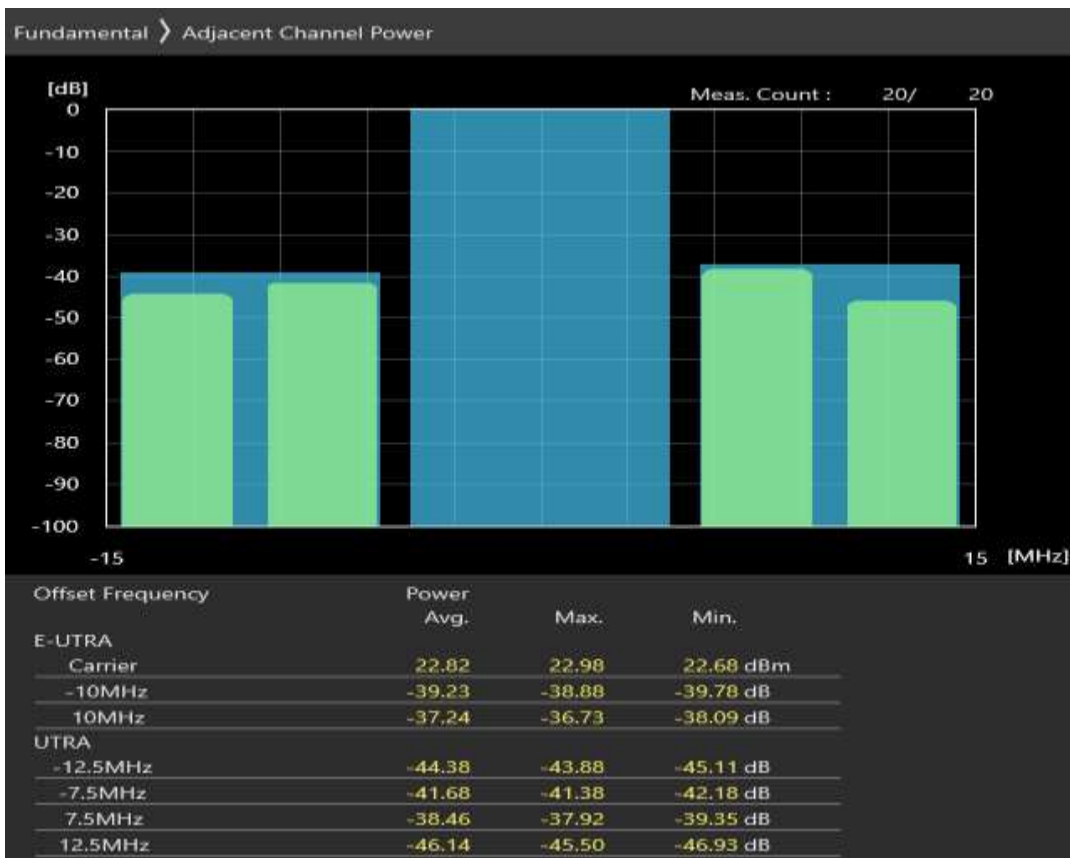
Band3 16QAM BW=10MHz Channel=1990 RB Size=12 Position=#0
