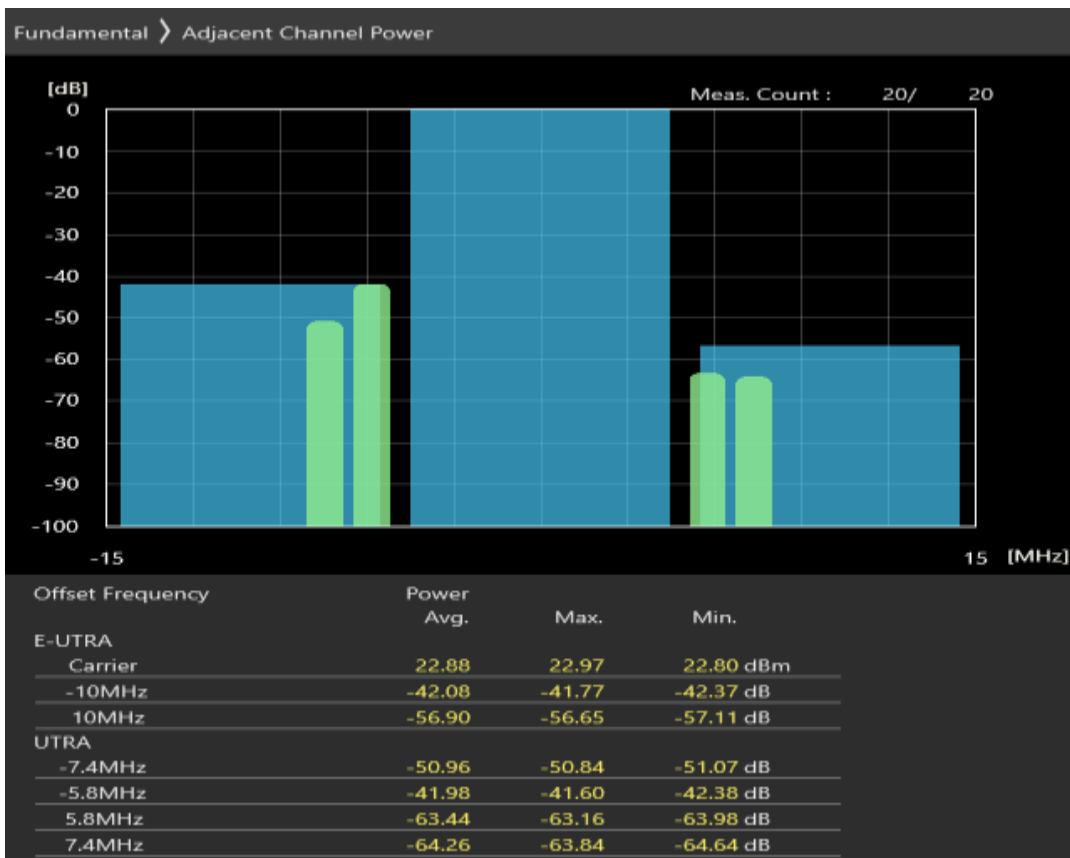
Band40 QPSK BW=10MHz Channel=38700 RB Size=12 Position=#Max
