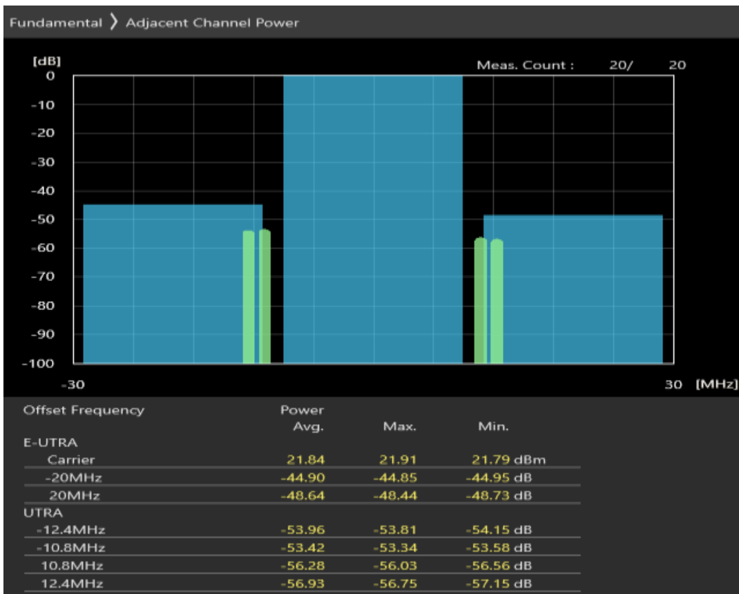
Band40 16QAM BW=20MHz Channel=39550 RB Size=18 Position=#0
