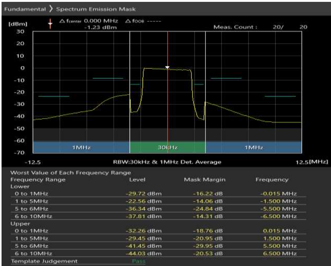
Band8 QAM16 BW=5MHz Channel=21775 RB Size=8 Position=#0
