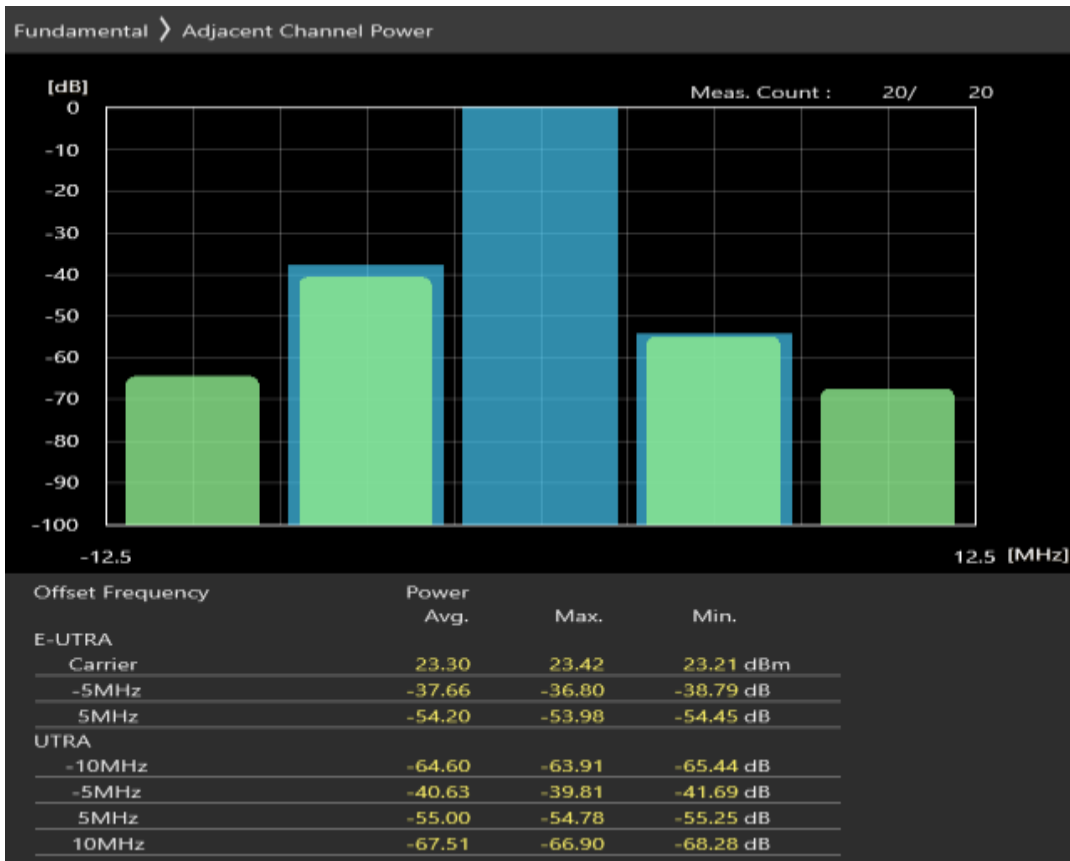
Band7 16QAM BW=5MHz Channel=21425 RB Size=8 Position=#Max
