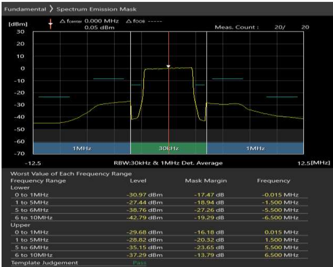
Band8 QPSK BW=5MHz Channel=21475 RB Size=8 Position=#0
