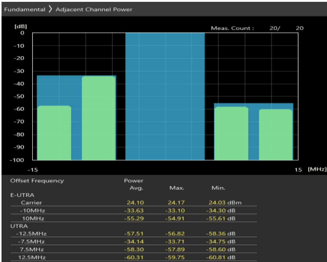
Band20 QPSK BW=10MHz Channel=24300 RB Size=12 Position=#Max
