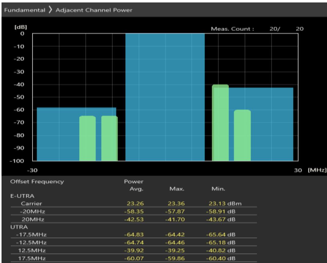
Band1 16QAM BW=20MHz Channel=18100 RB Size=100 Position=#0
