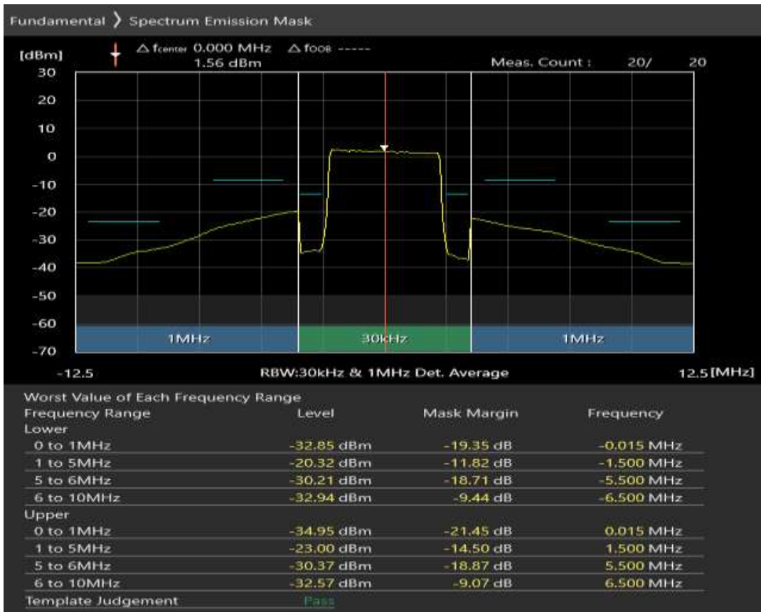
Band20 16QAM BW=5MHz Channel=24300 RB Size=8 Position=#0
