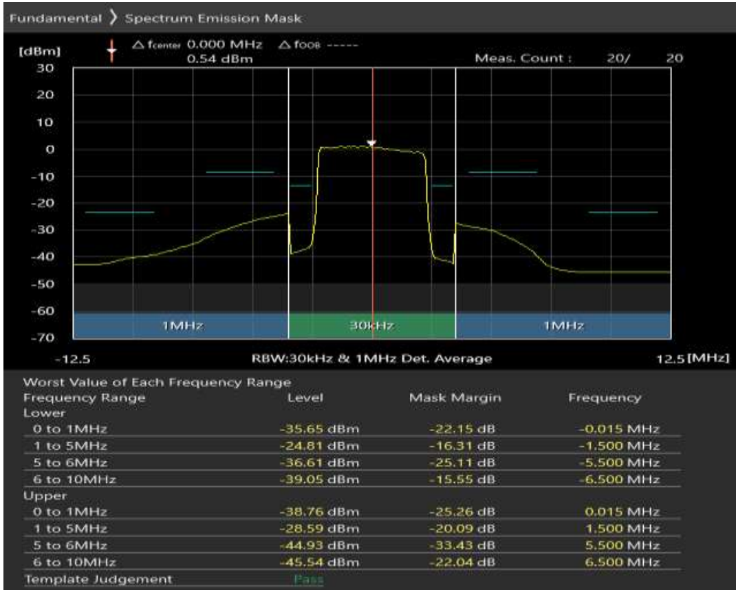
Band28 16QAM BW=5MHz Channel=27635 RB Size=8 Position=#0
