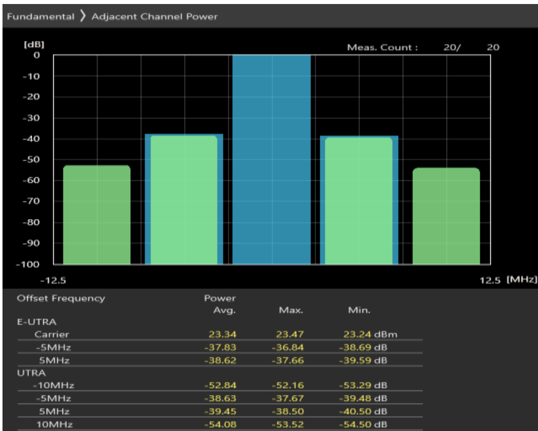
Band7 16QAM BW=5MHz Channel=21425 RB Size=8 Position=#0
