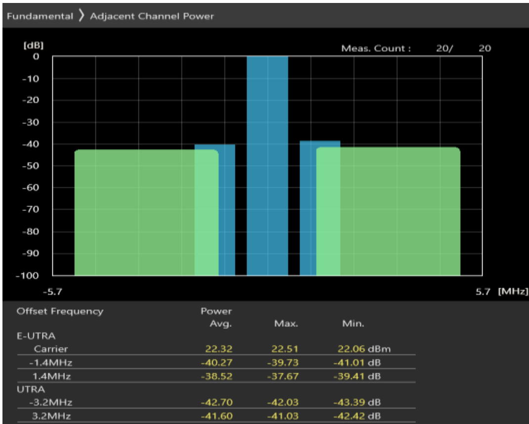
Band8 QPSK BW=1.4MHz Channel=21793 RB Size=6 Position=#0
