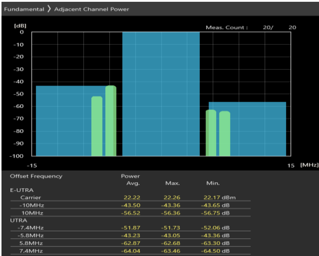
Band40 16QAM BW=10MHz Channel=38700 RB Size=12 Position=#Max
