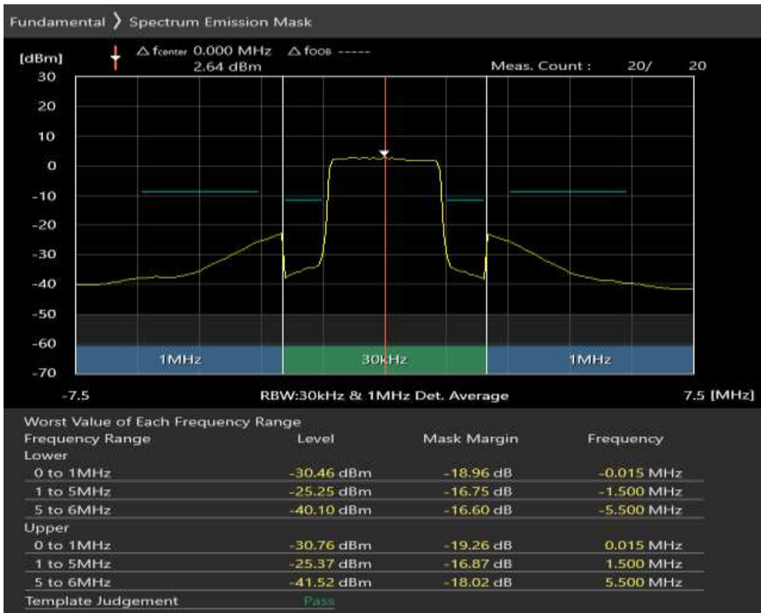
Band28 16QAM BW=3MHz Channel=27495 RB Size=4 Position=#0
