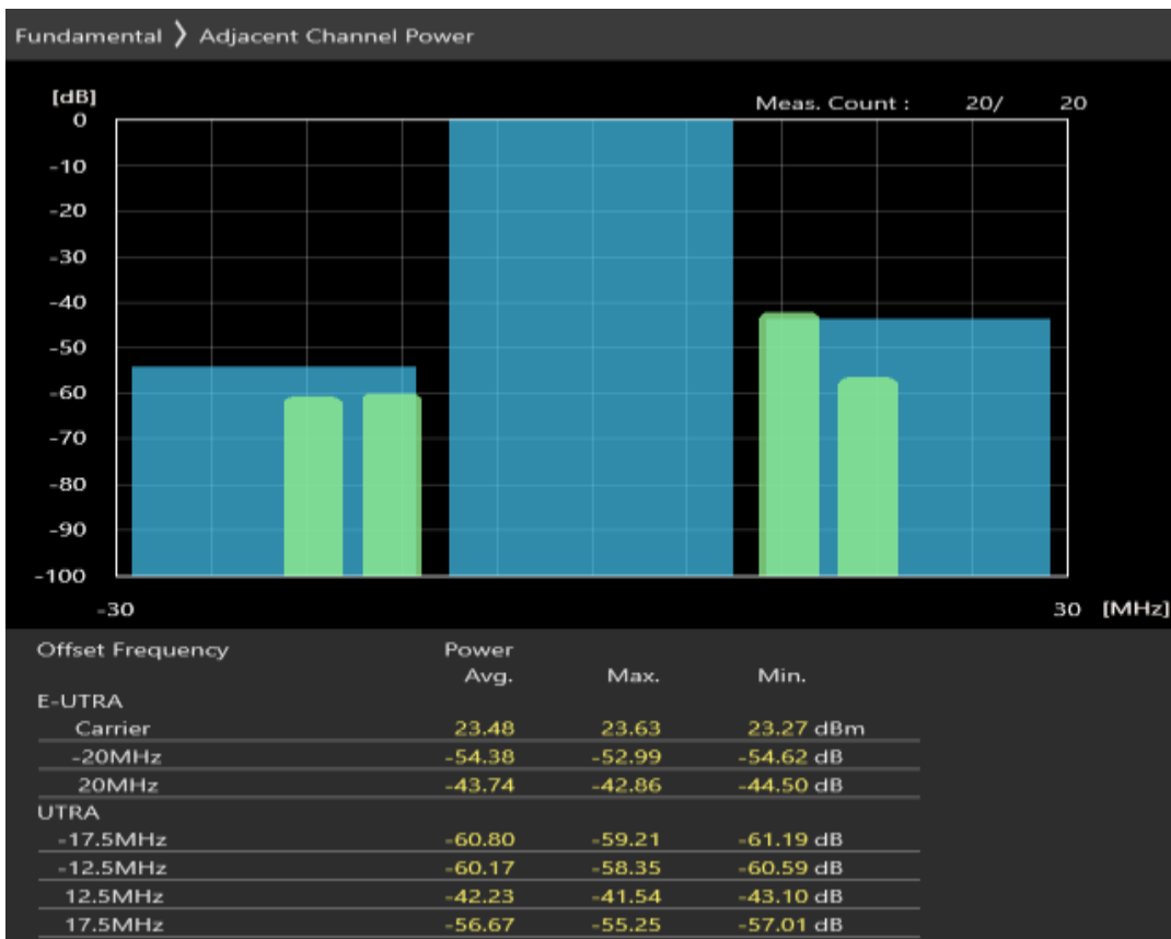
Band7 16QAM BW=20MHz Channel=21100 RB Size=100 Position=#0
