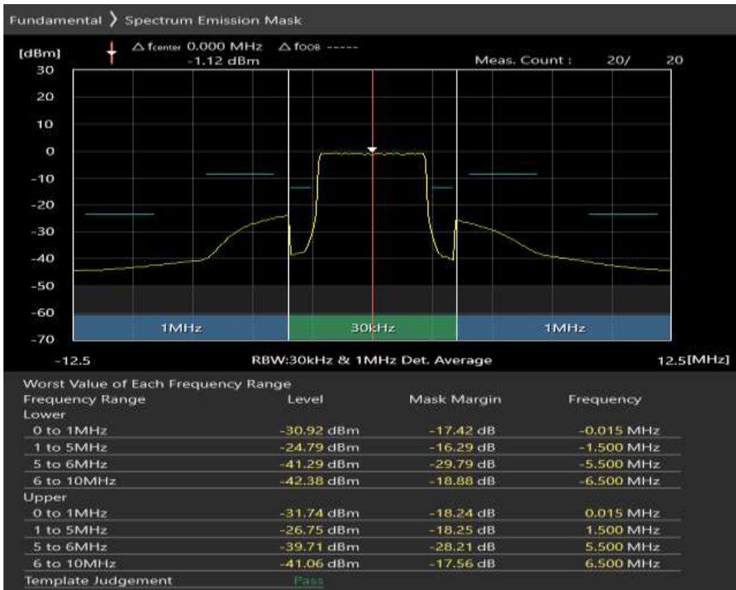
Band8 QAM16 BW=5MHz Channel=21625 RB Size=8 Position=#0
