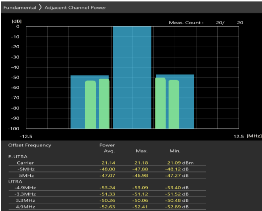
Band40 QPSK BW=10MHz Channel=38700 RB Size=12 Position=#0
