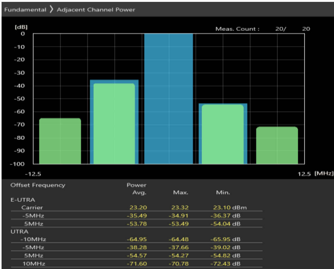
Band20 16QAM BW=5MHz Channel=24300 RB Size=8 Position=#Max
