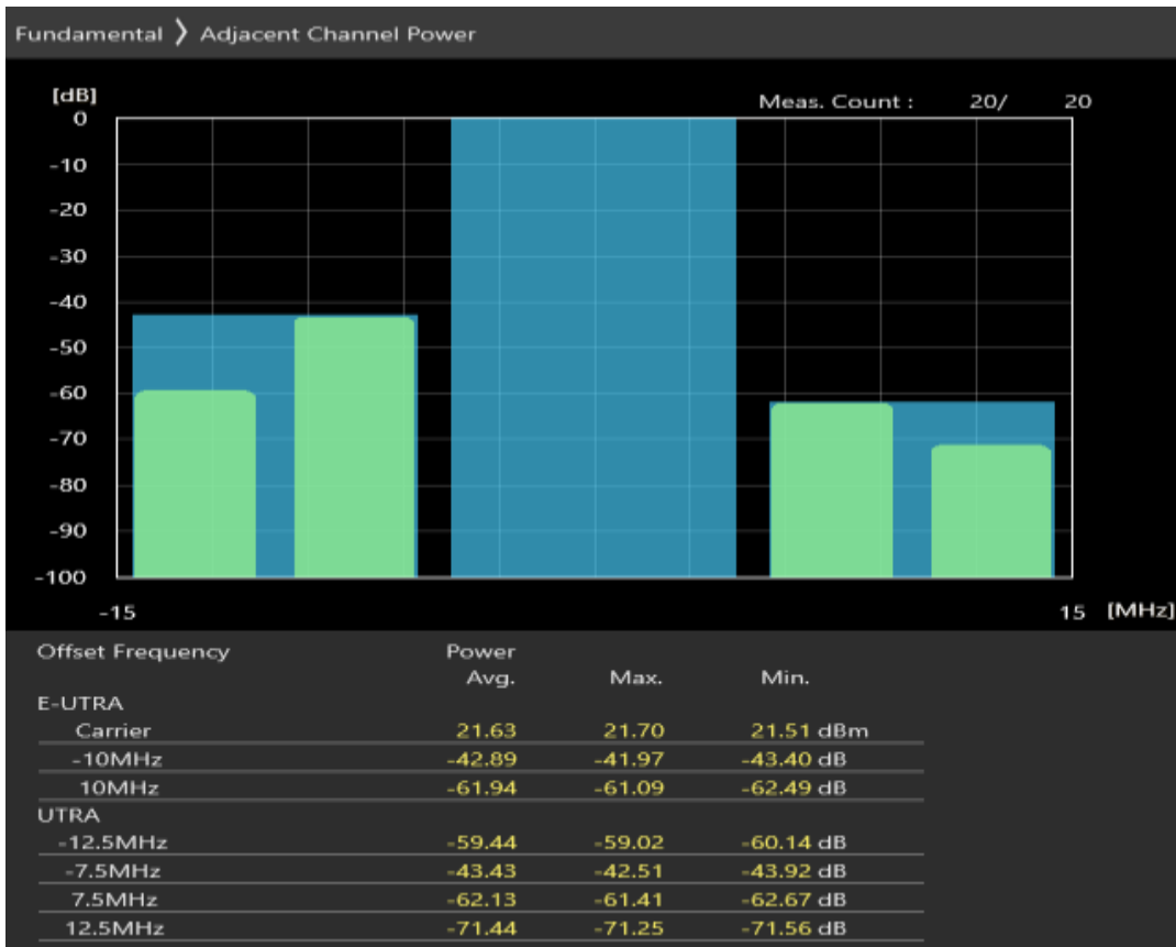
Band28 16QAM BW=10MHz Channel=27610 RB Size=12 Position=#Max
