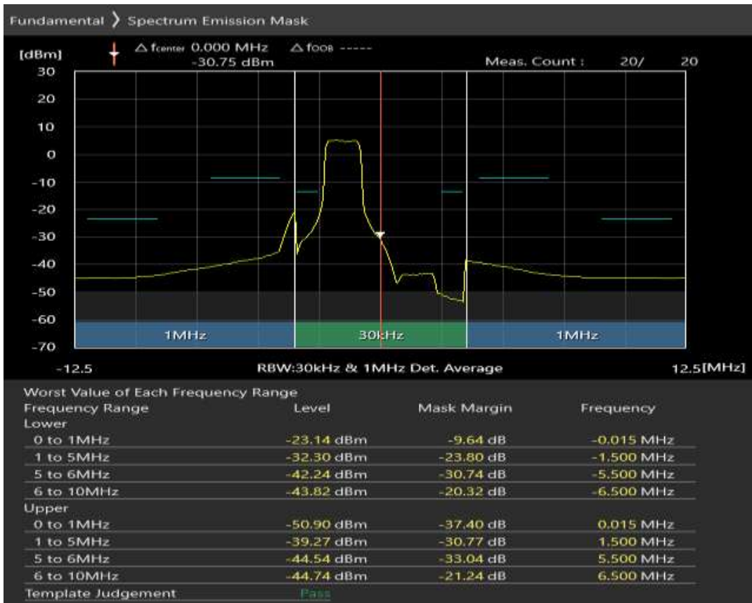
Band8 QAM16 BW=5MHz Channel=21775 RB Size=8 Position=#Max
