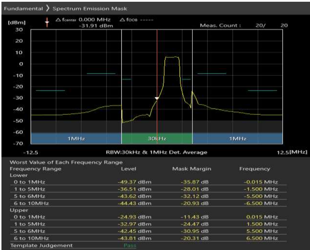
Band8 QPSK BW=5MHz Channel=21775 RB Size=25 Position=#0
