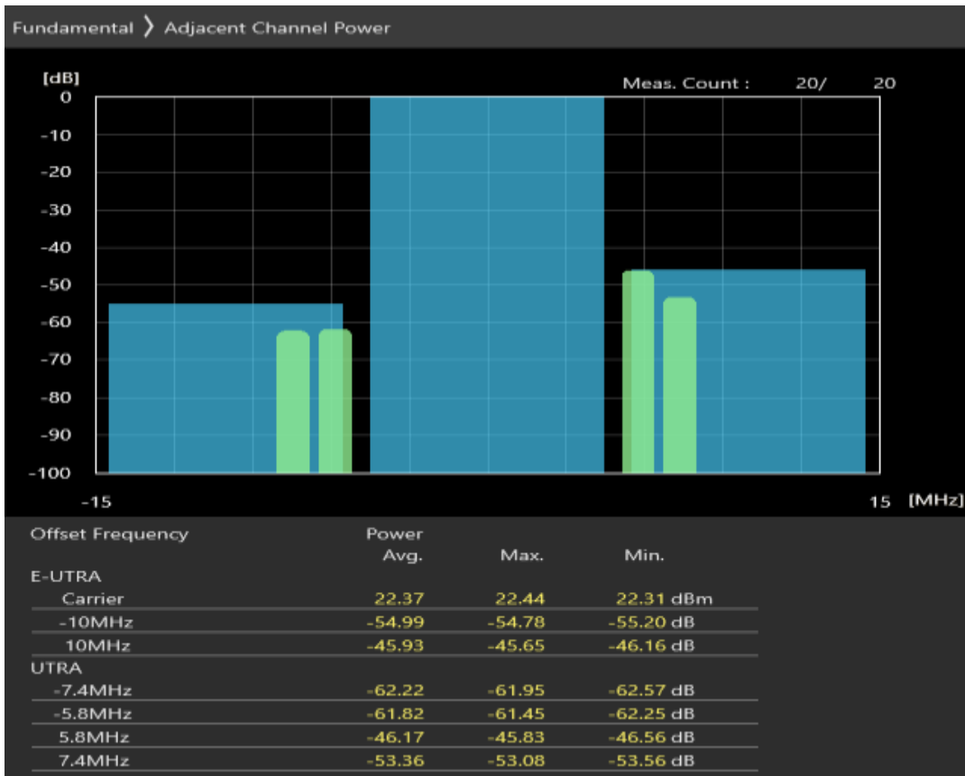
Band40 QPSK BW=10MHz Channel=39600 RB Size=50 Position=#0
