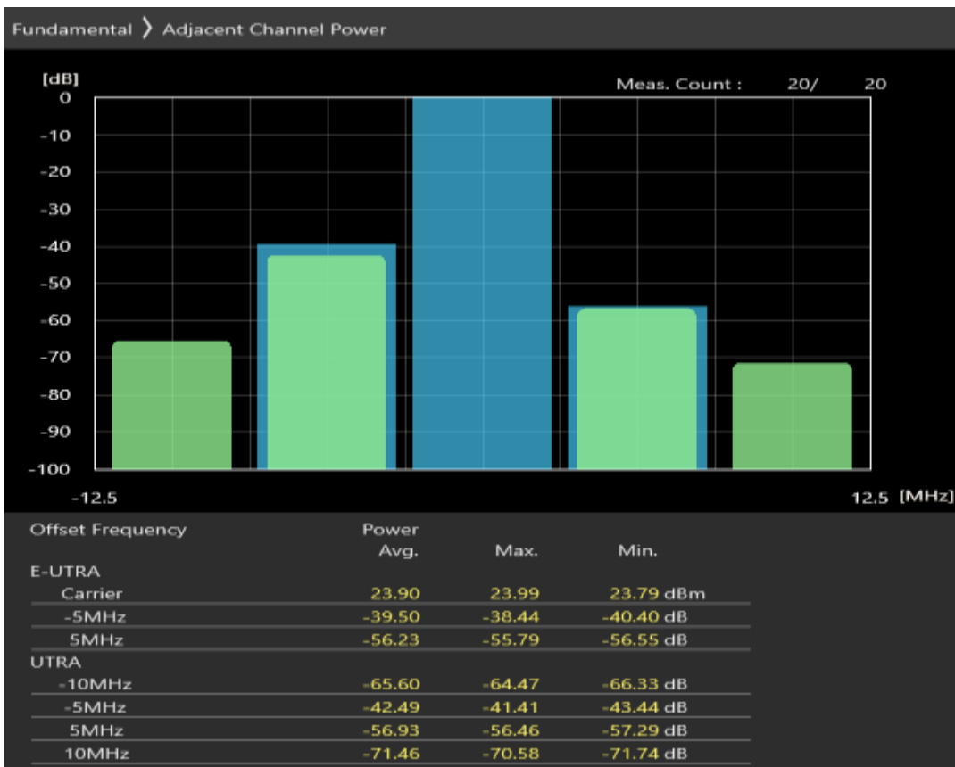
Band1 QPSK BW=5MHz Channel=18575 RB Size=8 Position=#Max
