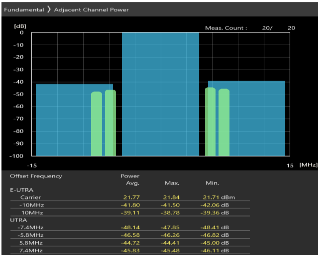
Band40 16QAM BW=10MHz Channel=39150 RB Size=12 Position=#0
