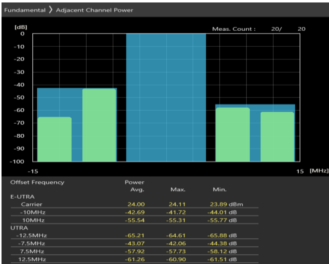
Band20 QPSK BW=10MHz Channel=24200 RB Size=12 Position=#Max
