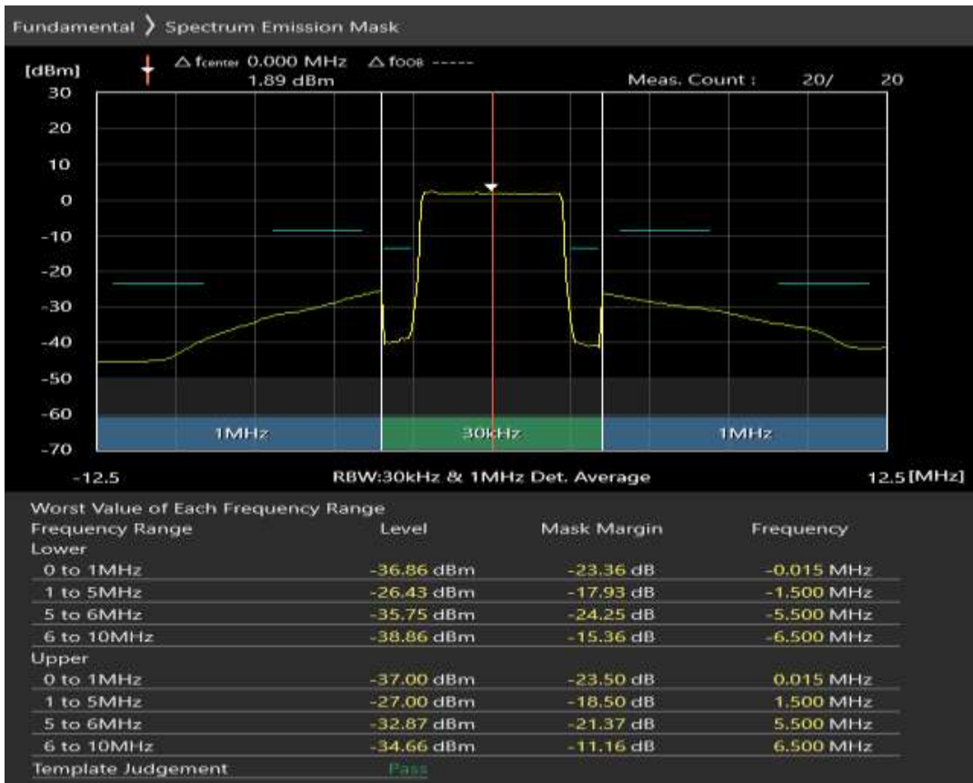
Band20 16QAM BW=5MHz Channel=24175 RB Size=8 Position=#0
