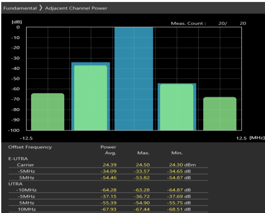
Band7 QPSK BW=5MHz Channel=21100 RB Size=8 Position=#Max
