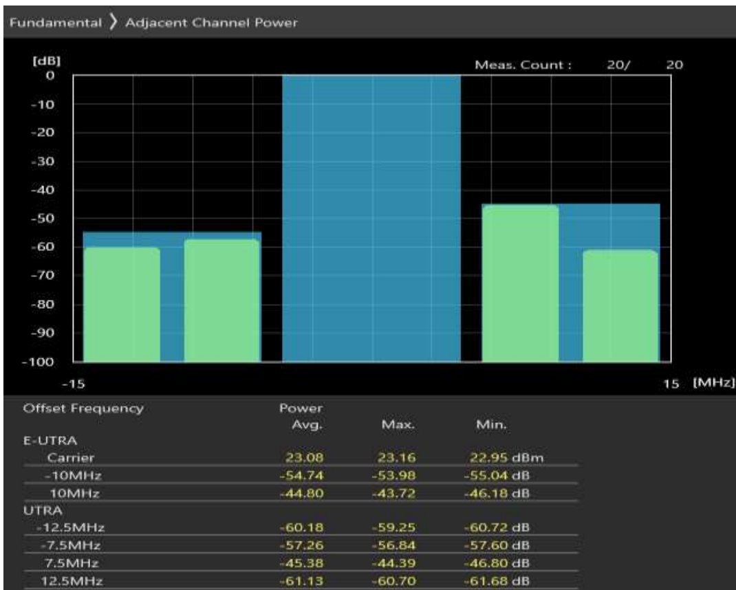
Band1 16QAM BW=10MHz Channel=18300 RB Size=50 Position=#0
