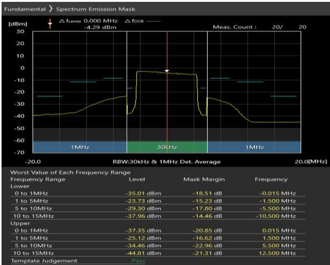
Band8 QAM16 BW=5MHz Channel=21475 RB Size=25 Position=#0
