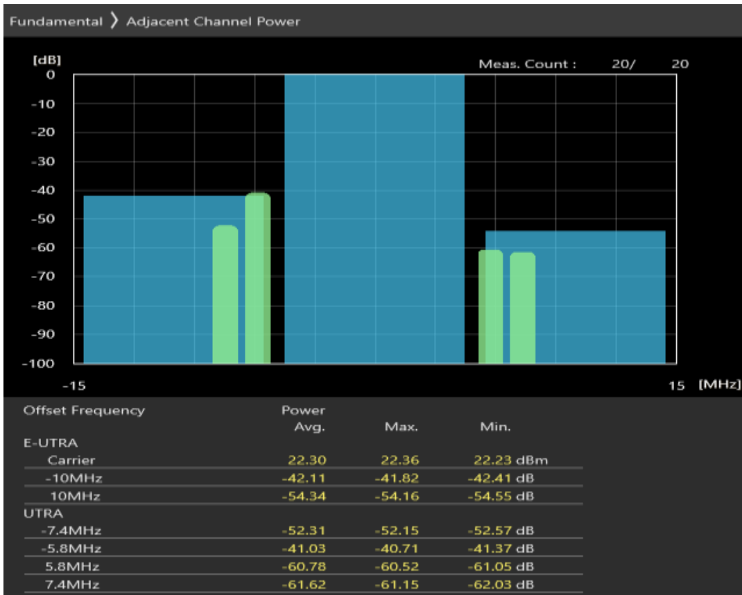
Band40 QPSK BW=10MHz Channel=39150 RB Size=12 Position=#Max
