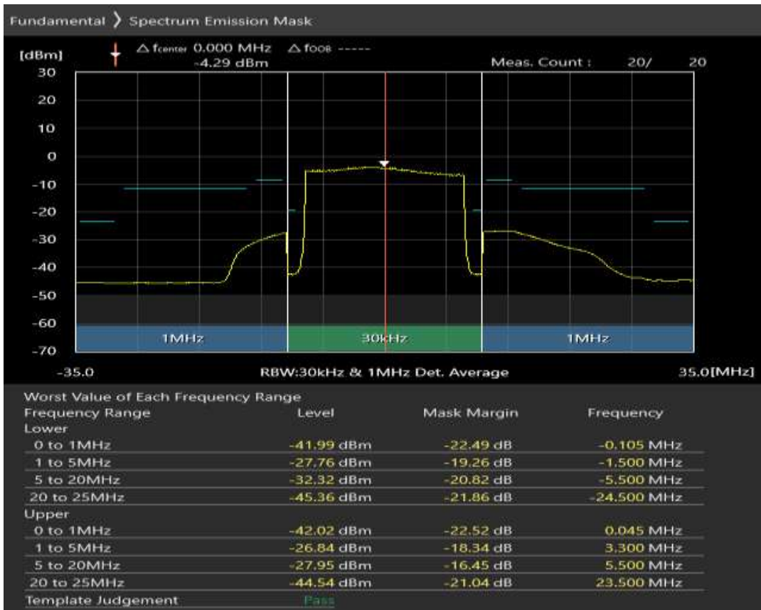
Band20 QPSK BW=20MHz Channel=24300 RB Size=18 Position=#0
