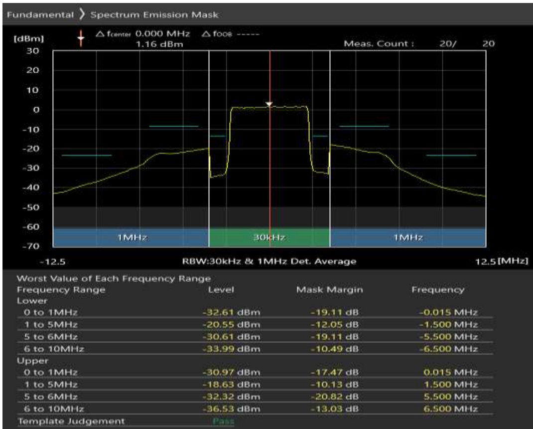
Band3 16QAM BW=5MHz Channel=19925 RB Size=8 Position=#0
