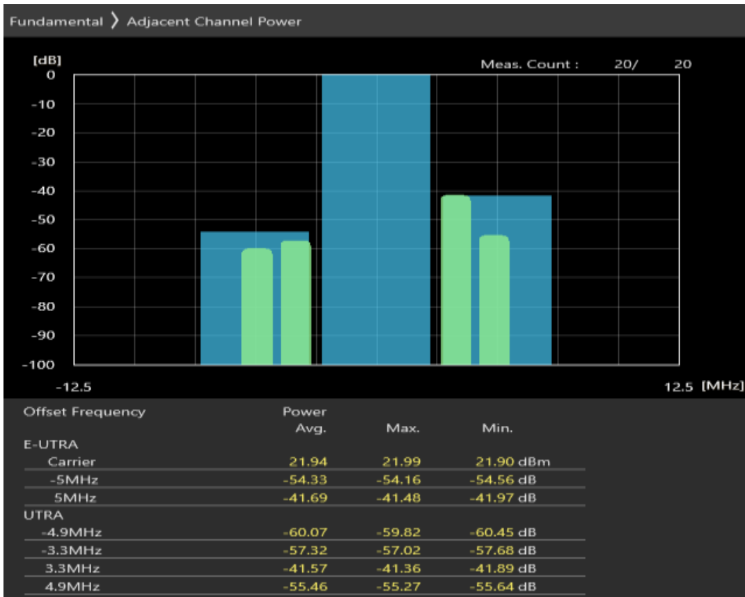
Band40 16QAM BW=5MHz Channel=38675 RB Size=25 Position=#0
