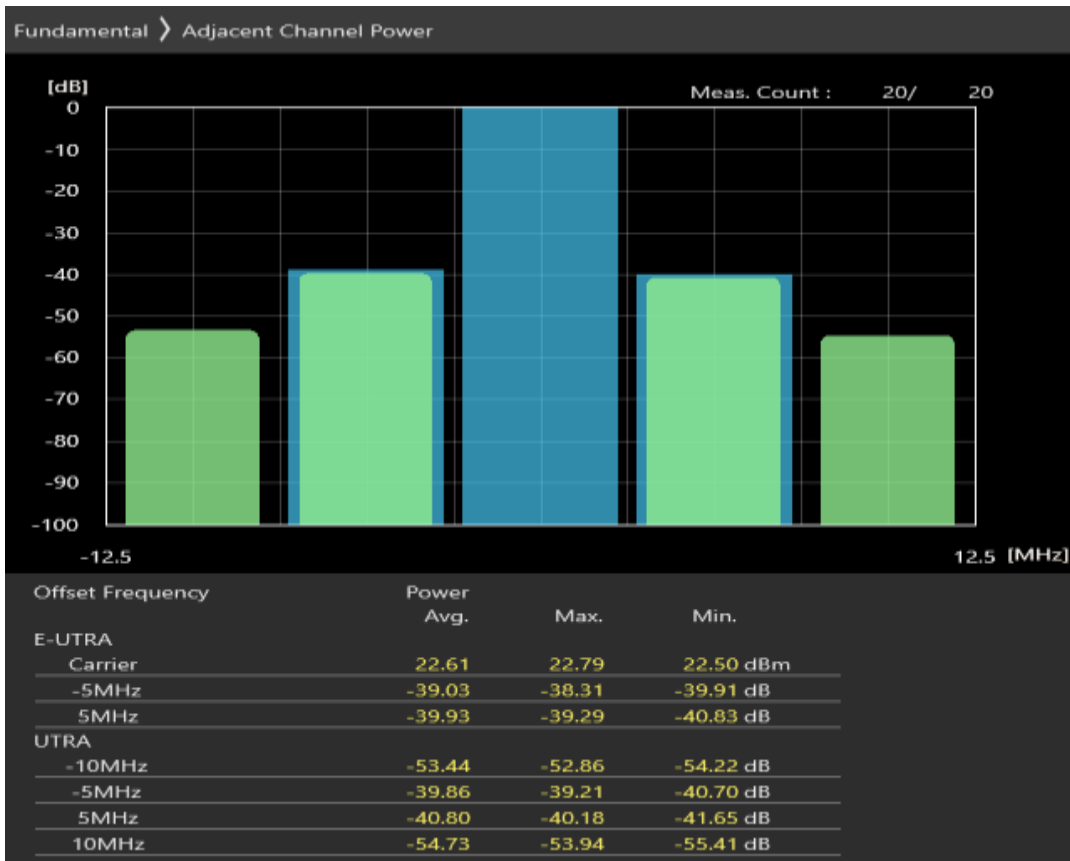
Band7 QPSK BW=10MHz Channel=20800 RB Size=12 Position=#0
