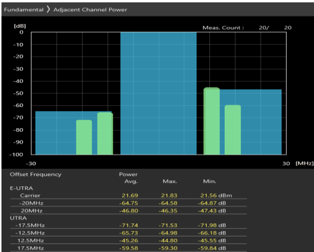
Band28 16QAM BW=20MHz Channel=27310 RB Size=100 Position=#0
