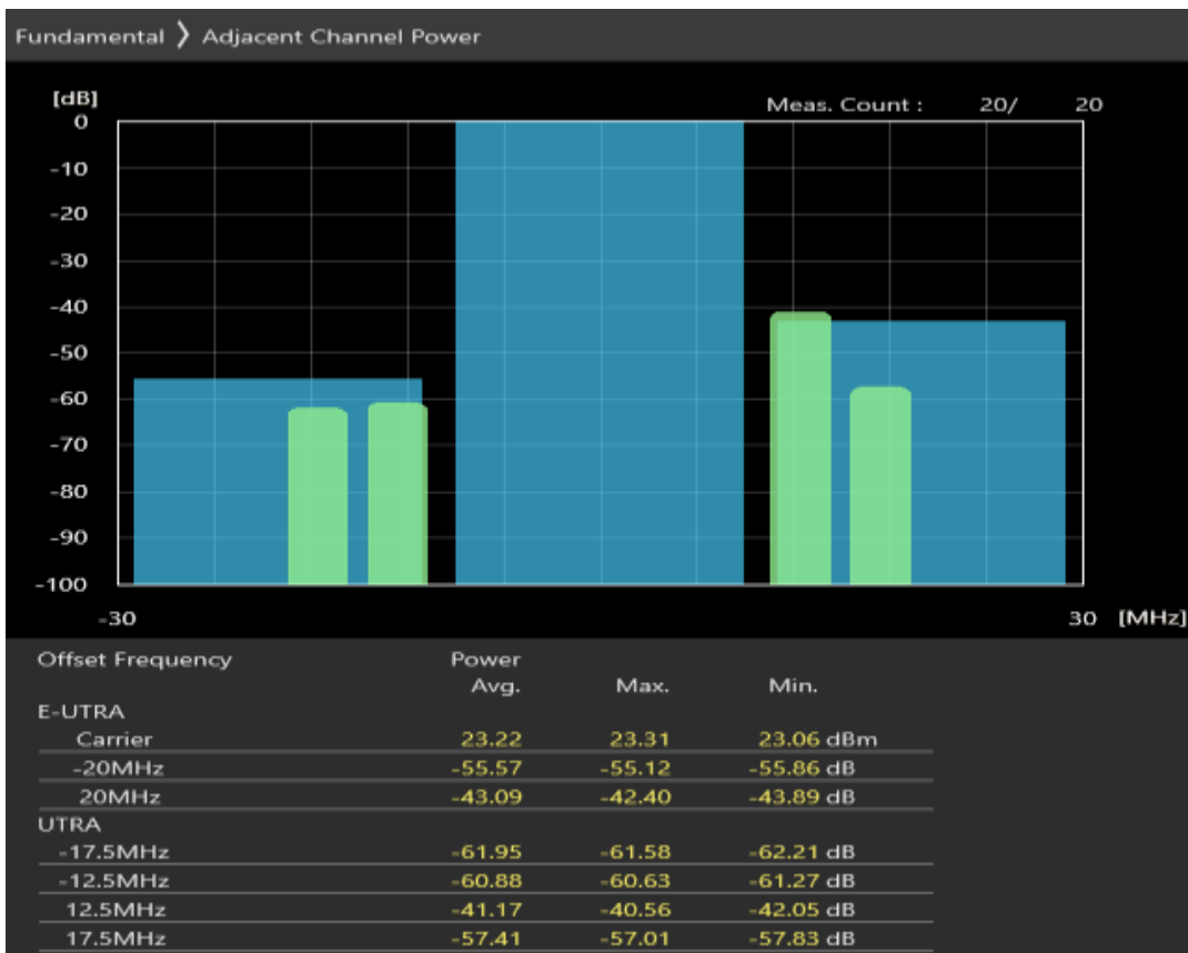
Band7 16QAM BW=20MHz Channel=21350 RB Size=100 Position=#0
