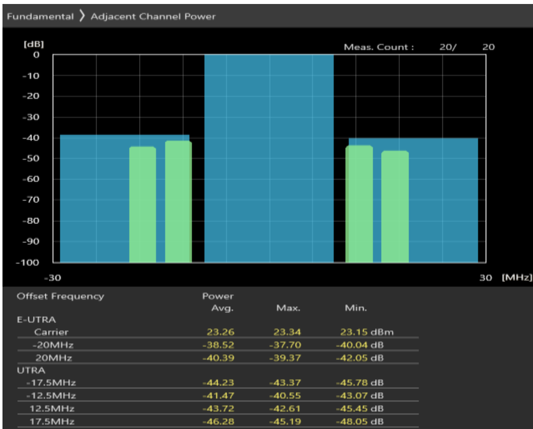
Band1 16QAM BW=20MHz Channel=18300 RB Size=18 Position=#0
