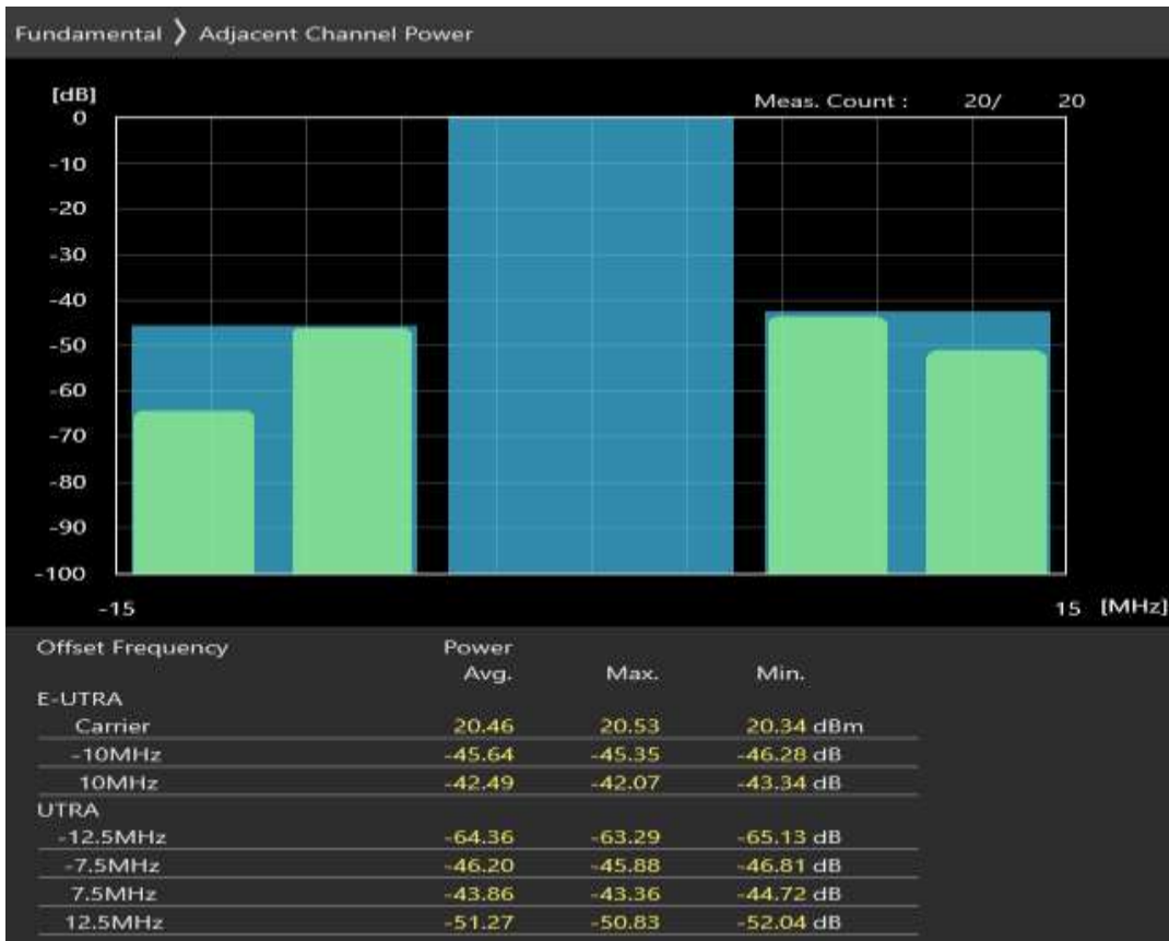
Band8 QAM16 BW=10MHz Channel=21625 RB Size=12 Position=#0
