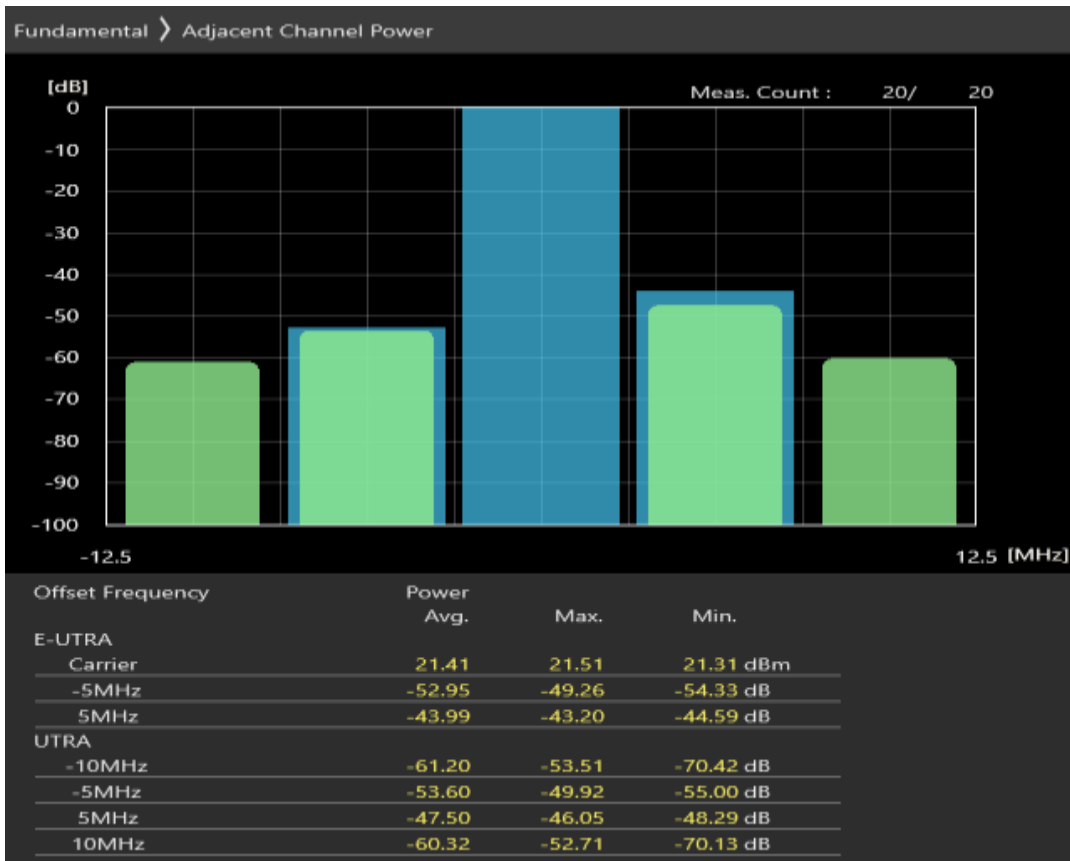
Band8 QAM16 BW=5MHz Channel=21775 RB Size=25 Position=#0
