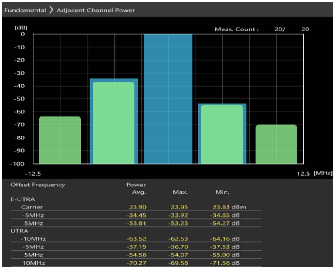
Band20 QPSK BW=5MHz Channel=24300 RB Size=8 Position=#Max
