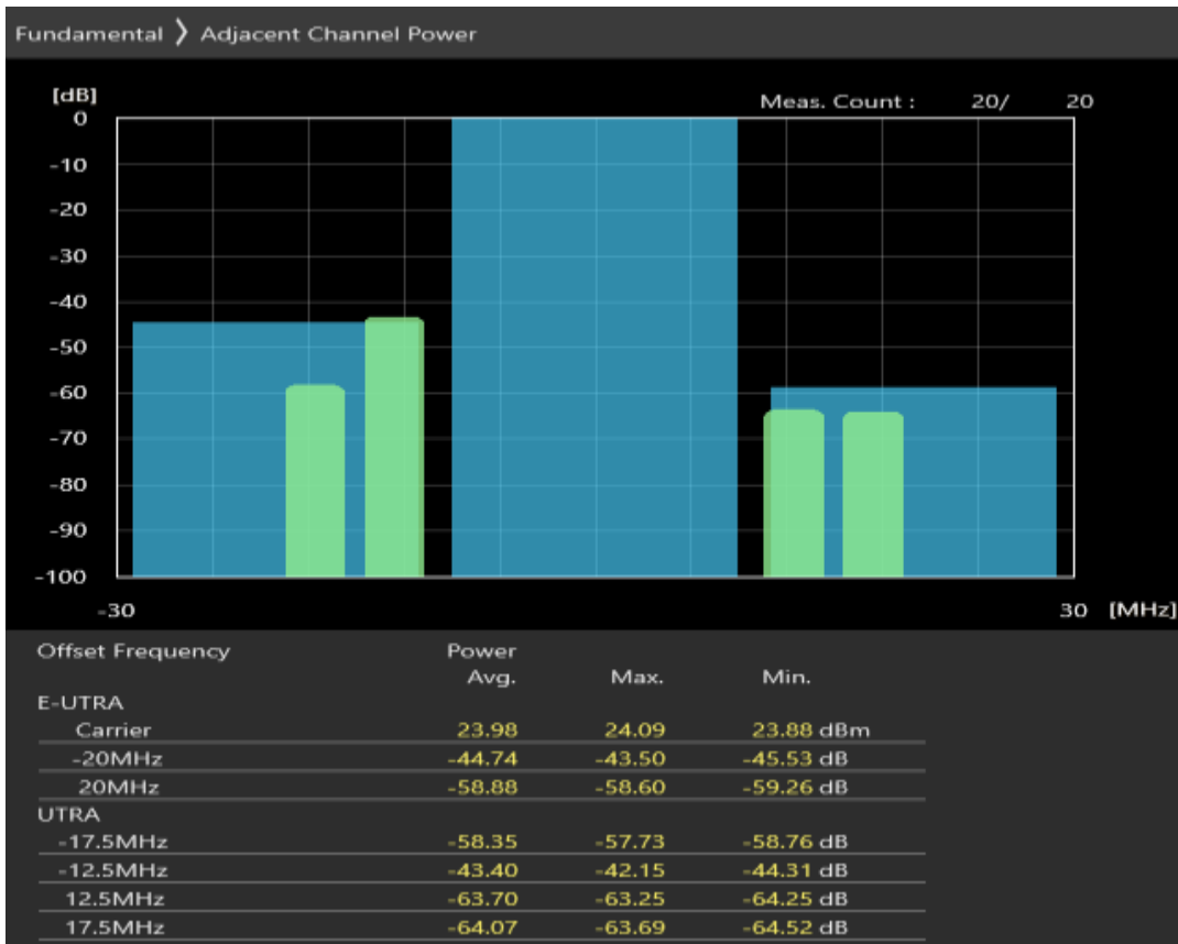
Band20 QPSK BW=20MHz Channel=24300 RB Size=18 Position=#Max
