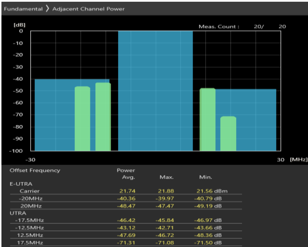
Band28 16QAM BW=20MHz Channel=27560 RB Size=18 Position=#0
