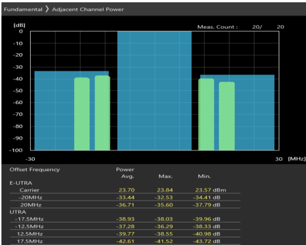
Band7 16QAM BW=20MHz Channel=21100 RB Size=18 Position=#0
