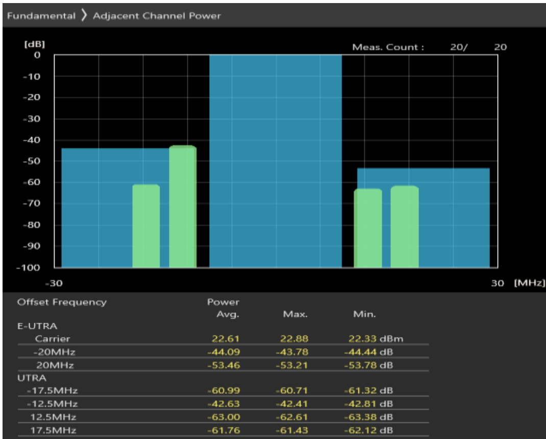
Band3 16QAM BW=20MHz Channel=19575 RB Size=18 Position=#Max
