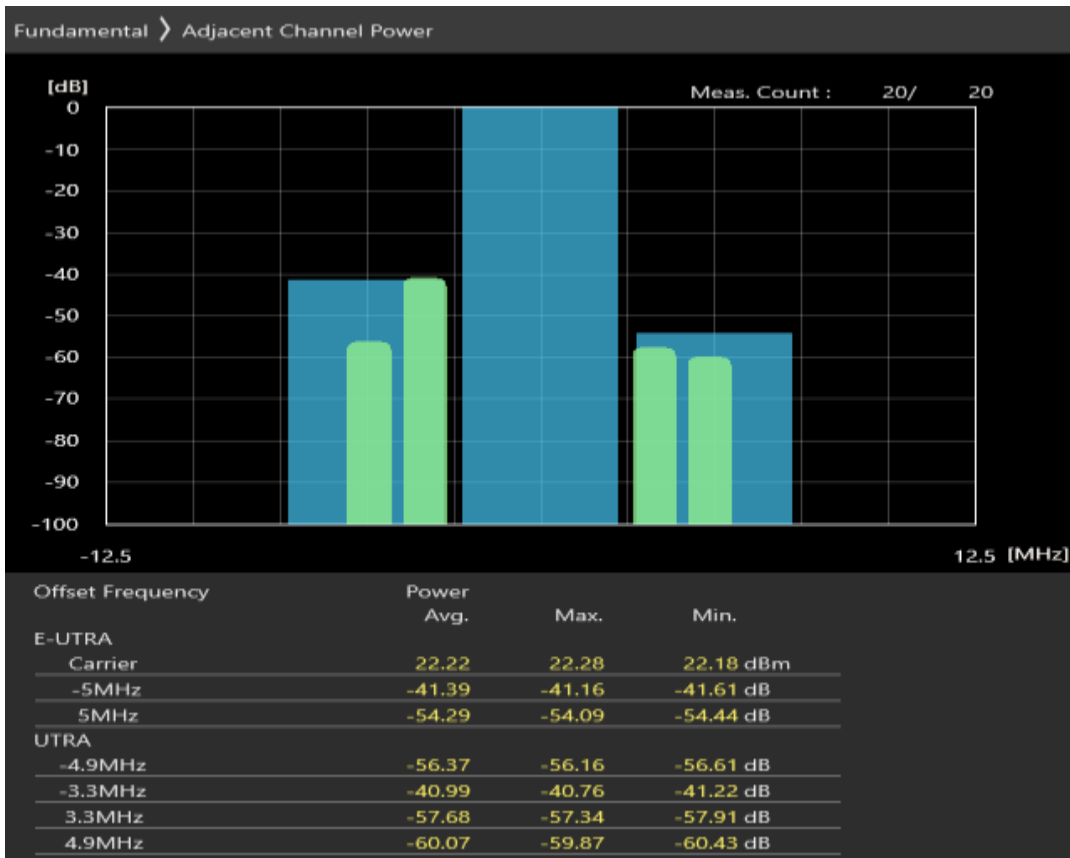
Band40 QPSK BW=5MHz Channel=39150 RB Size=8 Position=#Max
