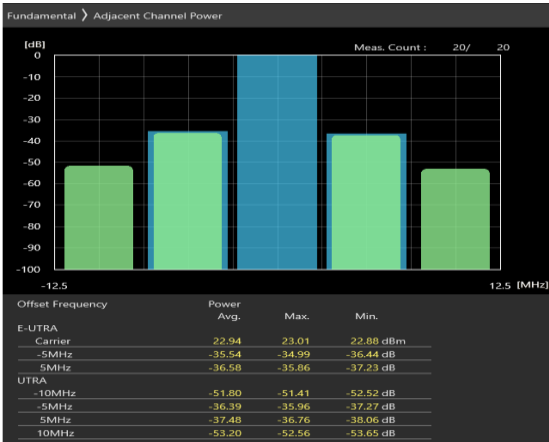
Band7 QPSK BW=5MHz Channel=21425 RB Size=8 Position=#0
