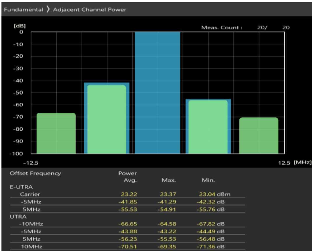
Band3 QPSK BW=5MHz Channel=19575 RB Size=8 Position=#Max
