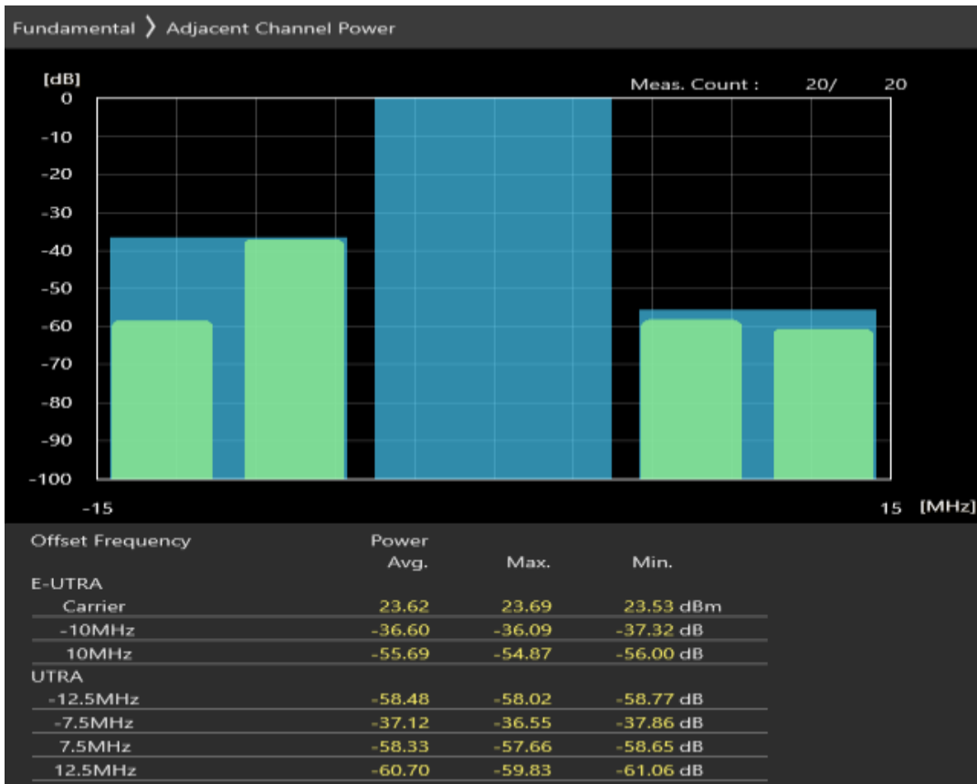
Band7 16QAM BW=10MHz Channel=21100 RB Size=12 Position=#Max
