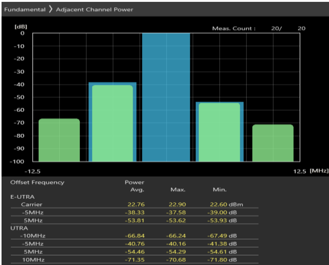
Band3 16QAM BW=5MHz Channel=19925 RB Size=8 Position=#Max
