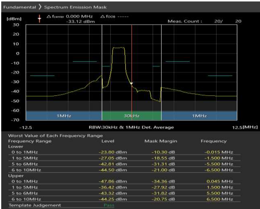
Band8 QPSK BW=5MHz Channel=21475 RB Size=8 Position=#Max
