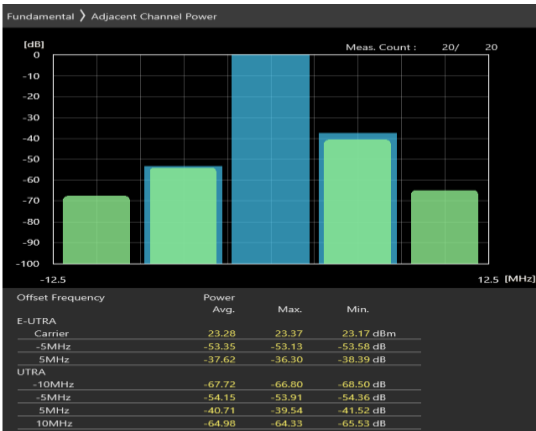
Band7 16QAM BW=5MHz Channel=21425 RB Size=25 Position=#0
