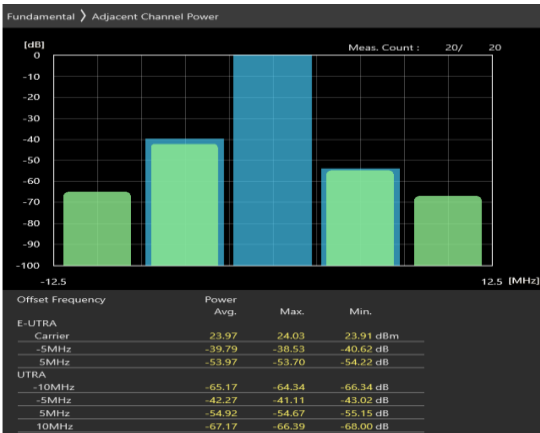
Band7 QPSK BW=5MHz Channel=20775 RB Size=8 Position=#Max
