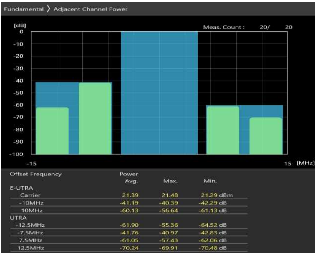
Band8 QAM16 BW=10MHz Channel=21750 RB Size=12 Position=#Max
