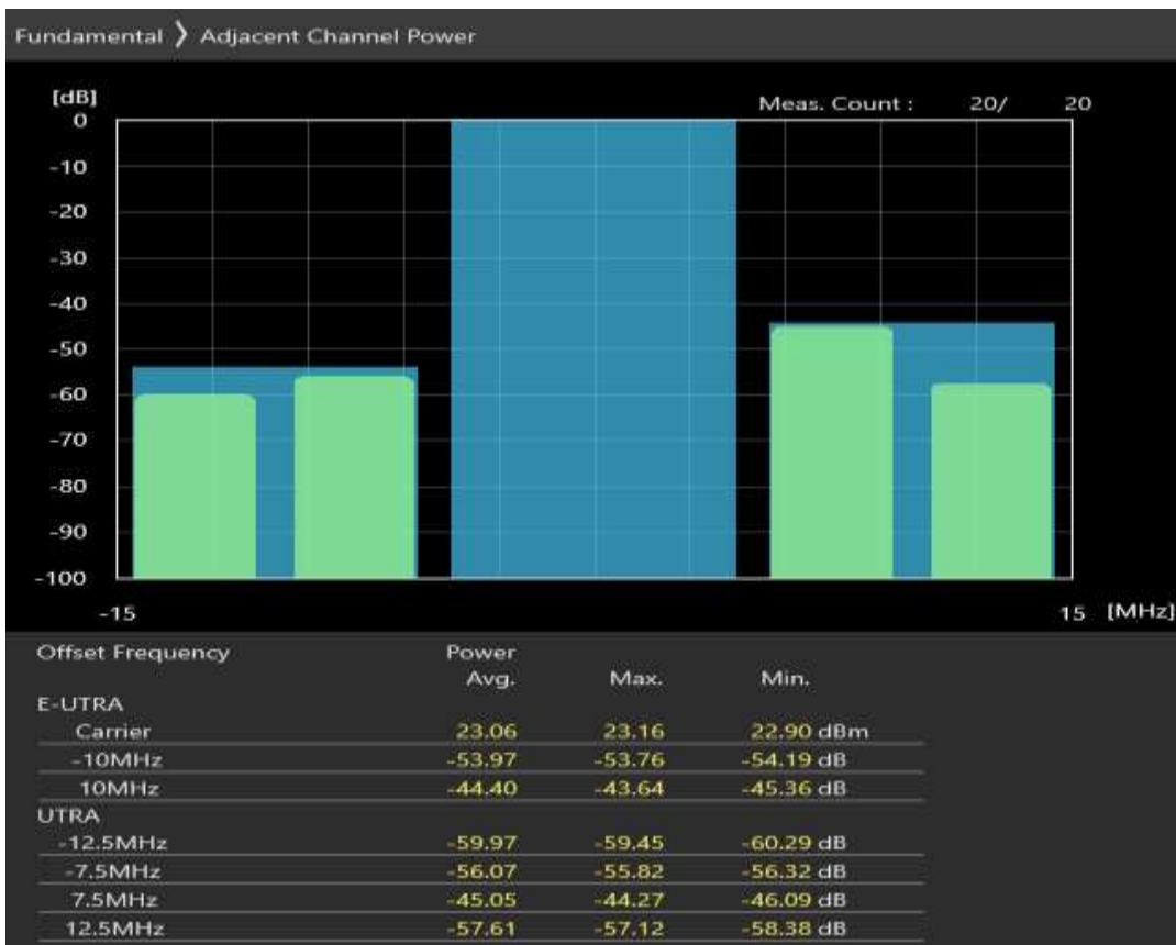
Band20 16QAM BW=10MHz Channel=24300 RB Size=50 Position=#0
