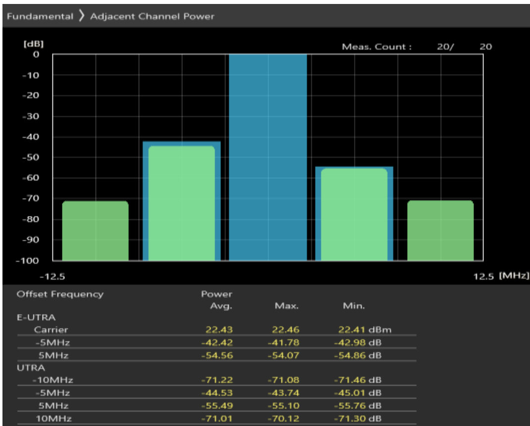
Band8 QPSK BW=5MHz Channel=21475 RB Size=8 Position=#Max
