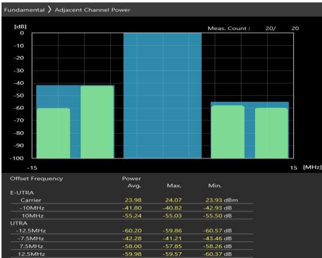
Band7 QPSK BW=10MHz Channel=20800 RB Size=12 Position=#Max
