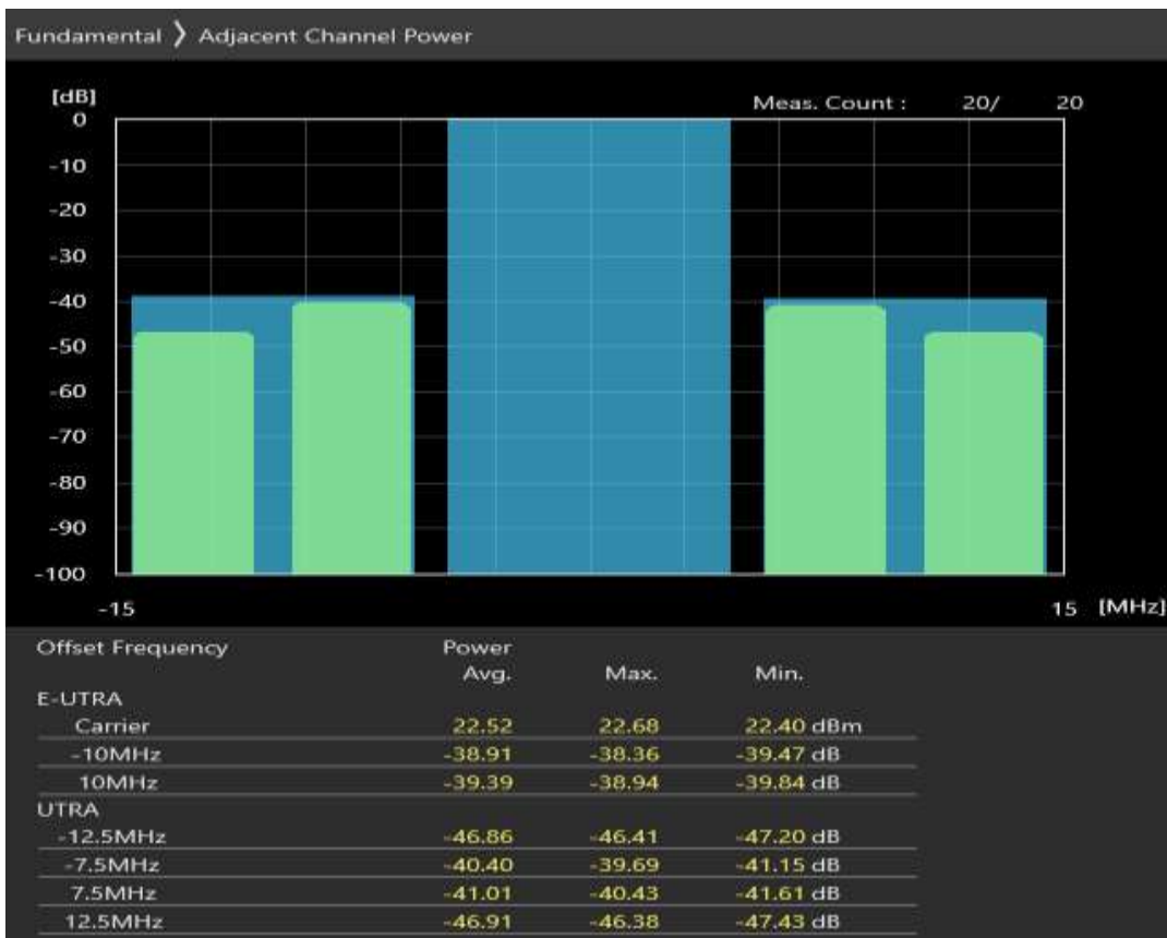
Band3 16QAM BW=10MHz Channel=19575 RB Size=12 Position=#0
