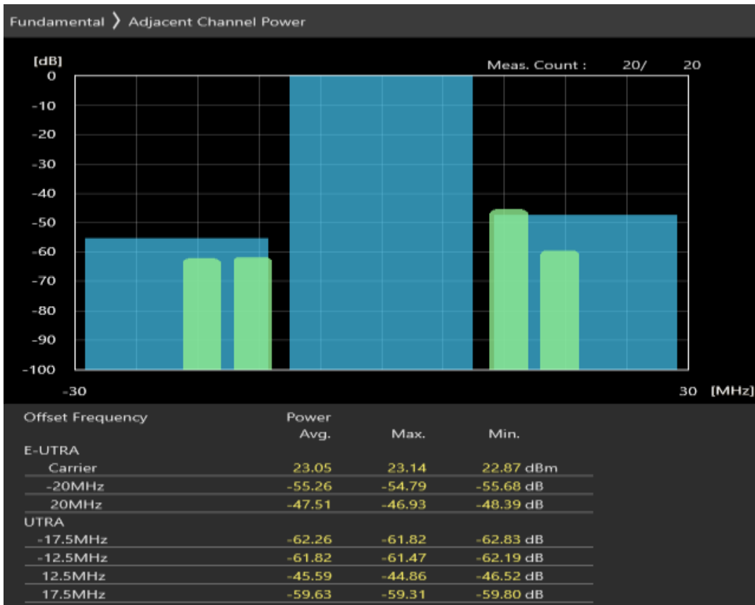
Band1 16QAM BW=20MHz Channel=18500 RB Size=100 Position=#0
