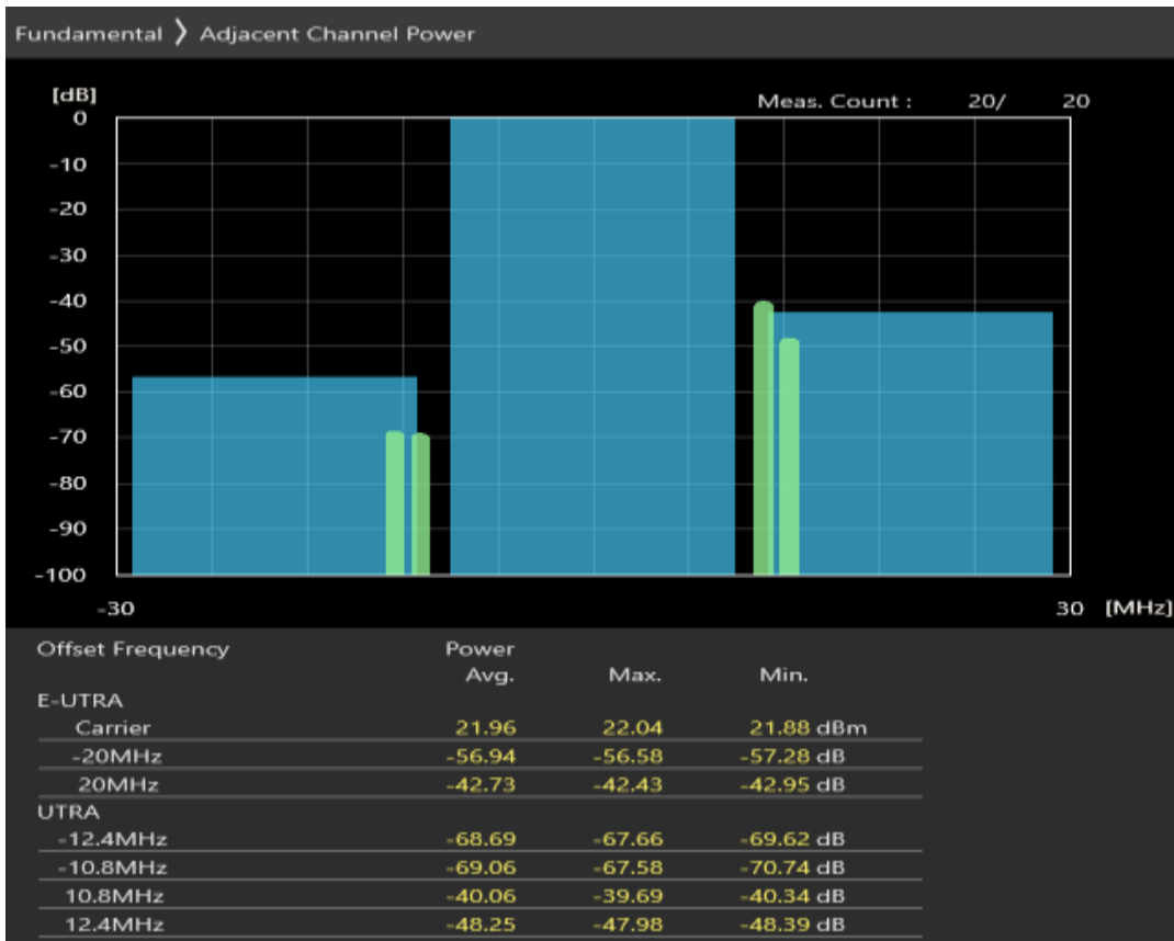
Band40 16QAM BW=20MHz Channel=39150 RB Size=100 Position=#0
