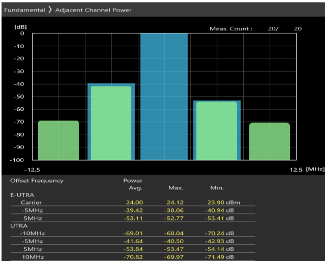
Band20 QPSK BW=5MHz Channel=24175 RB Size=8 Position=#Max
