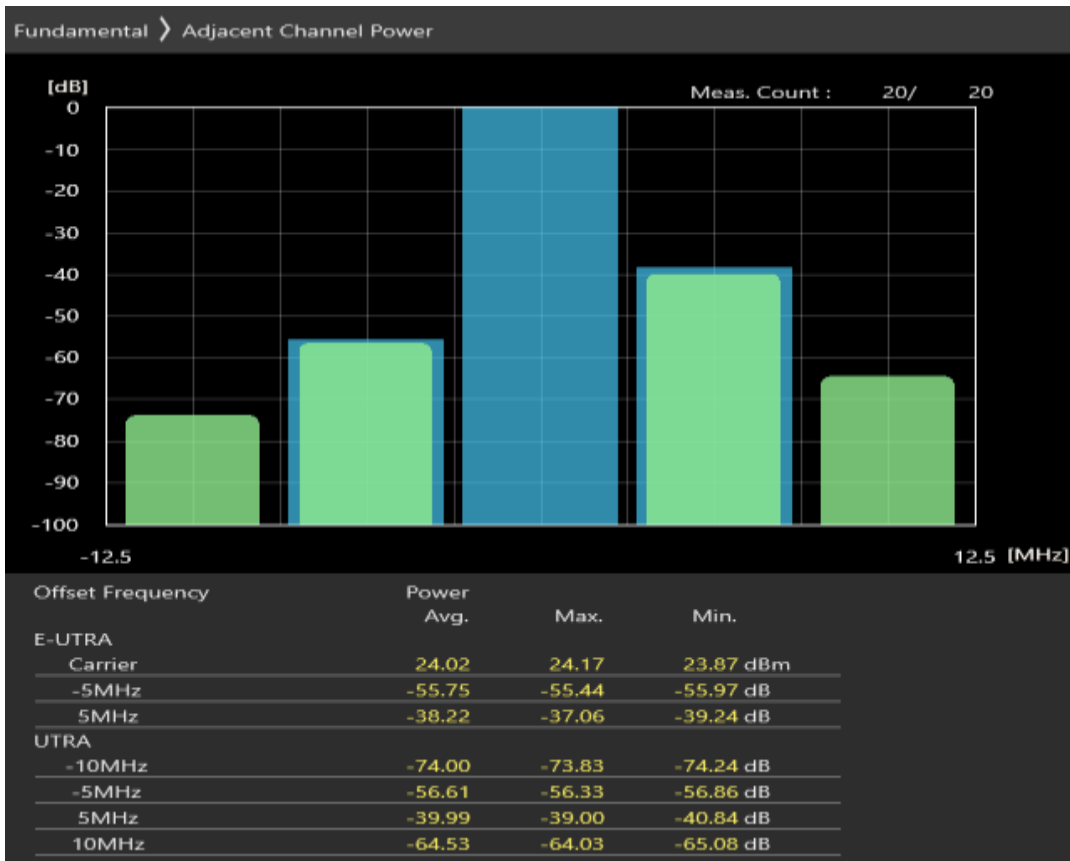
Band28 QPSK BW=5MHz Channel=27235 RB Size=25 Position=#0
