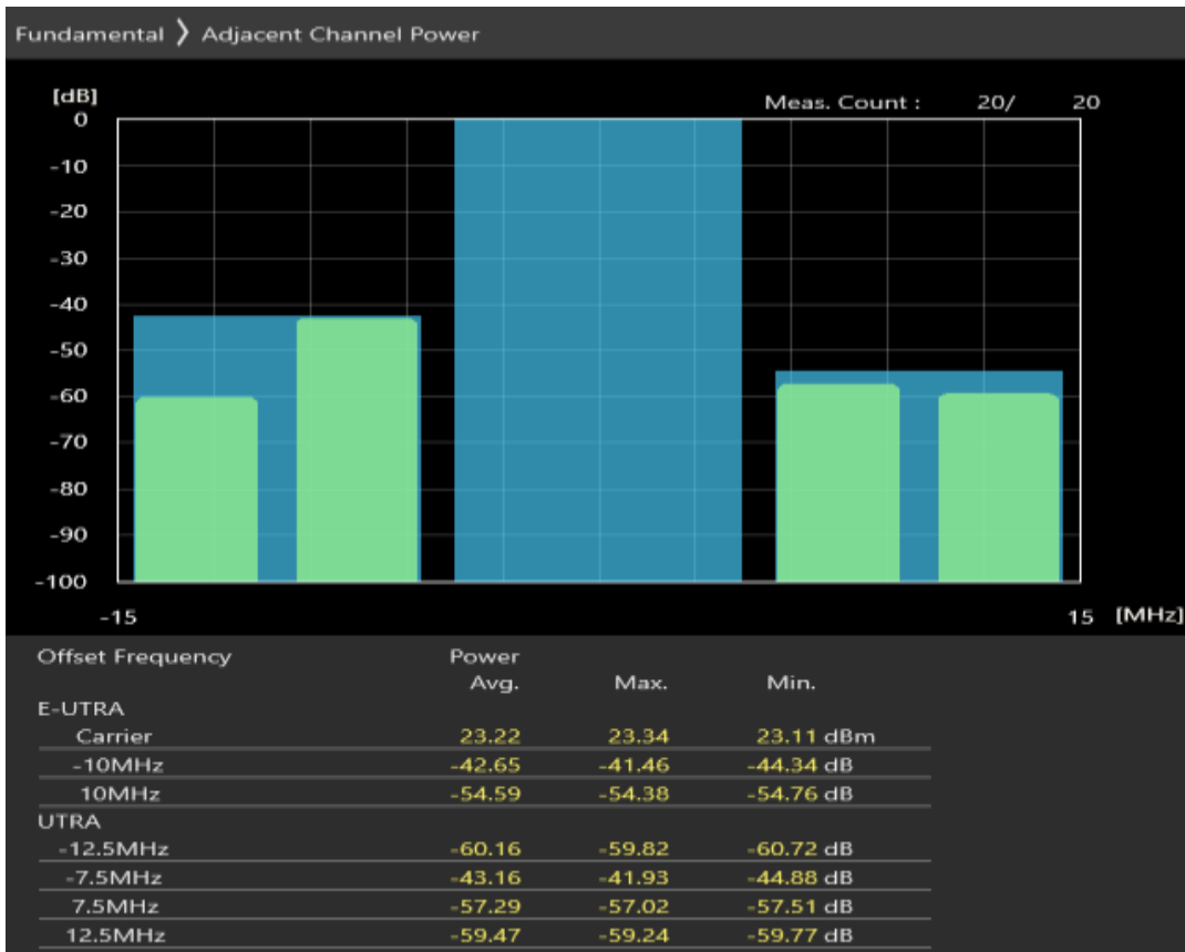
Band7 16QAM BW=10MHz Channel=20800 RB Size=12 Position=#Max
