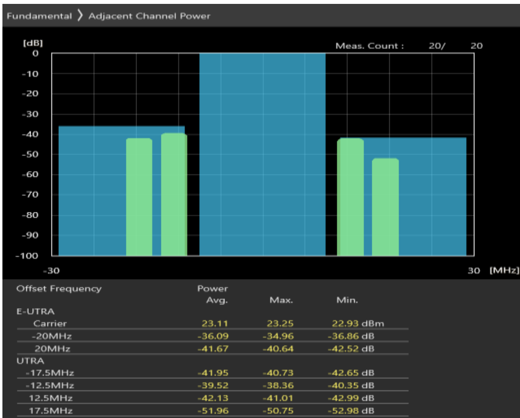
Band20 16QAM BW=20MHz Channel=24350 RB Size=18 Position=#0
