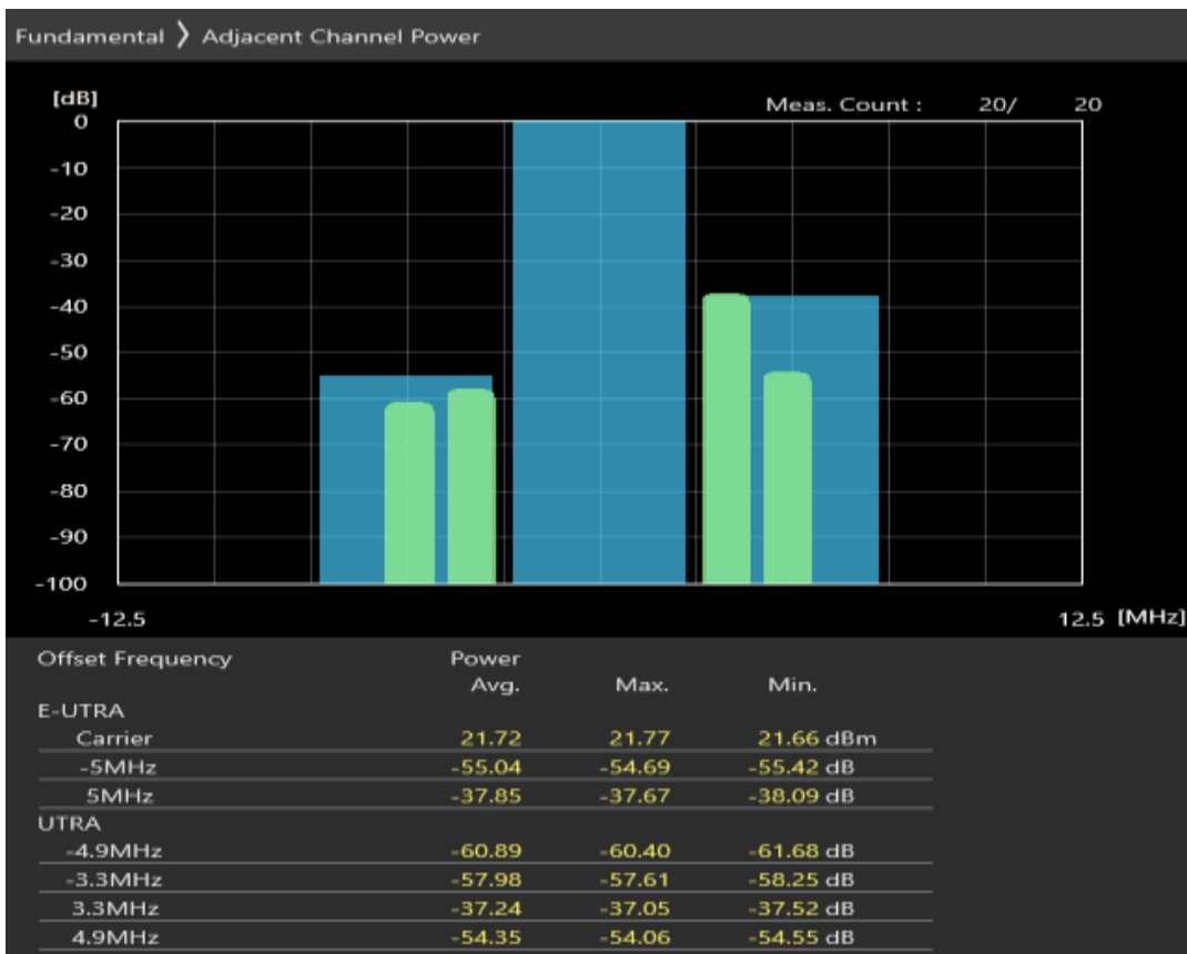
Band40 16QAM BW=5MHz Channel=39150 RB Size=25 Position=#0
