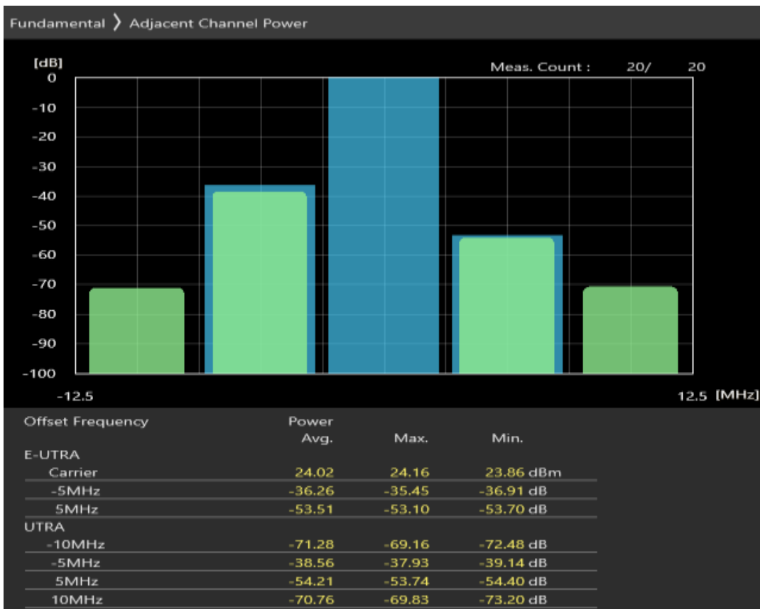
Band28 QPSK BW=5MHz Channel=27235 RB Size=8 Position=#Max
