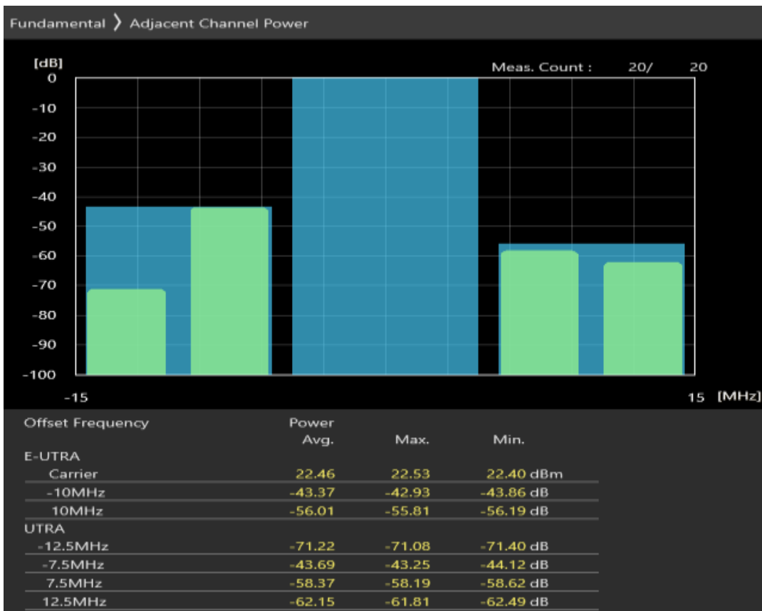
Band8 QPSK BW=10MHz Channel=21500 RB Size=12 Position=#Max
