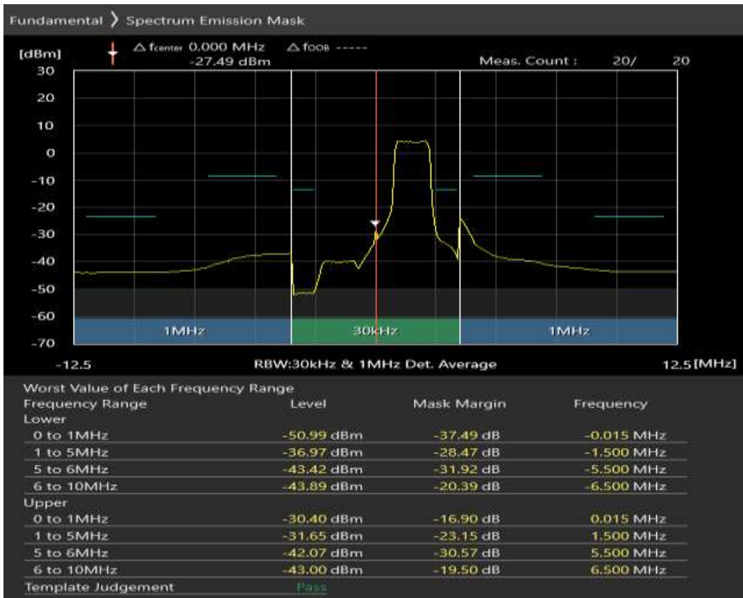
Band3 16QAM BW=5MHz Channel=19225 RB Size=25 Position=#0
