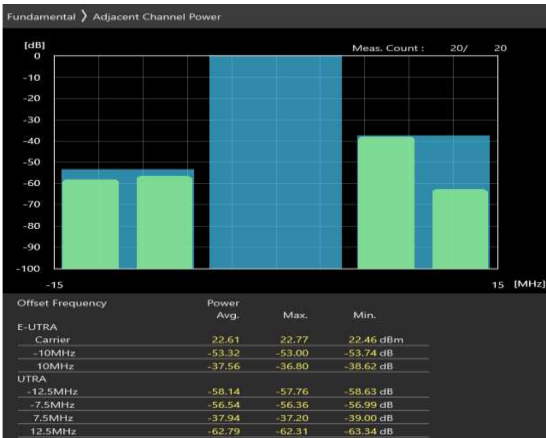
Band3 16QAM BW=10MHz Channel=1990 RB Size=50 Position=#0
