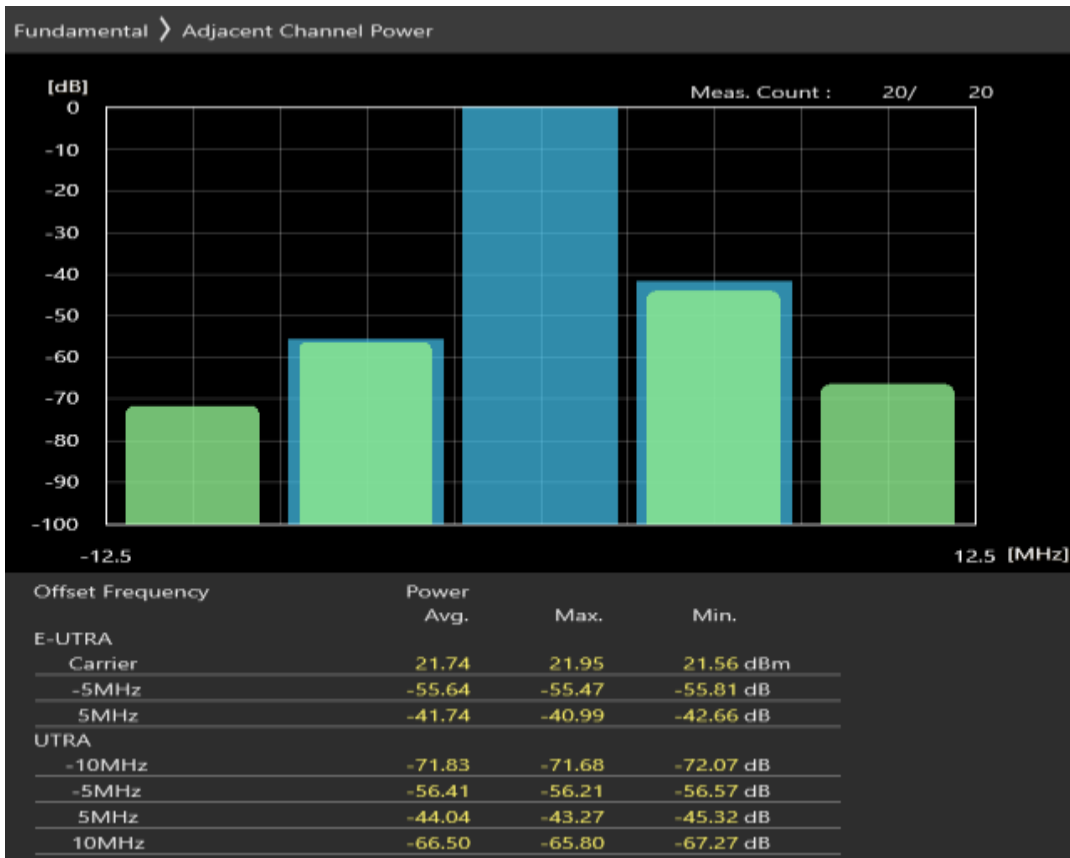
Band28 16QAM BW=5MHz Channel=27235 RB Size=25 Position=#0
