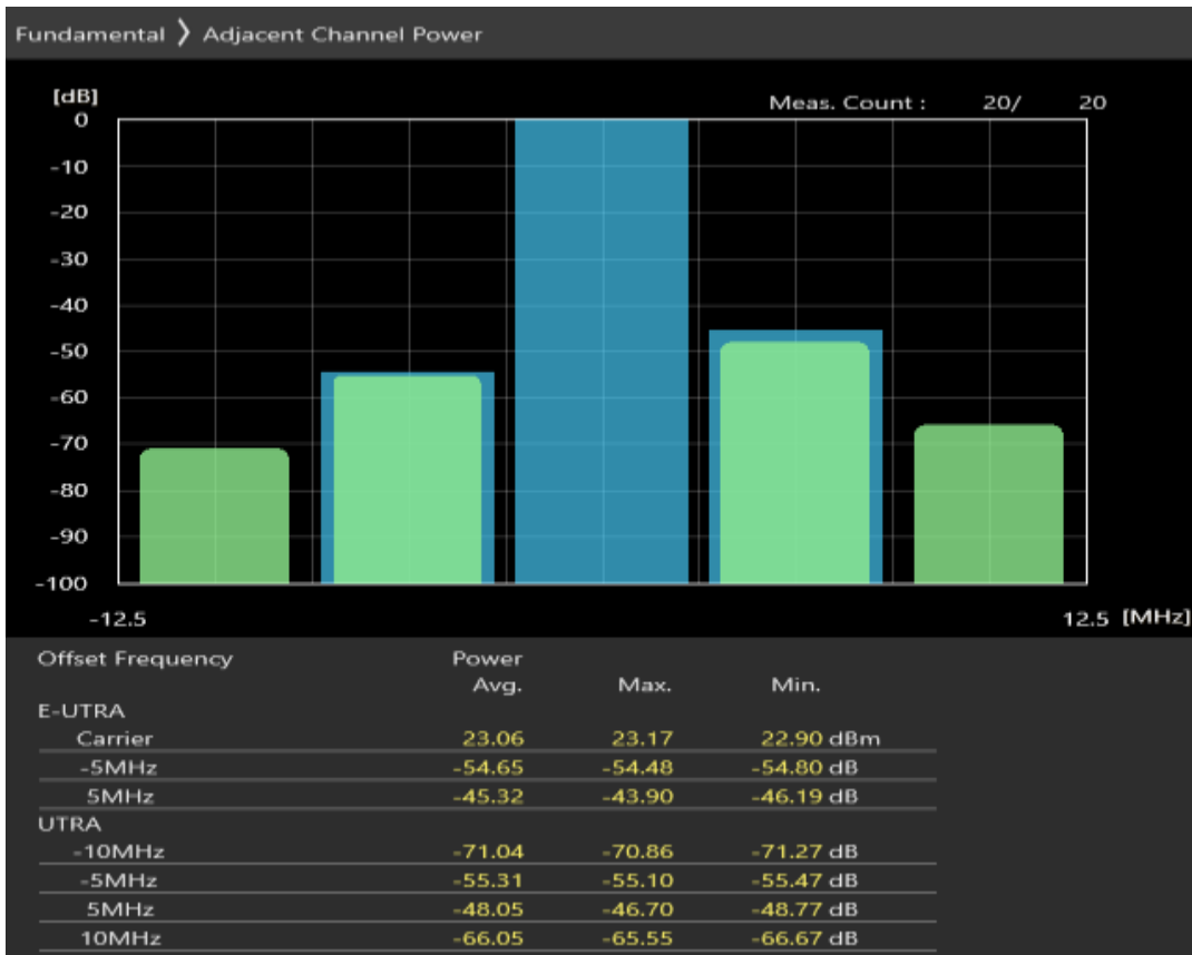
Band1 16QAM BW=5MHz Channel=18025 RB Size=25 Position=#0
