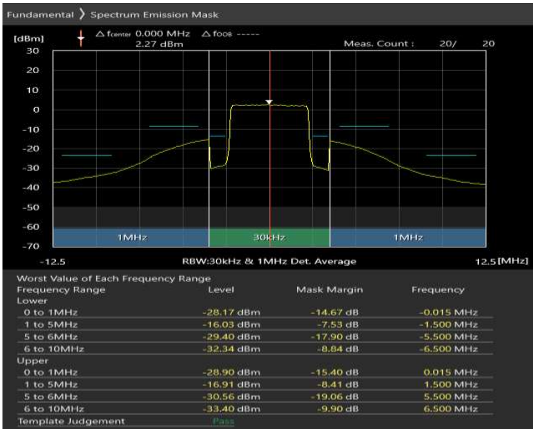
Band7 16QAM BW=5MHz Channel=21100 RB Size=8 Position=#0
