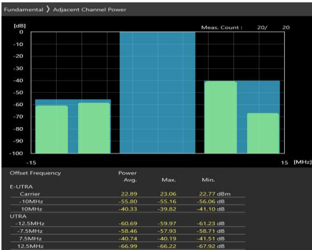
Band20 16QAM BW=10MHz Channel=24400 RB Size=50 Position=#0
