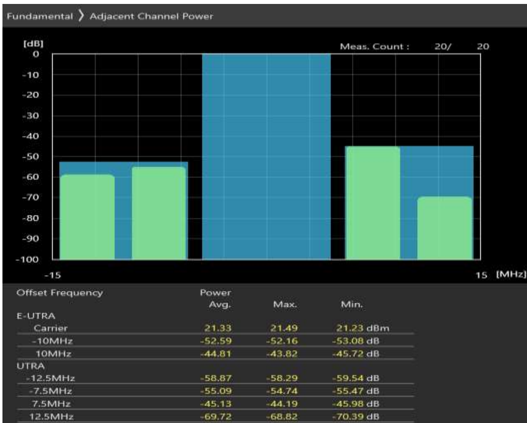
Band8 QAM16 BW=10MHz Channel=21750 RB Size=50 Position=#0
