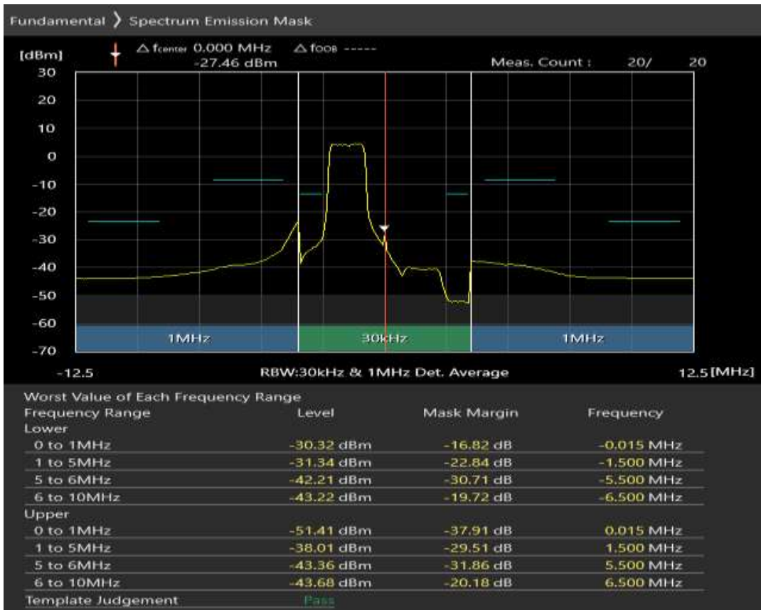
Band3 16QAM BW=5MHz Channel=19225 RB Size=8 Position=#Max
