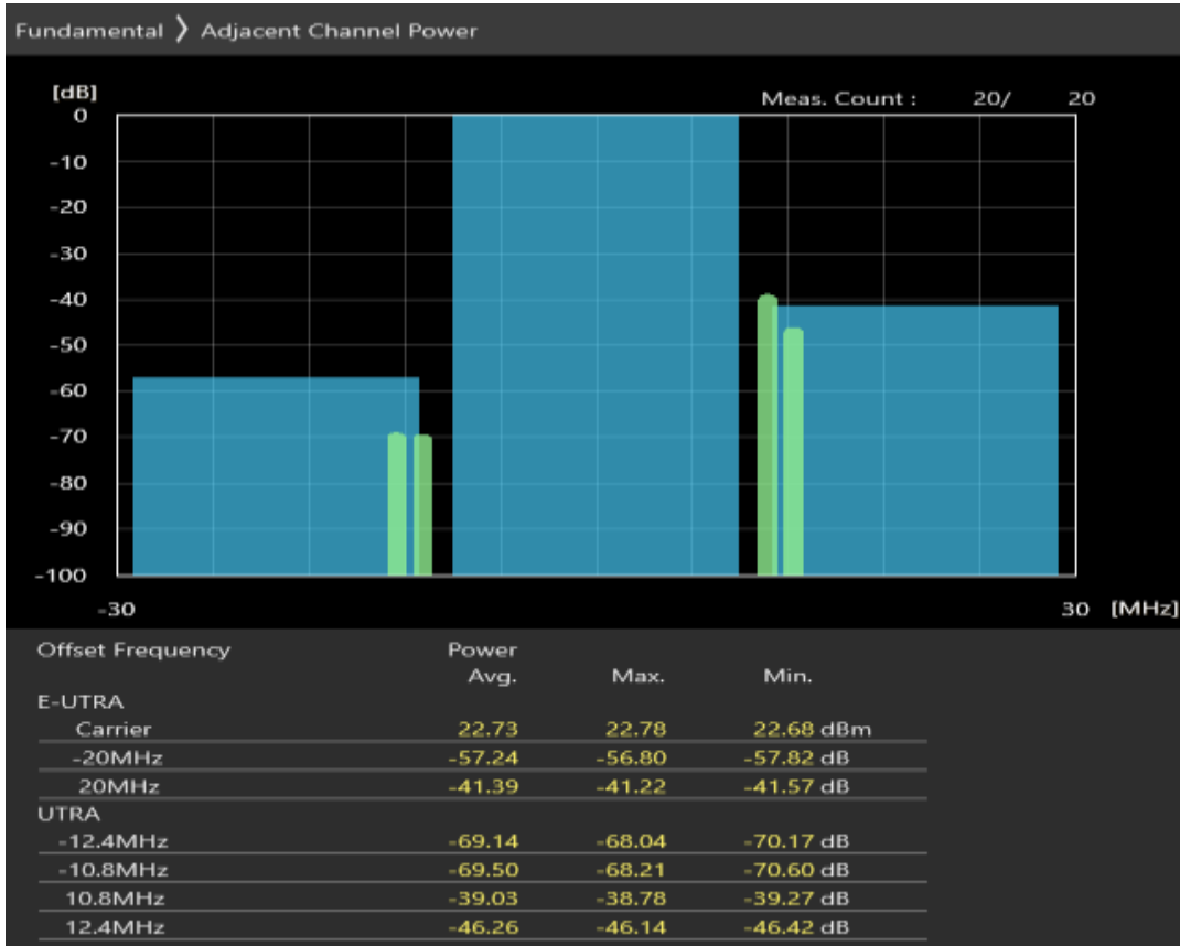
Band40 QPSK BW=20MHz Channel=39150 RB Size=100 Position=#0
