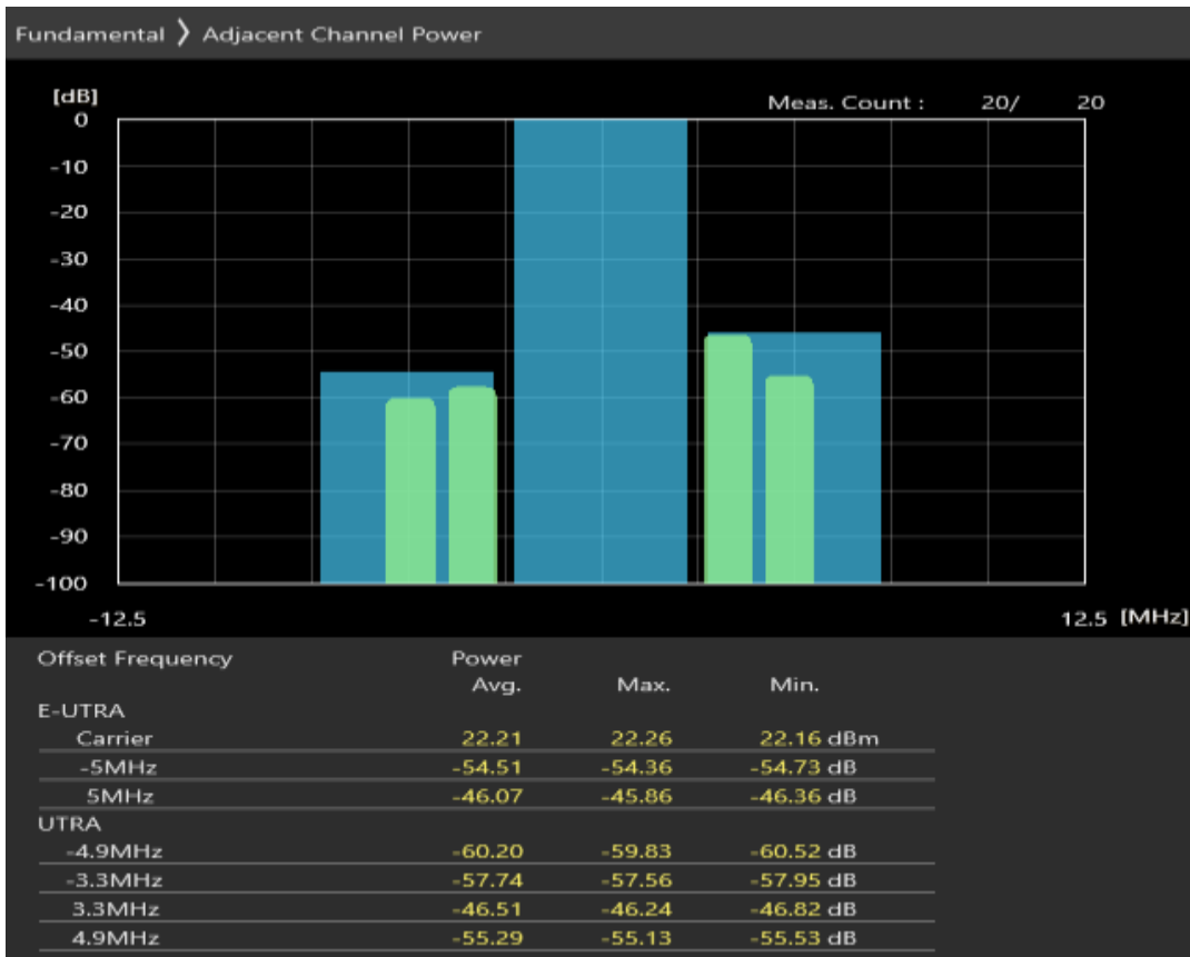
Band40 QPSK BW=5MHz Channel=39625 RB Size=25 Position=#0
