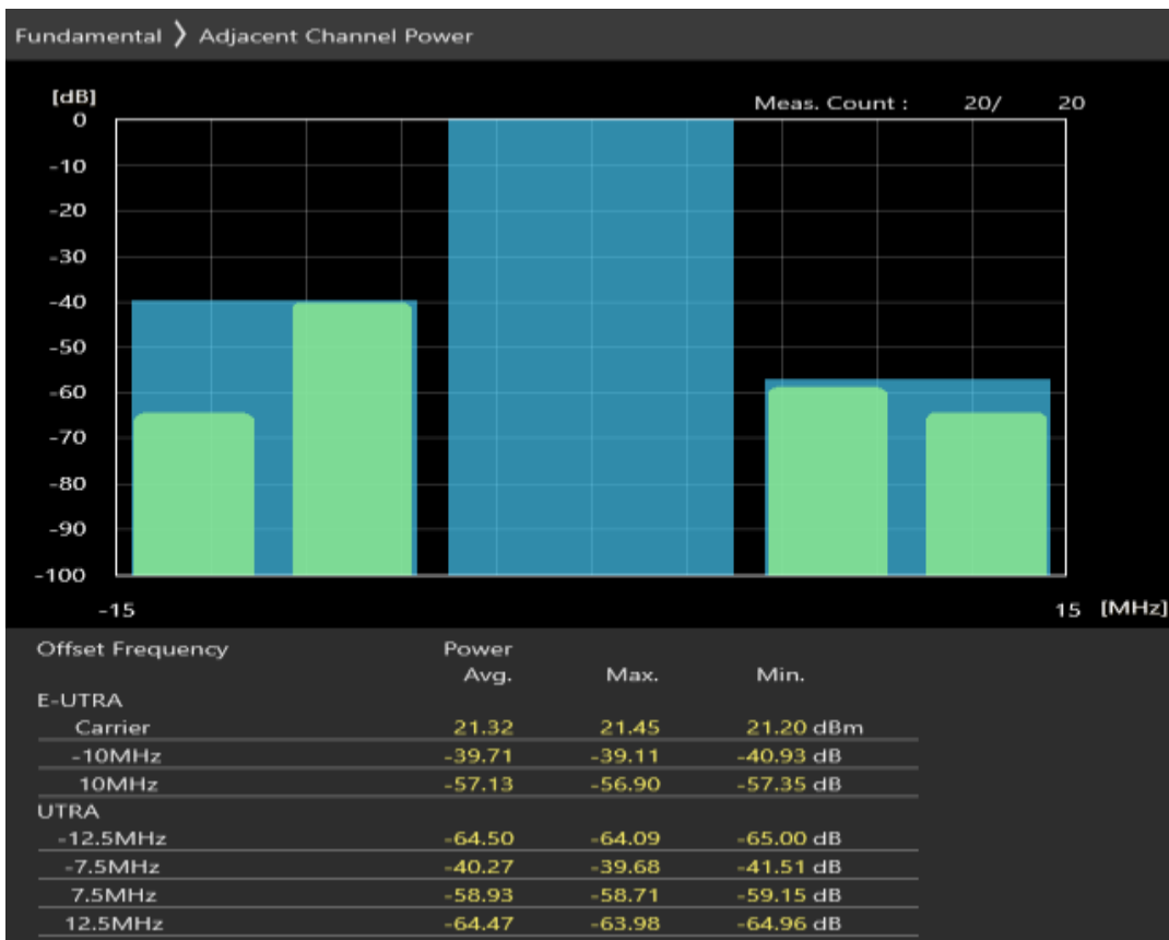
Band8 QAM16 BW=10MHz Channel=21625 RB Size=12 Position=#Max
