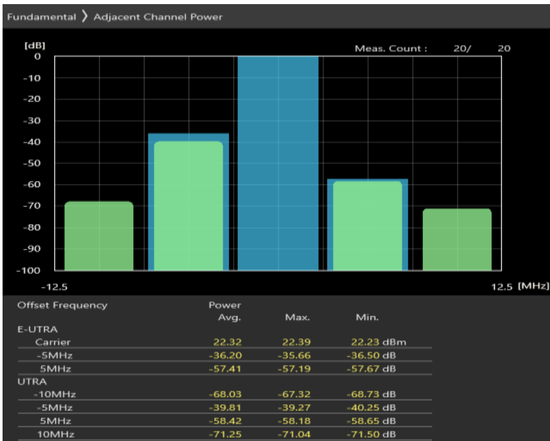
Band8 QPSK BW=5MHz Channel=21775 RB Size=8 Position=#Max
