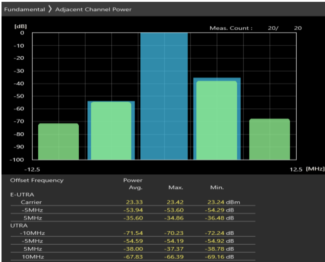
Band3 QPSK BW=5MHz Channel=19925 RB Size=25 Position=#0
