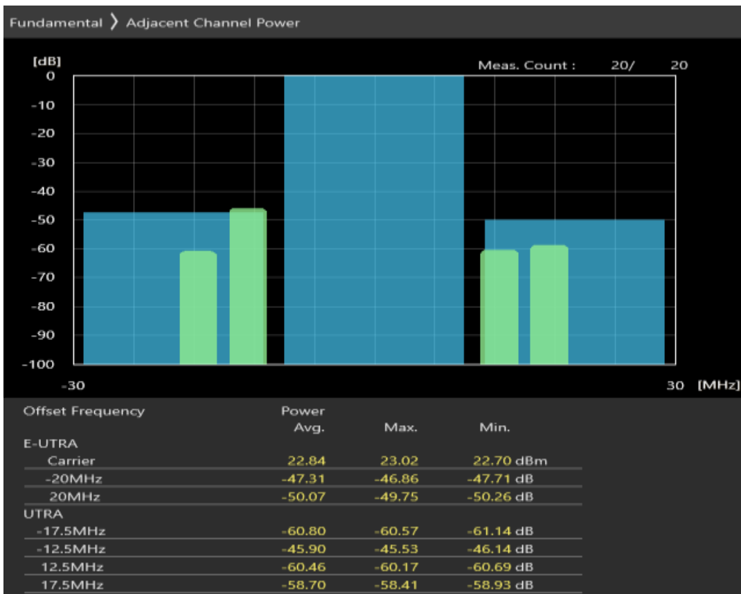
Band3 QPSK BW=20MHz Channel=19300 RB Size=18 Position=#Max
