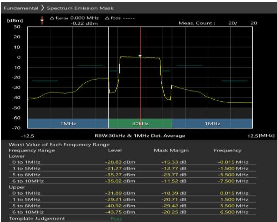
Band8 QPSK BW=5MHz Channel=21775 RB Size=8 Position=#0
