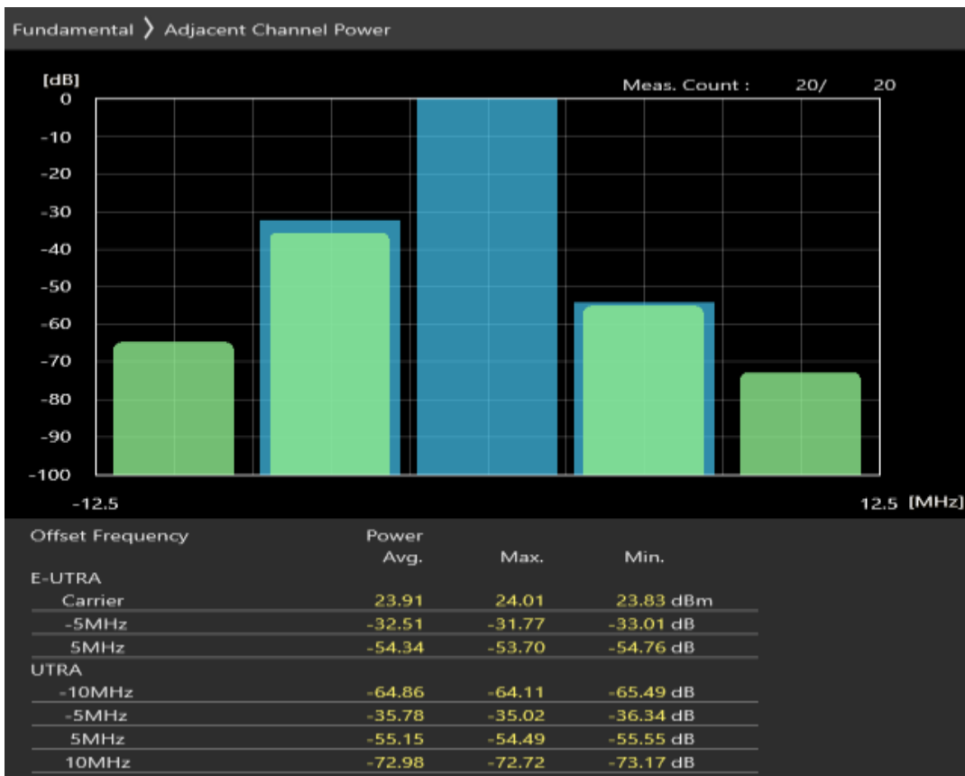
Band20 QPSK BW=5MHz Channel=24425 RB Size=8 Position=#Max
