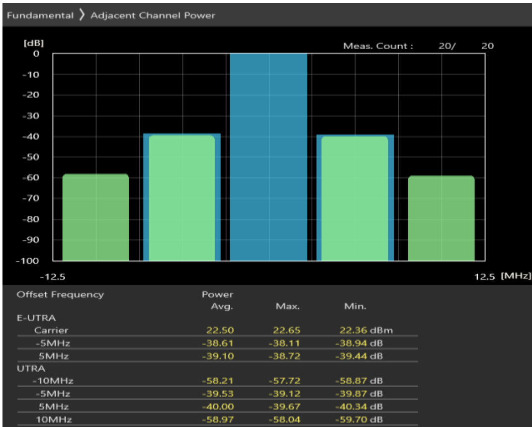
Band3 16QAM BW=5MHz Channel=19575 RB Size=8 Position=#0
