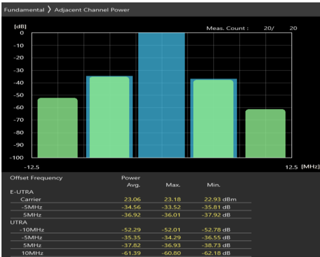
Band20 16QAM BW=5MHz Channel=24425 RB Size=8 Position=#0
