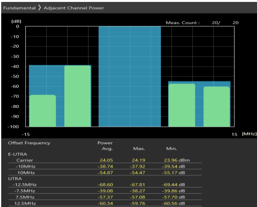
Band28 QPSK BW=10MHz Channel=27260 RB Size=12 Position=#Max
