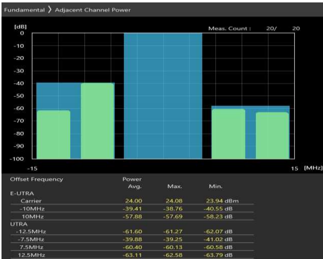
Band1 QPSK BW=10MHz Channel=18300 RB Size=12 Position=#Max
