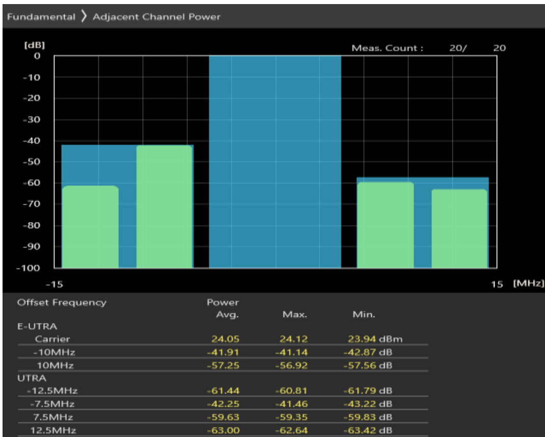
Band28 QPSK BW=10MHz Channel=27410 RB Size=12 Position=#Max
