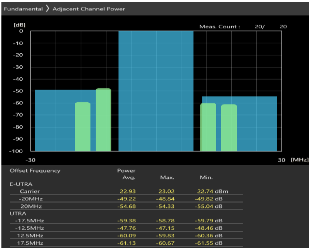
Band1 16QAM BW=20MHz Channel=18100 RB Size=18 Position=#Max
