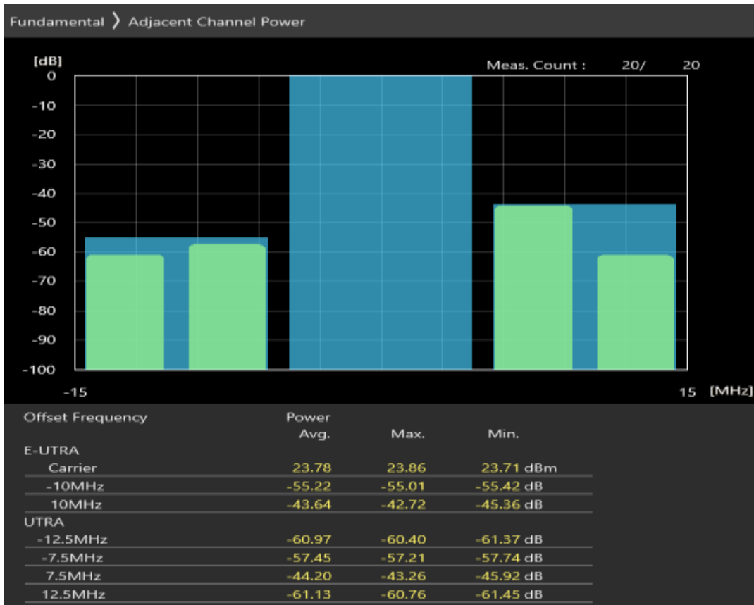
Band1 QPSK BW=10MHz Channel=18550 RB Size=50 Position=#0
