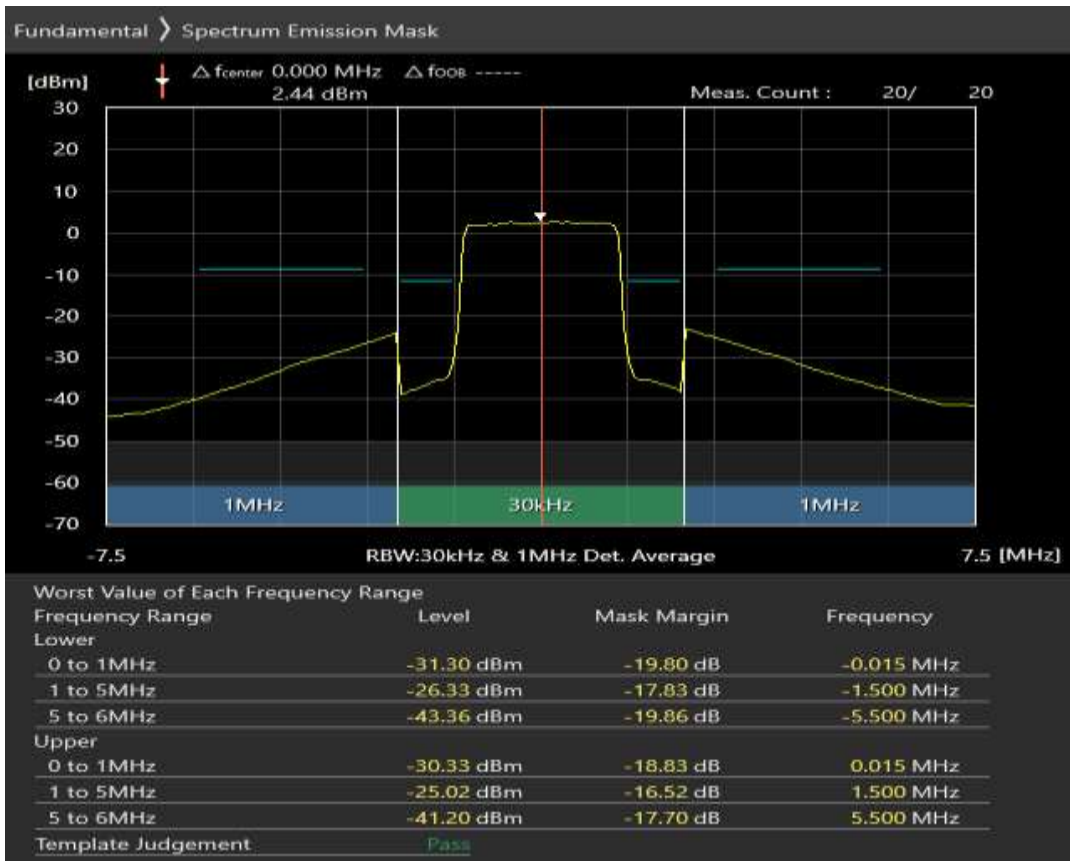
Band28 16QAM BW=3MHz Channel=27225 RB Size=4 Position=#0
