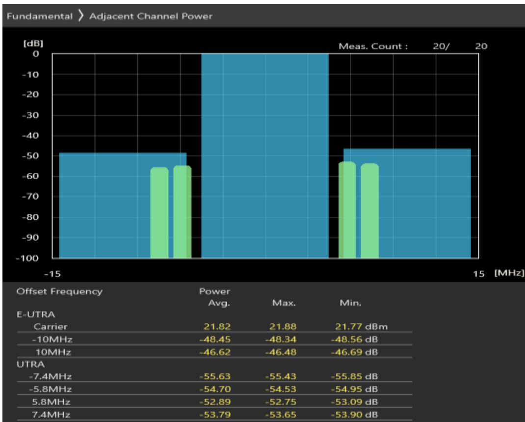
Band40 16QAM BW=10MHz Channel=39600 RB Size=12 Position=#0
