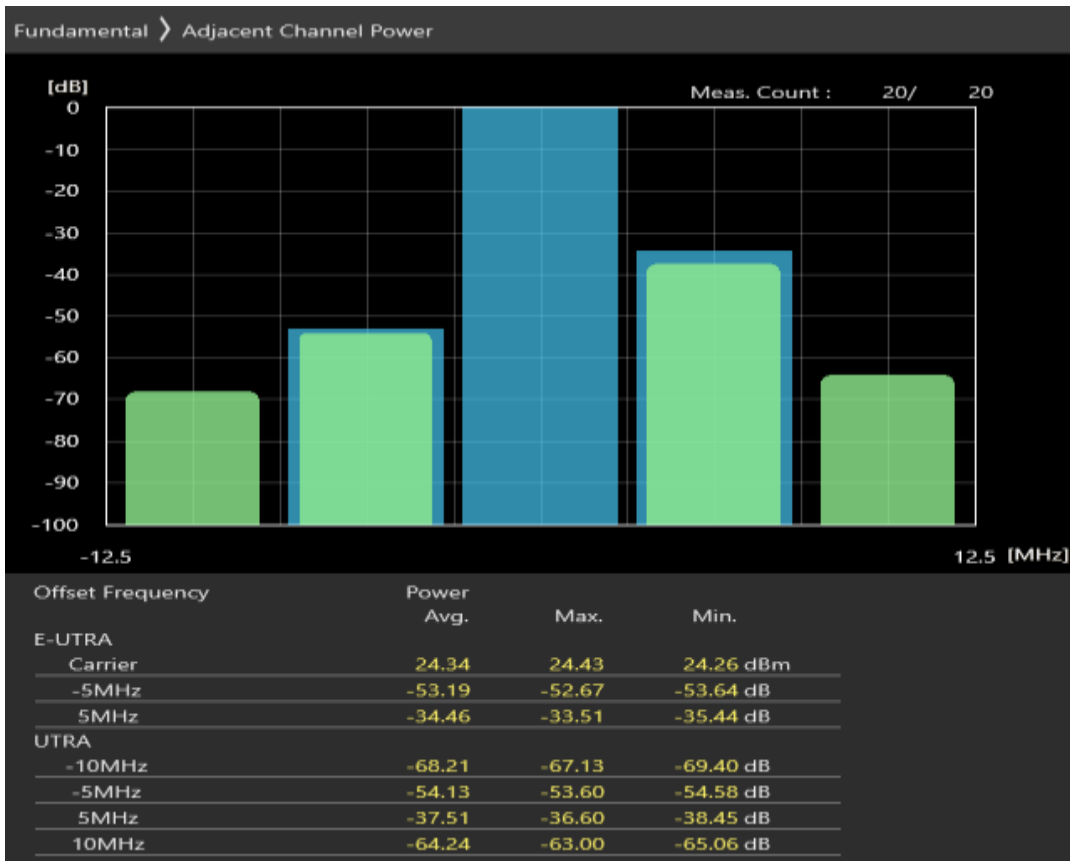
Band7 QPSK BW=5MHz Channel=21100 RB Size=25 Position=#0
