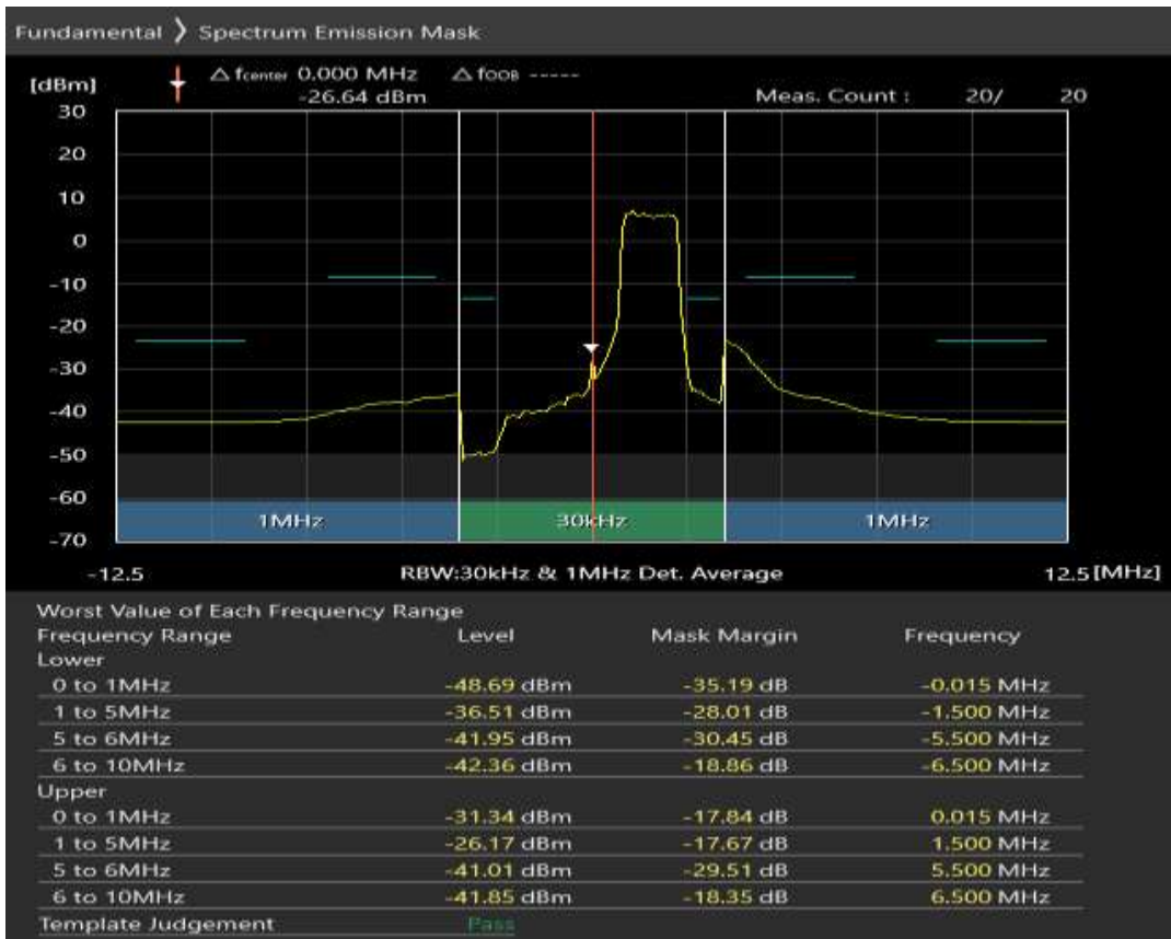
Band40 QPSK BW=5MHz Channel=38675 RB Size=25 Position=#0
