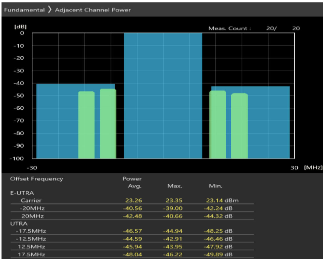
Band7 16QAM BW=20MHz Channel=21350 RB Size=18 Position=#0
