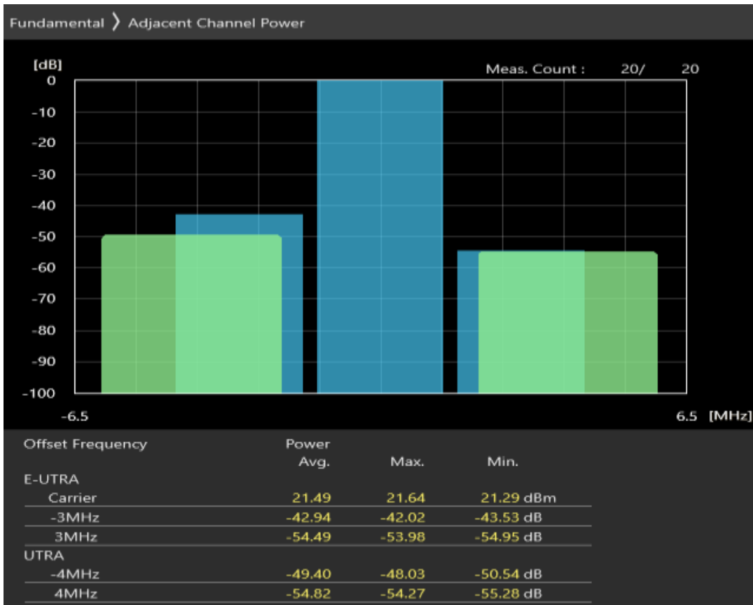
Band28 16QAM BW=3MHz Channel=27495 RB Size=4 Position=#Max
