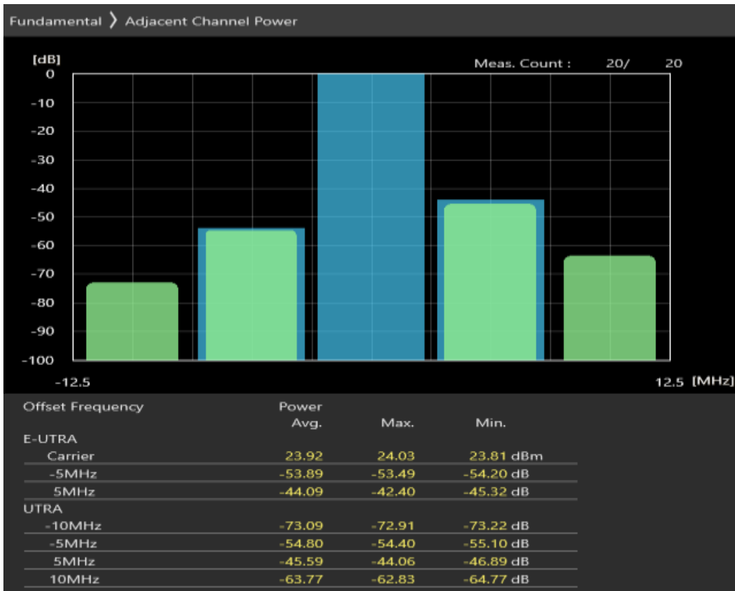
Band20 QPSK BW=5MHz Channel=24175 RB Size=25 Position=#0
