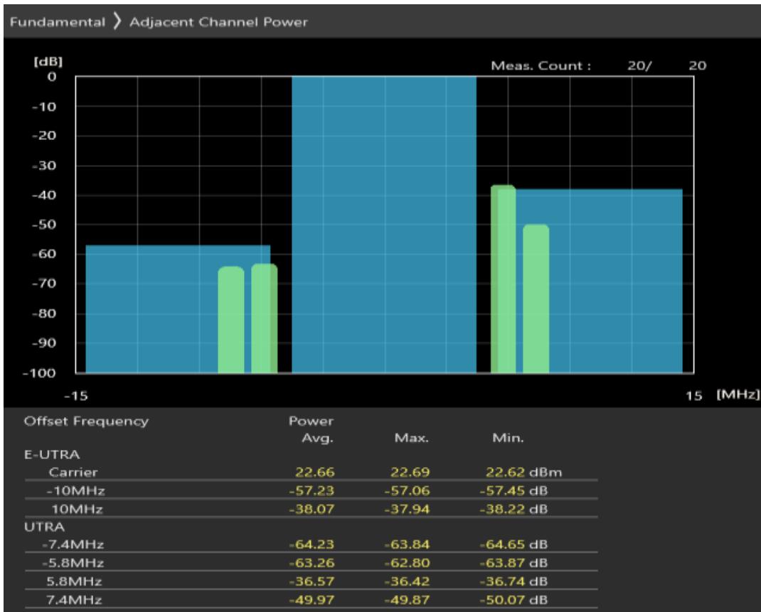
Band40 QPSK BW=10MHz Channel=39150 RB Size=50 Position=#0
