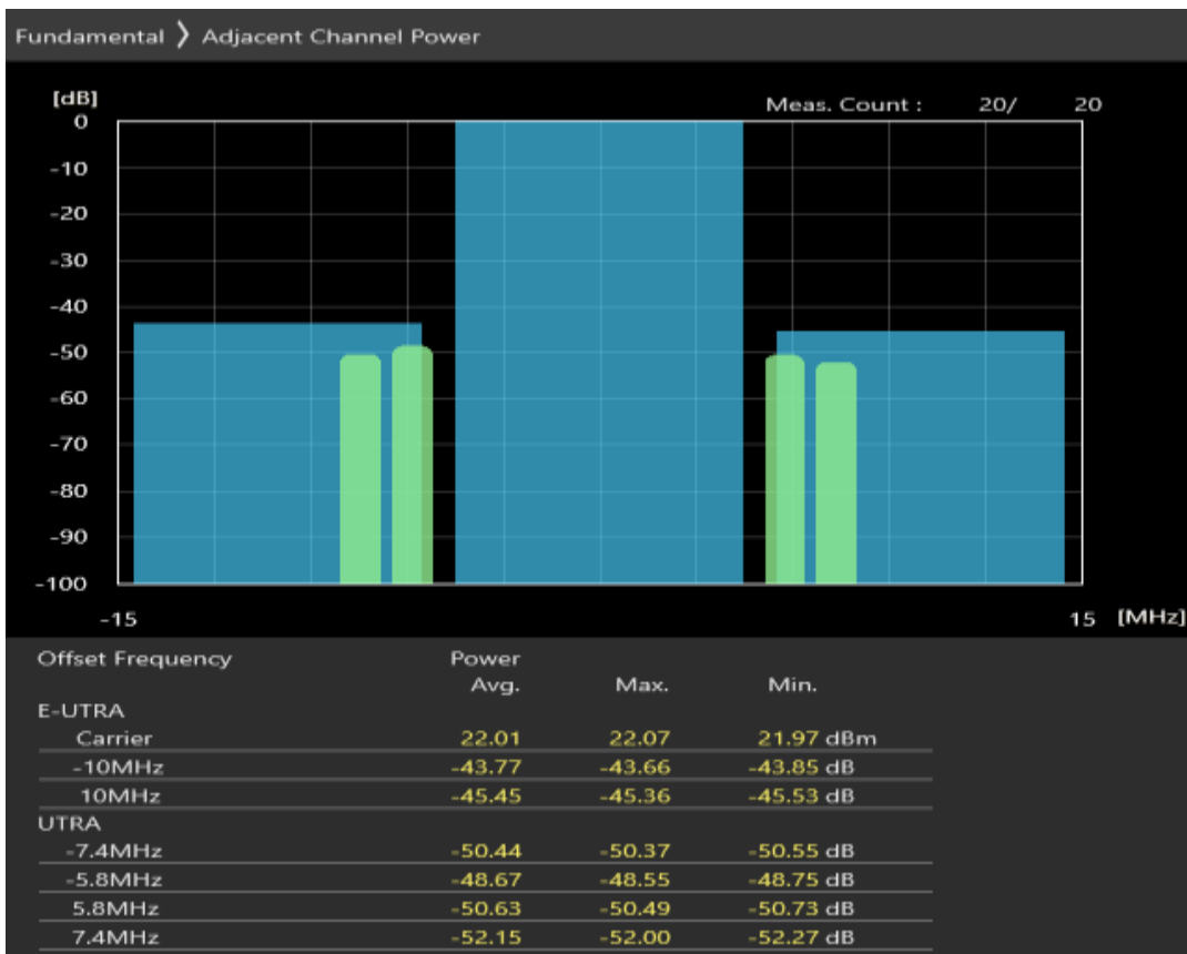
Band40 16QAM BW=10MHz Channel=38700 RB Size=12 Position=#0
