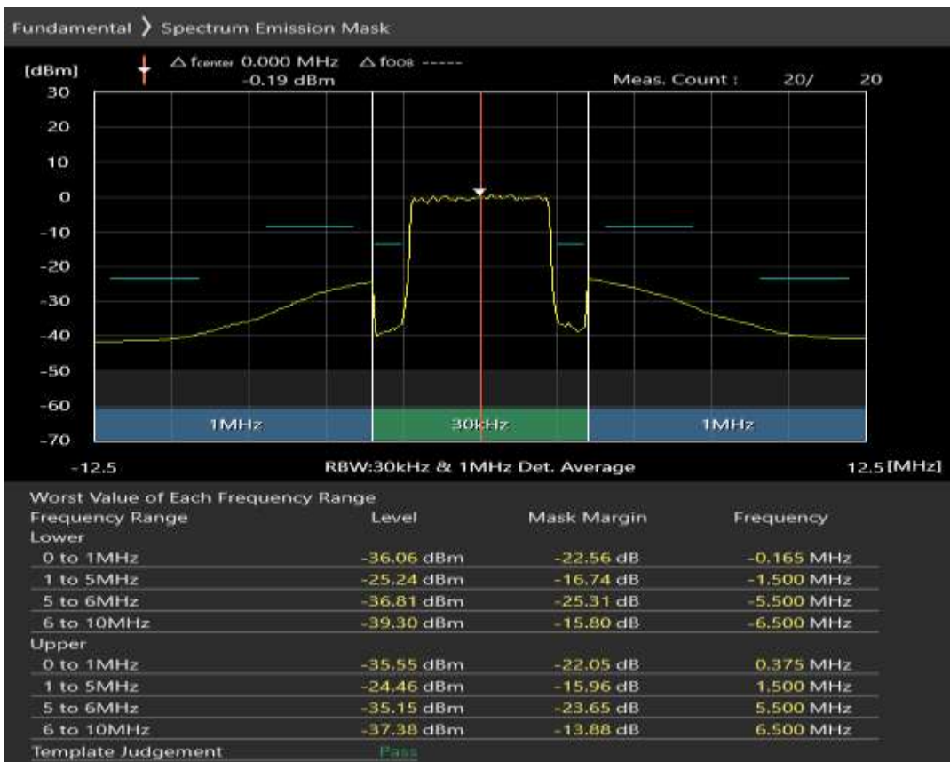
Band40 QPSK BW=5MHz Channel=39625 RB Size=8 Position=#0
