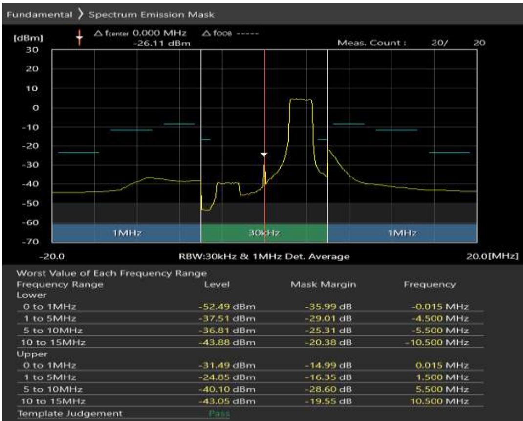
Band3 16QAM BW=10MHz Channel=19575 RB Size=50 Position=#0
