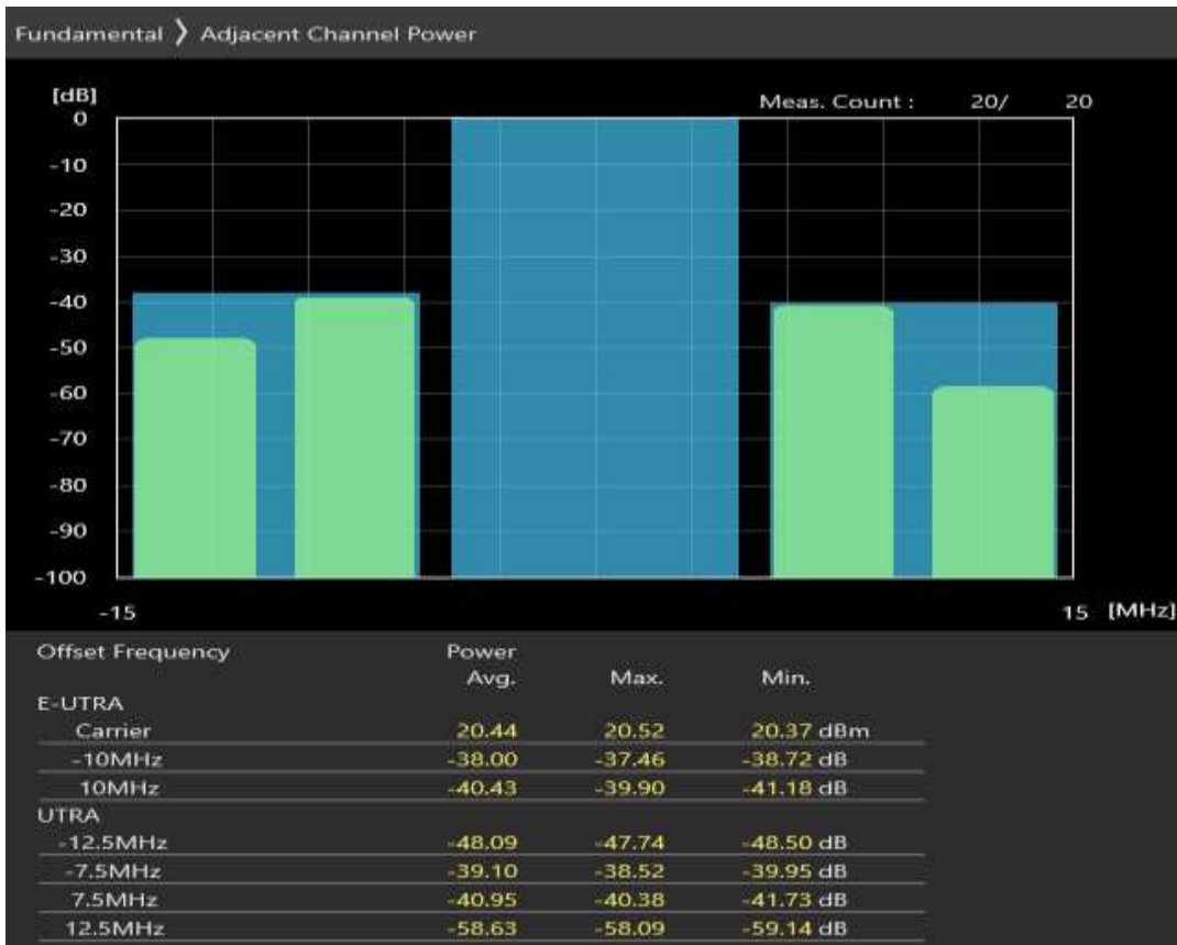
Band8 QAM16 BW=5MHz Channel=21475 RB Size=25 Position=#0
