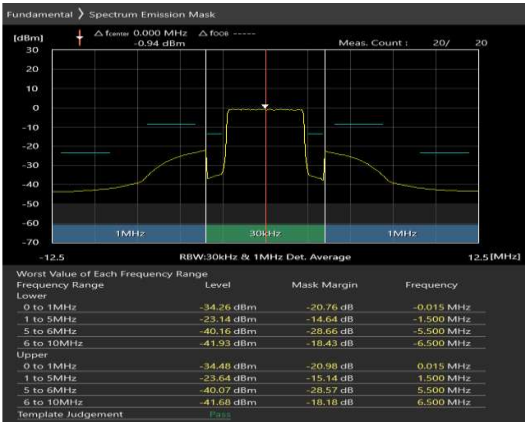
Band3 16QAM BW=5MHz Channel=19225 RB Size=8 Position=#0
