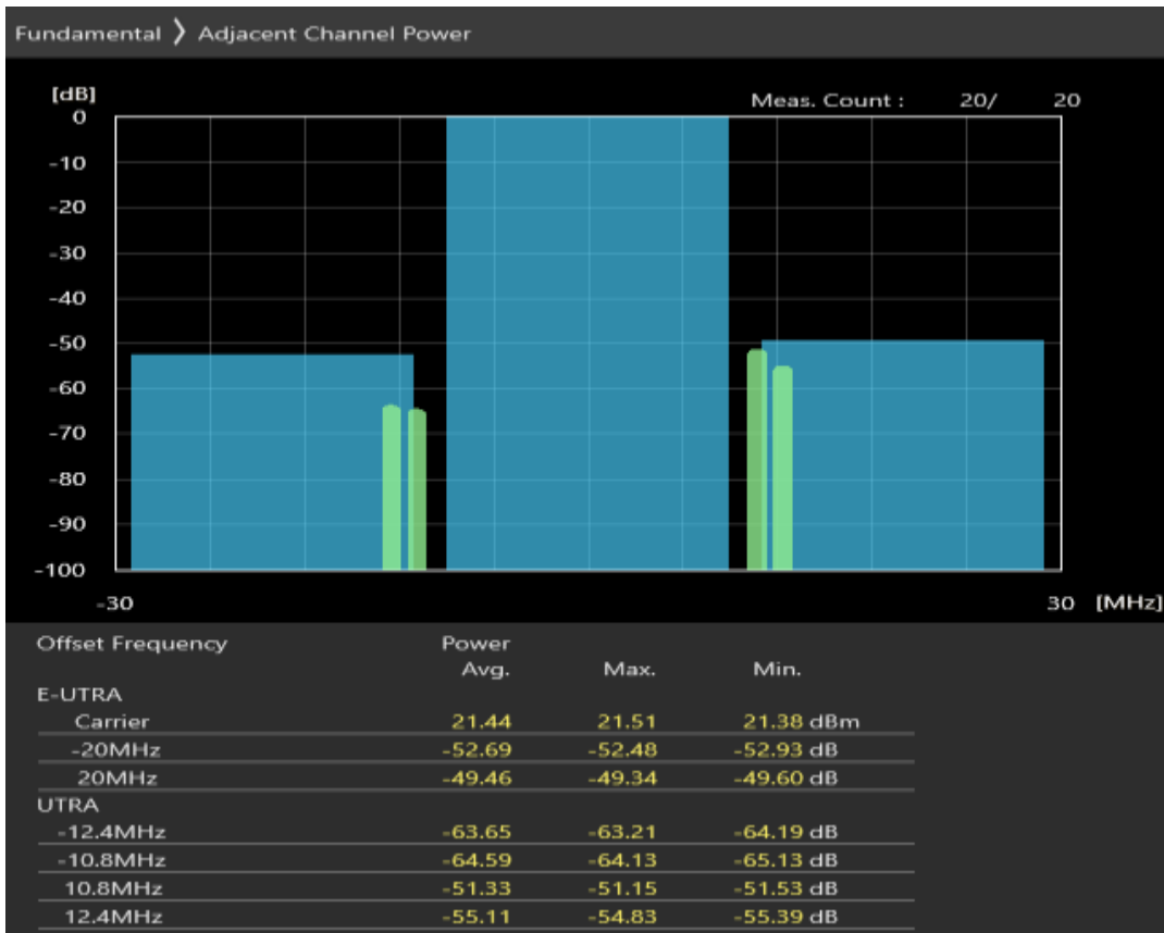
Band40 16QAM BW=20MHz Channel=39550 RB Size=100 Position=#0
