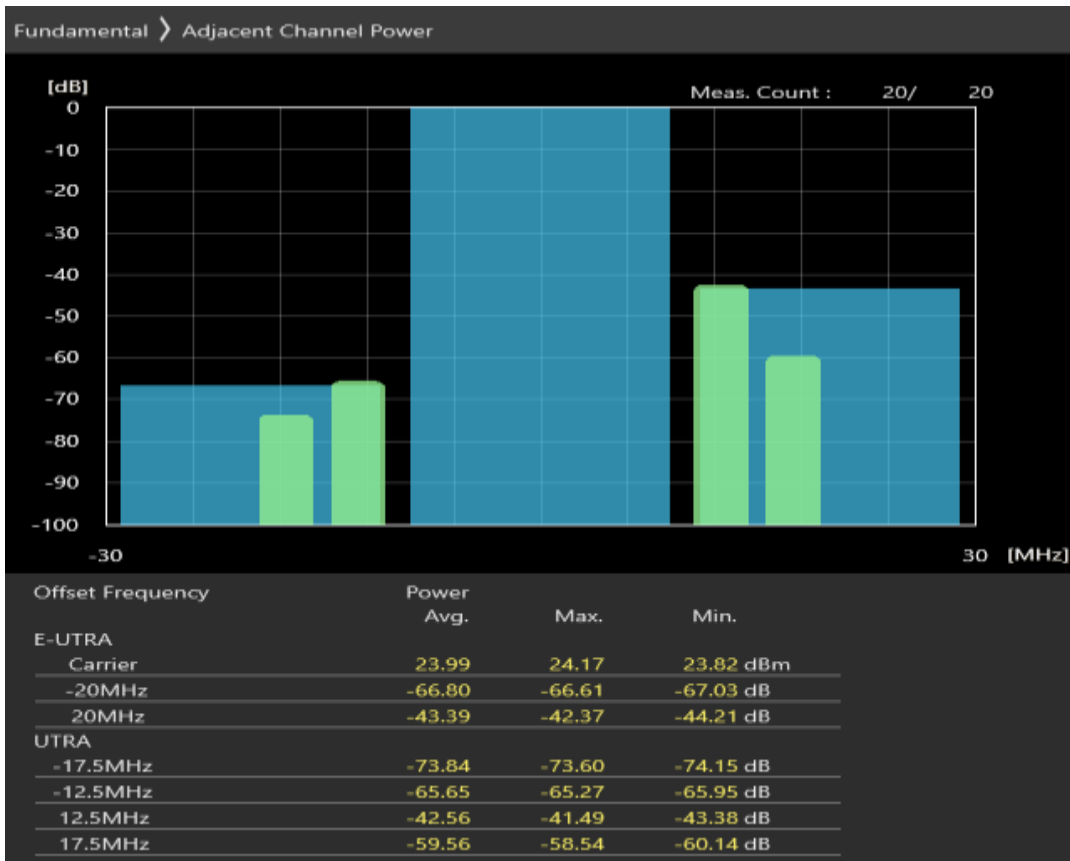
Band28 QPSK BW=20MHz Channel=27310 RB Size=100 Position=#0
