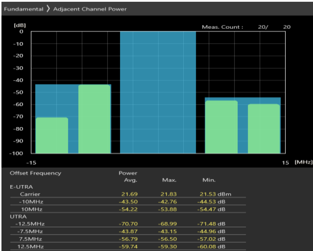
Band28 16QAM BW=10MHz Channel=27260 RB Size=12 Position=#Max
