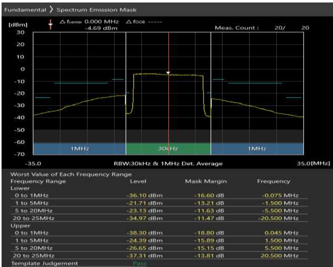
Band7 QPSK BW=20MHz Channel=21350 RB Size=18 Position=#0
