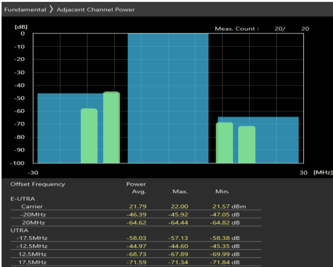
Band28 16QAM BW=20MHz Channel=27560 RB Size=18 Position=#Max
