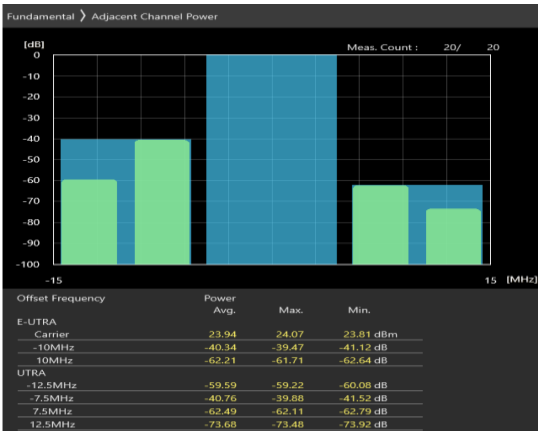
Band28 QPSK BW=10MHz Channel=27610 RB Size=12 Position=#Max
