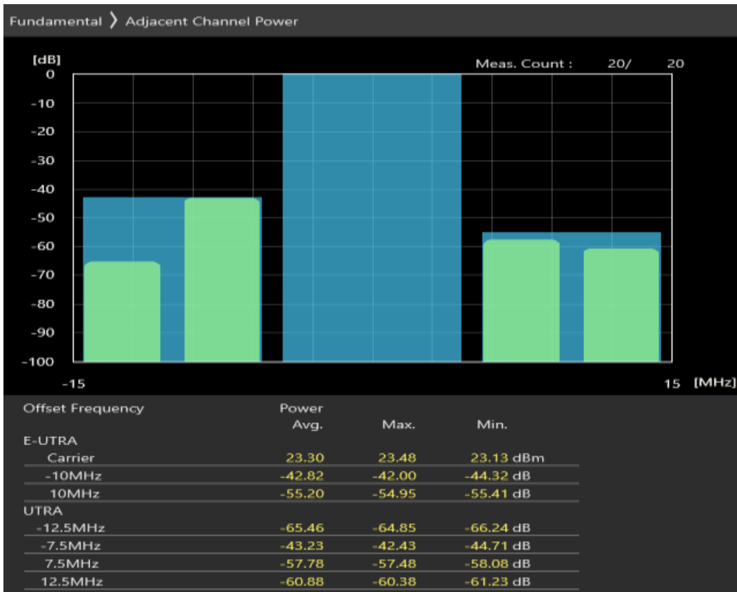
Band20 16QAM BW=10MHz Channel=24200 RB Size=12 Position=#Max
