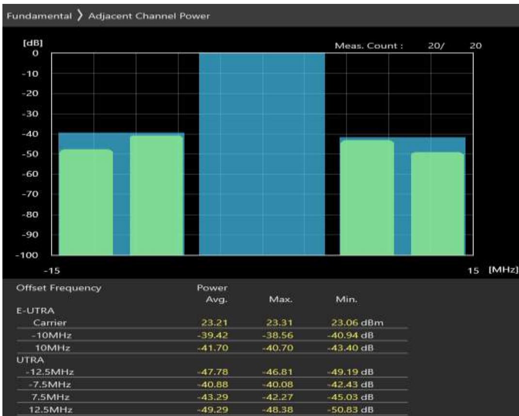
Band1 16QAM BW=10MHz Channel=18300 RB Size=12 Position=#0
