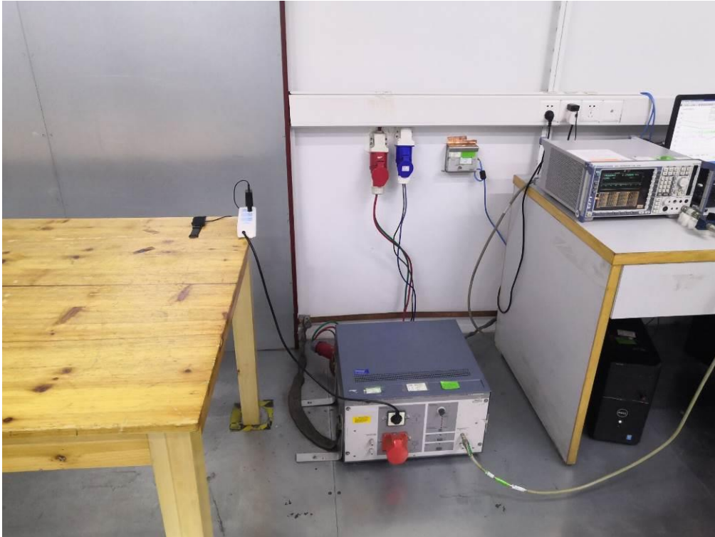
RADIATED EMISSION TEST SETUP BELOW 1GHZ
