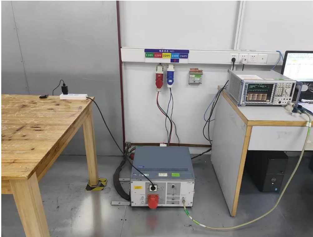
RADIATED EMISSION TEST SETUP BELOW 1GHZ
