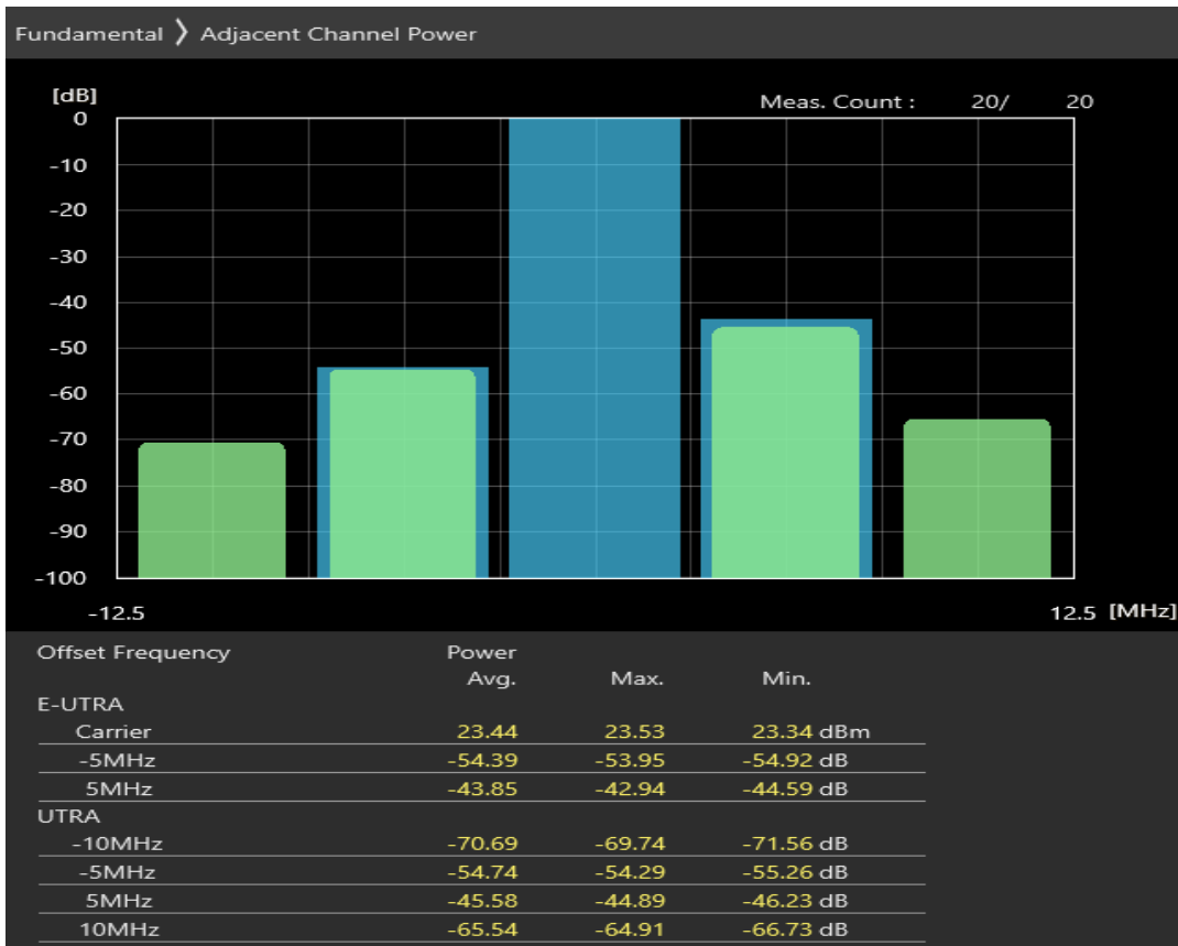
Band3 QPSK BW=5MHz Channel=19225 RB Size=25 Position=#0
