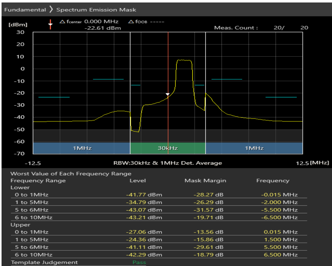
Band3 16QAM BW=5MHz Channel=19575 RB Size=25 Position=#0
