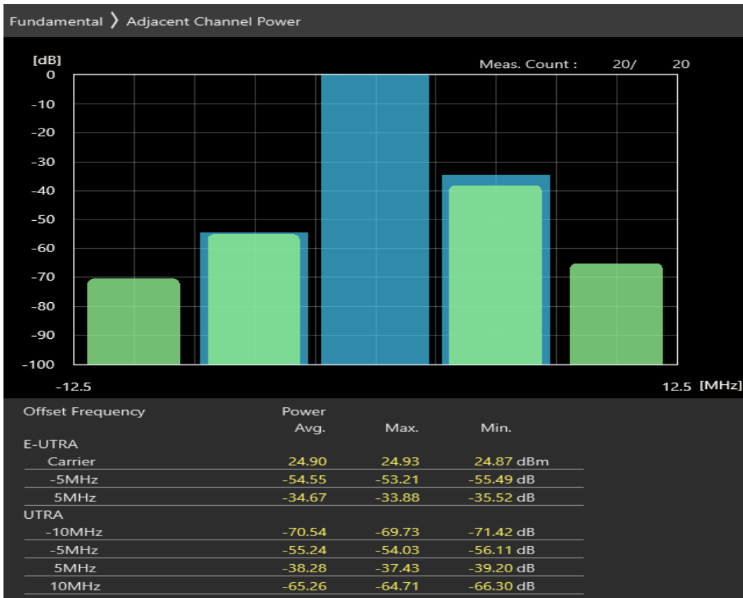
Band1 QPSK BW=5MHz Channel=18300 RB Size=25 Position=#0
