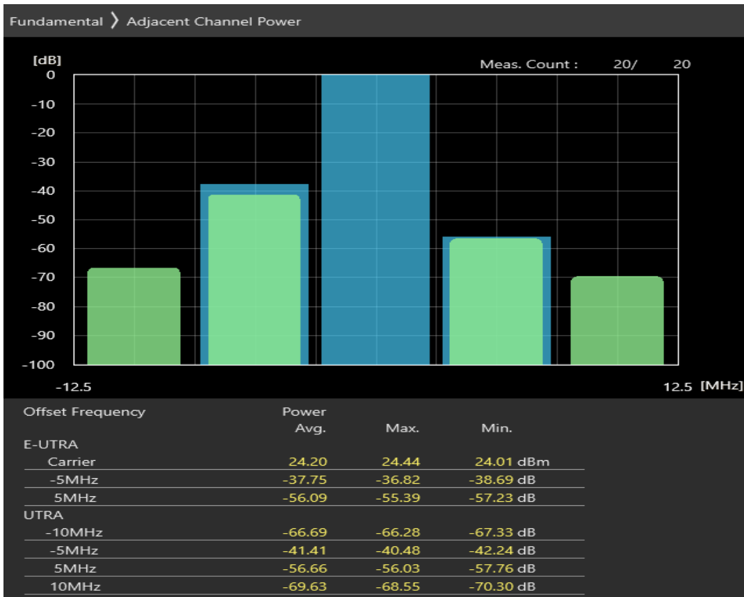
Band1 16QAM BW=5MHz Channel=18025 RB Size=8 Position=#Max
