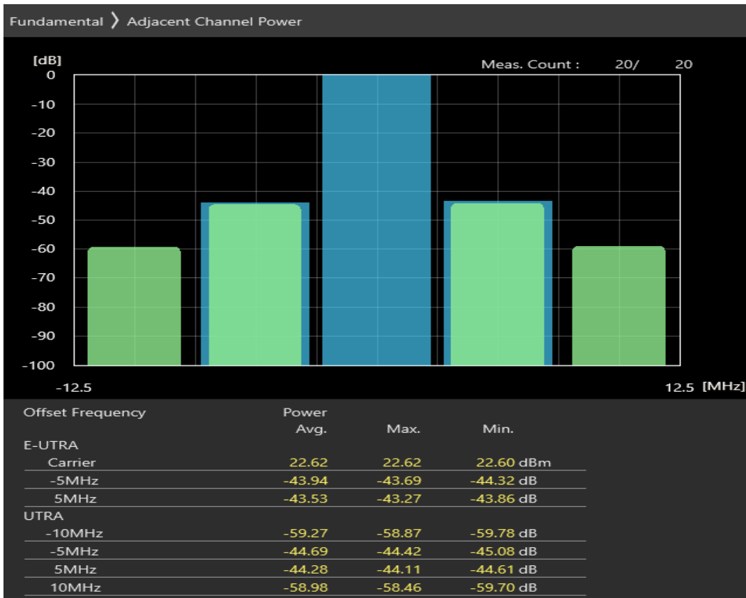
Band3 16QAM BW=5MHz Channel=19575 RB Size=8 Position=#0
