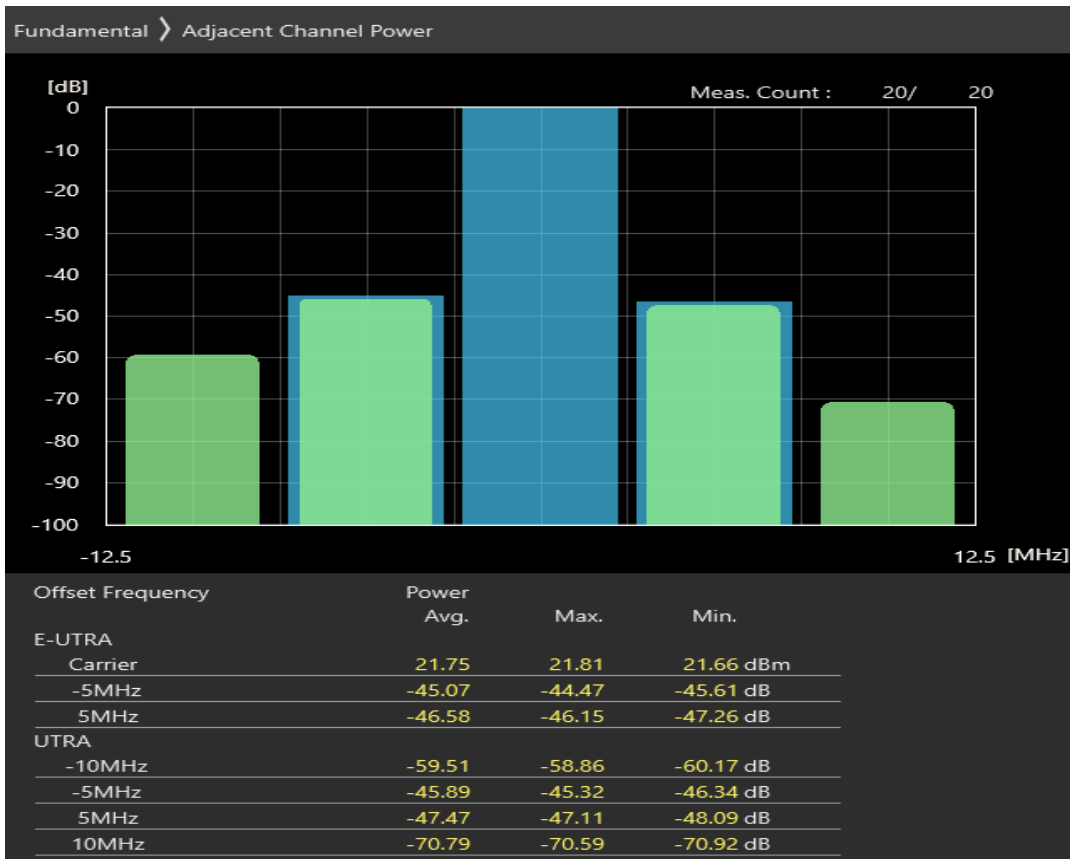
Band8 QPSK BW=10MHz Channel=21500 RB Size=12 Position=#0
