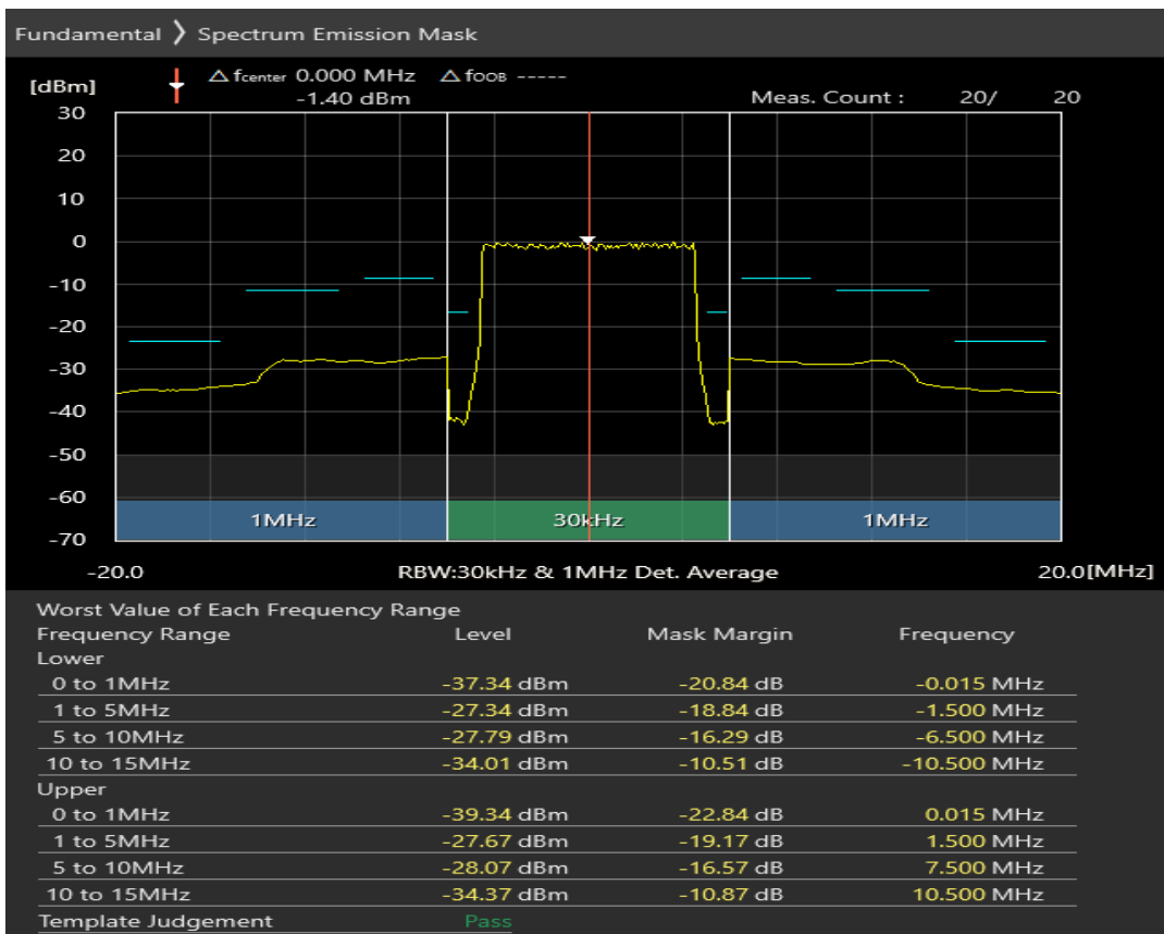
Band40 16QAM BW=10MHz Channel=39150 RB Size=12 Position=#0
