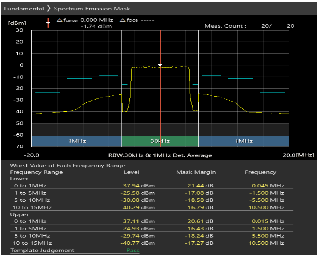
Band1 QPSK BW=10MHz Channel=18300 RB Size=12 Position=#0
