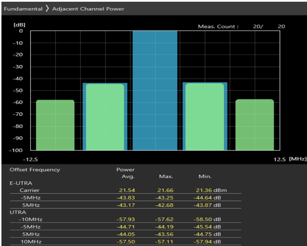
Band8 QPSK BW=5MHz Channel=21775 RB Size=8 Position=#0
