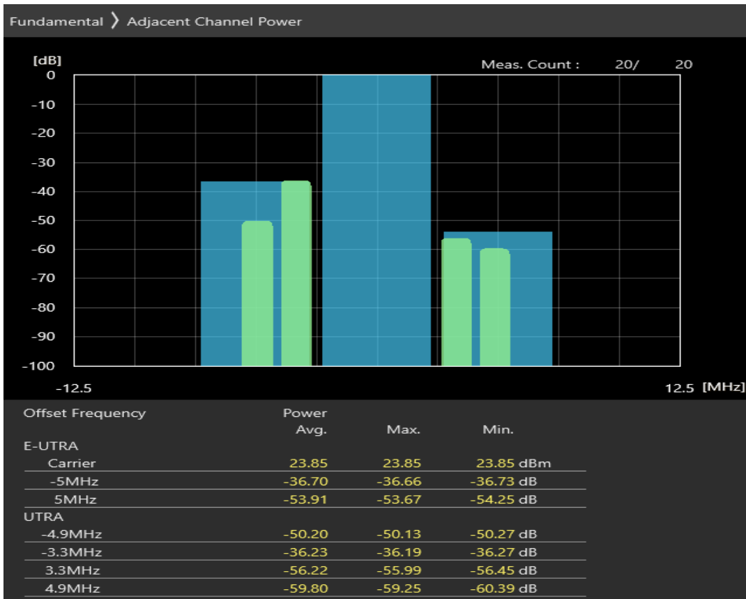
Band40 16QAM BW=5MHz Channel=38675 RB Size=8 Position=#Max
