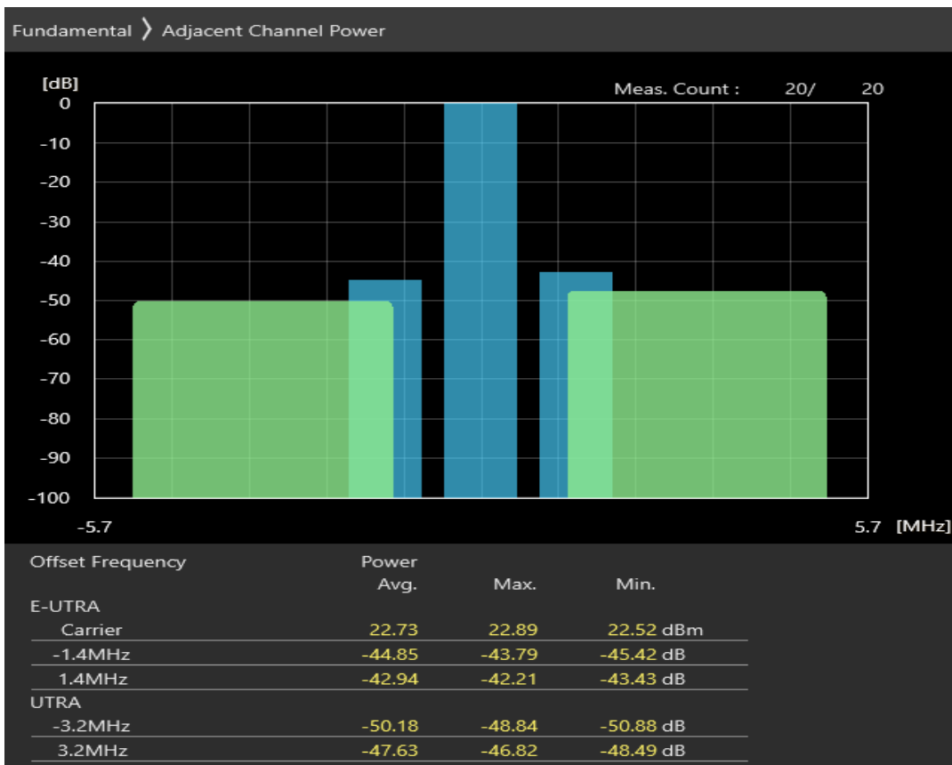
Band3 16QAM BW=1.4MHz Channel=19207 RB Size=6 Position=#0
