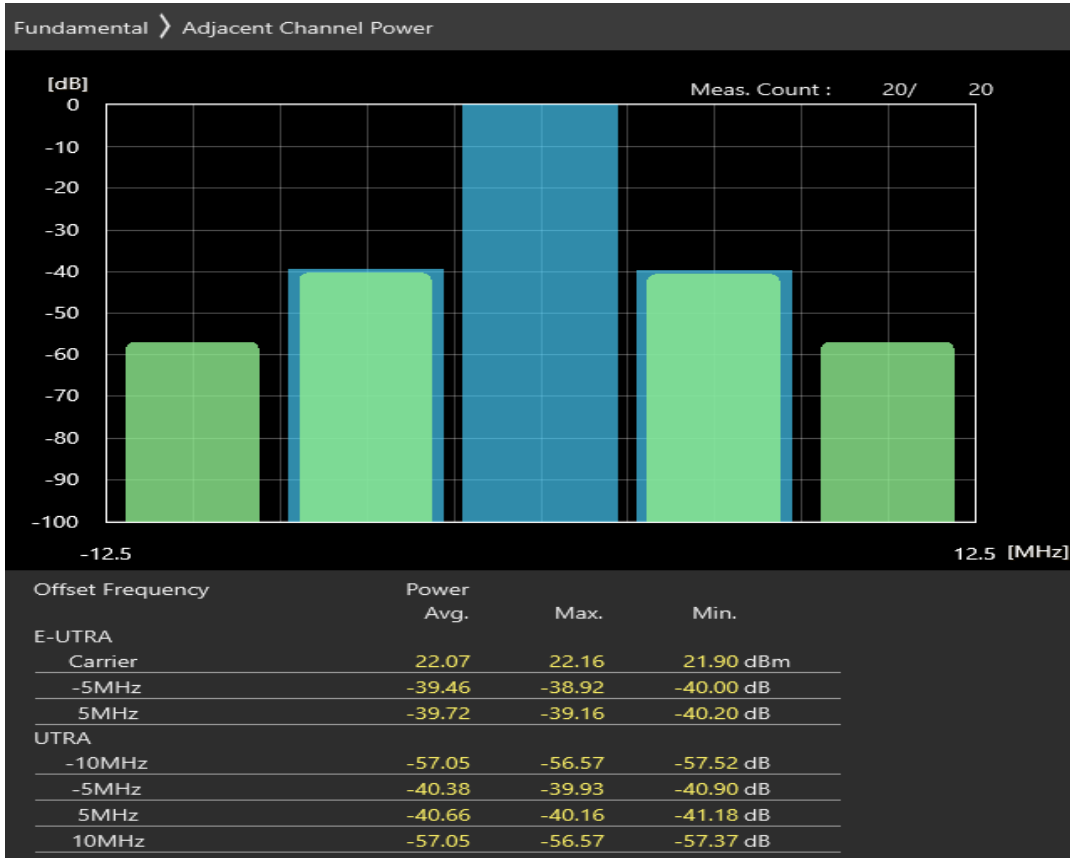
Band7 QPSK BW=5MHz Channel=21100 RB Size=8 Position=#0
