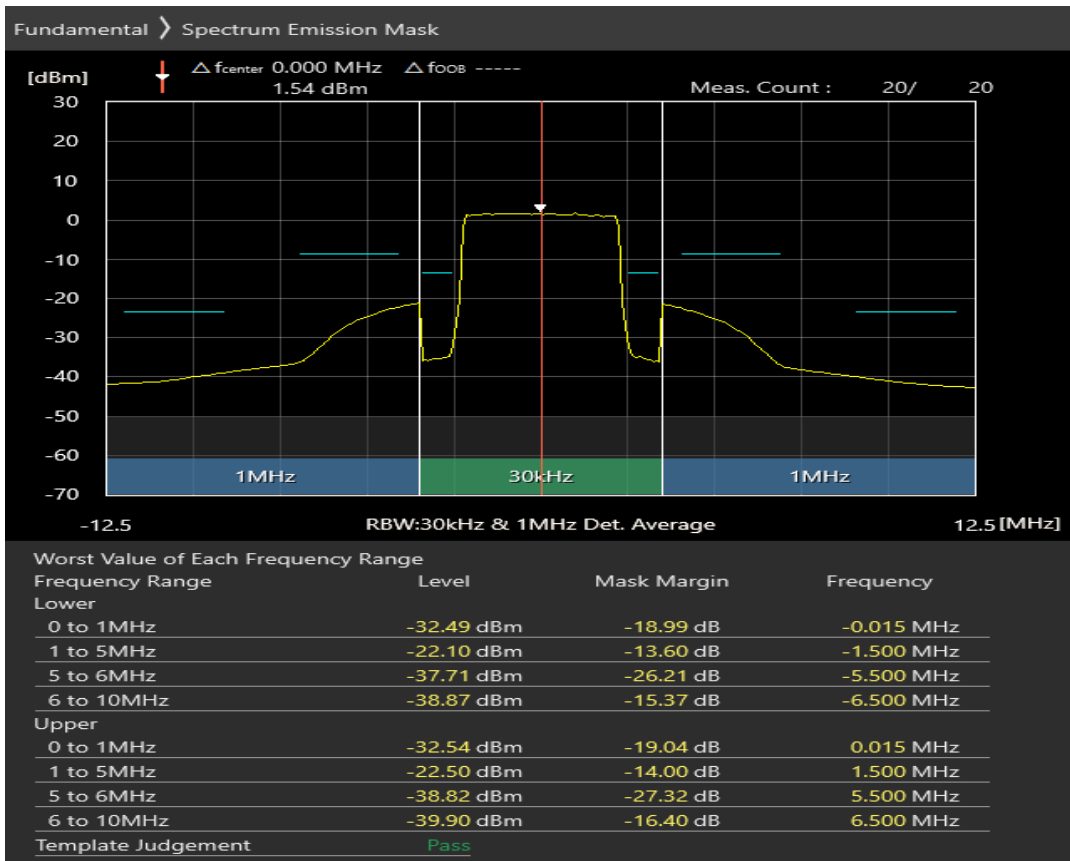
Band1 QPSK BW=10MHz Channel=18050 RB Size=12 Position=#0
