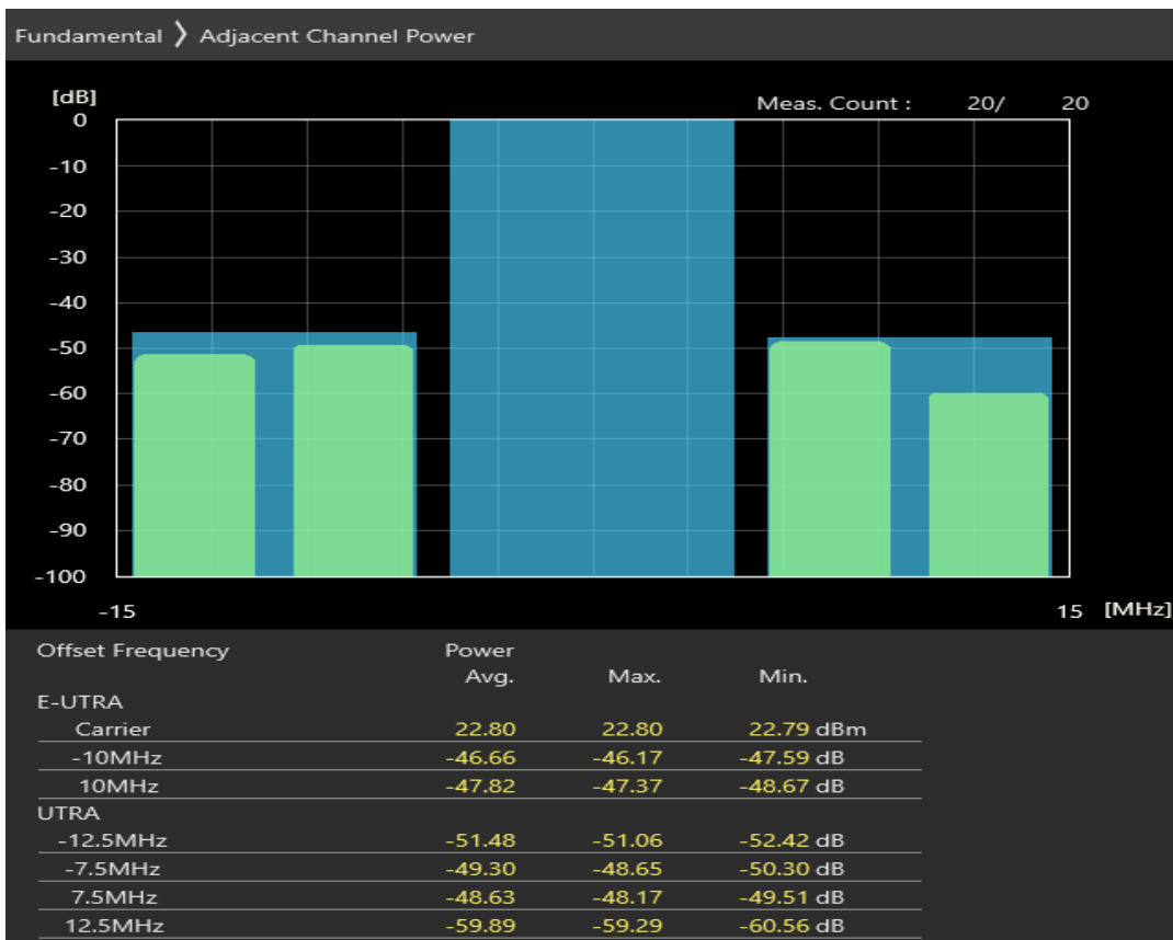
Band3 16QAM BW=10MHz Channel=19900 RB Size=12 Position=#0
