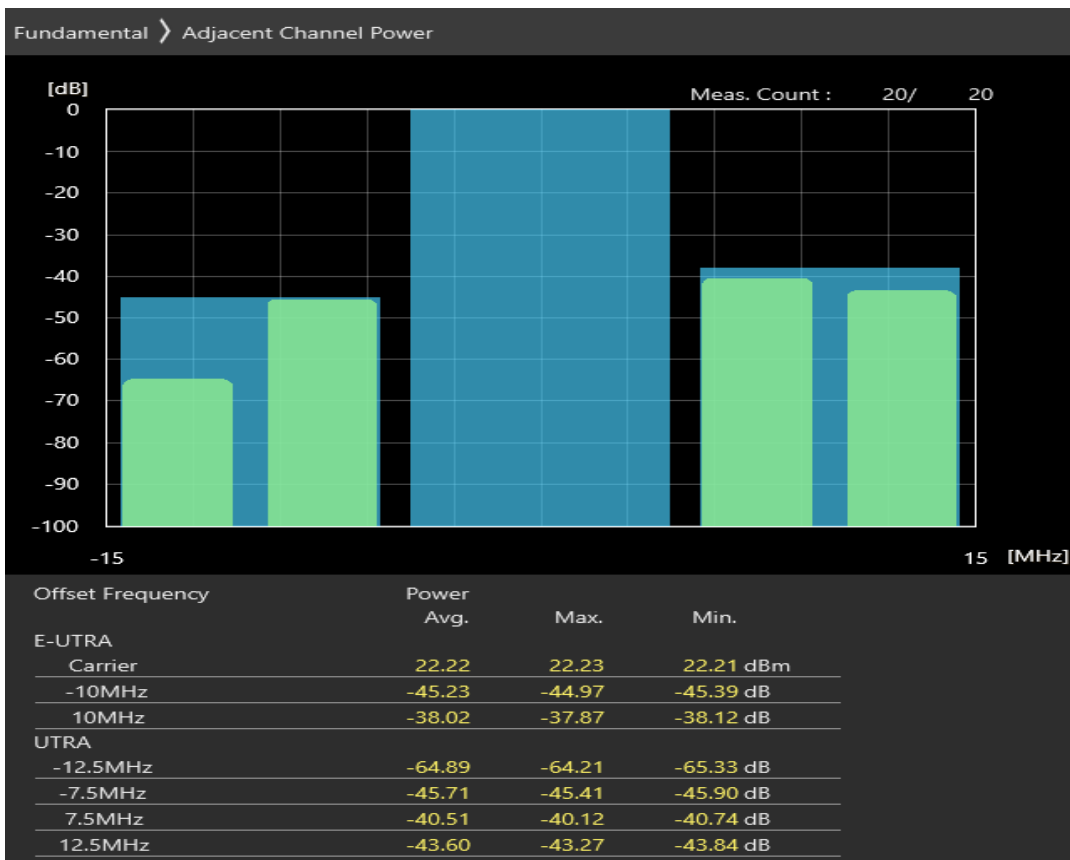
Band20 16QAM BW=10MHz Channel=24200 RB Size=12 Position=#0
