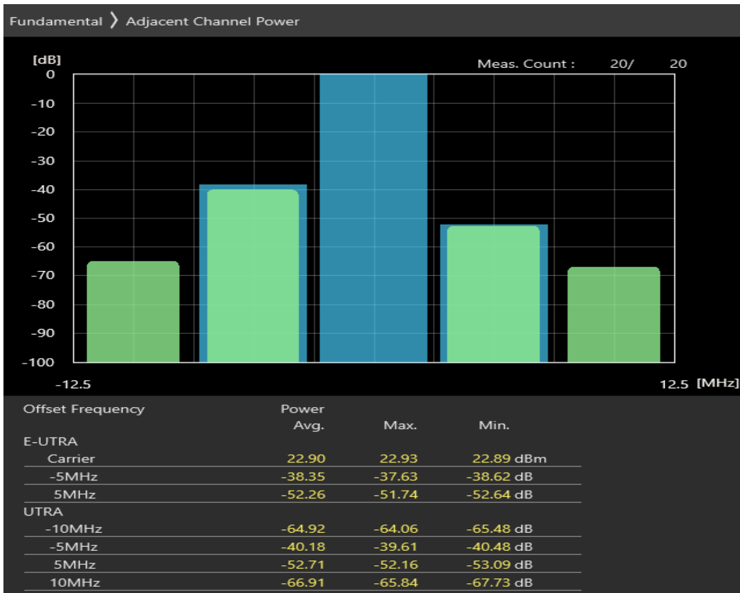
Band7 QPSK BW=5MHz Channel=21425 RB Size=8 Position=#Max
