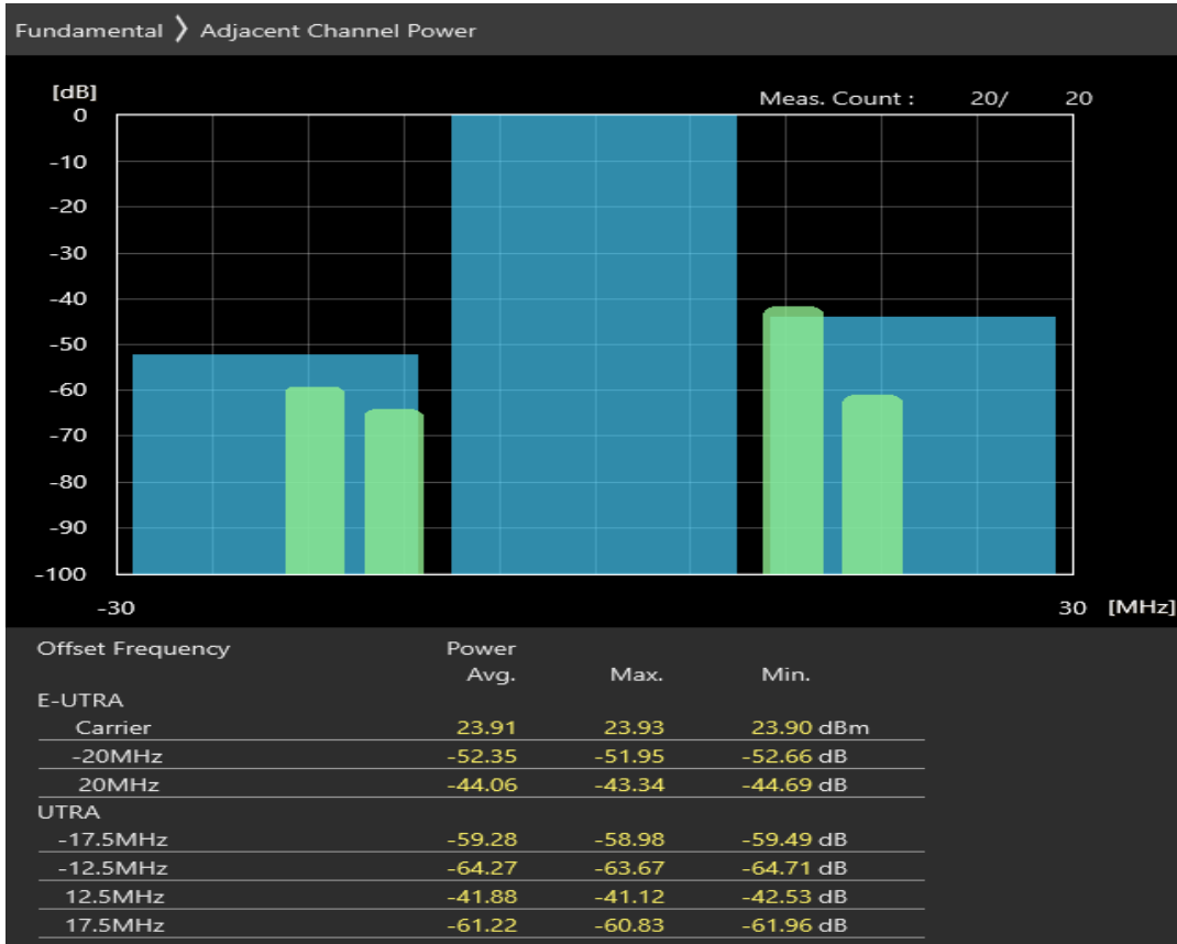
Band7 QPSK BW=20MHz Channel=21100 RB Size=100 Position=#0
