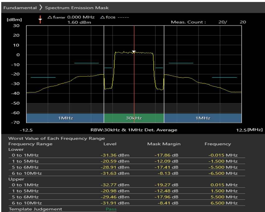
Band40 16QAM BW=5MHz Channel=38675 RB Size=8 Position=#0
