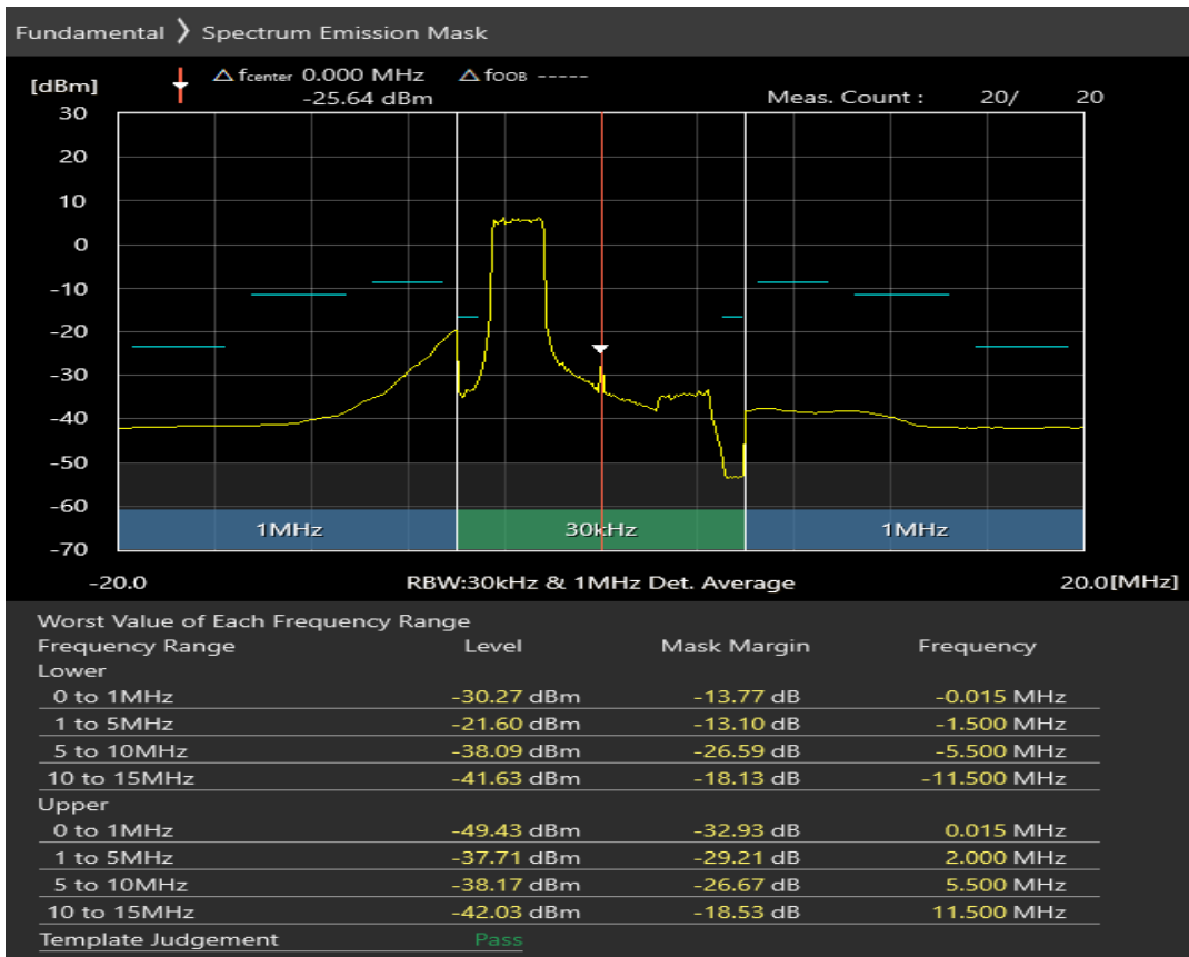
Band40 16QAM BW=10MHz Channel=39150 RB Size=12 Position=#Max
