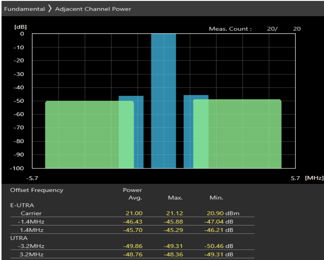
Band8 QPSK BW=1.4MHz Channel=21625 RB Size=5 Position=#0
