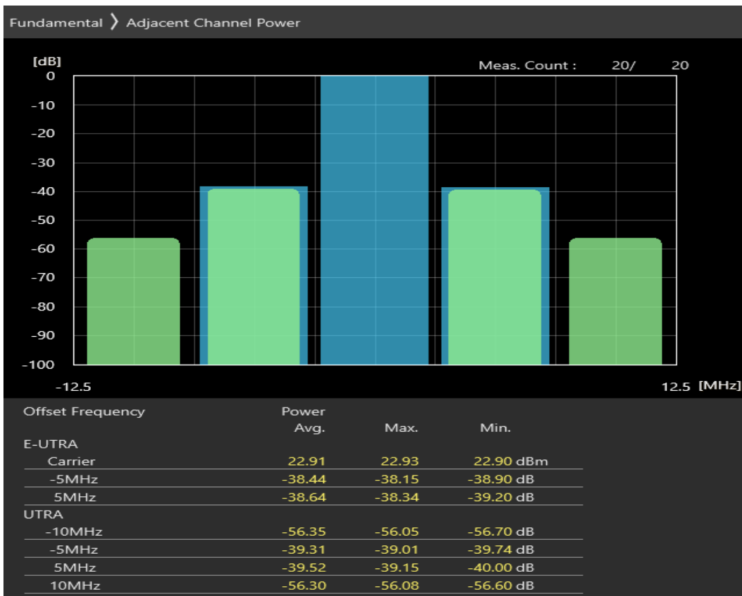
Band7 16QAM BW=5MHz Channel=20775 RB Size=8 Position=#0
