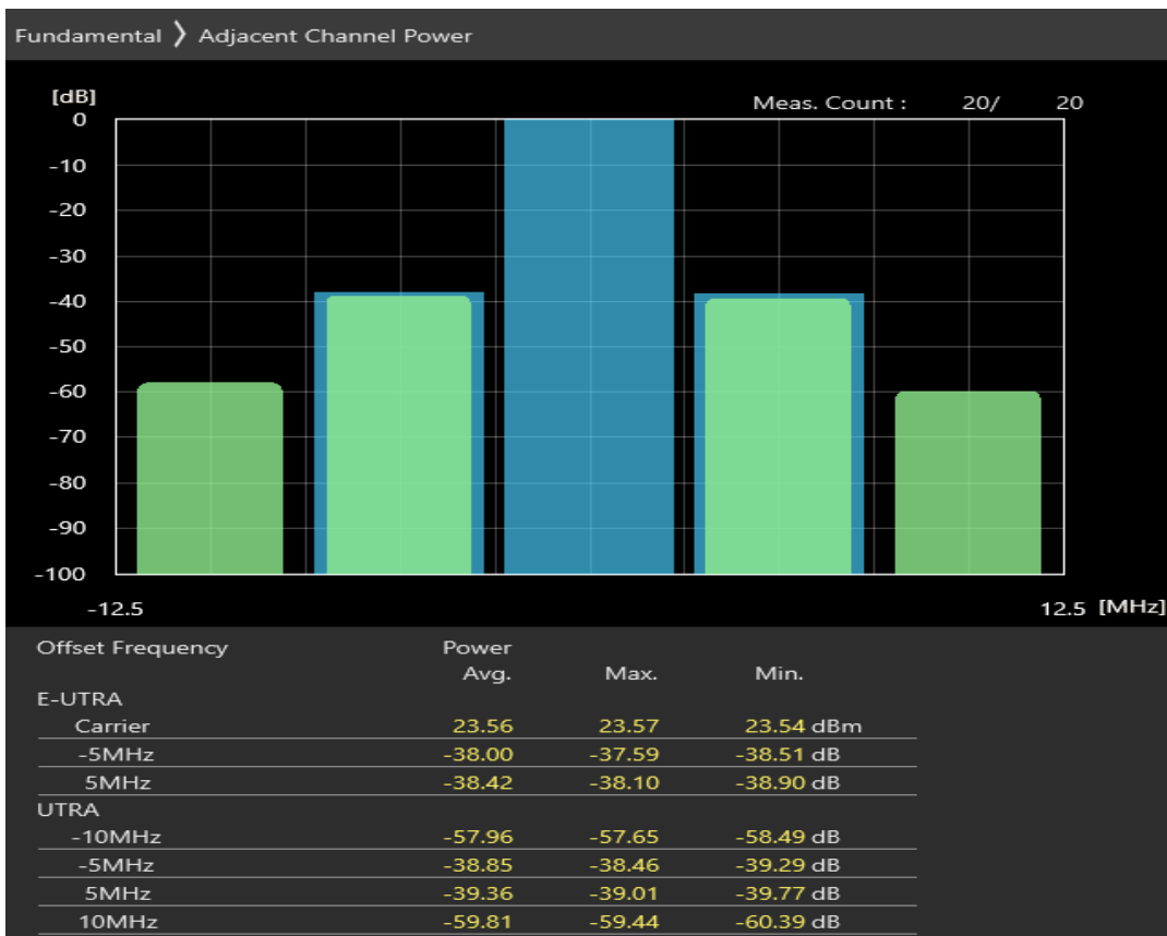
Band1 16QAM BW=5MHz Channel=18575 RB Size=8 Position=#0
