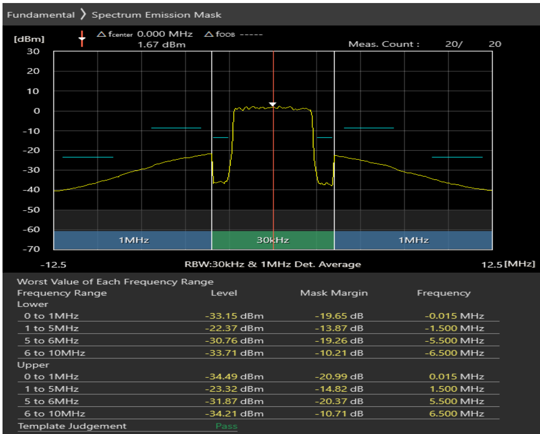
Band40 QPSK BW=5MHz Channel=39150 RB Size=8 Position=#0
