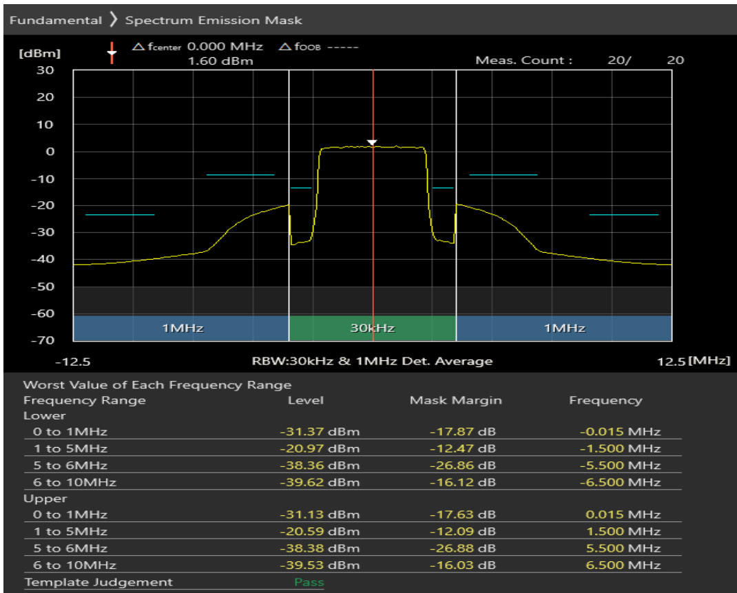
Band1 QPSK BW=5MHz Channel=18575 RB Size=8 Position=#0
