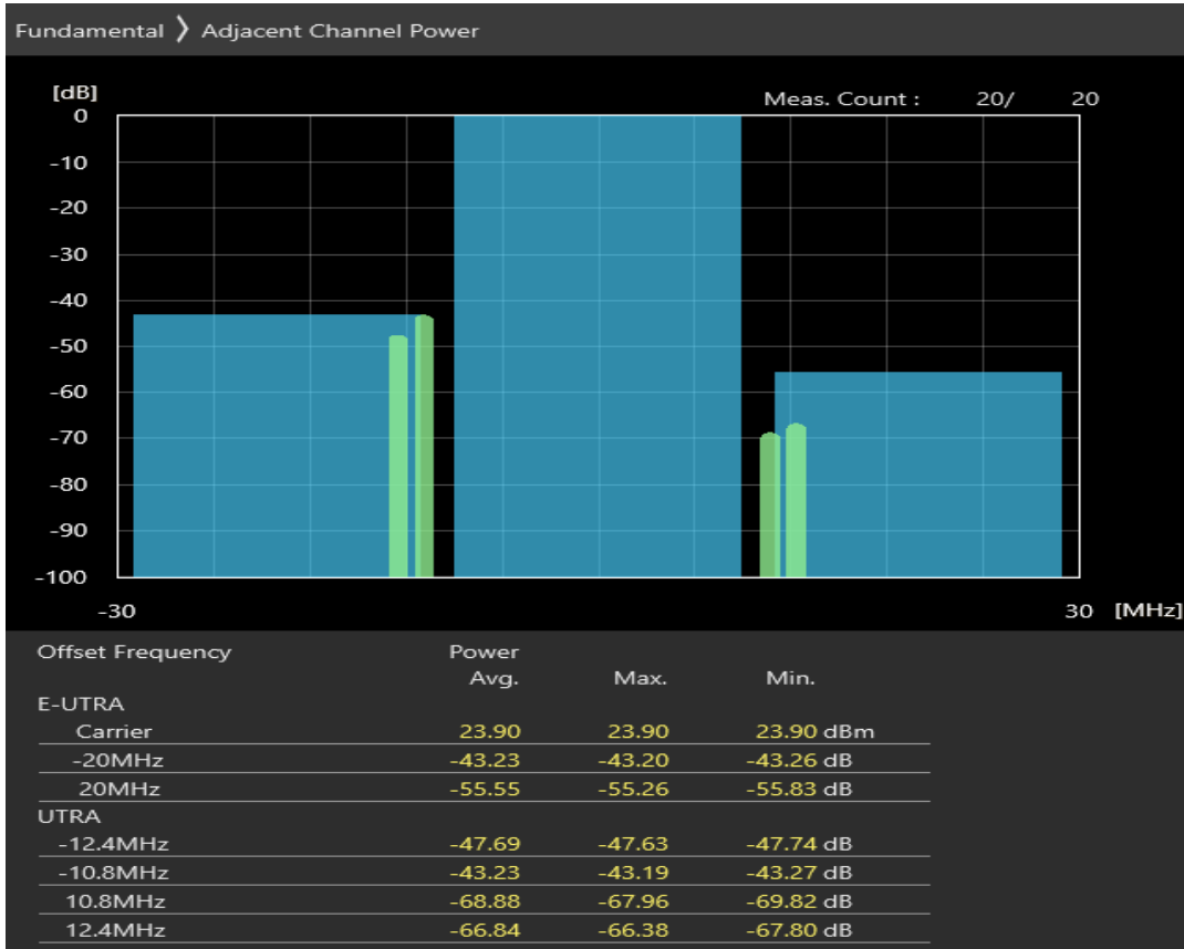
Band40 16QAM BW=20MHz Channel=39150 RB Size=18 Position=#Max
