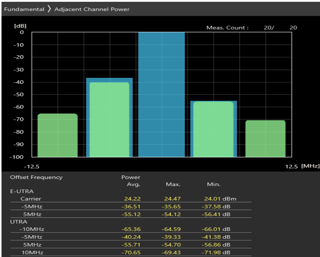
Band1 16QAM BW=5MHz Channel=18575 RB Size=8 Position=#Max
