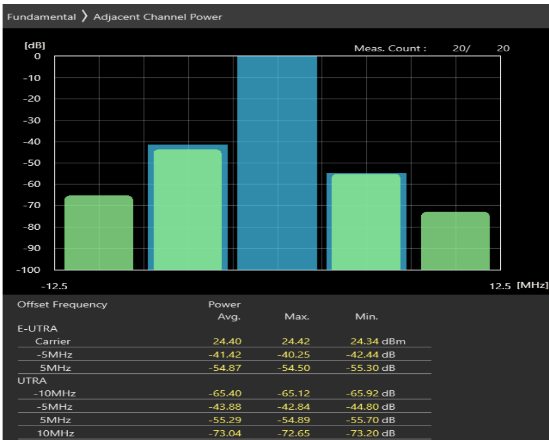
Band3 QPSK BW=5MHz Channel=19925 RB Size=8 Position=#Max
