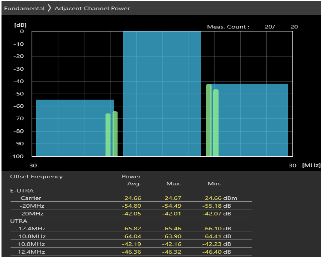
Band40 QPSK BW=20MHz Channel=38750 RB Size=100 Position=#0
