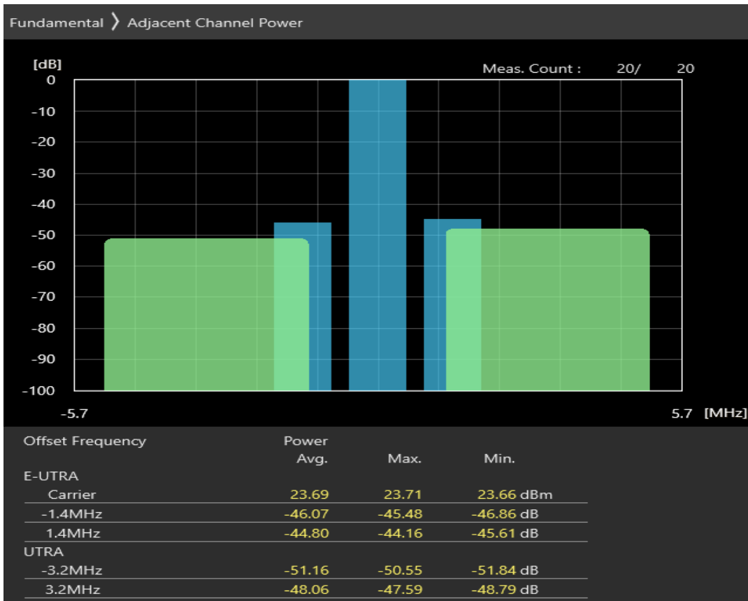
Band8 QPSK BW=1.4MHz Channel=21457 RB Size=6 Position=#0
