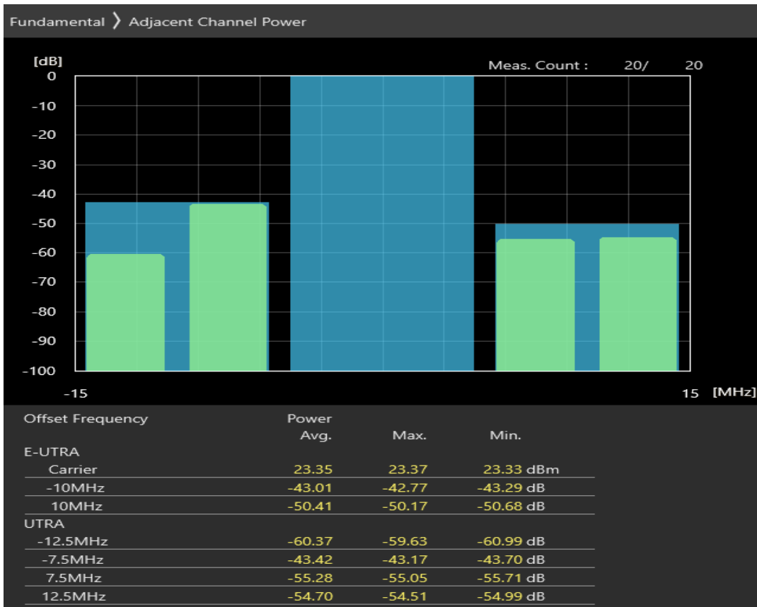
Band20 QPSK BW=10MHz Channel=24300 RB Size=12 Position=#Max
