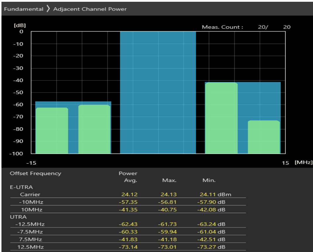
Band8 QPSK BW=10MHz Channel=21750 RB Size=50 Position=#0
