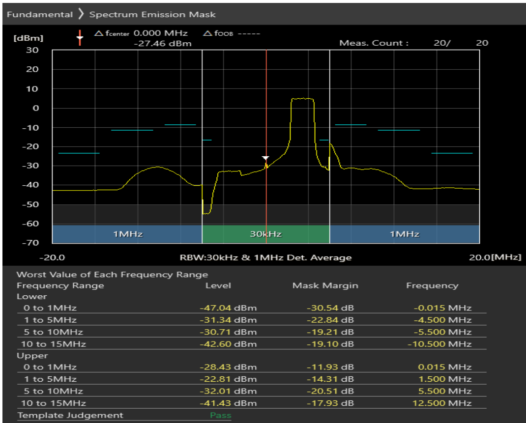
Band7 QPSK BW=10MHz Channel=21400 RB Size=50 Position=#0
