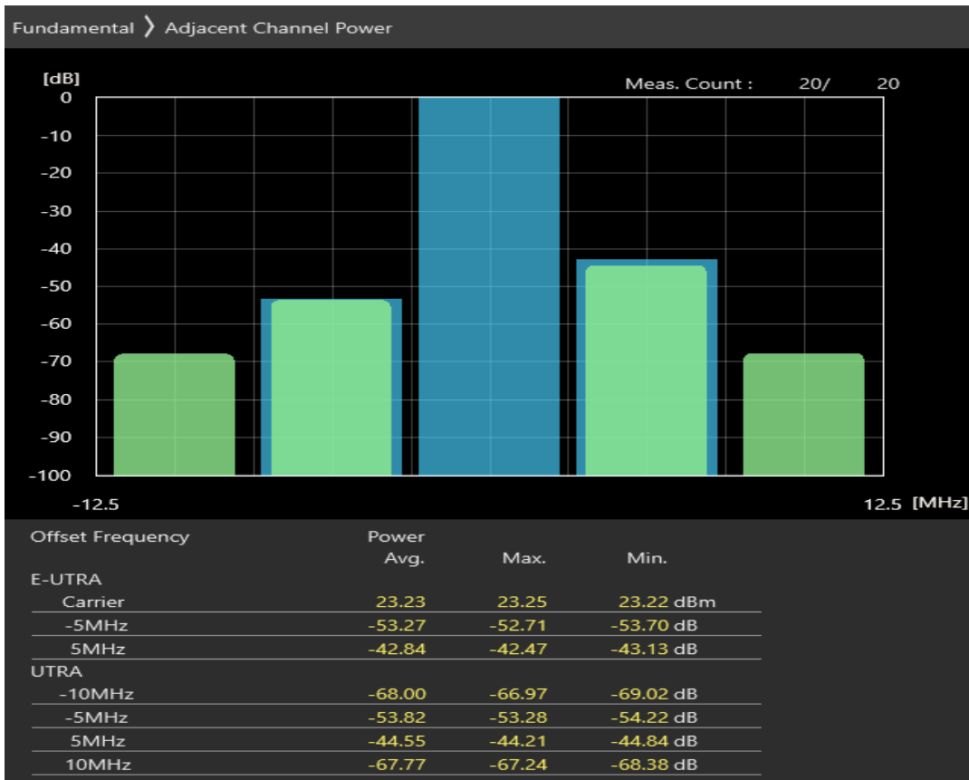
Band20 QPSK BW=5MHz Channel=24425 RB Size=25 Position=#0
