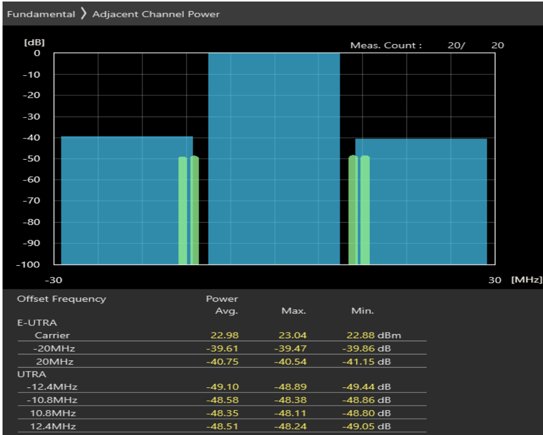
Band7 QPSK BW=5MHz Channel=20775 RB Size=8 Position=#0
