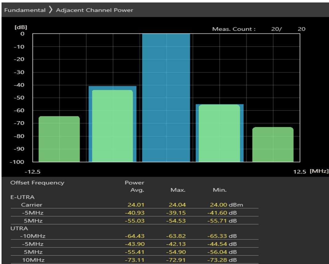
Band8 QPSK BW=5MHz Channel=21775 RB Size=8 Position=#Max
