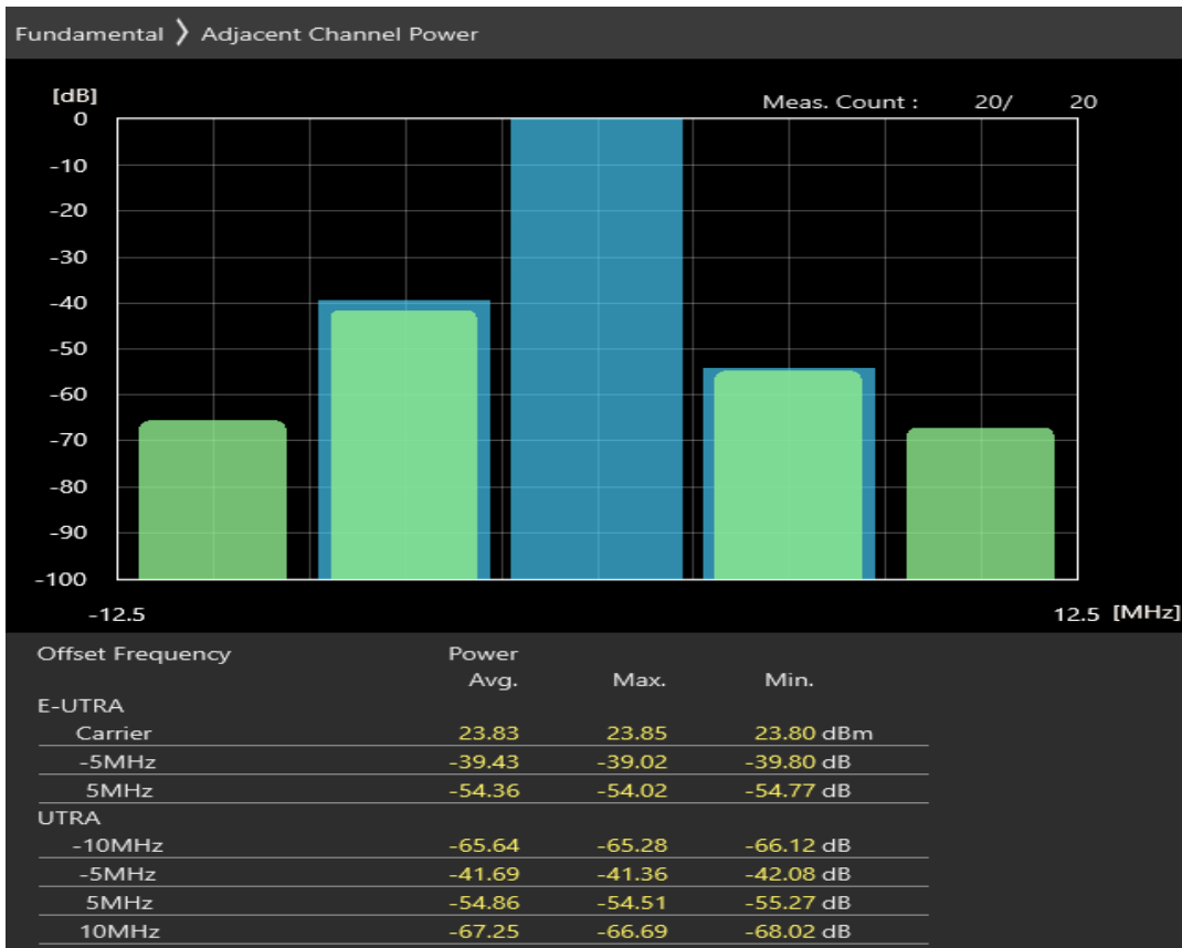
Band7 QPSK BW=5MHz Channel=21100 RB Size=8 Position=#Max
