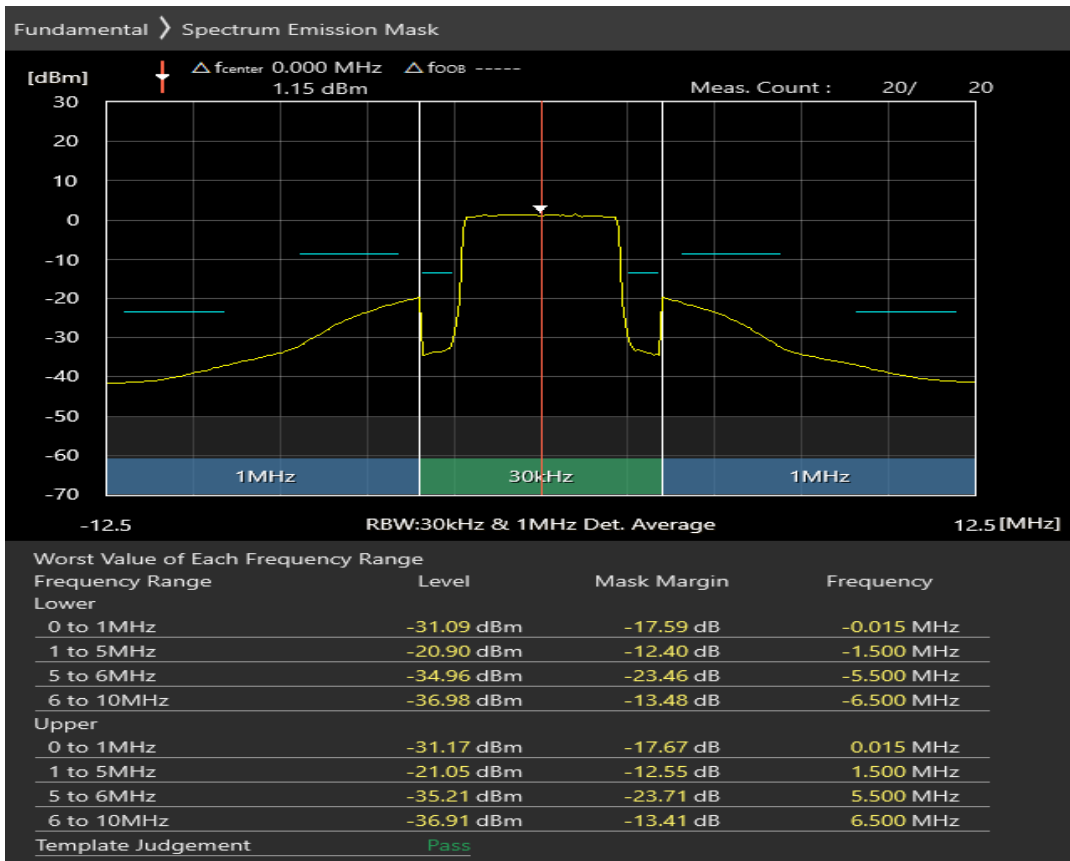
Band7 QPSK BW=5MHz Channel=21100 RB Size=8 Position=#0
