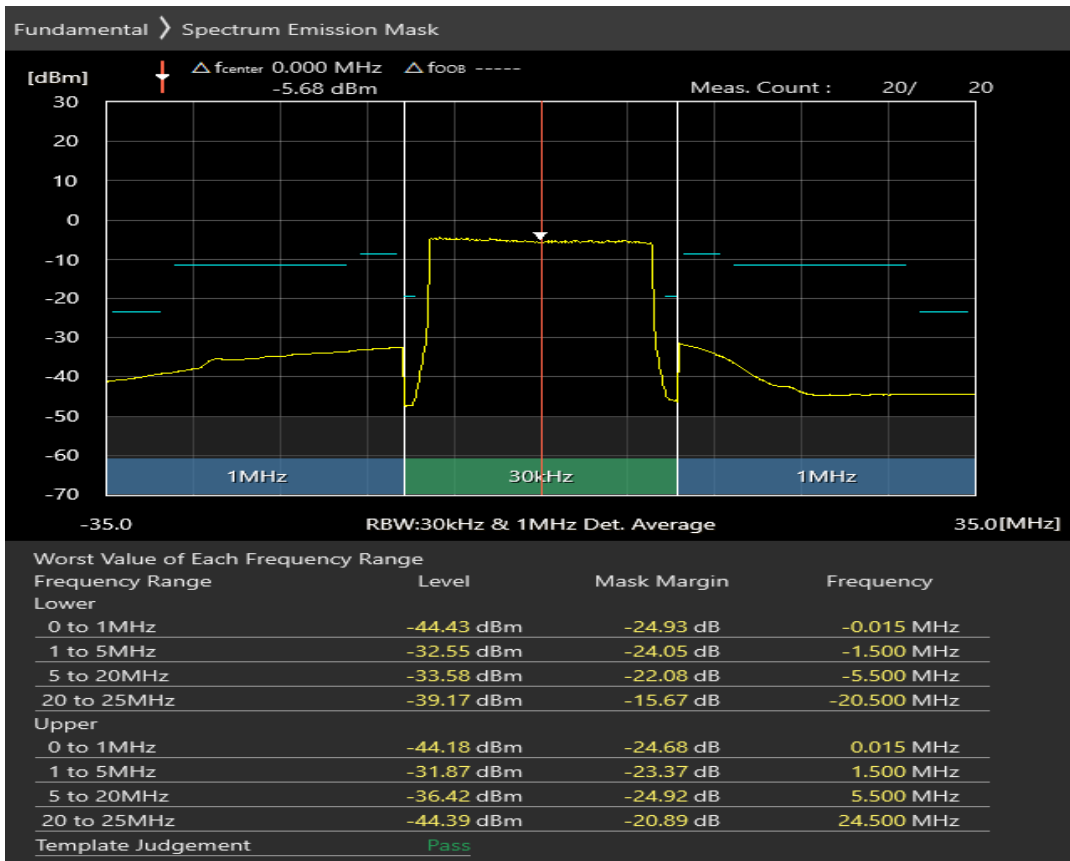
Band40 QPSK BW=5MHz Channel=38675 RB Size=8 Position=#0
