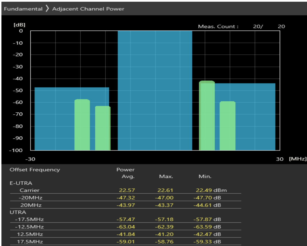
Band7 16QAM BW=20MHz Channel=21350 RB Size=100 Position=#0
