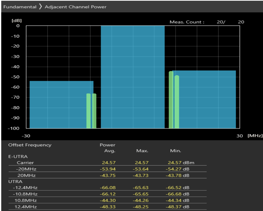
Band40 QPSK BW=20MHz Channel=39150 RB Size=100 Position=#0
