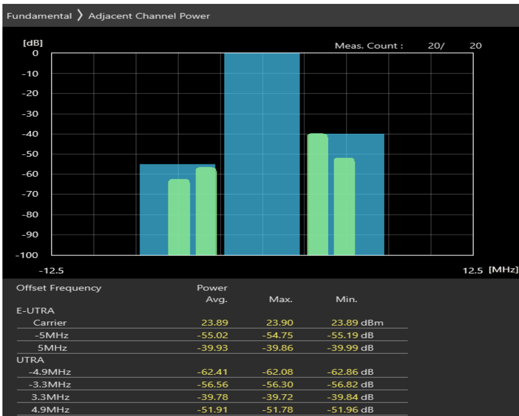
Band40 16QAM BW=5MHz Channel=39150 RB Size=25 Position=#0
