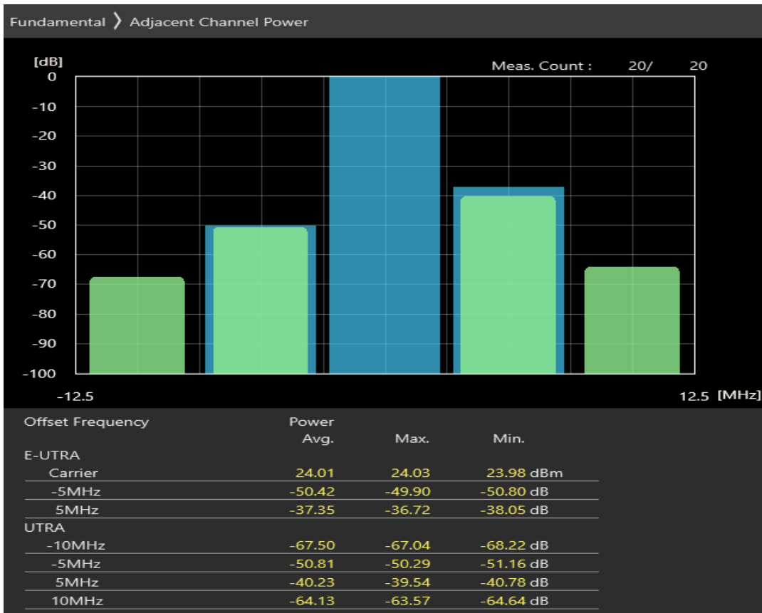
Band7 QPSK BW=5MHz Channel=20775 RB Size=25 Position=#0
