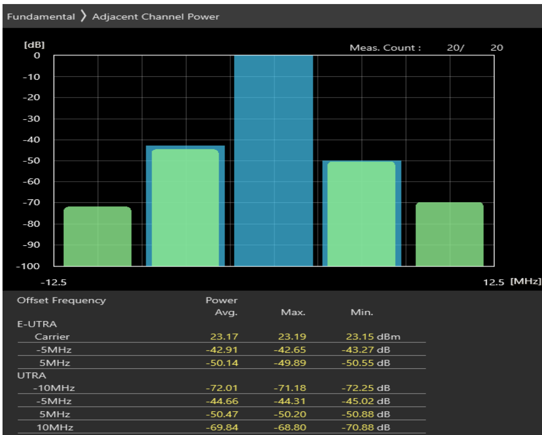
Band20 QPSK BW=5MHz Channel=24175 RB Size=8 Position=#Max
