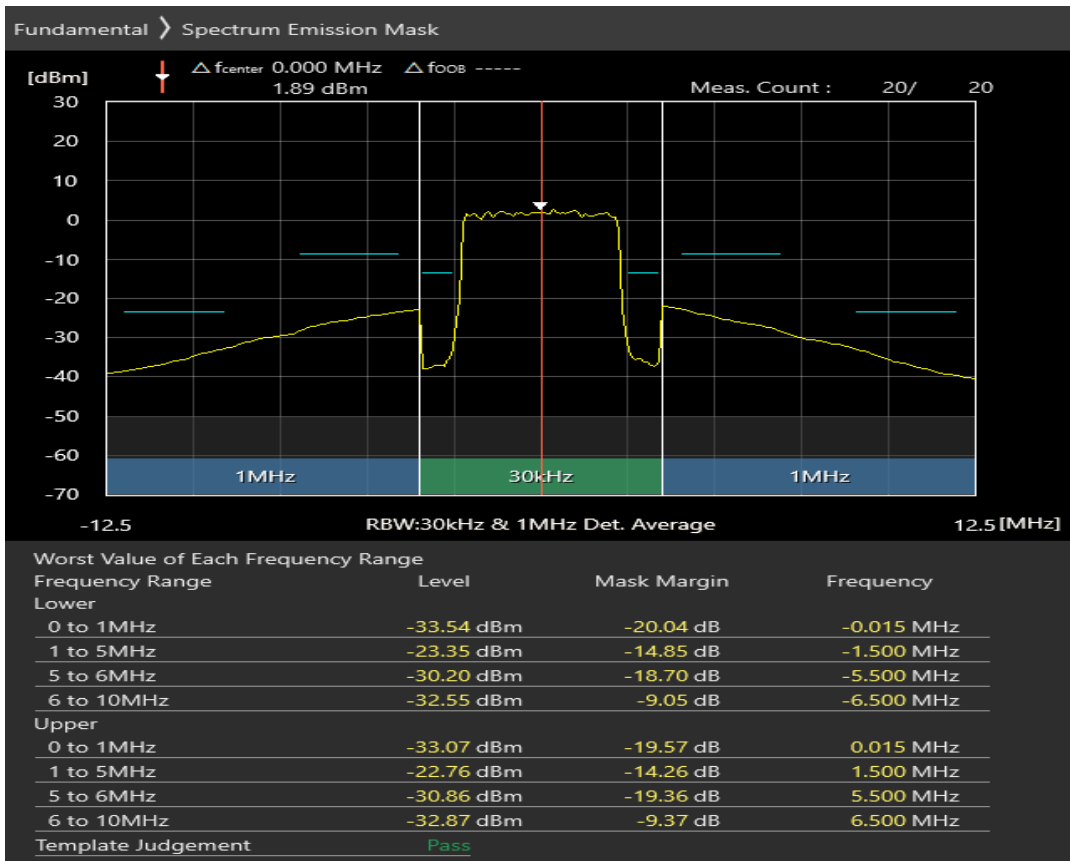
Band40 QPSK BW=10MHz Channel=38700 RB Size=12 Position=#0
