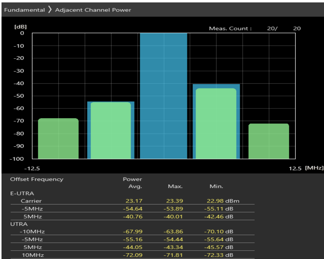
Band8 16QAM BW=5MHz Channel=21775 RB Size=25 Position=#0
