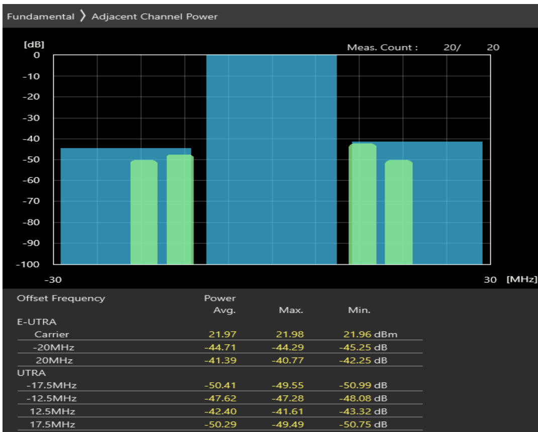
Band20 16QAM BW=20MHz Channel=24350 RB Size=18 Position=#0
