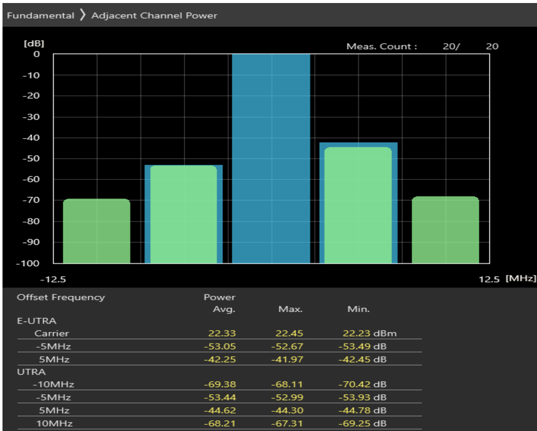
Band20 16QAM BW=5MHz Channel=24425 RB Size=25 Position=#0
