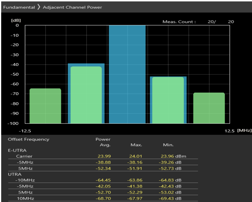
Band8 QPSK BW=5MHz Channel=21625 RB Size=8 Position=#Max
