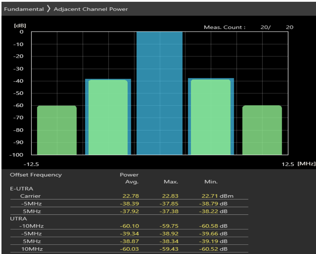
Band1 QPSK BW=5MHz Channel=18575 RB Size=8 Position=#0
