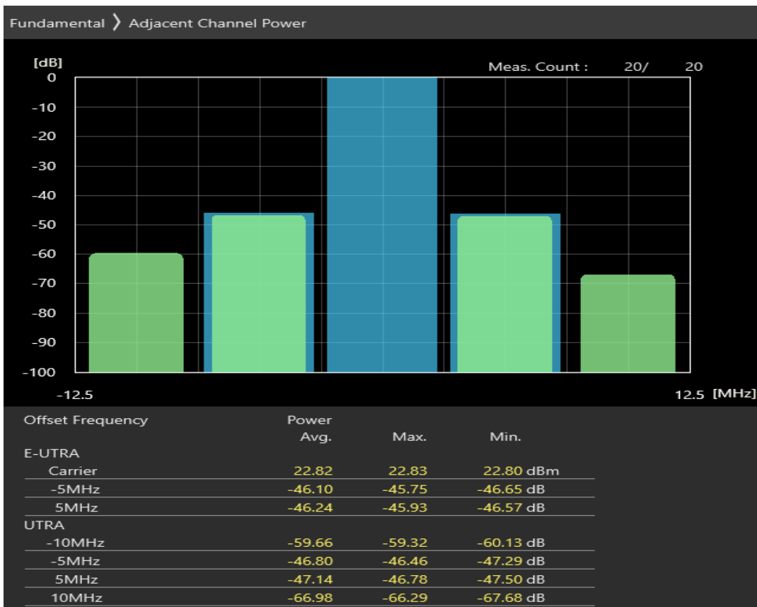
Band3 16QAM BW=5MHz Channel=19925 RB Size=8 Position=#0
