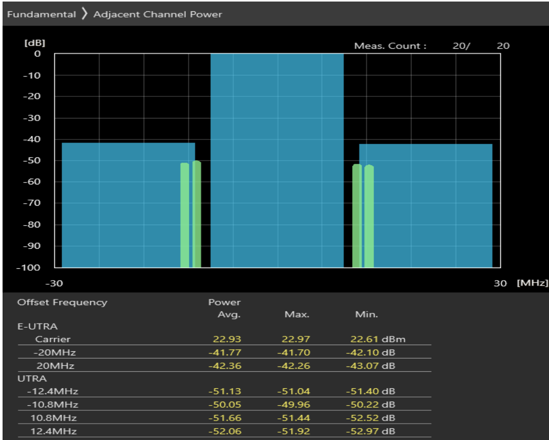
Band40 QPSK BW=20MHz Channel=39550 RB Size=18 Position=#0
