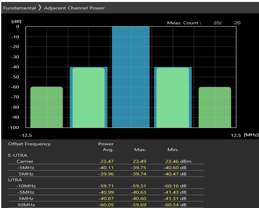
Band1 16QAM BW=5MHz Channel=18025 RB Size=8 Position=#0
