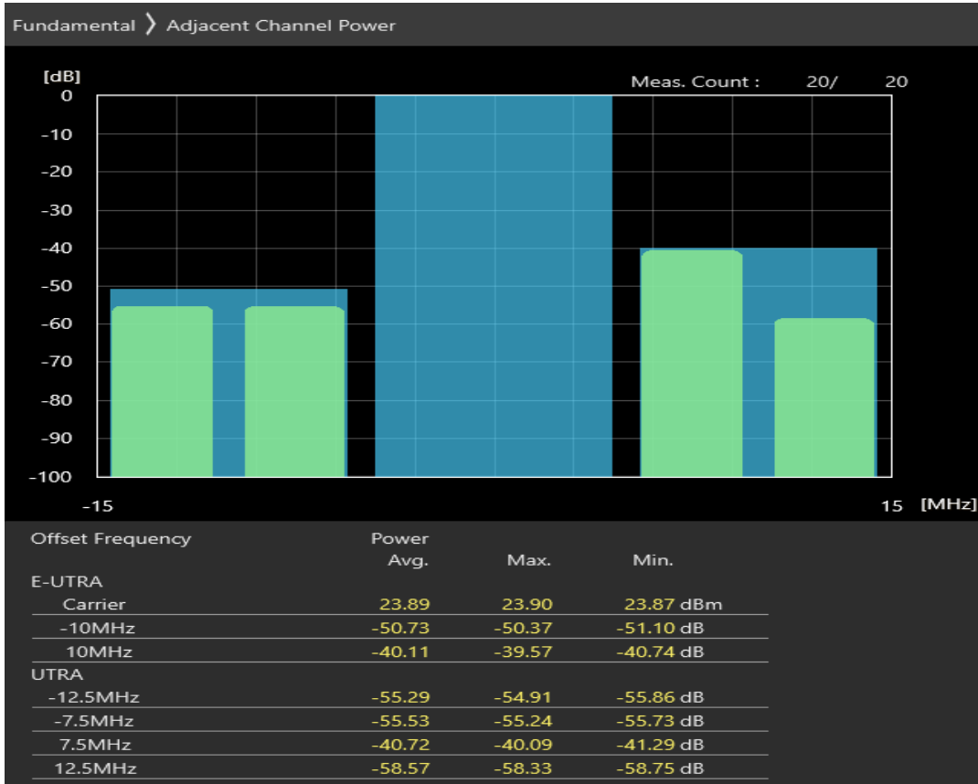
Band7 QPSK BW=10MHz Channel=20800 RB Size=50 Position=#0
