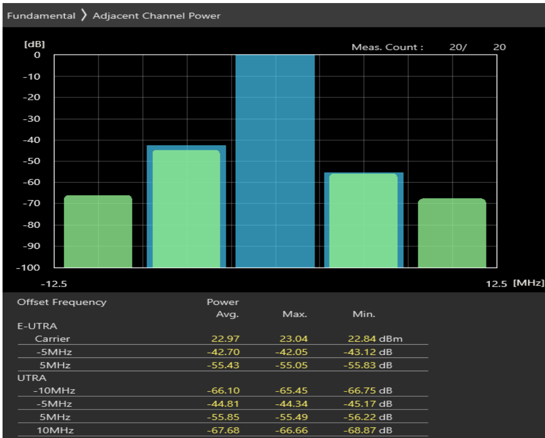
Band3 16QAM BW=5MHz Channel=19575 RB Size=8 Position=#Max
