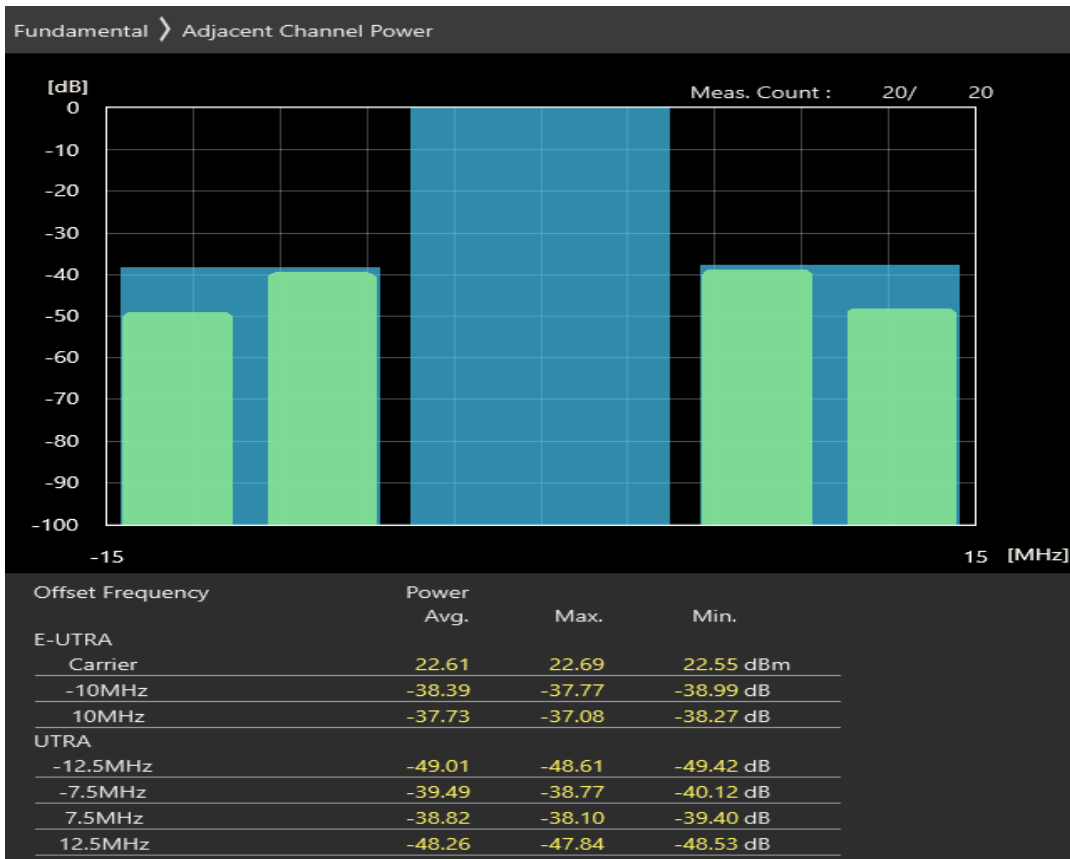
Band1 QPSK BW=10MHz Channel=18550 RB Size=12 Position=#0
