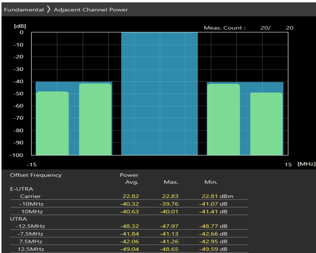
Band7 16QAM BW=10MHz Channel=21100 RB Size=12 Position=#0
