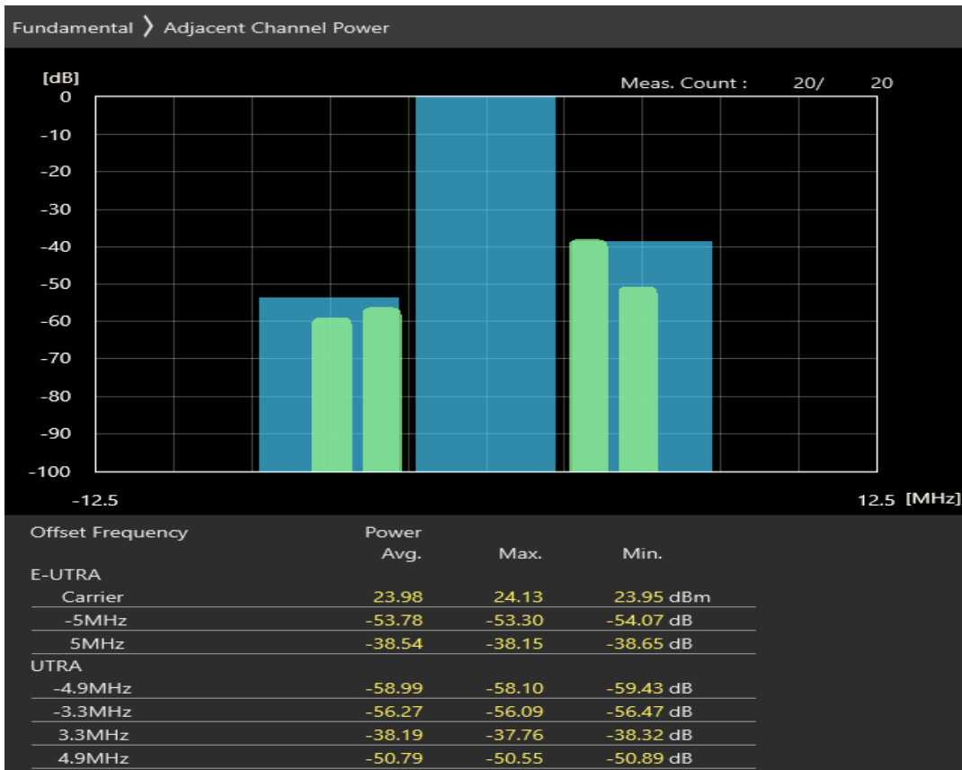
Band40 16QAM BW=5MHz Channel=39625 RB Size=25 Position=#0
