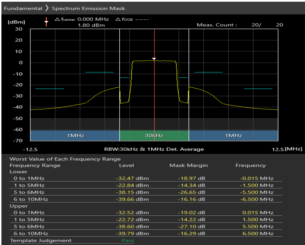
Band1 QPSK BW=5MHz Channel=18300 RB Size=8 Position=#0
