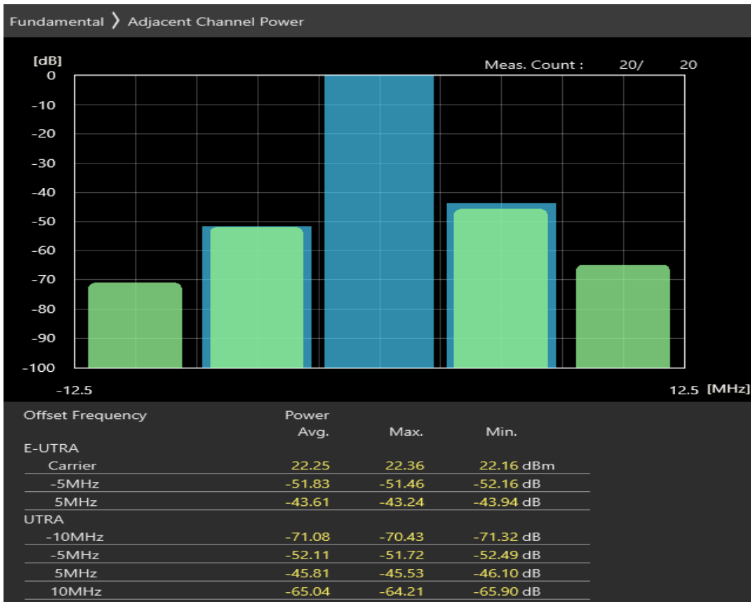
Band20 16QAM BW=5MHz Channel=24300 RB Size=25 Position=#0
