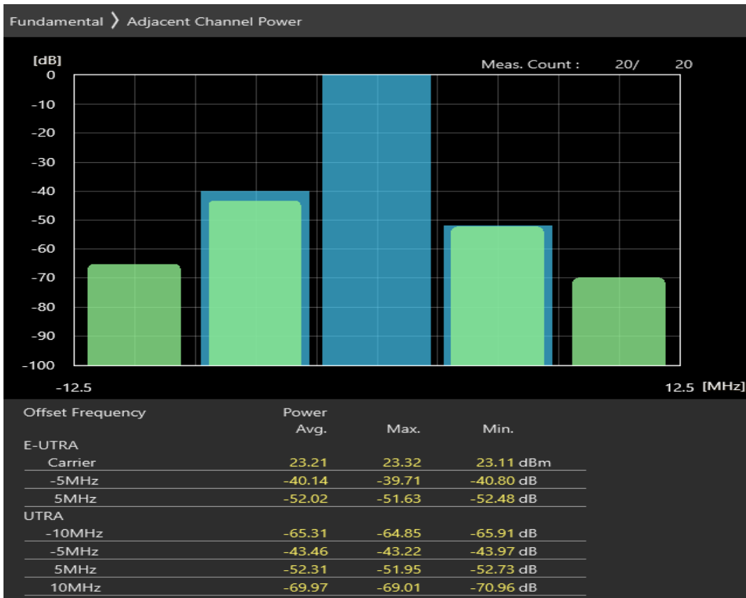
Band8 16QAM BW=5MHz Channel=21625 RB Size=8 Position=#Max
