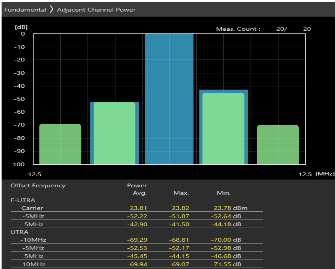
Band3 QPSK BW=5MHz Channel=19925 RB Size=25 Position=#0
