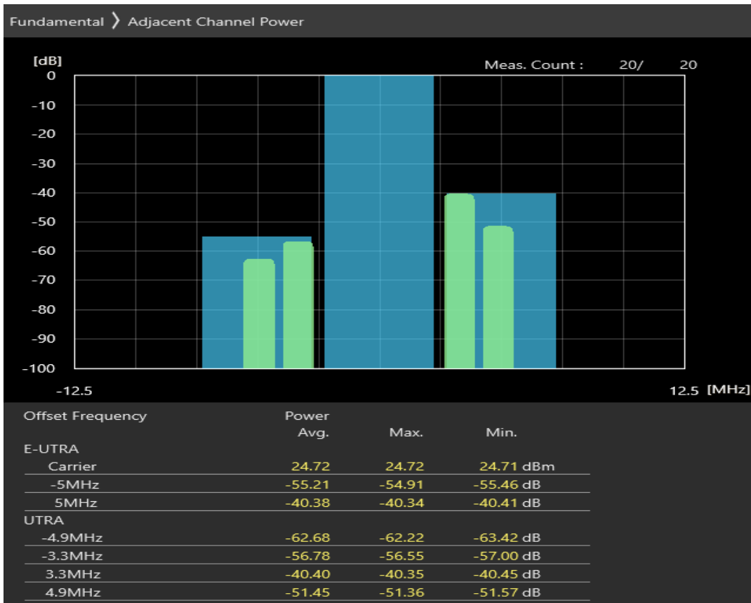
Band40 QPSK BW=5MHz Channel=39150 RB Size=25 Position=#0
