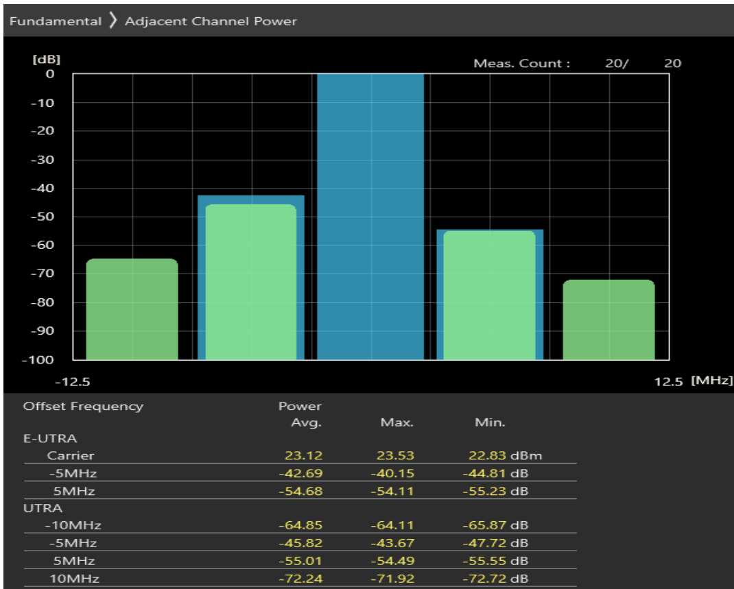
Band8 16QAM BW=5MHz Channel=21775 RB Size=8 Position=#Max
