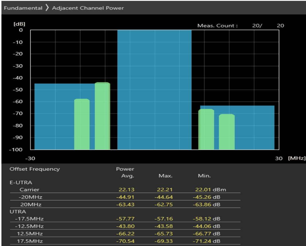
Band20 16QAM BW=20MHz Channel=24350 RB Size=18 Position=#Max
