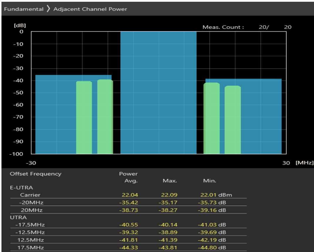
Band8 QPSK BW=1.4MHz Channel=21457 RB Size=5 Position=#0
