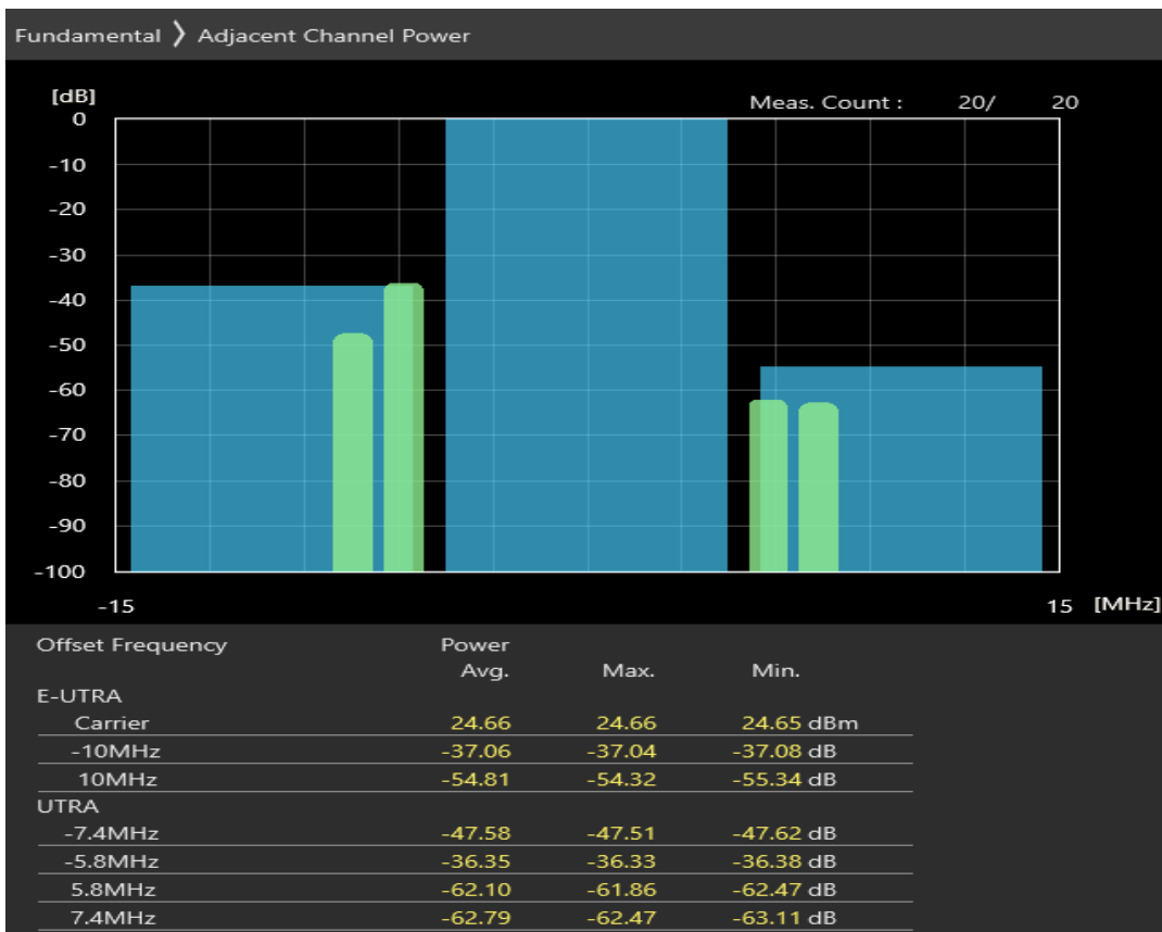
Band40 QPSK BW=10MHz Channel=38700 RB Size=12 Position=#Max
