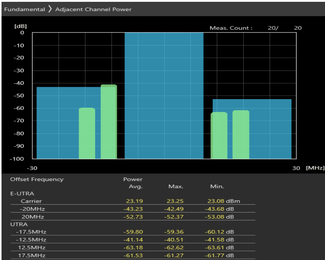
Band7 16QAM BW=20MHz Channel=20850 RB Size=18 Position=#Max
