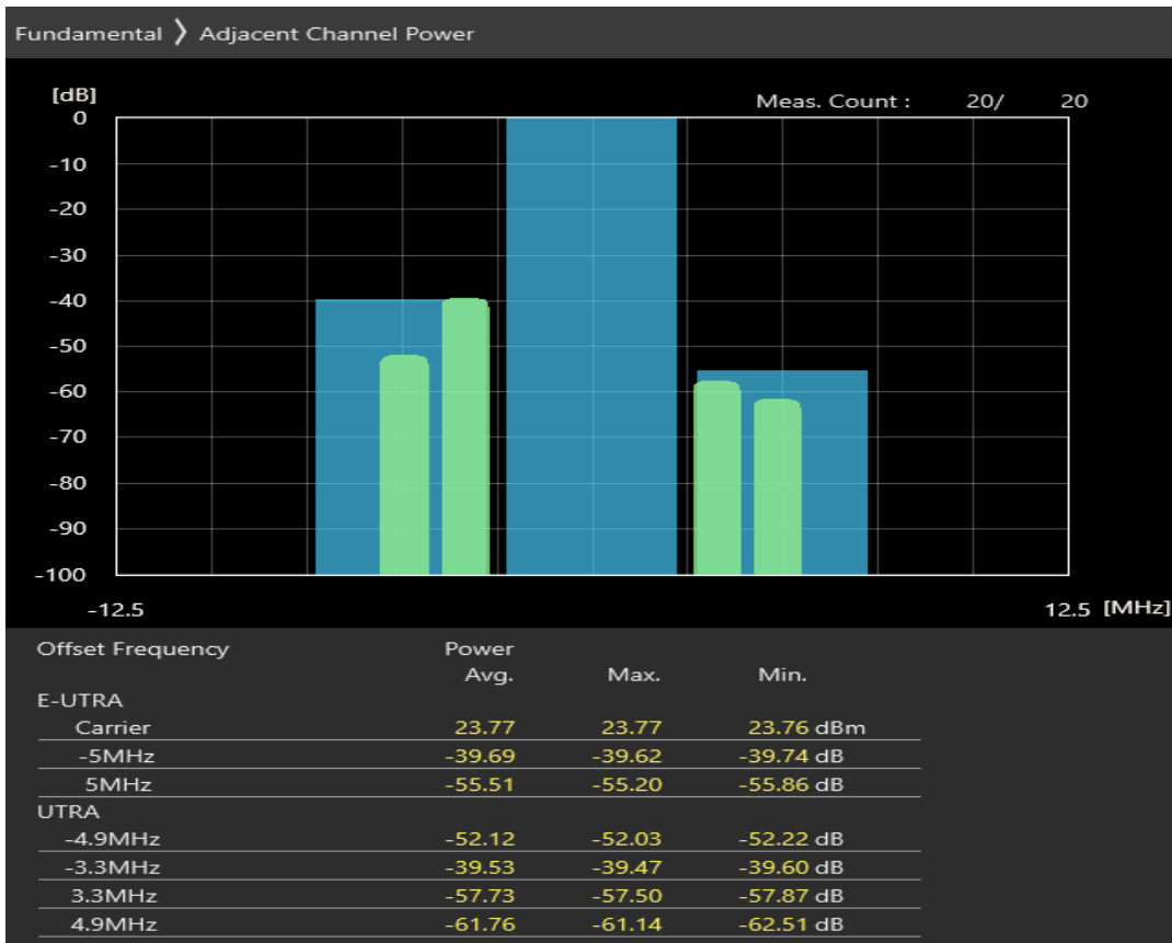
Band40 16QAM BW=5MHz Channel=39150 RB Size=8 Position=#Max
