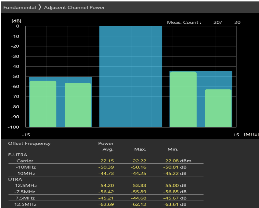
Band20 16QAM BW=10MHz Channel=24300 RB Size=50 Position=#0
