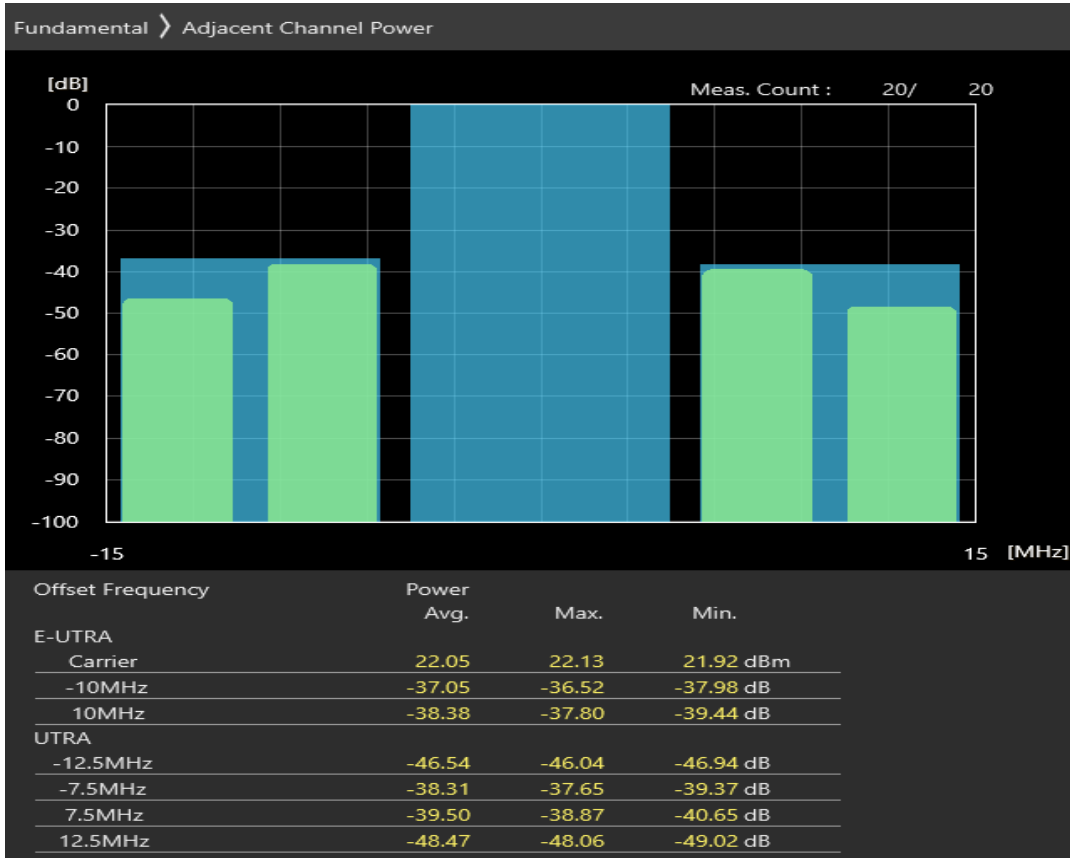
Band7 QPSK BW=20MHz Channel=20850 RB Size=18 Position=#0
