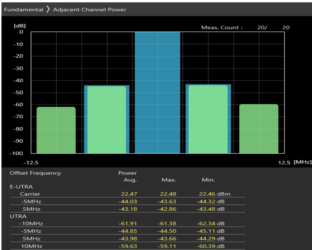
Band3 16QAM BW=5MHz Channel=19225 RB Size=8 Position=#0
