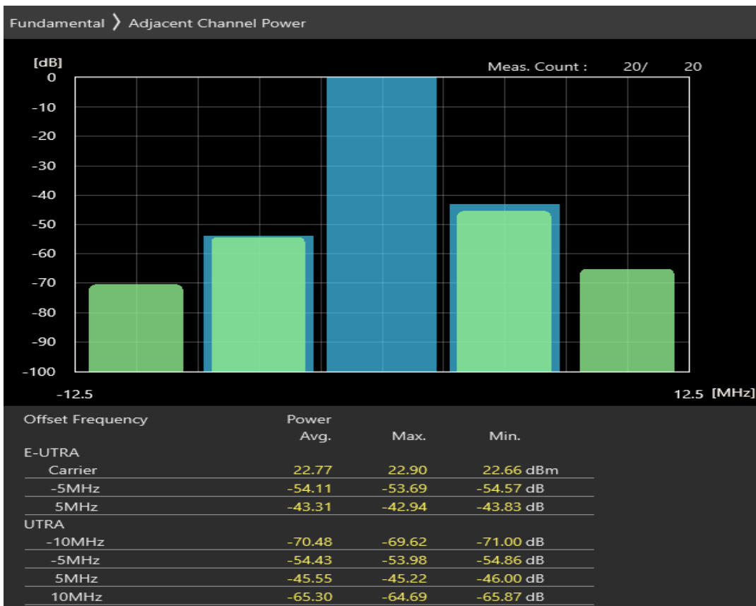
Band3 16QAM BW=5MHz Channel=19225 RB Size=25 Position=#0
