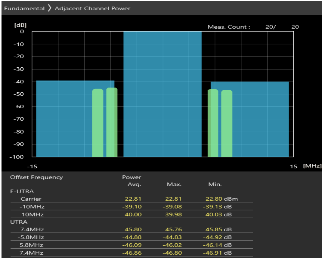
Band40 QPSK BW=10MHz Channel=39150 RB Size=12 Position=#0
