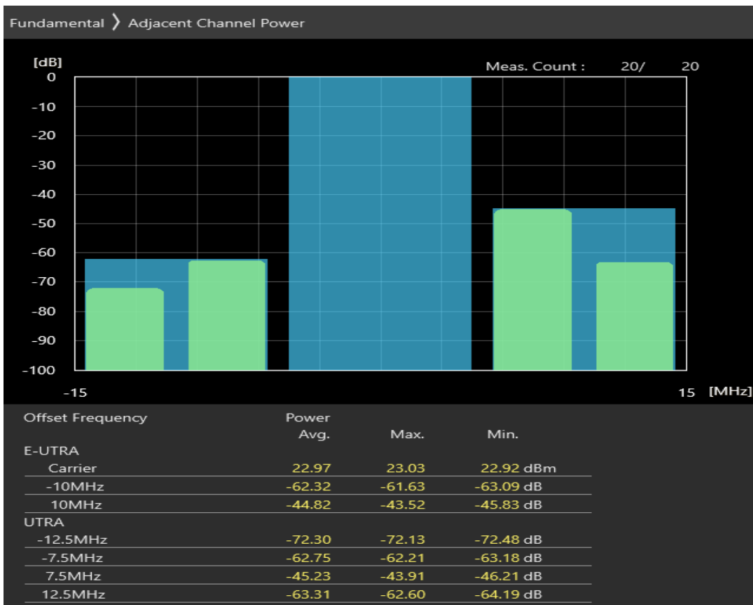
Band8 16QAM BW=10MHz Channel=21500 RB Size=50 Position=#0
