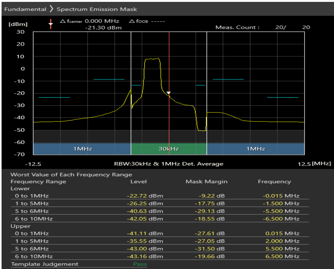
Band1 16QAM BW=5MHz Channel=18025 RB Size=8 Position=#Max
