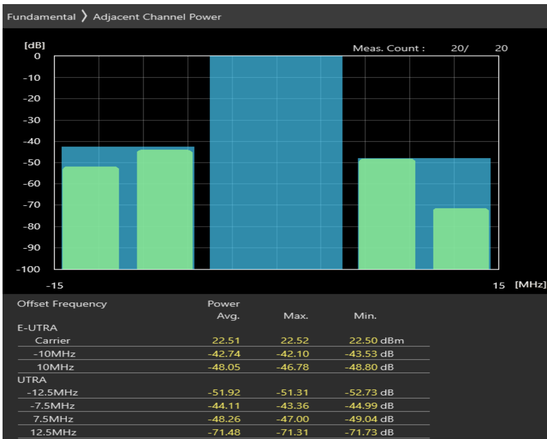
Band8 16QAM BW=10MHz Channel=21750 RB Size=12 Position=#0
