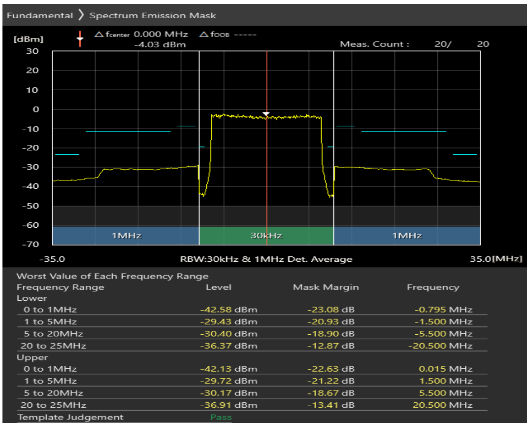
Band40 16QAM BW=20MHz Channel=39150 RB Size=18 Position=#0
