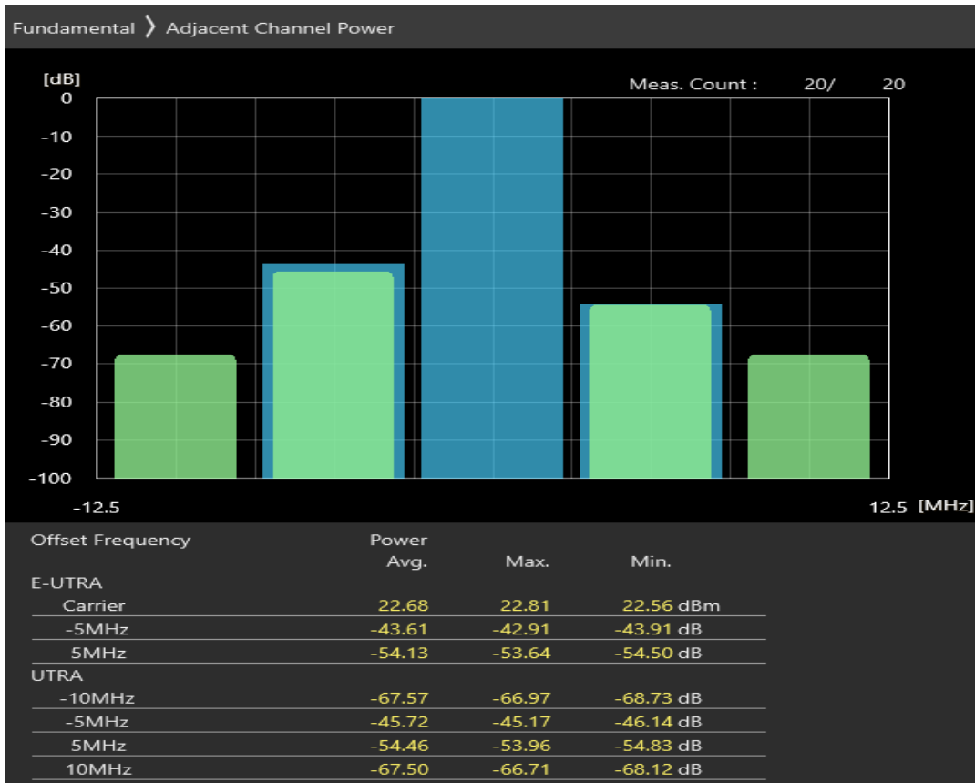
Band3 16QAM BW=5MHz Channel=19225 RB Size=8 Position=#Max
