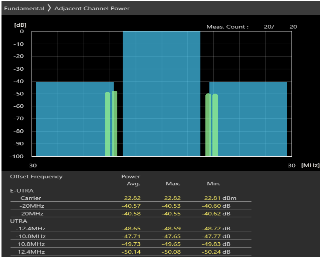
Band40 QPSK BW=20MHz Channel=39150 RB Size=18 Position=#0
