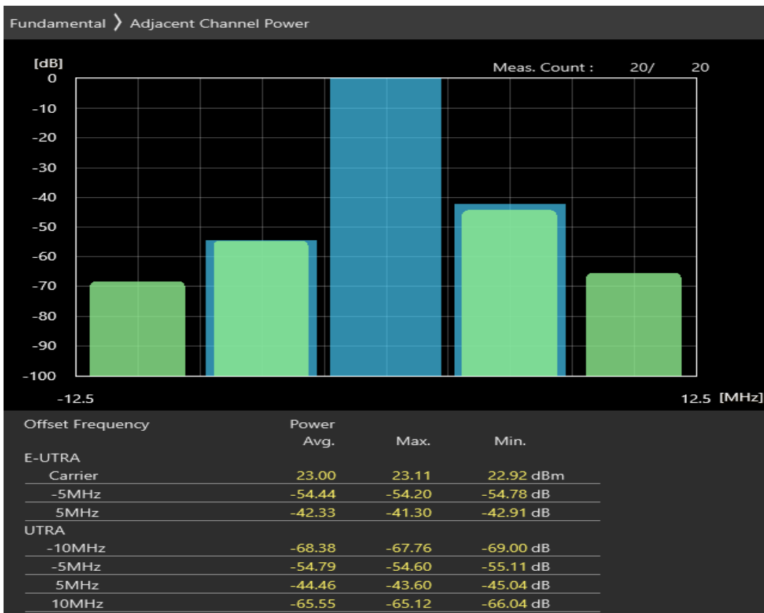
Band3 16QAM BW=5MHz Channel=19575 RB Size=25 Position=#0
