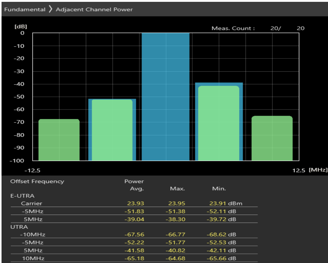
Band7 QPSK BW=5MHz Channel=21100 RB Size=25 Position=#0
