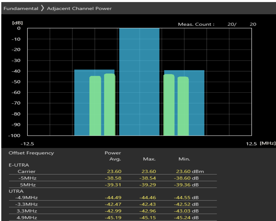
Band40 16QAM BW=5MHz Channel=38675 RB Size=8 Position=#0
