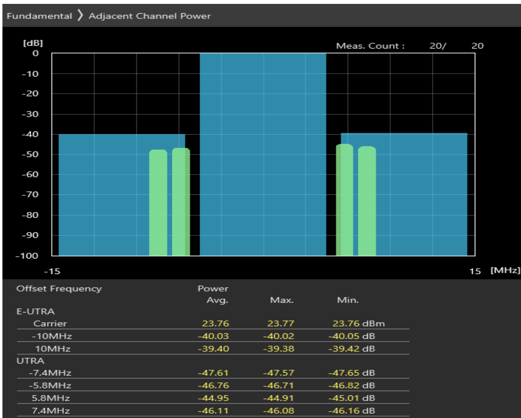
Band40 16QAM BW=10MHz Channel=39600 RB Size=12 Position=#0
