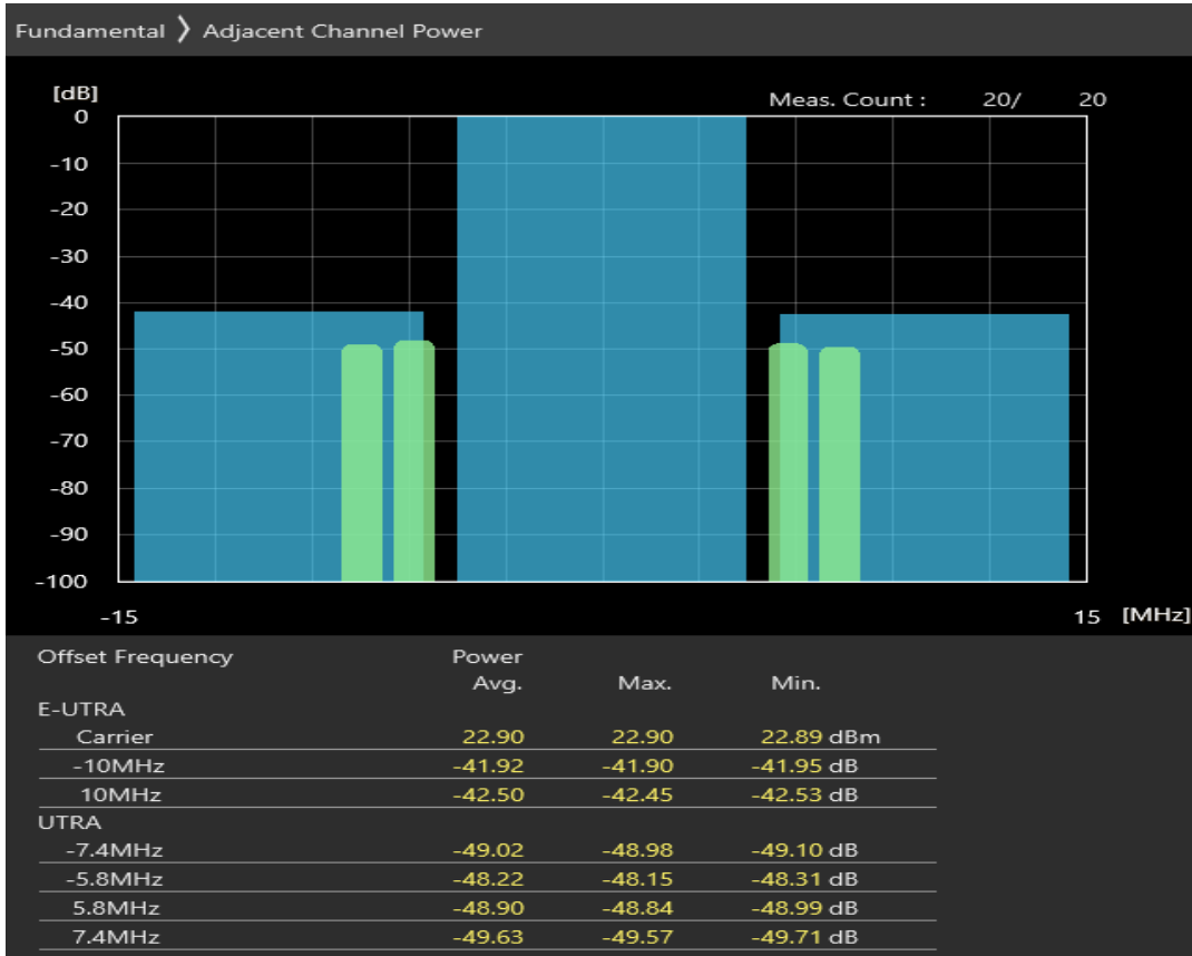
Band40 QPSK BW=10MHz Channel=39600 RB Size=12 Position=#0
