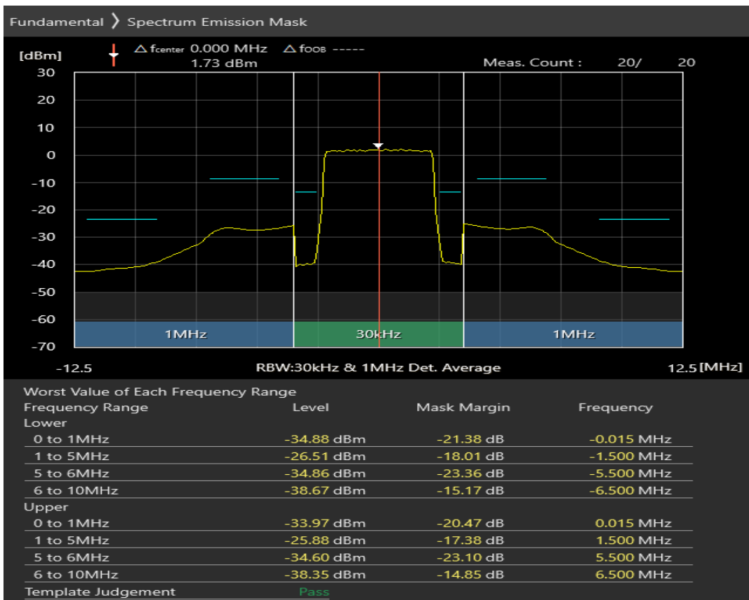
Band3 16QAM BW=5MHz Channel=19575 RB Size=8 Position=#0
