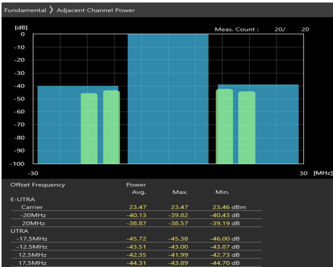
Band1 16QAM BW=20MHz Channel=18100 RB Size=18 Position=#0
