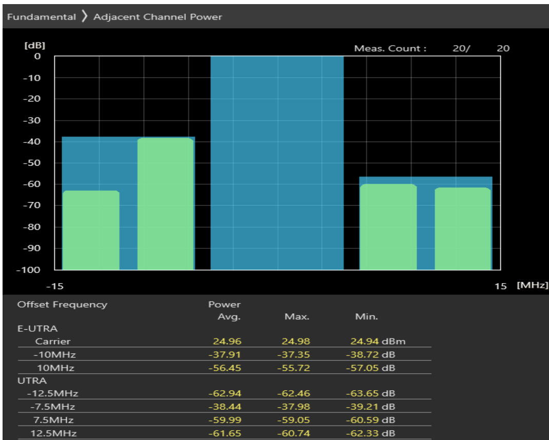
Band1 QPSK BW=10MHz Channel=18300 RB Size=12 Position=#Max
