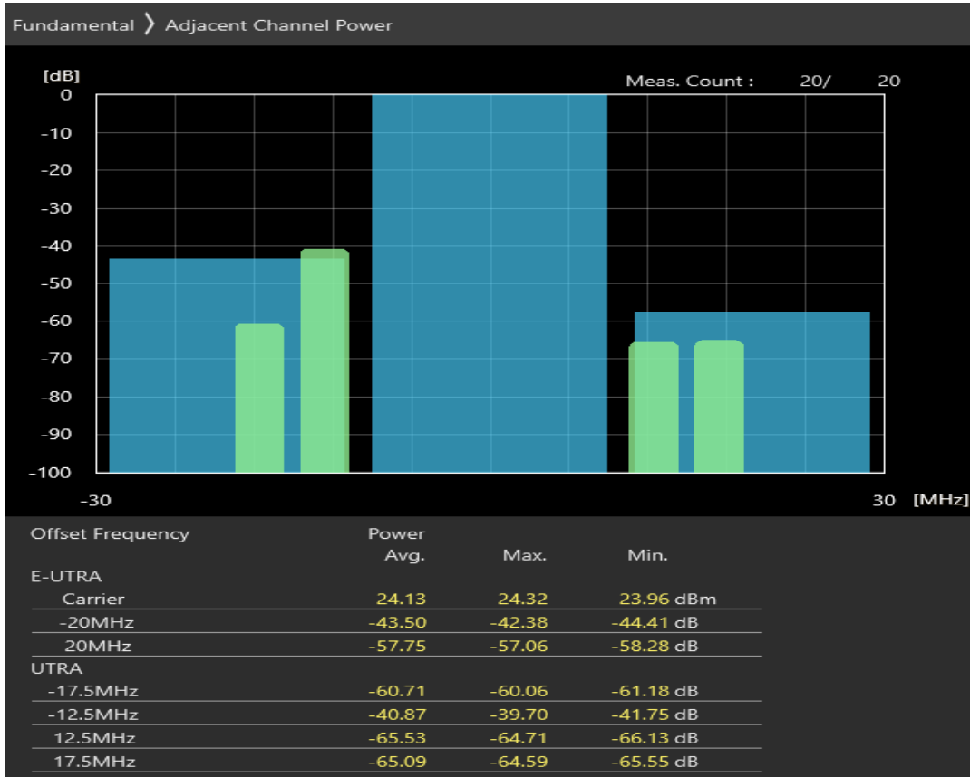
Band1 16QAM BW=20MHz Channel=18100 RB Size=18 Position=#Max
