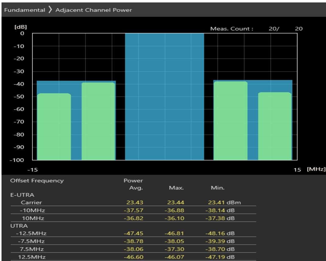
Band1 16QAM BW=10MHz Channel=18300 RB Size=12 Position=#0
