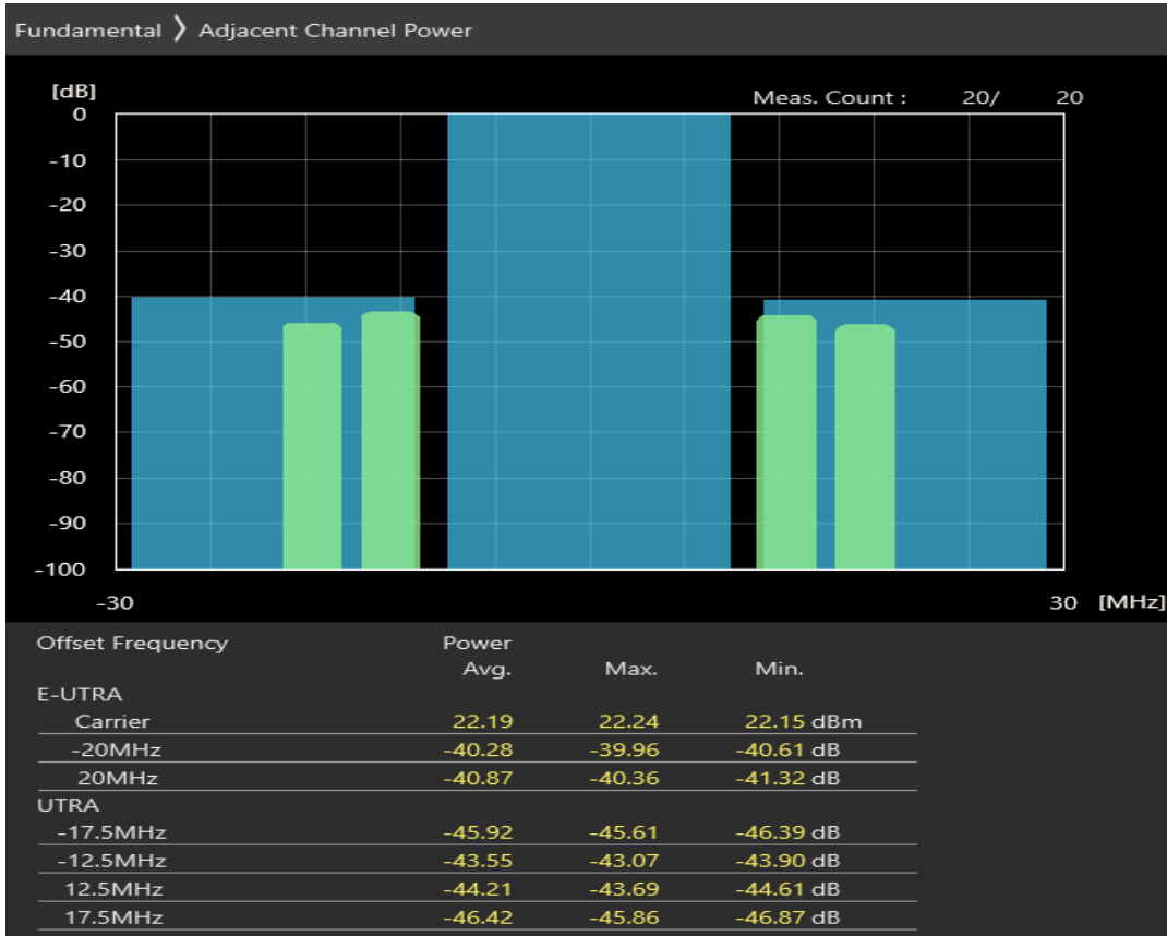
Band7 QPSK BW=20MHz Channel=21350 RB Size=18 Position=#0
