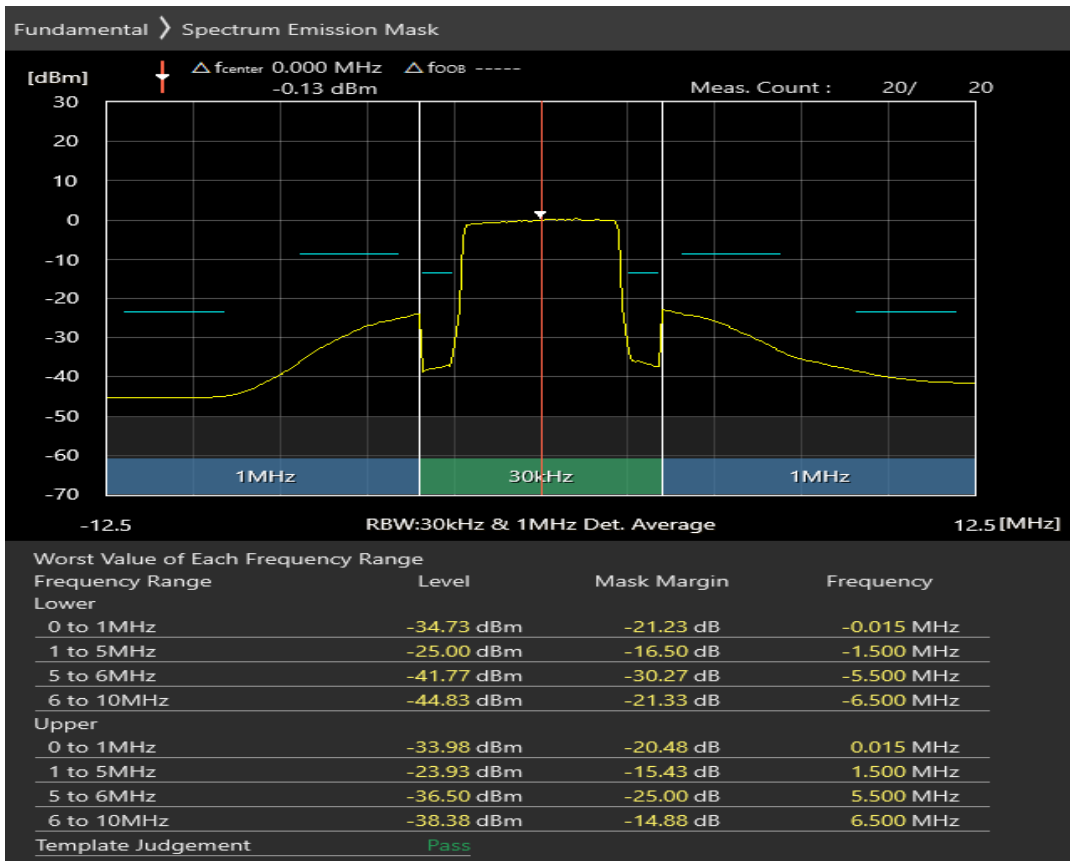
Band20 QPSK BW=5MHz Channel=24300 RB Size=8 Position=#0
