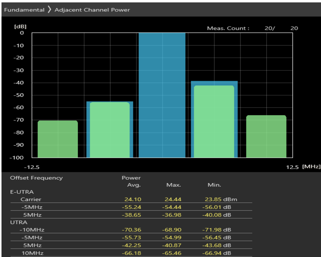
Band1 16QAM BW=5MHz Channel=18025 RB Size=25 Position=#0
