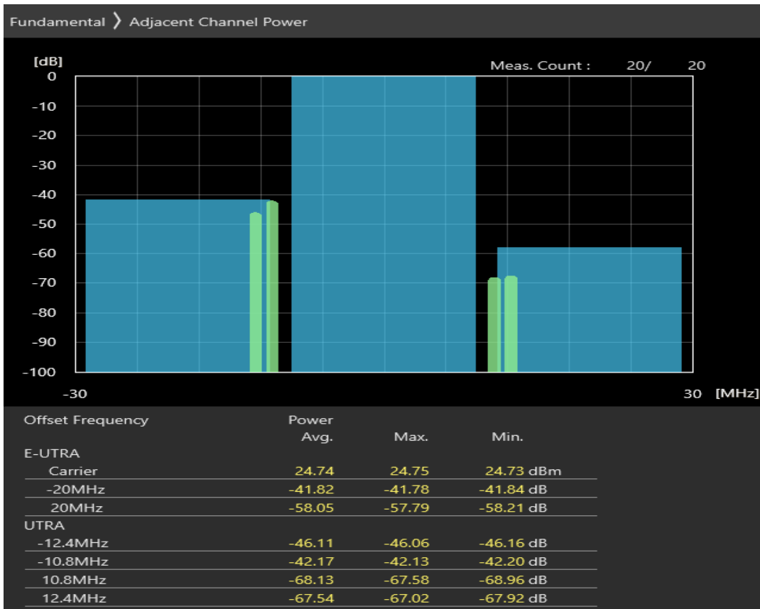
Band40 QPSK BW=20MHz Channel=39550 RB Size=18 Position=#Max
