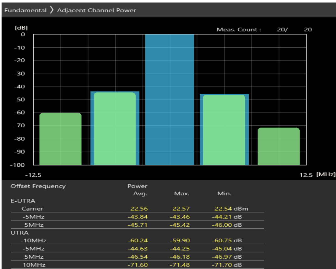
Band8 16QAM BW=5MHz Channel=21775 RB Size=8 Position=#0
