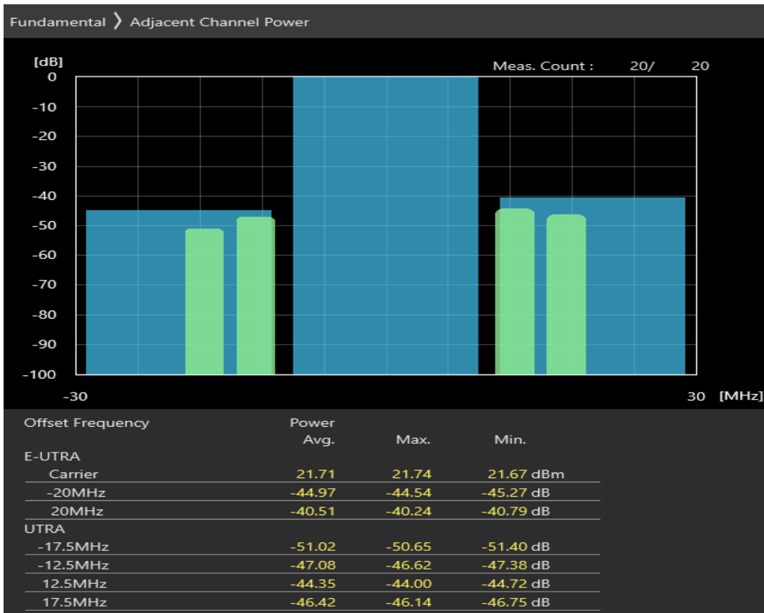
Band3 QPSK BW=20MHz Channel=19575 RB Size=18 Position=#0
