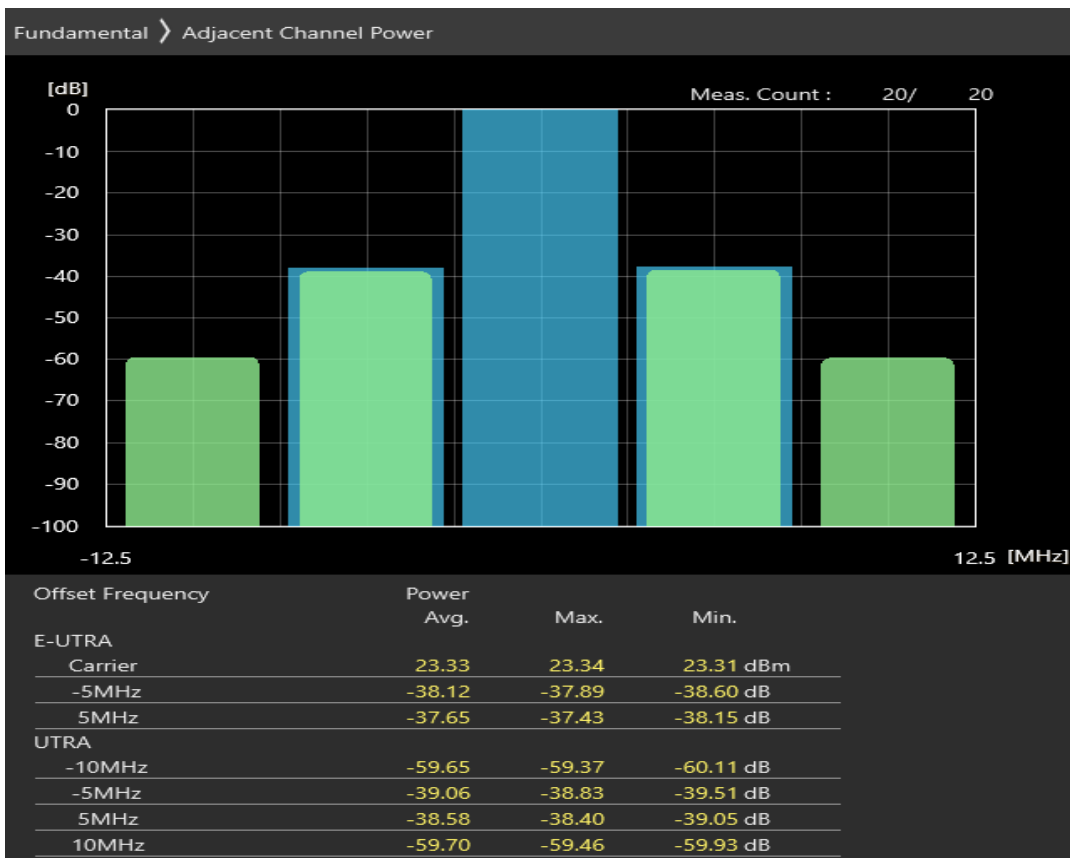
Band1 16QAM BW=5MHz Channel=18300 RB Size=8 Position=#0
