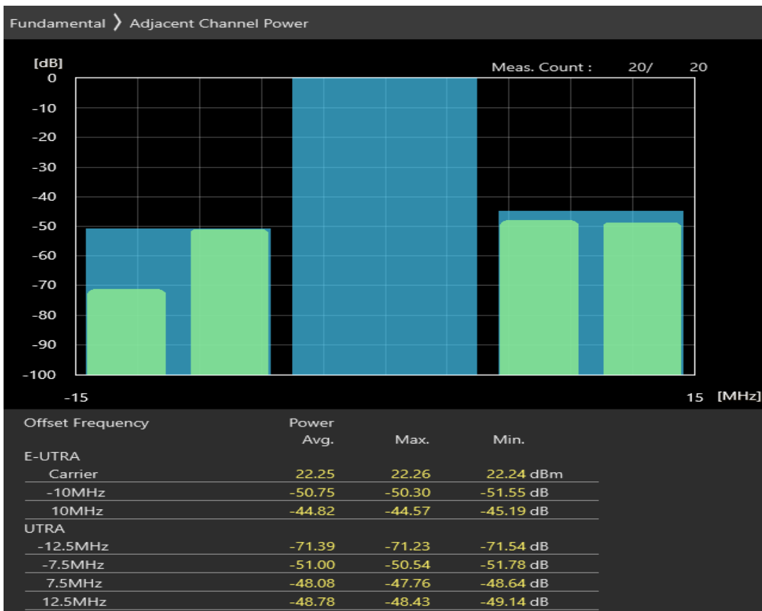
Band8 16QAM BW=10MHz Channel=21500 RB Size=12 Position=#0
