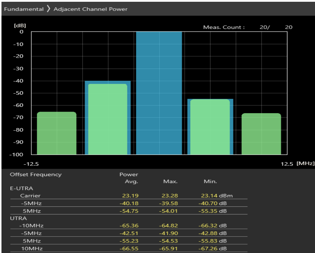
Band7 16QAM BW=5MHz Channel=21100 RB Size=8 Position=#Max
