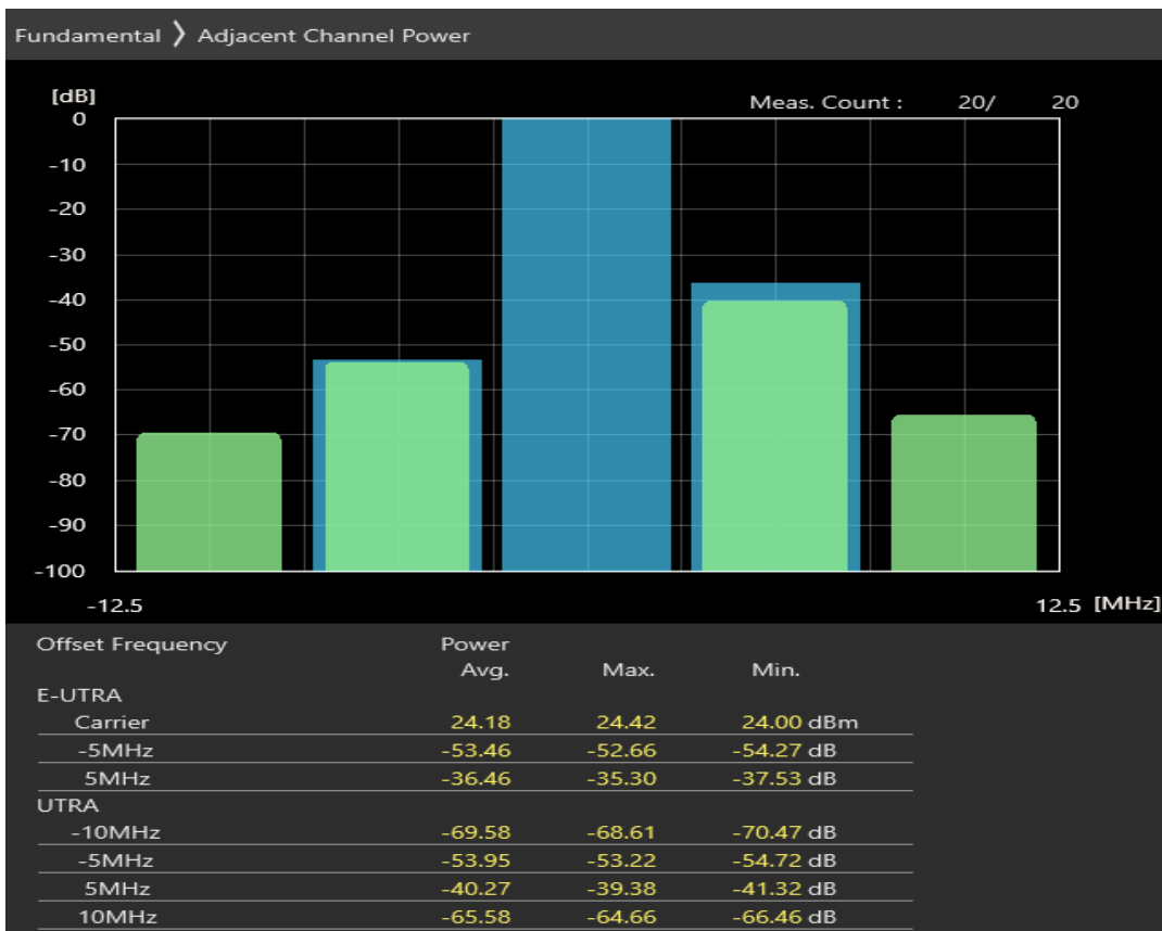
Band1 16QAM BW=5MHz Channel=18575 RB Size=25 Position=#0
