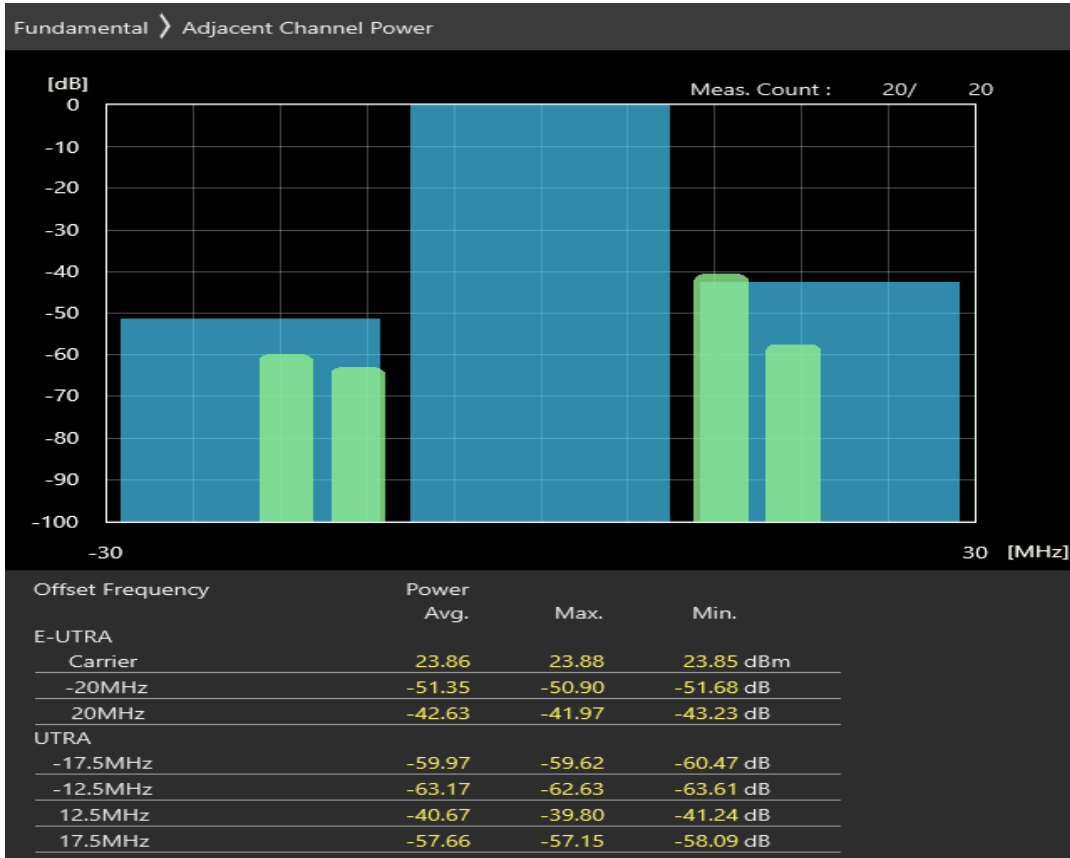
Band7 QPSK BW=20MHz Channel=20850 RB Size=100 Position=#0
