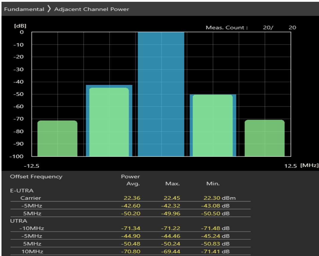
Band20 16QAM BW=5MHz Channel=24175 RB Size=8 Position=#Max
