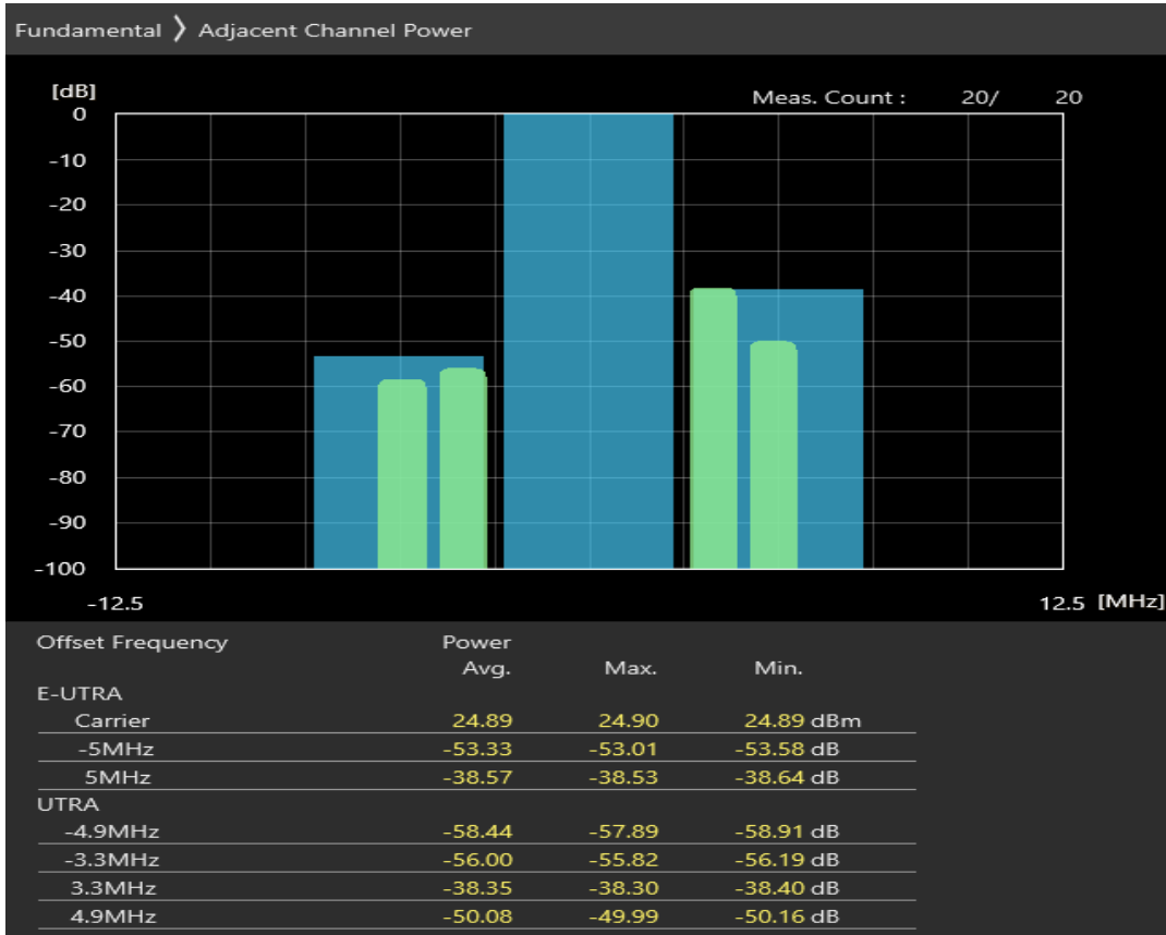
Band40 QPSK BW=5MHz Channel=39625 RB Size=25 Position=#0
