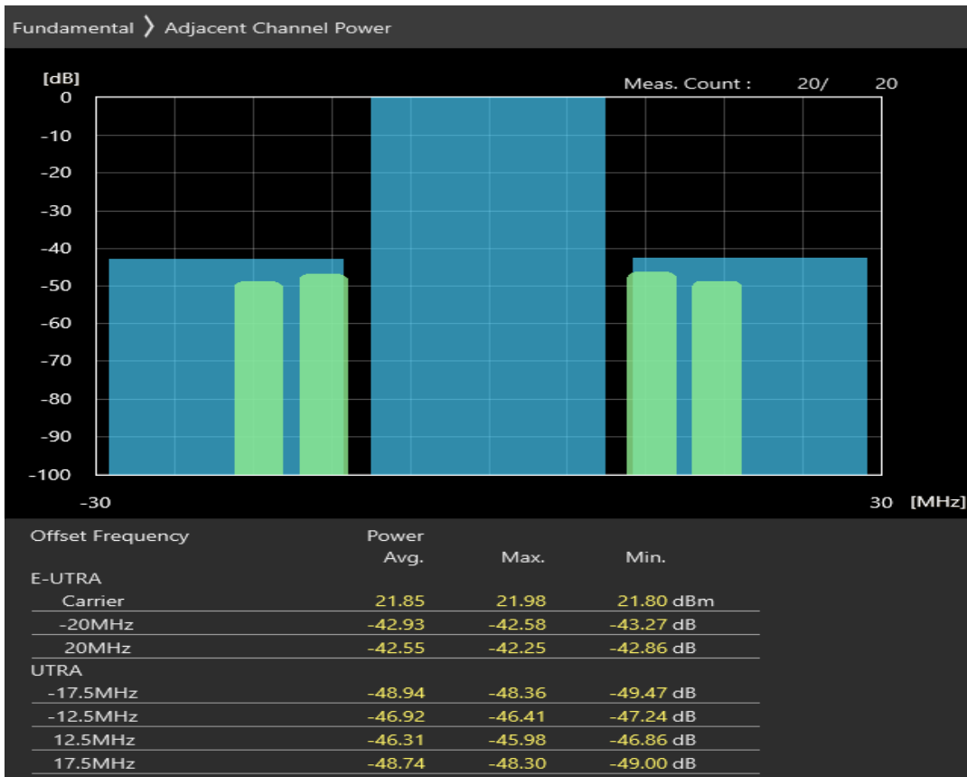
Band3 QPSK BW=20MHz Channel=19850 RB Size=18 Position=#0
