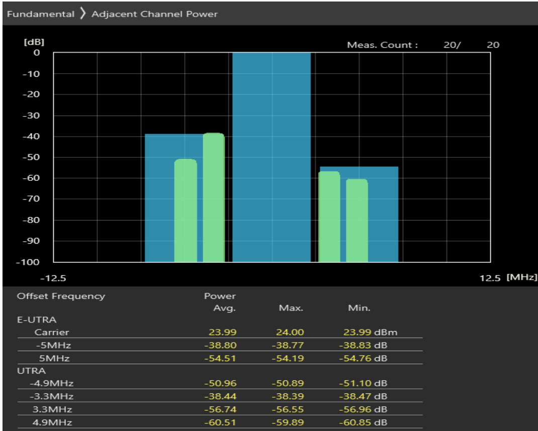
Band40 16QAM BW=5MHz Channel=39625 RB Size=8 Position=#Max
