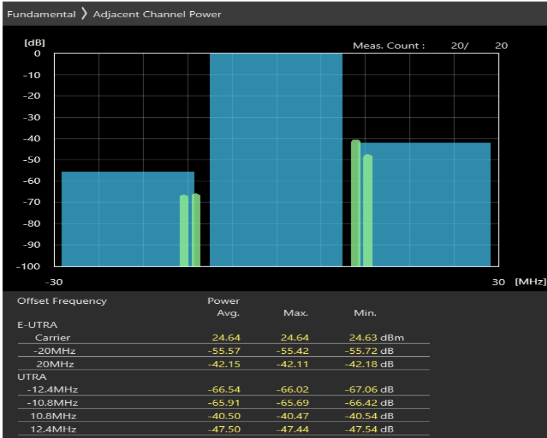
Band40 QPSK BW=20MHz Channel=39550 RB Size=100 Position=#0
