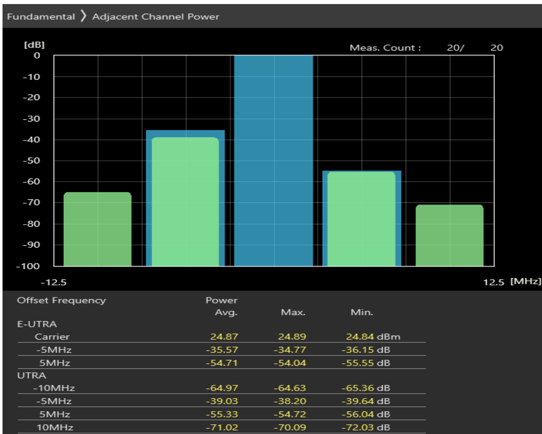
Band1 QPSK BW=5MHz Channel=18575 RB Size=8 Position=#Max
