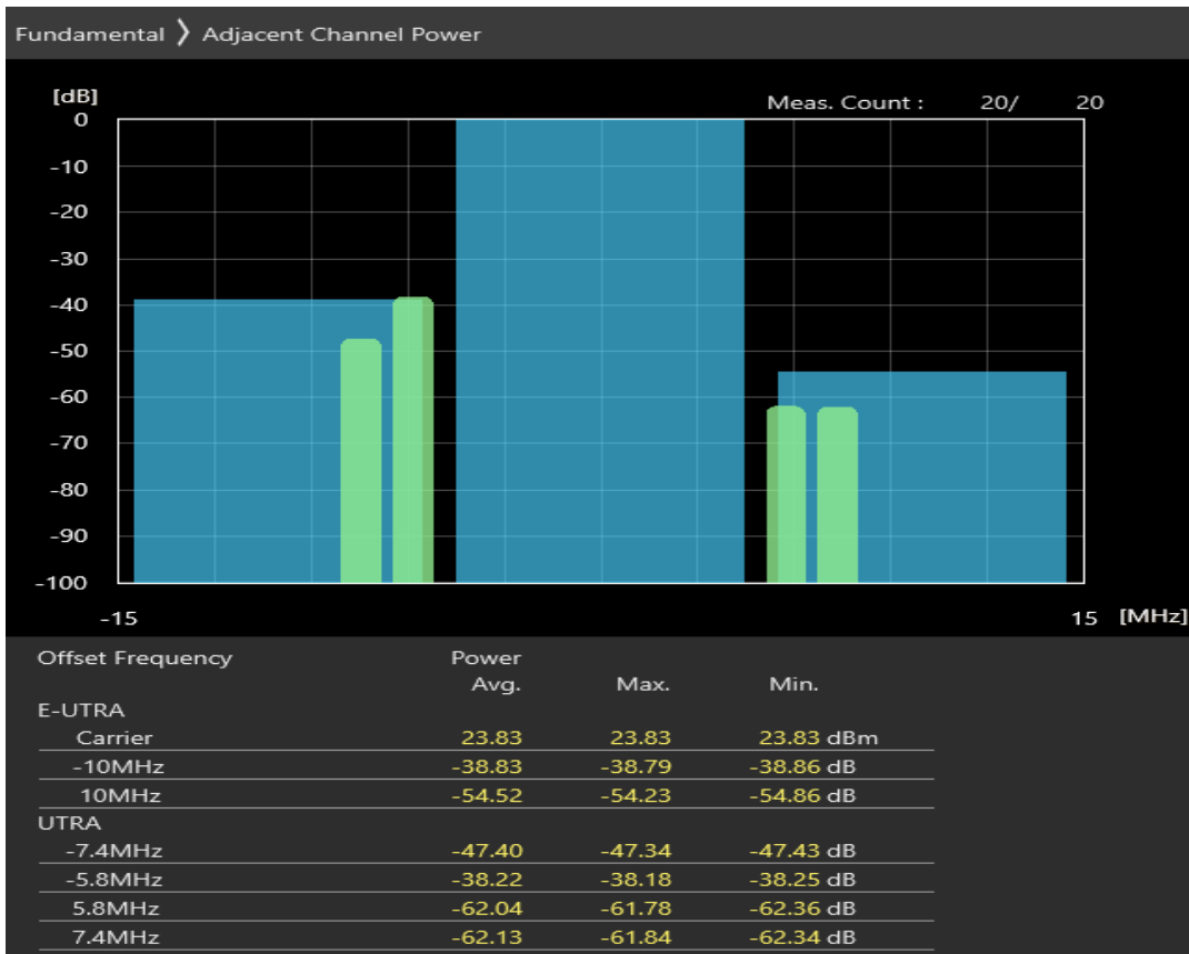
Band40 16QAM BW=10MHz Channel=38700 RB Size=12 Position=#Max
