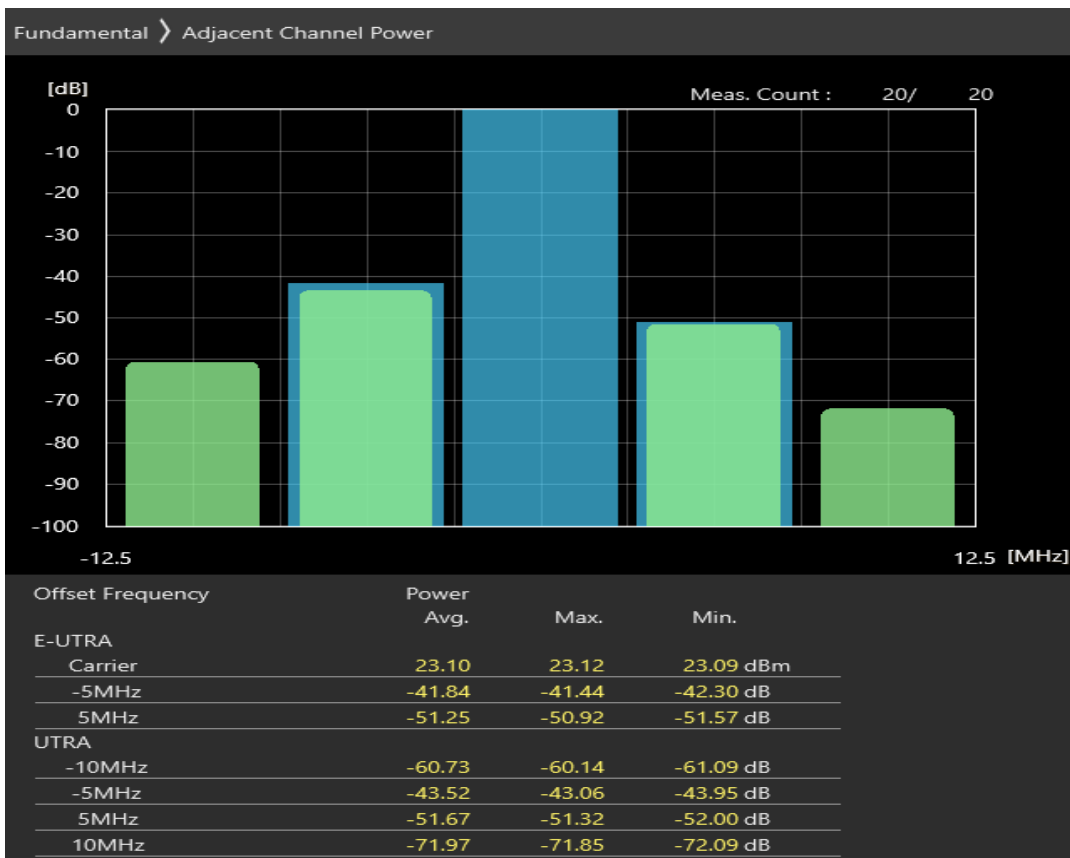
Band20 QPSK BW=5MHz Channel=24425 RB Size=8 Position=#Max
