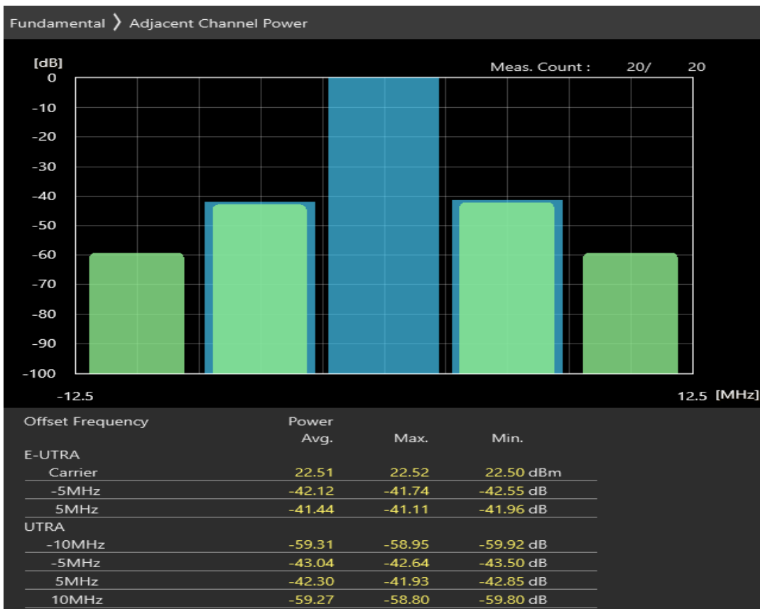
Band8 16QAM BW=5MHz Channel=21625 RB Size=8 Position=#0
