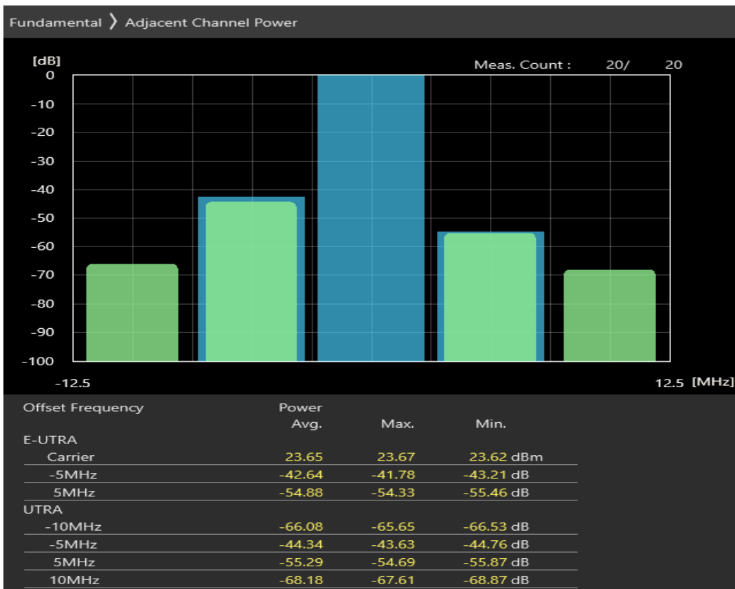
Band3 QPSK BW=5MHz Channel=19575 RB Size=8 Position=#Max
