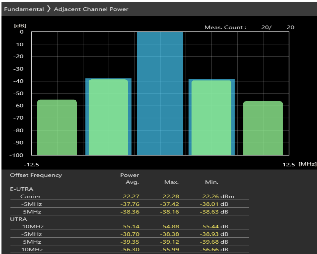
Band7 16QAM BW=5MHz Channel=21425 RB Size=8 Position=#0
