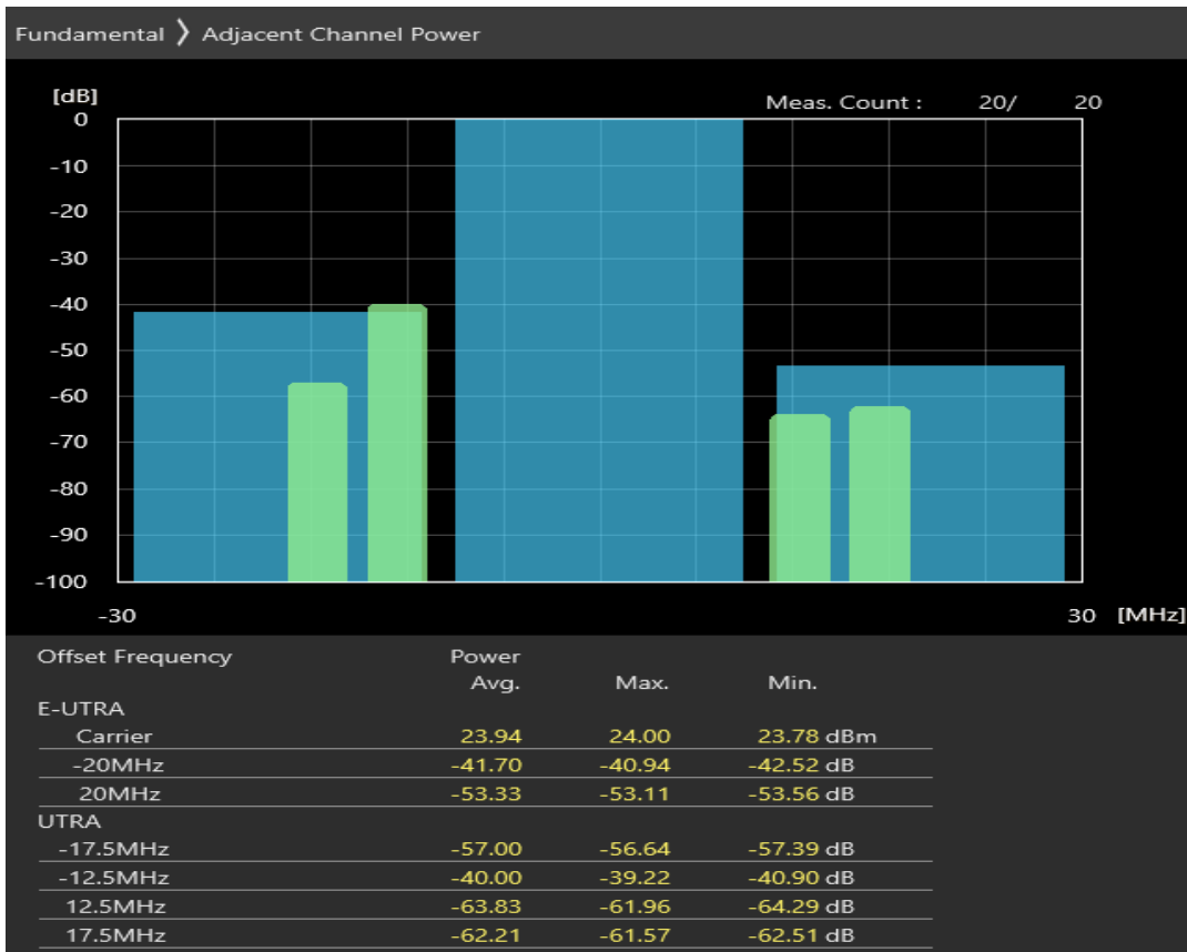
Band7 QPSK BW=20MHz Channel=21350 RB Size=18 Position=#Max
