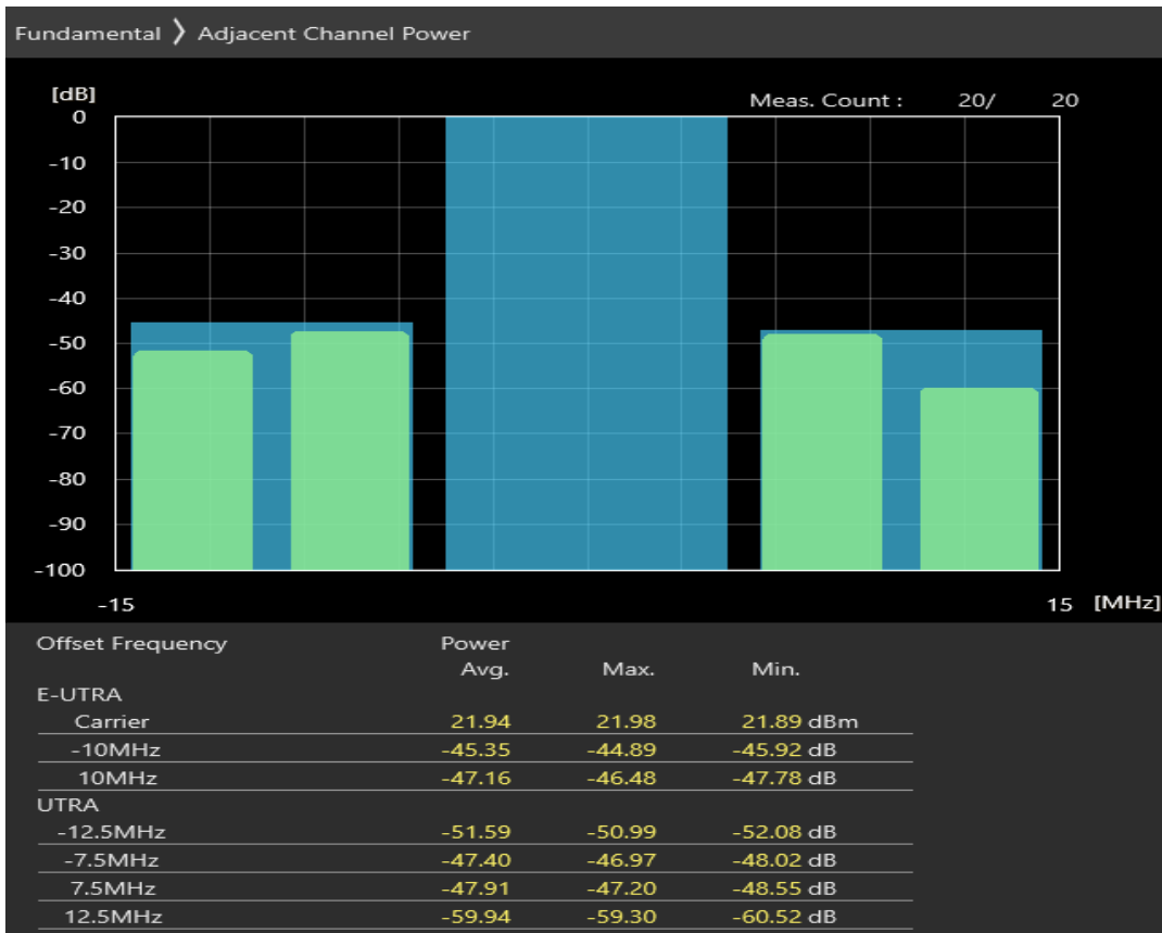
Band3 QPSK BW=20MHz Channel=19300 RB Size=18 Position=#0
