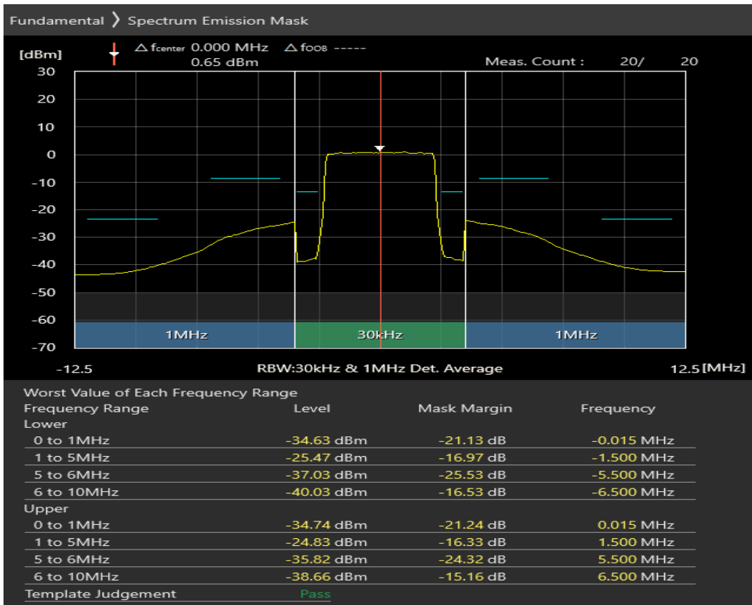
Band3 QPSK BW=5MHz Channel=19575 RB Size=8 Position=#0
