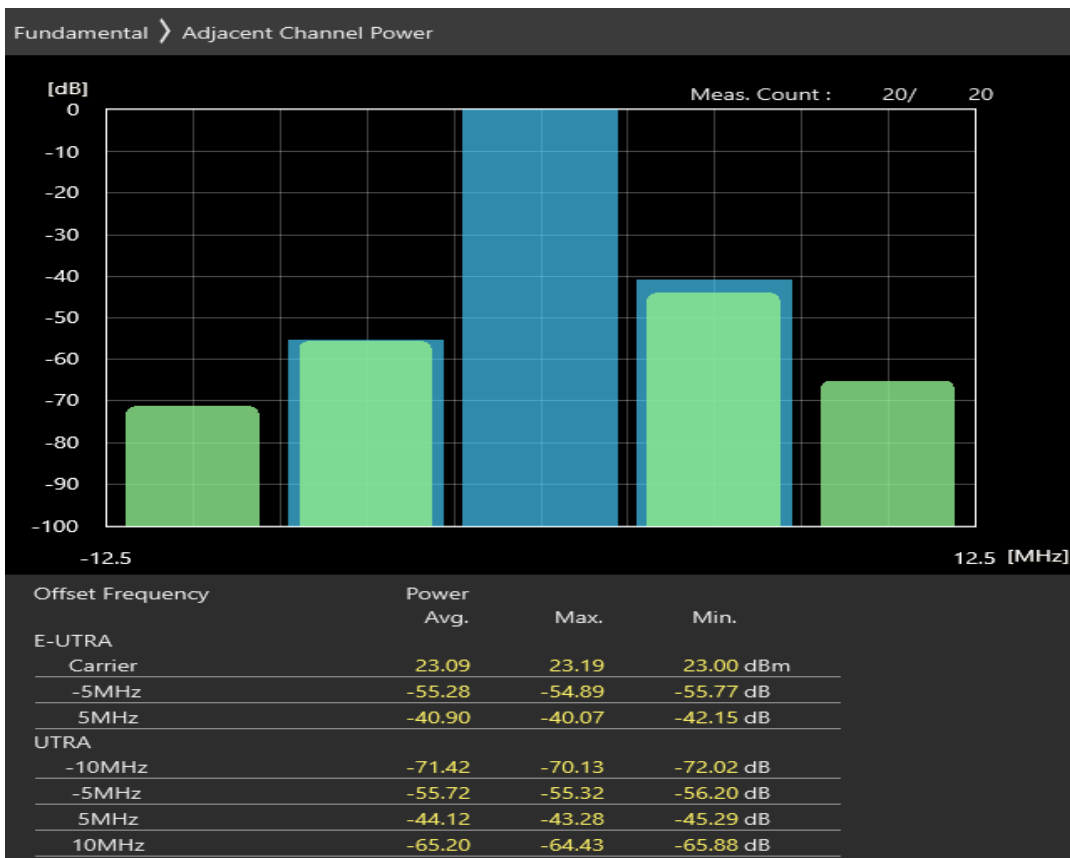
Band8 16QAM BW=5MHz Channel=21625 RB Size=25 Position=#0
