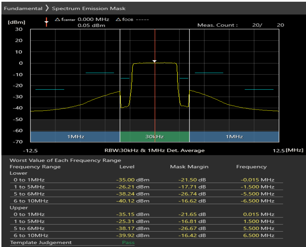
Band8 QPSK BW=5MHz Channel=21775 RB Size=8 Position=#0
