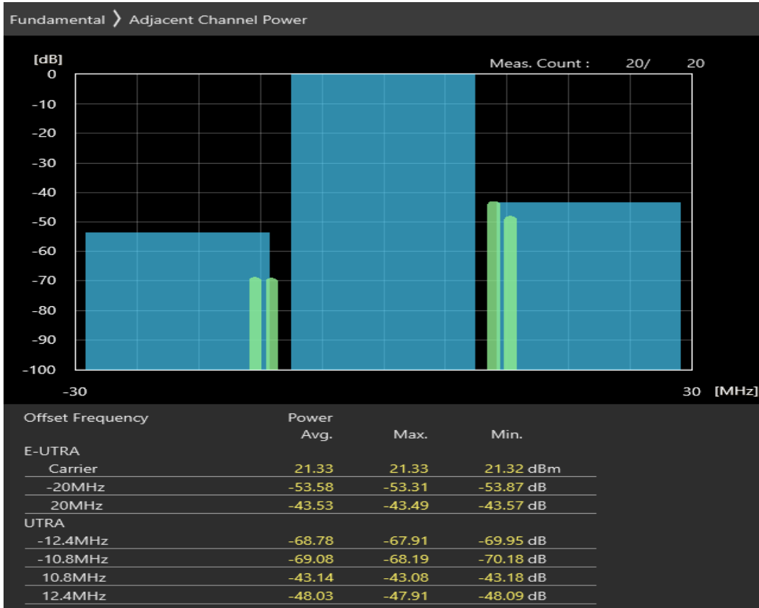
Band40 16QAM BW=20MHz Channel=38750 RB Size=100 Position=#0
