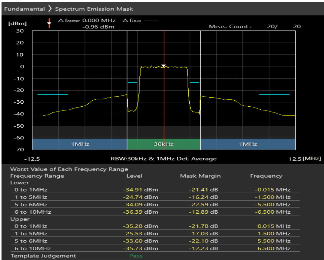
Band40 16QAM BW=5MHz Channel=38675 RB Size=8 Position=#0
