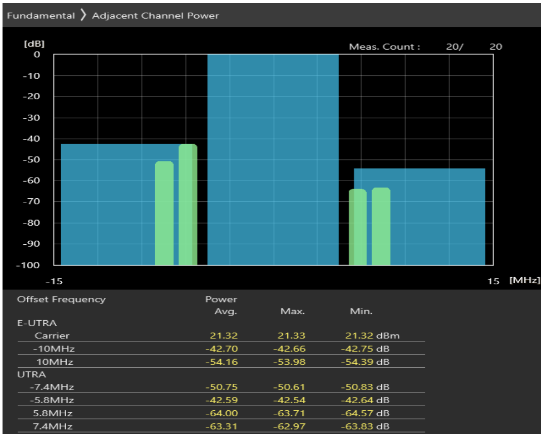
Band40 16QAM BW=10MHz Channel=39600 RB Size=12 Position=#Max
