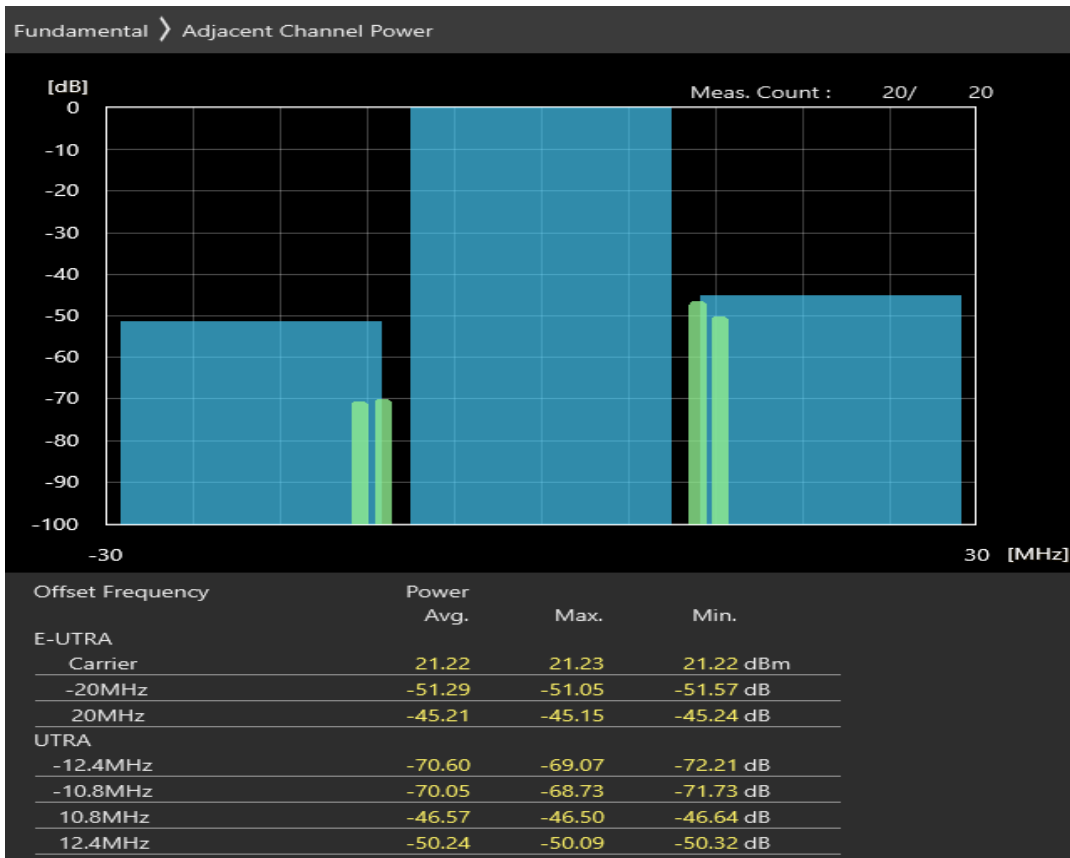
Band40 QAM16 BW=5MHz Channel=38675 RB Size=25 Position=#0
