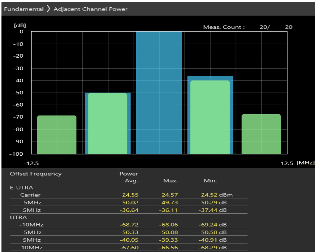
Band3 QPSK BW=5MHz Channel=19925 RB Size=25 Position=#0
