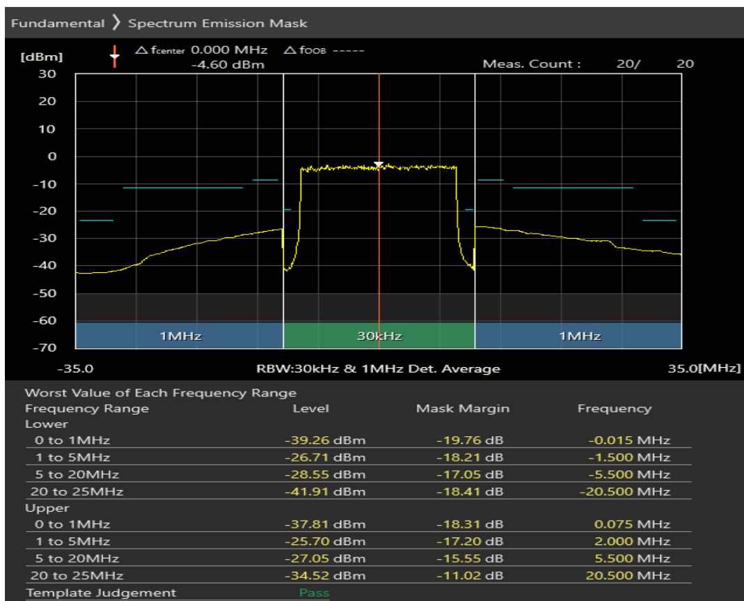
Band40 QAM16 BW=20MHz Channel=38750 RB Size=18 Position=#0
