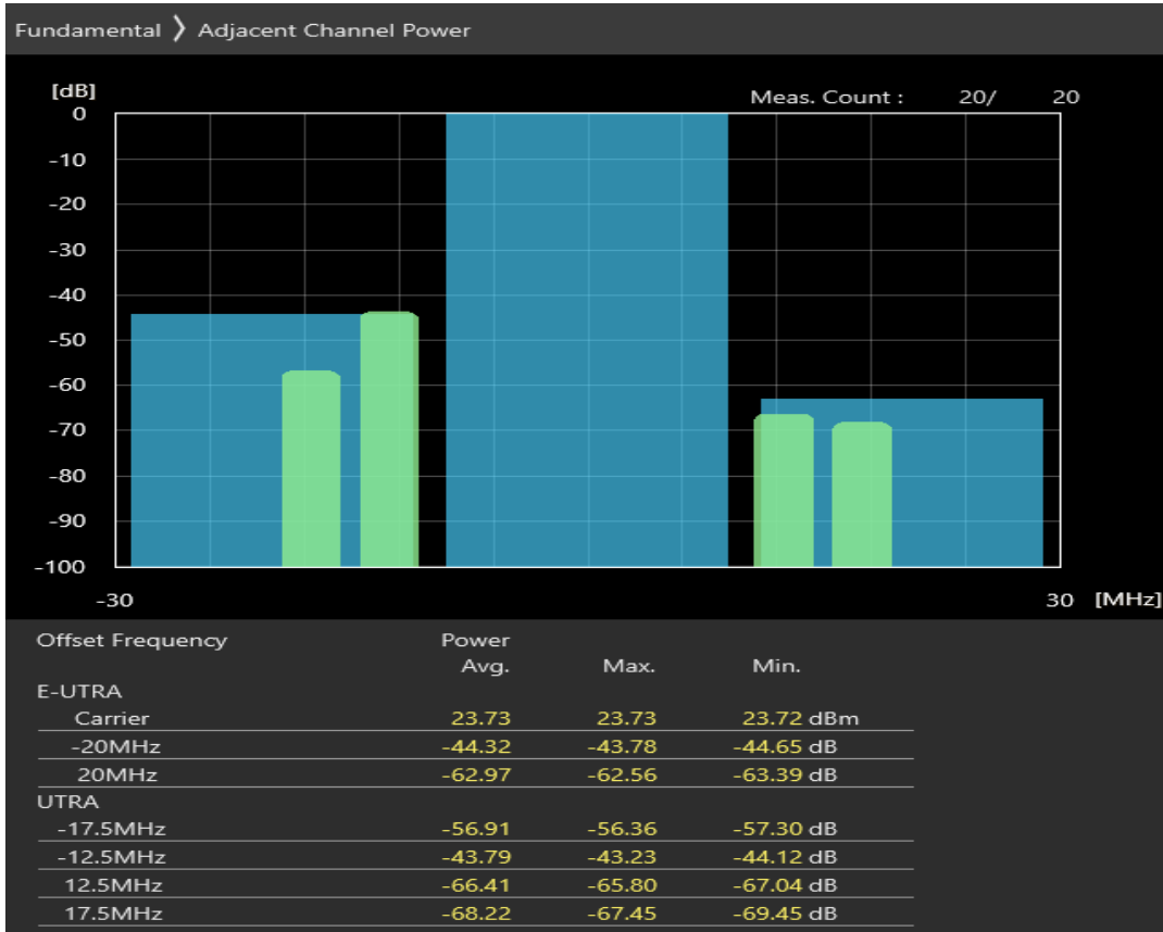
Band20 QPSK BW=20MHz Channel=24350 RB Size=18 Position=#Max
