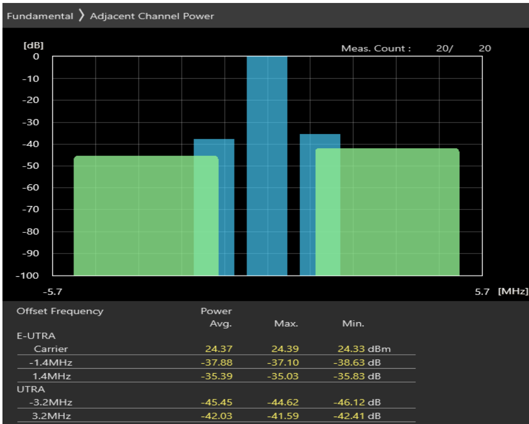
Band3 QPSK BW=1.4MHz Channel=19575 RB Size=6 Position=#0
