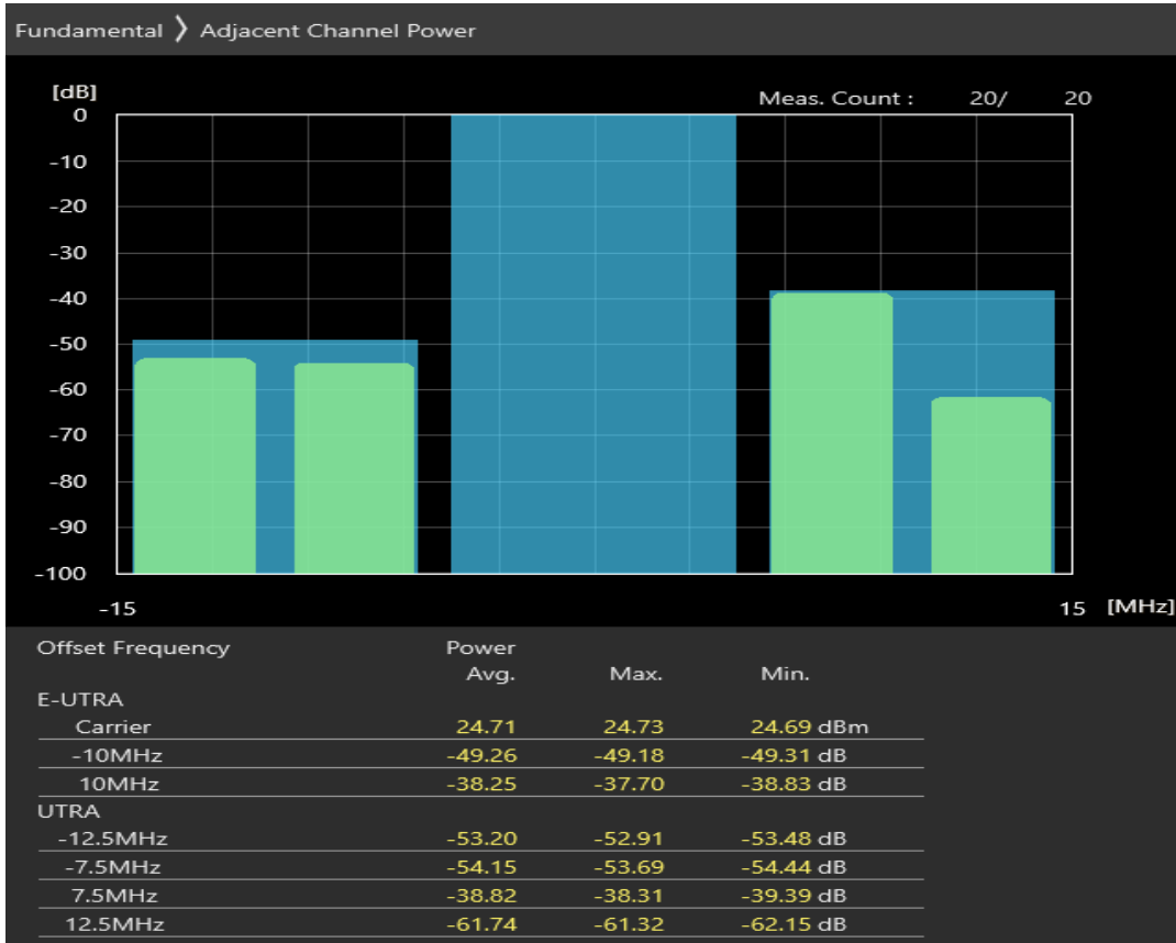
Band8 QPSK BW=10MHz Channel=21625 RB Size=50 Position=#0
