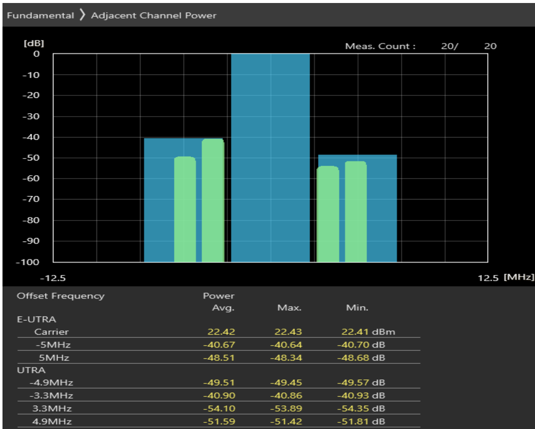
Band40 QAM16 BW=5MHz Channel=39625 RB Size=8 Position=#Max
