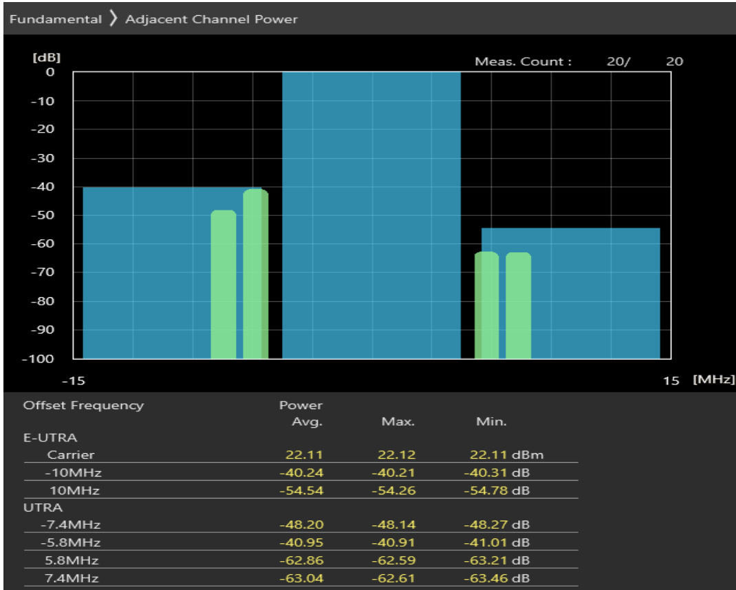
Band40 QPSK BW=10MHz Channel=38700 RB Size=12 Position=#Max
