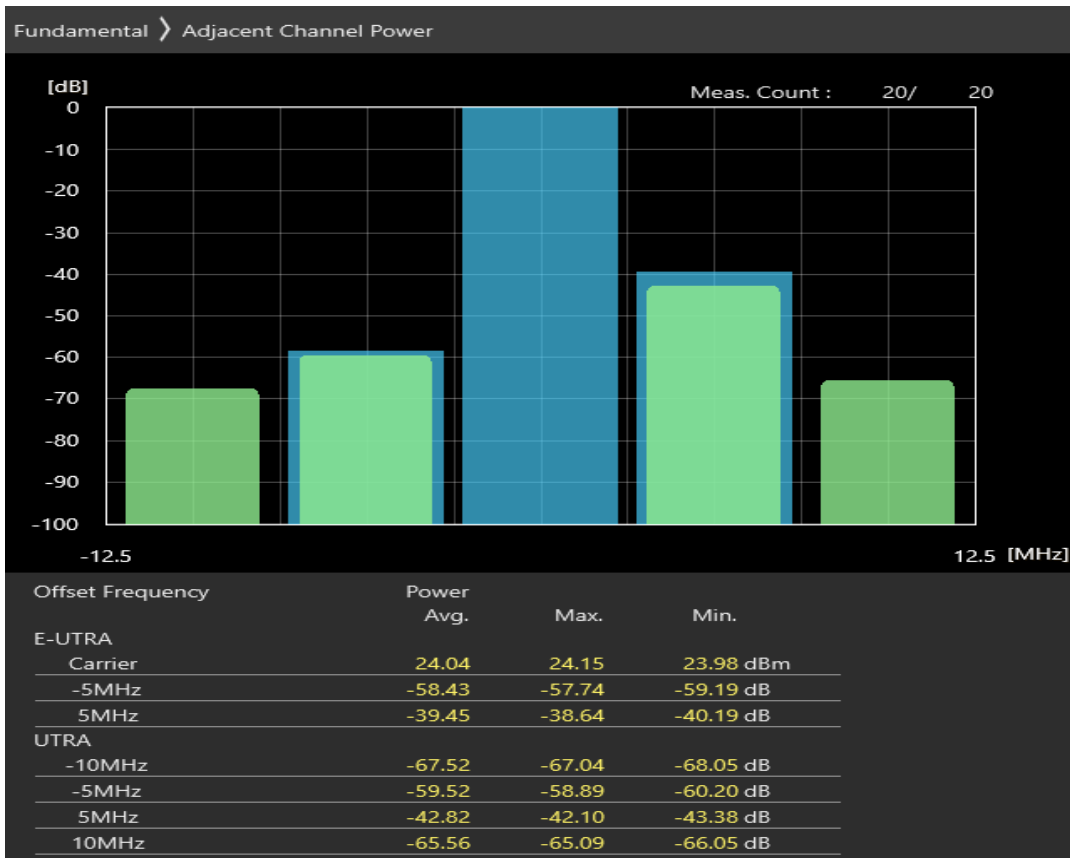
Band7 16QAM BW=5MHz Channel=21100 RB Size=25 Position=#0
