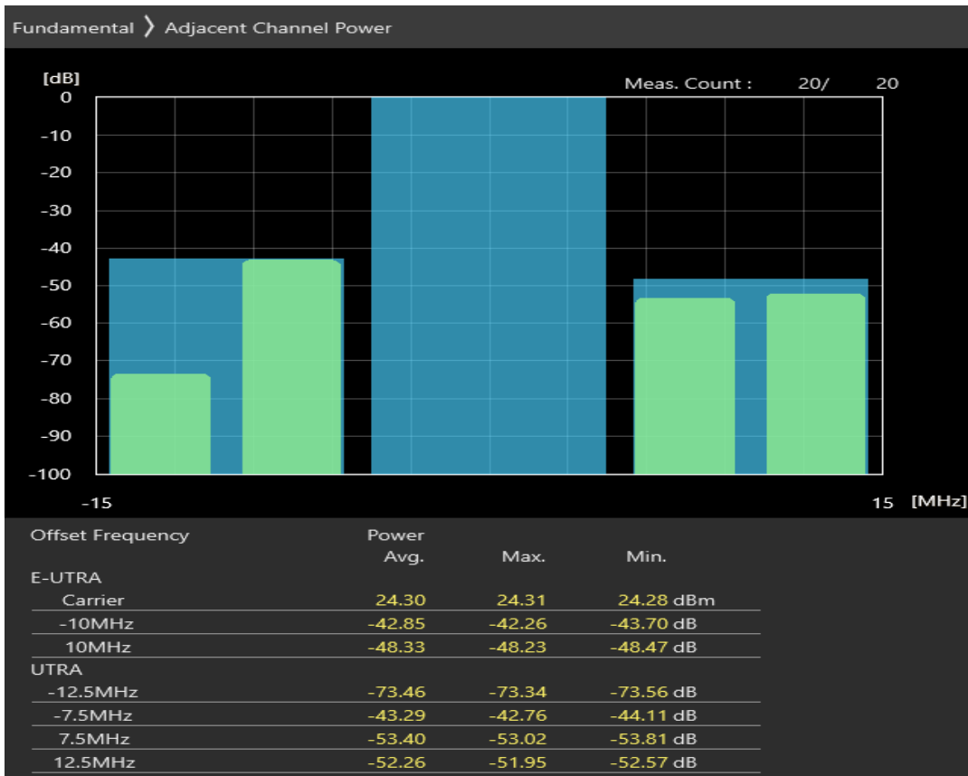
Band8 QPSK BW=10MHz Channel=21500 RB Size=12 Position=#Max
