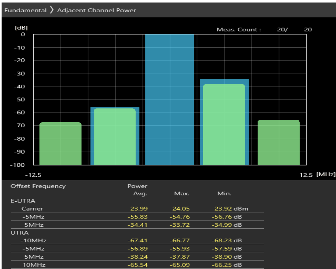
Band7 16QAM BW=5MHz Channel=21425 RB Size=25 Position=#0
