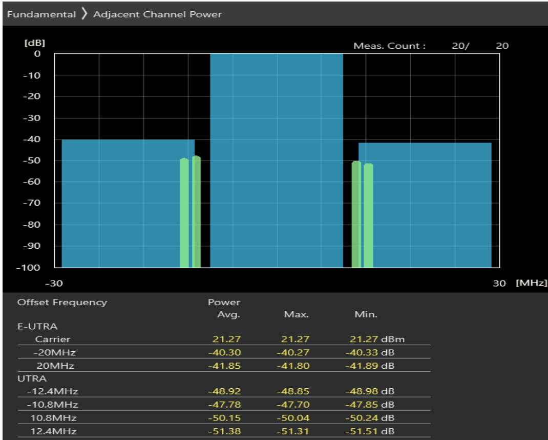
Band40 16QAM BW=20MHz Channel=39150 RB Size=18 Position=#0
