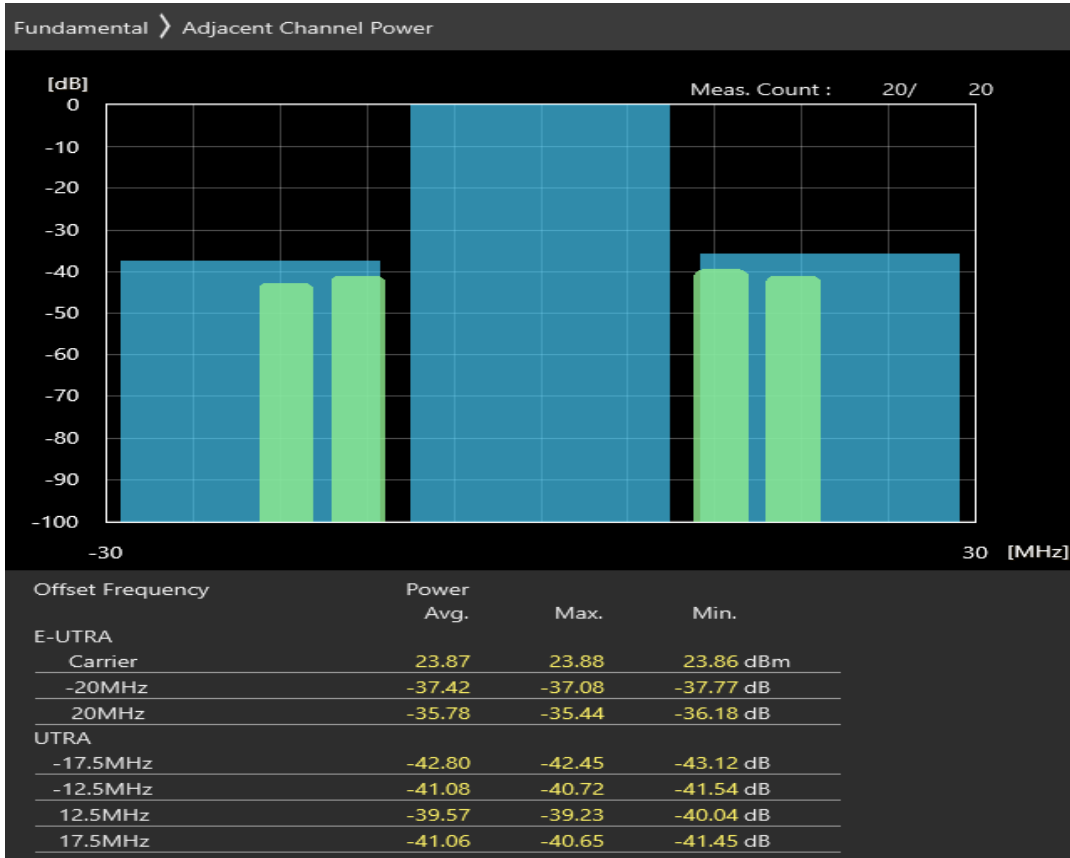
Band1 16QAM BW=20MHz Channel=18300 RB Size=18 Position=#0
