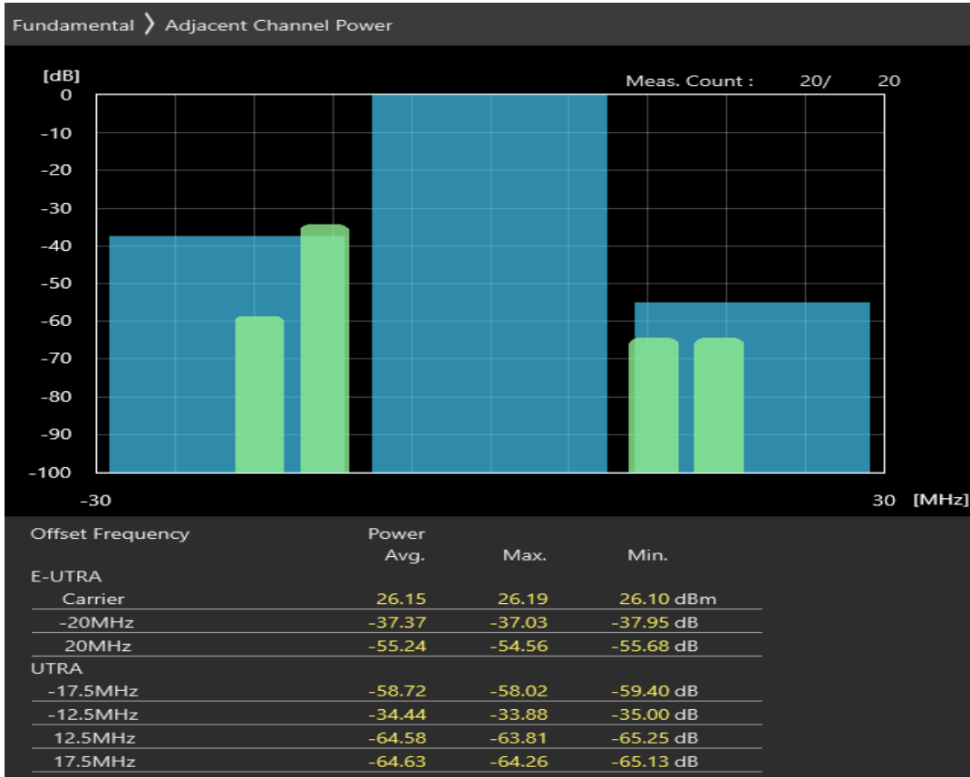
Band1 QPSK BW=20MHz Channel=18100 RB Size=18 Position=#Max
