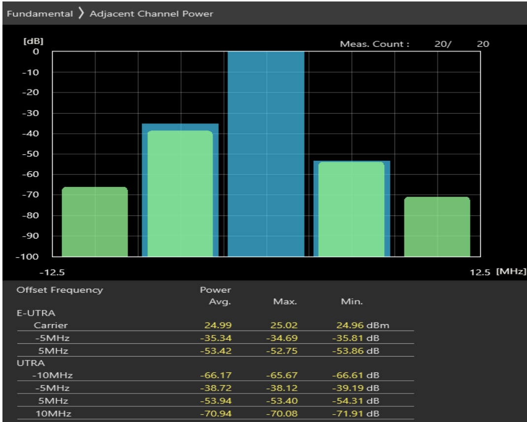
Band1 QPSK BW=5MHz Channel=18025 RB Size=8 Position=#Max
