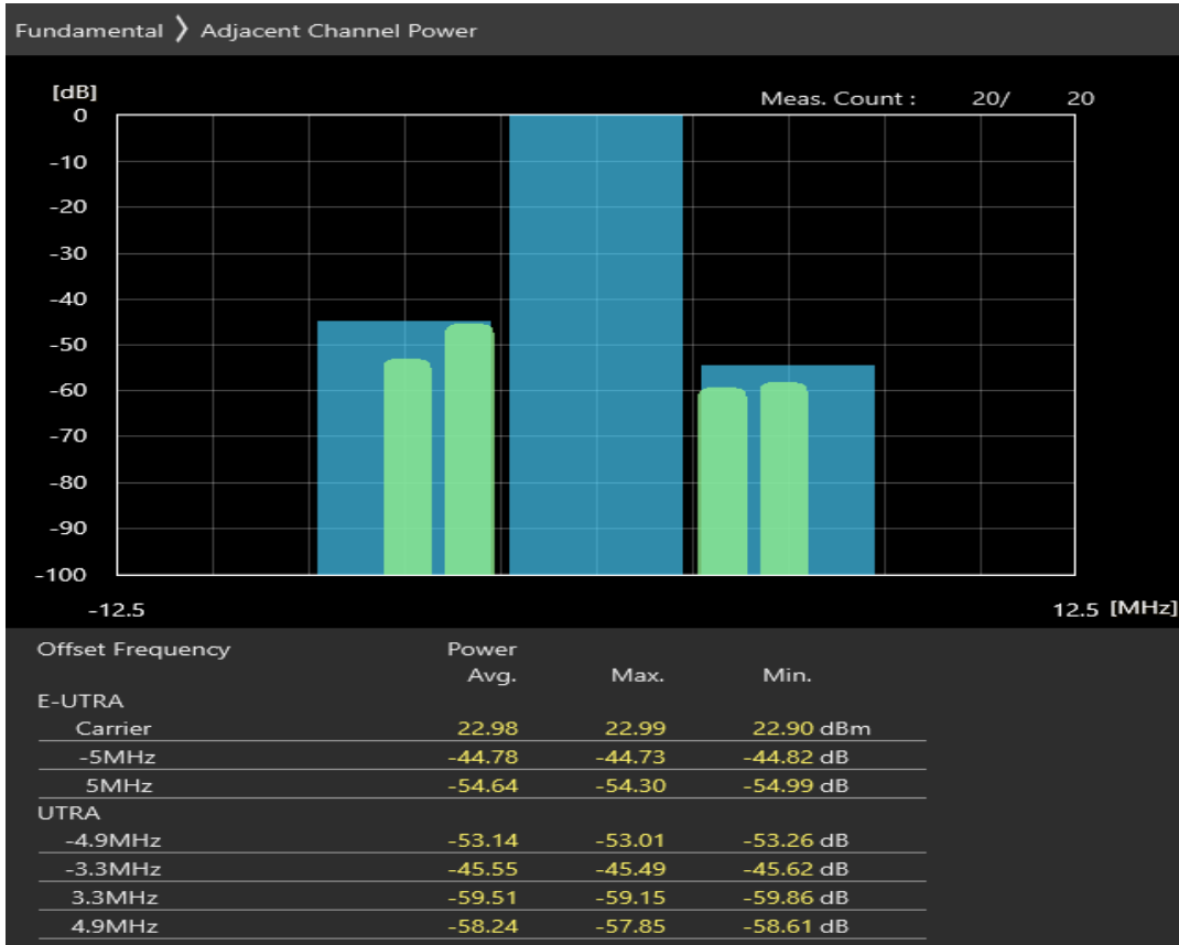
Band40 QAM16 BW=5MHz Channel=39150 RB Size=8 Position=#Max
