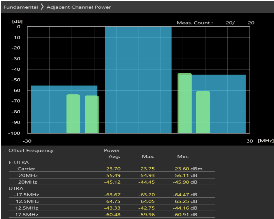
Band3 16QAM BW=20MHz Channel=19575 RB Size=100 Position=#0
