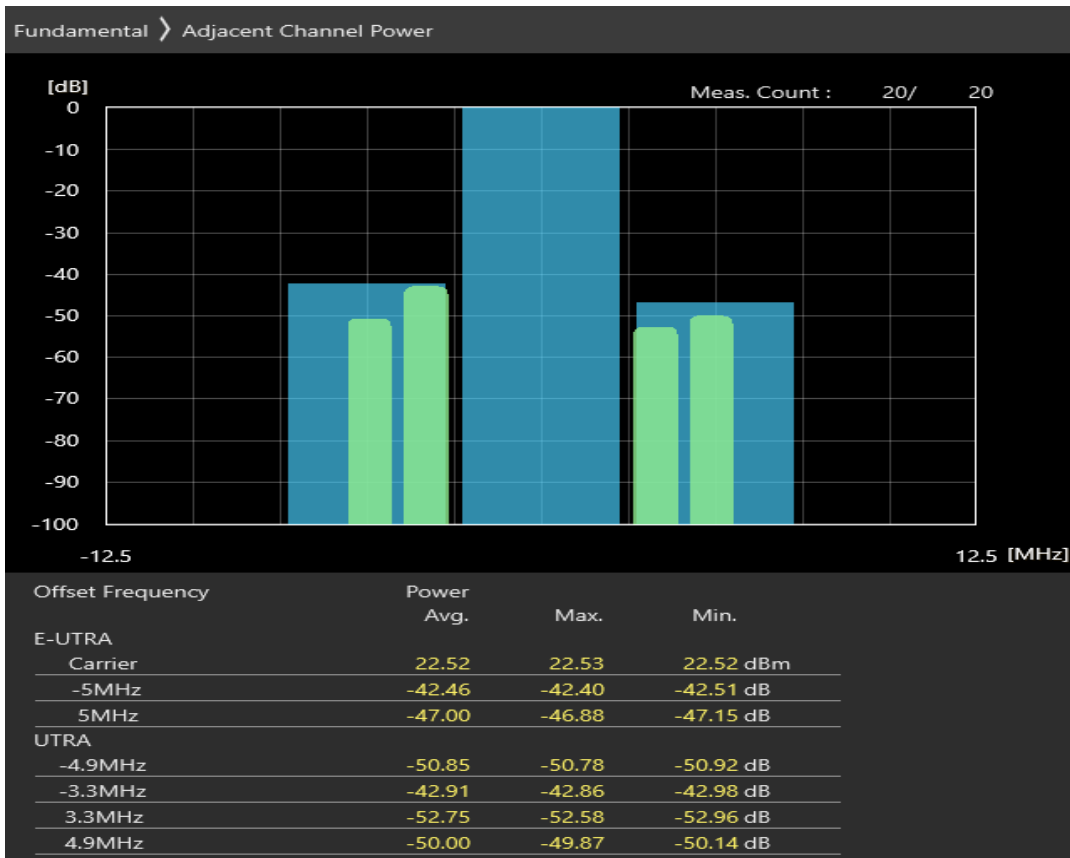
Band40 QAM16 BW=5MHz Channel=38675 RB Size=8 Position=#Max
