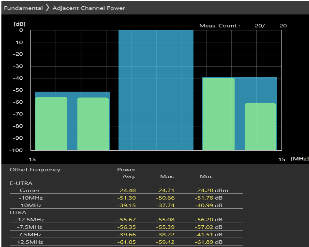
Band1 16QAM BW=10MHz Channel=18550 RB Size=50 Position=#0
