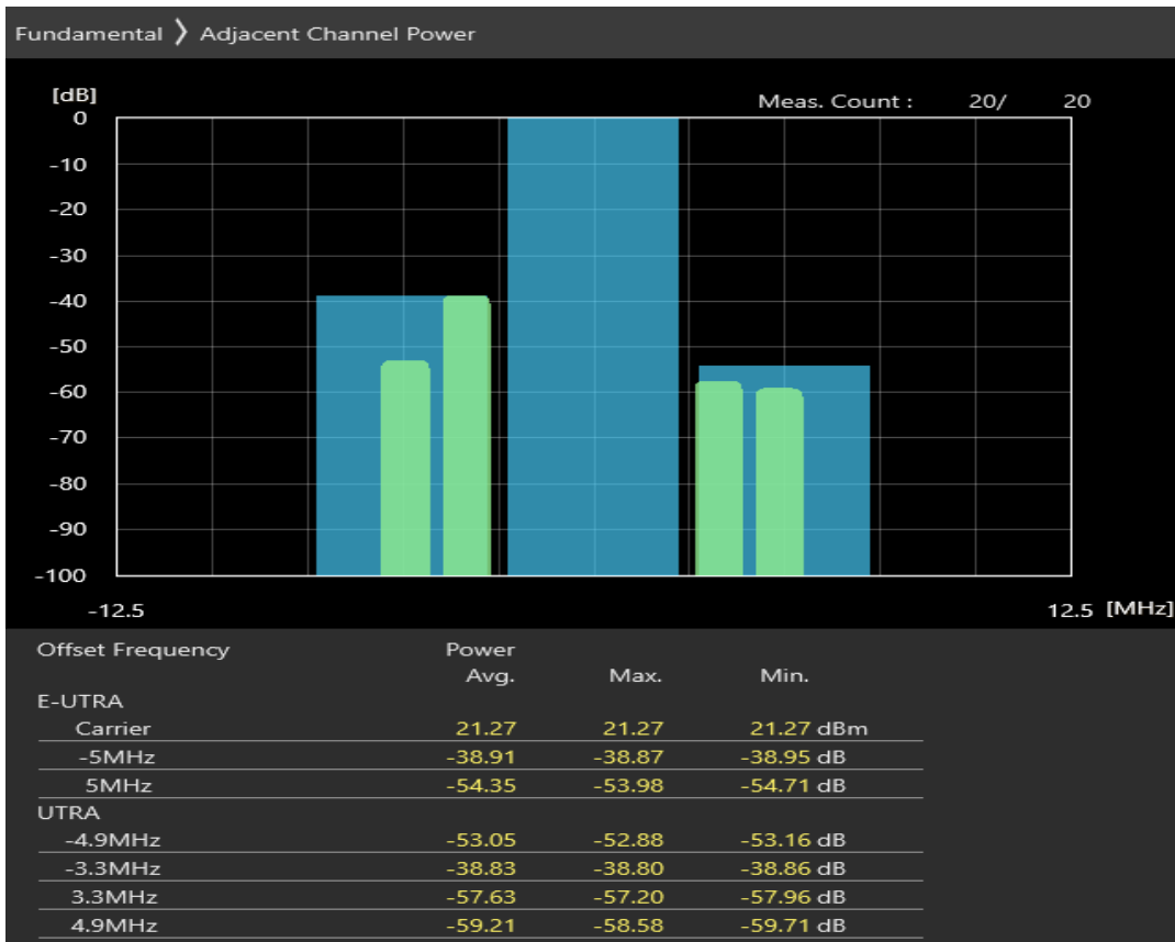
Band40 16QAM BW=5MHz Channel=38675 RB Size=8 Position=#Max
