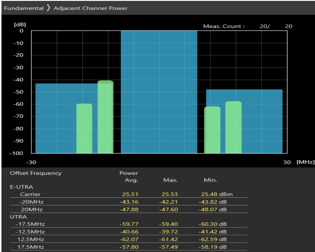
Band1 QPSK BW=20MHz Channel=18300 RB Size=18 Position=#Max
