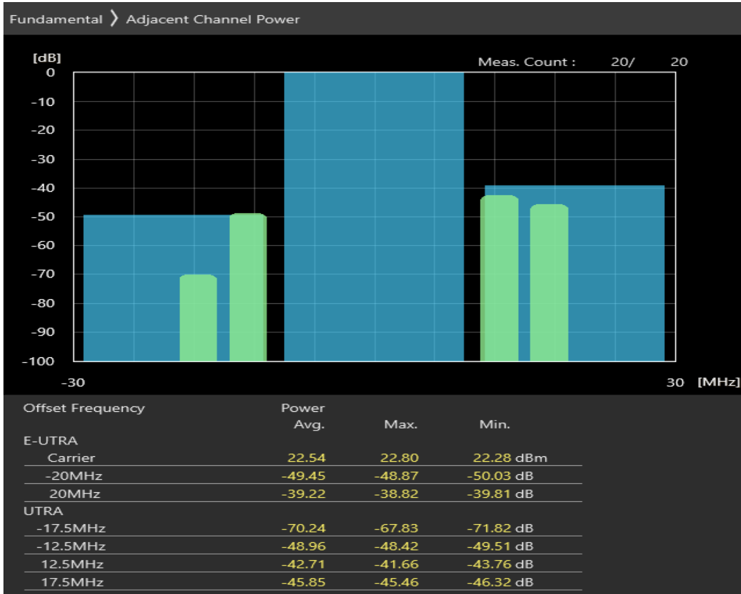
Band20 16QAM BW=20MHz Channel=24250 RB Size=18 Position=#0
