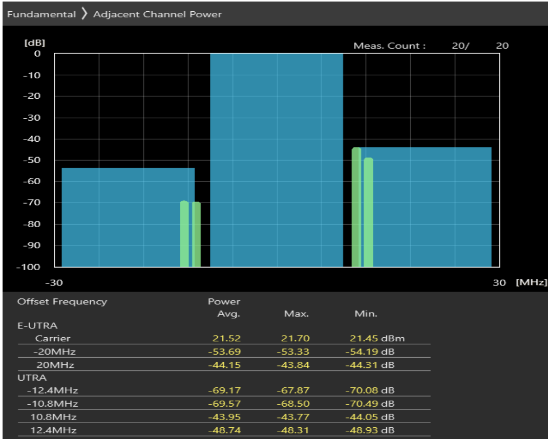
Band40 16QAM BW=20MHz Channel=39150 RB Size=100 Position=#0
