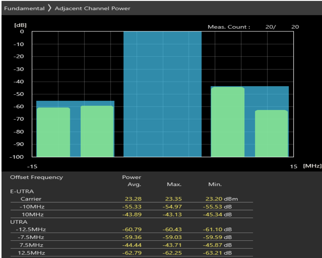
Band3 16QAM BW=10MHz Channel=19250 RB Size=50 Position=#0
