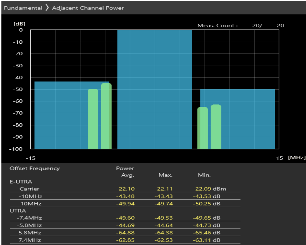
Band40 QAM16 BW=10MHz Channel=38700 RB Size=12 Position=#Max
