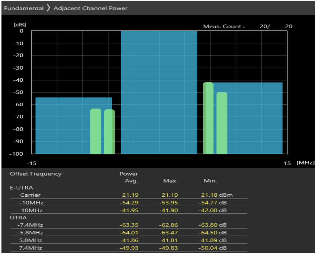
Band40 16QAM BW=10MHz Channel=38700 RB Size=50 Position=#0
