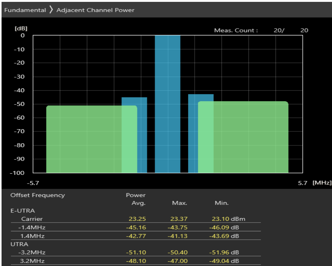
Band8 16QAM BW=1.4MHz Channel=21457 RB Size=6 Position=#0
