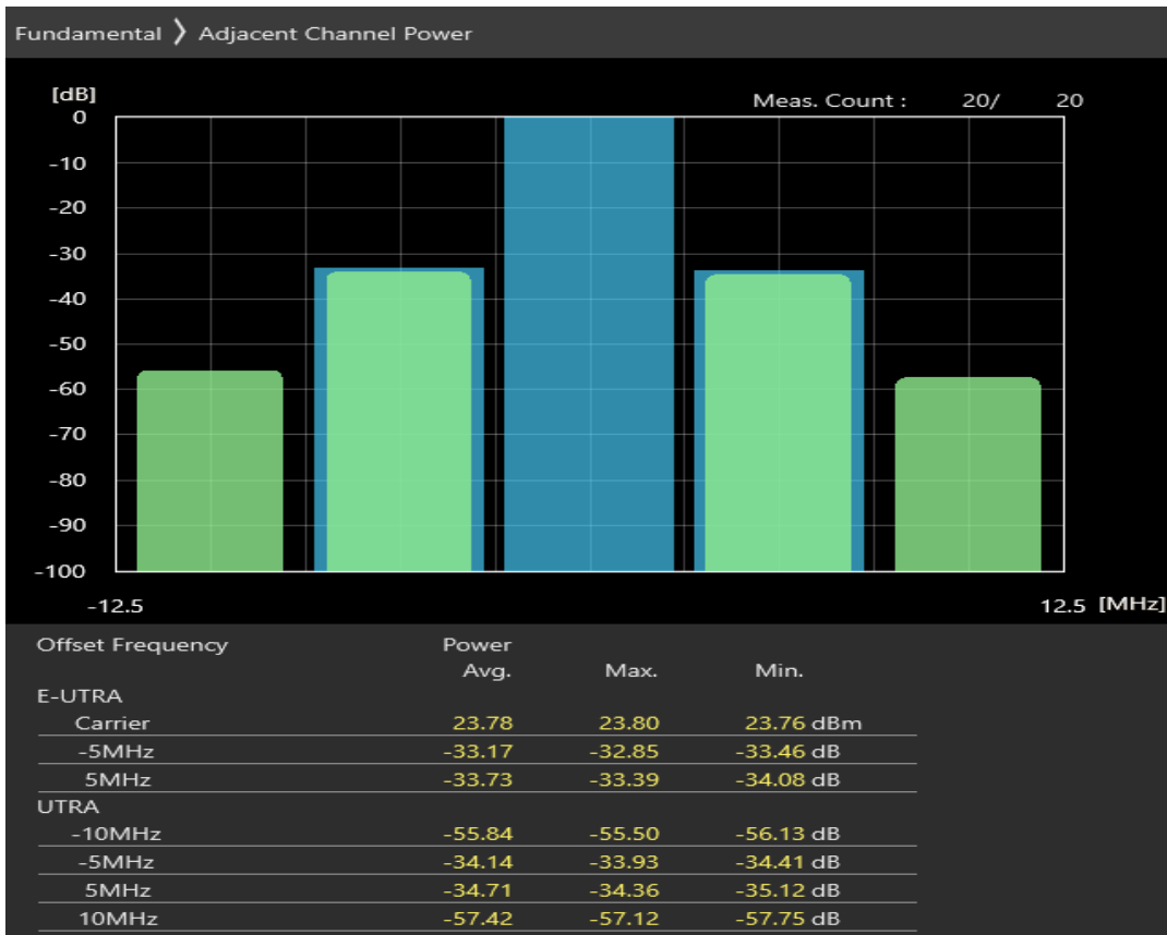
Band7 16QAM BW=5MHz Channel=21425 RB Size=8 Position=#0
