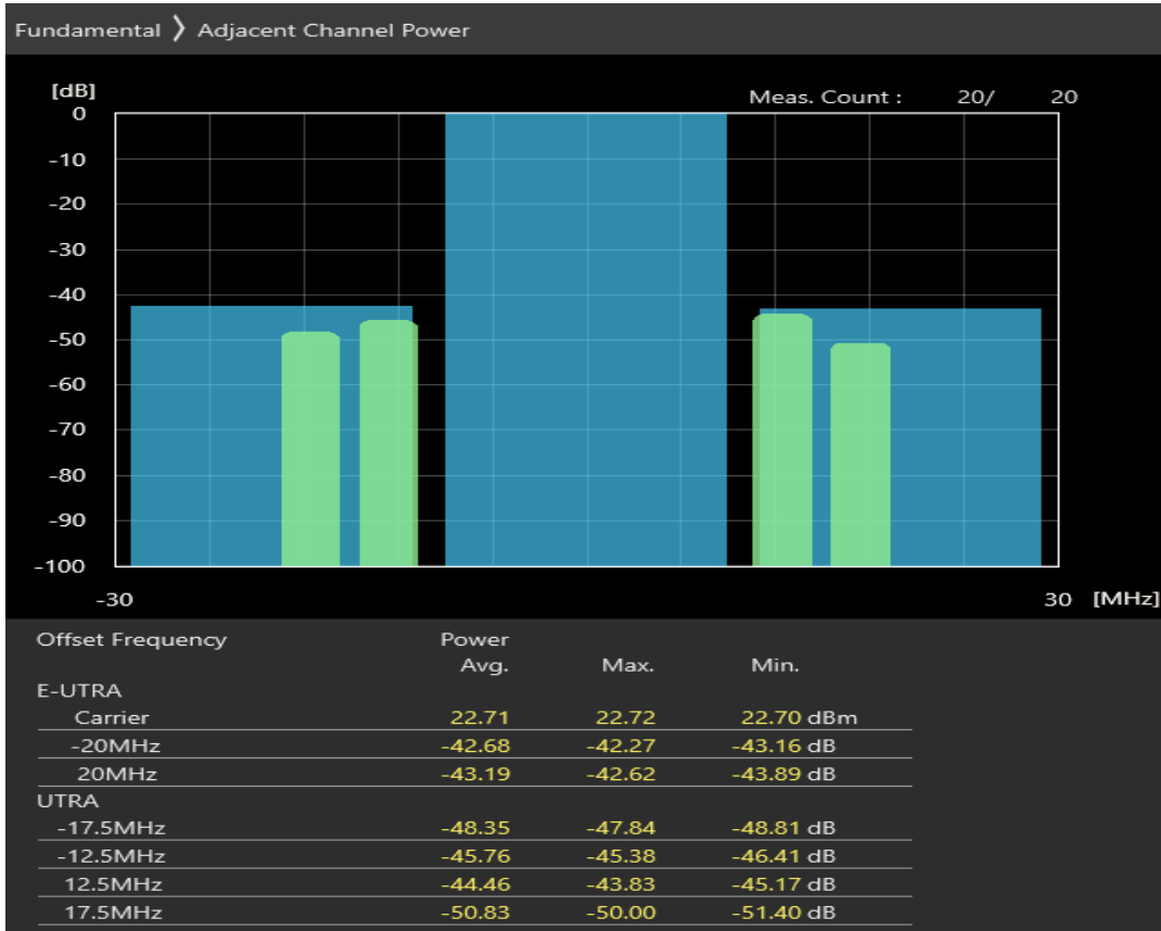
Band20 16QAM BW=20MHz Channel=24350 RB Size=18 Position=#0
