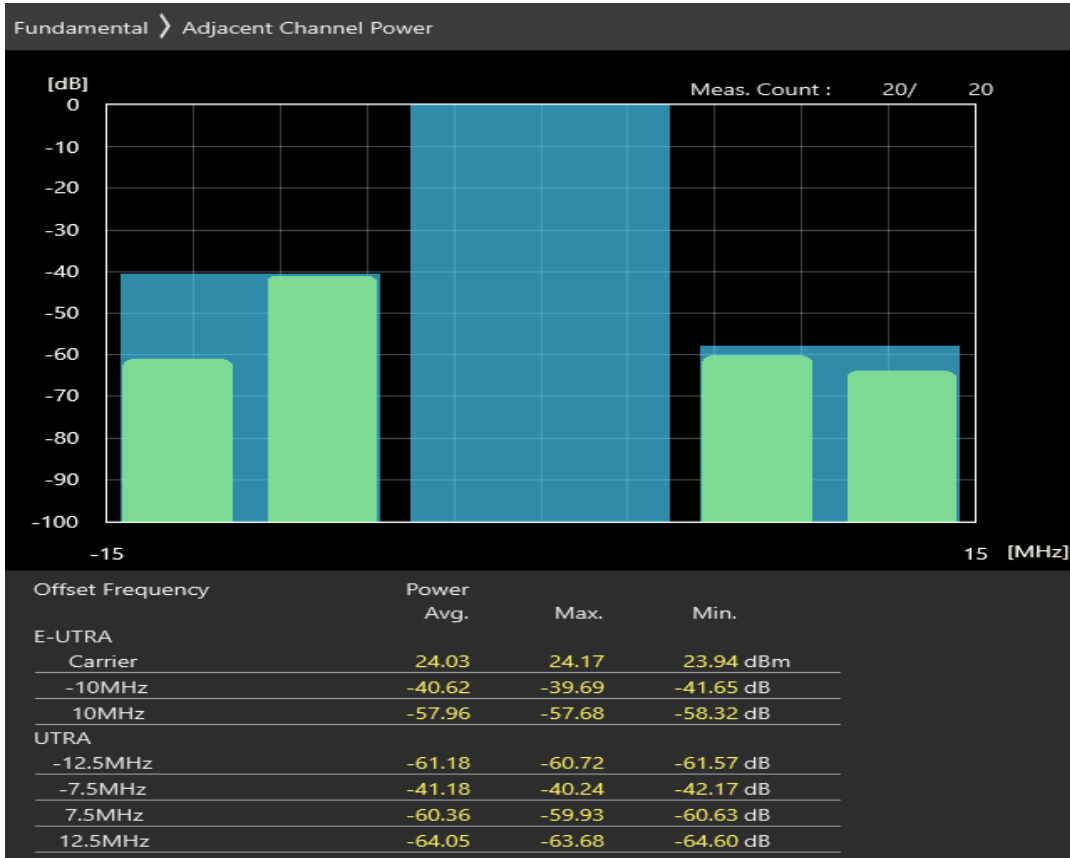
Band7 16QAM BW=10MHz Channel=21100 RB Size=12 Position=#Max
