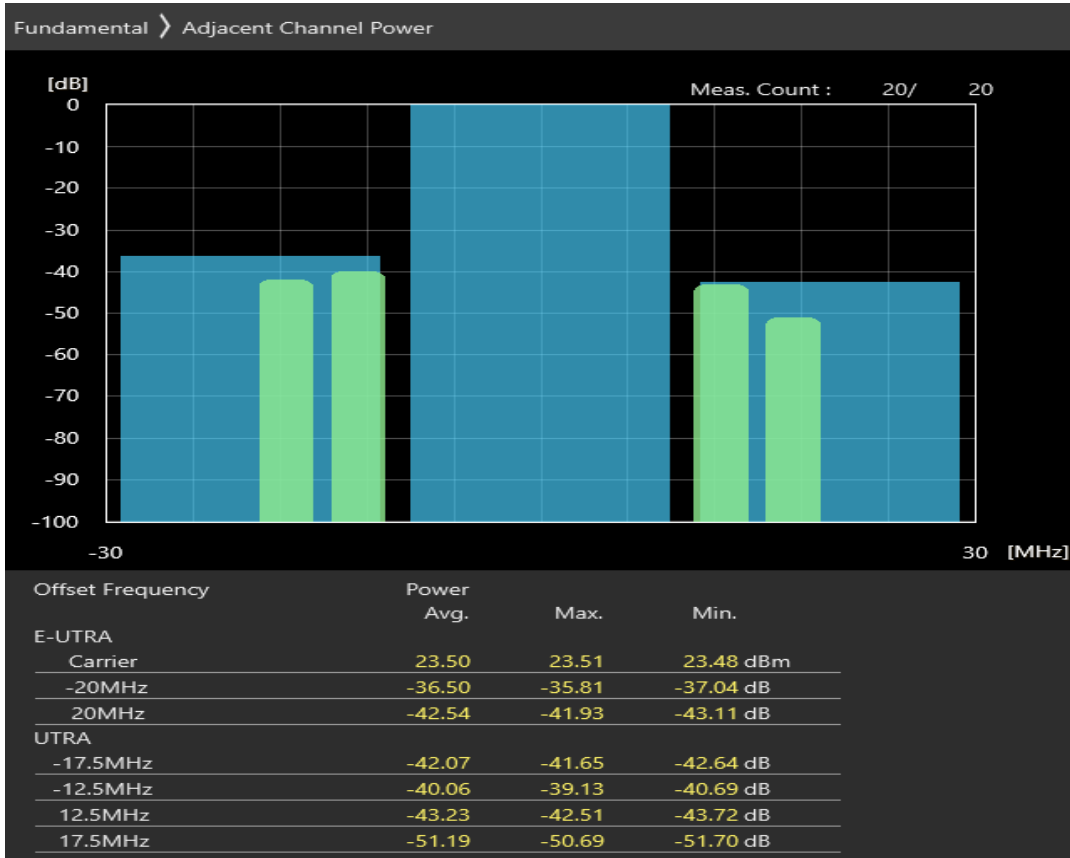
Band3 16QAM BW=20MHz Channel=19850 RB Size=18 Position=#0
