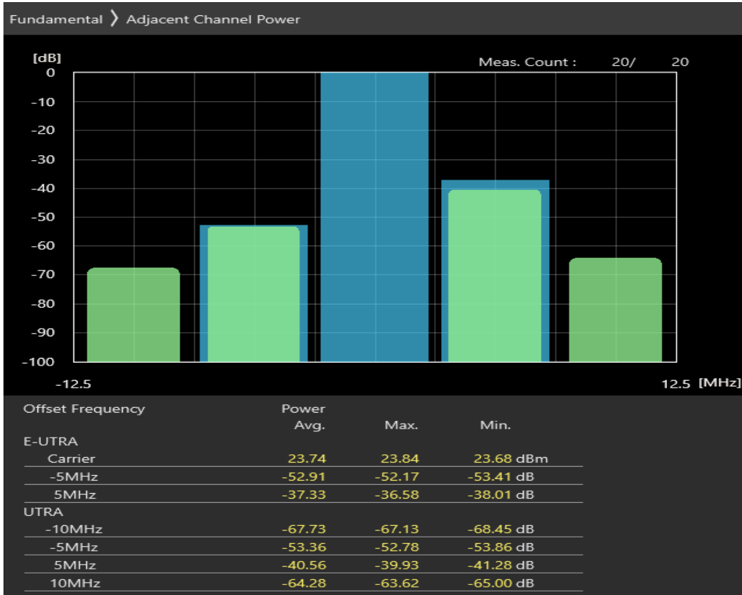
Band3 16QAM BW=5MHz Channel=19575 RB Size=25 Position=#0
