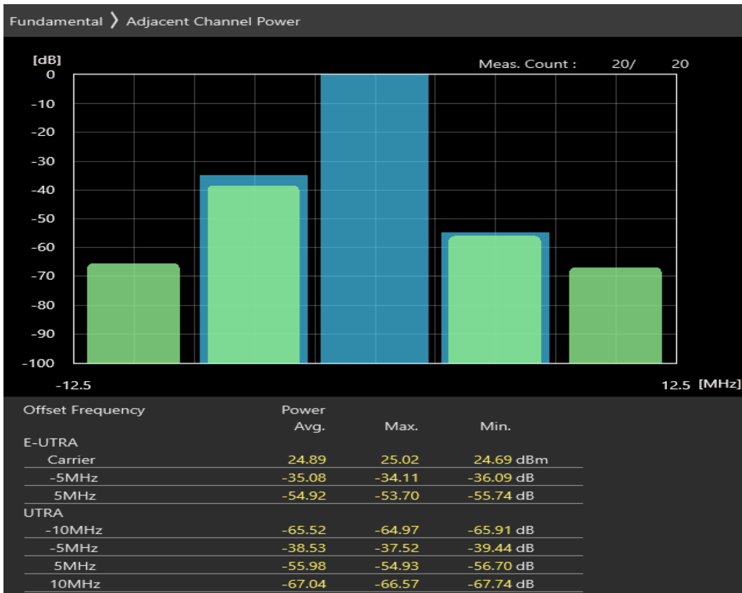
Band7 QPSK BW=5MHz Channel=20775 RB Size=8 Position=#Max
