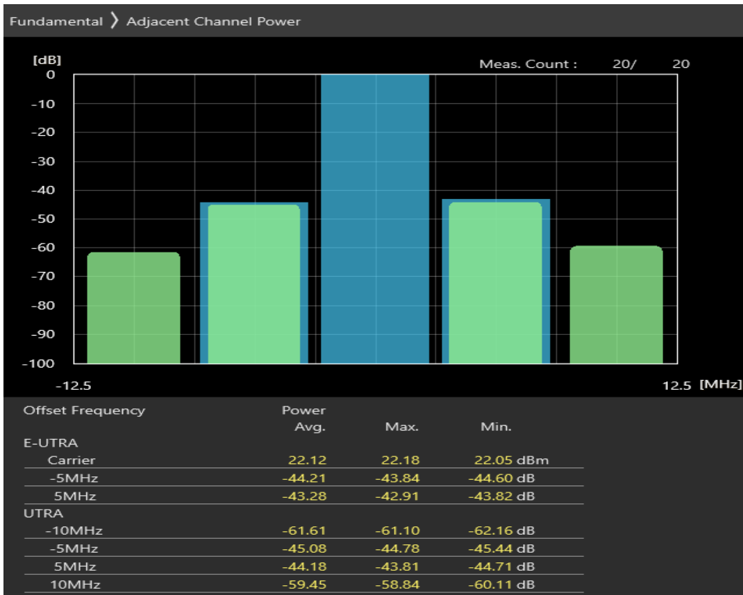
Band3 QPSK BW=5MHz Channel=19575 RB Size=8 Position=#0
