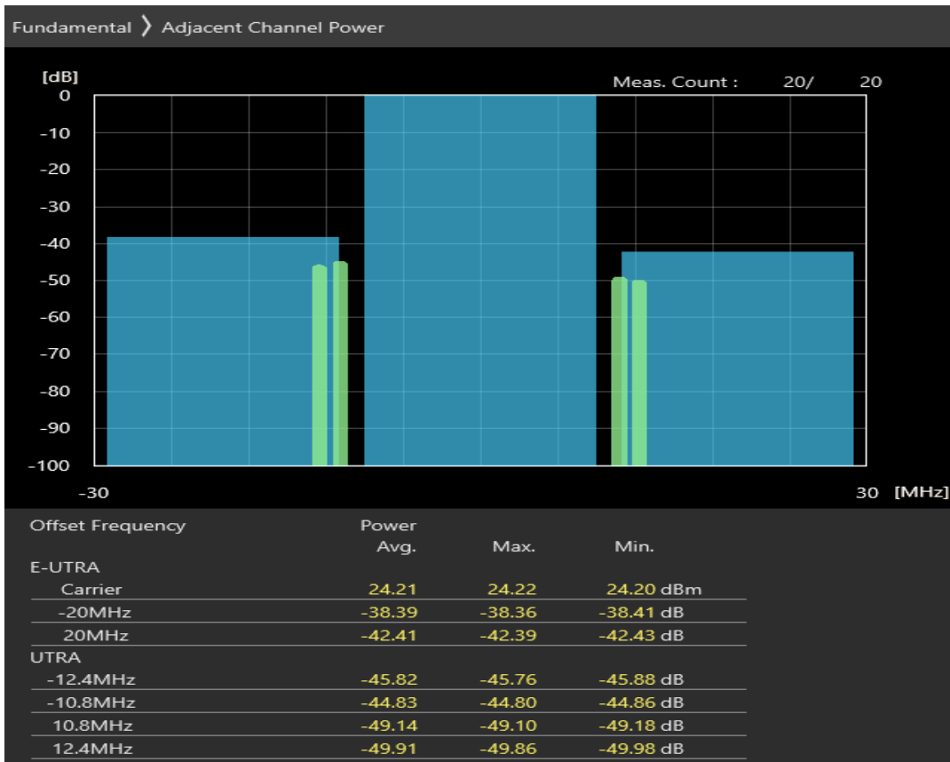
Band40 QAM16 BW=20MHz Channel=39550 RB Size=18 Position=#0
