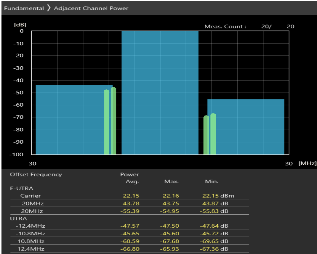
Band40 QPSK BW=20MHz Channel=39550 RB Size=18 Position=#Max
