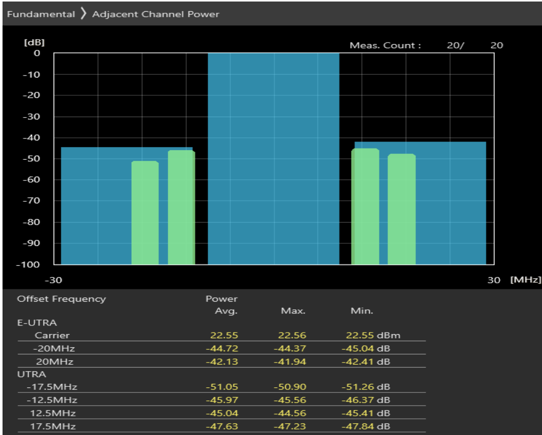
Band20 16QAM BW=20MHz Channel=24300 RB Size=18 Position=#0
