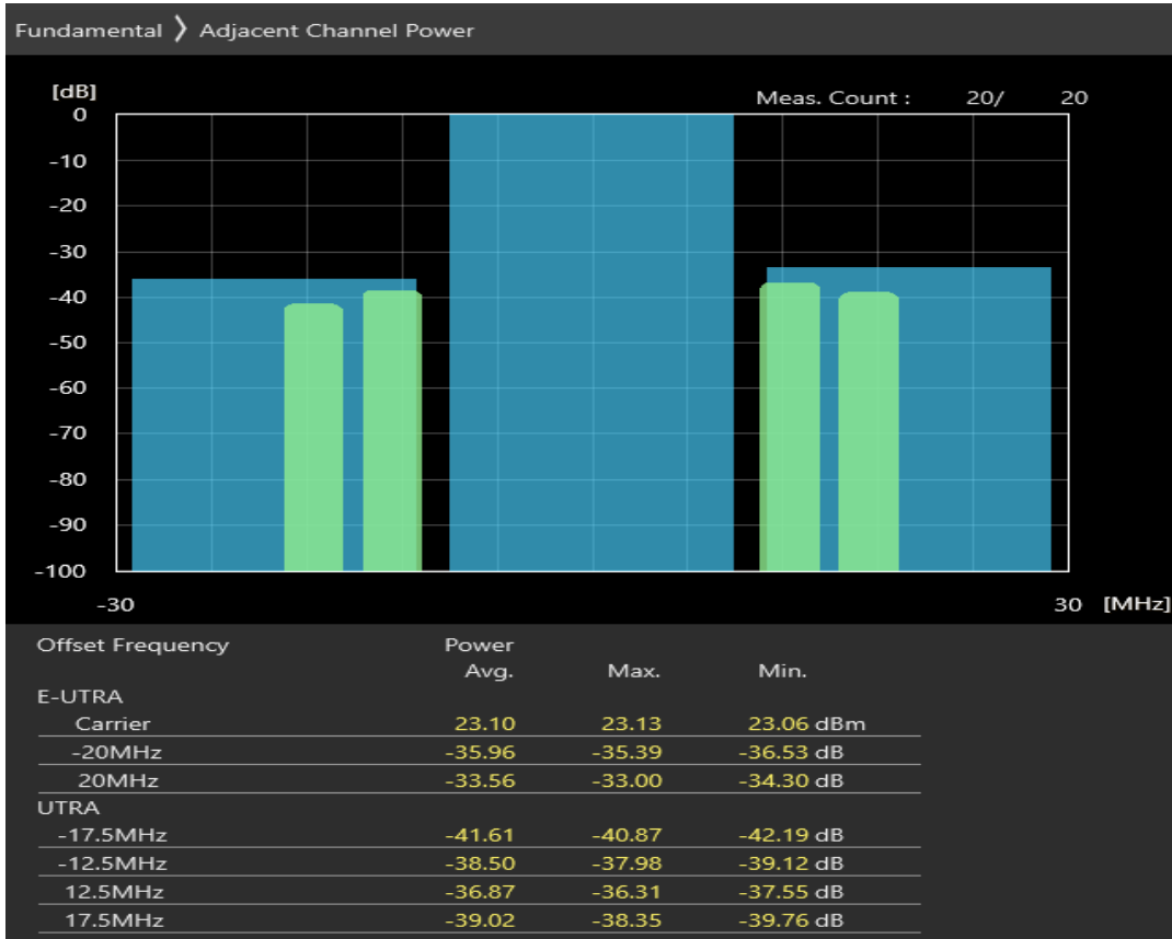
Band7 QPSK BW=20MHz Channel=21100 RB Size=18 Position=#0
