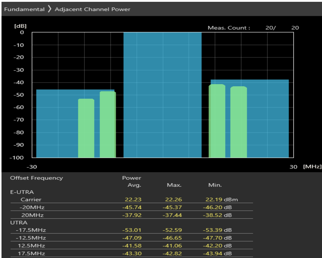
Band3 QPSK BW=20MHz Channel=19575 RB Size=18 Position=#0
