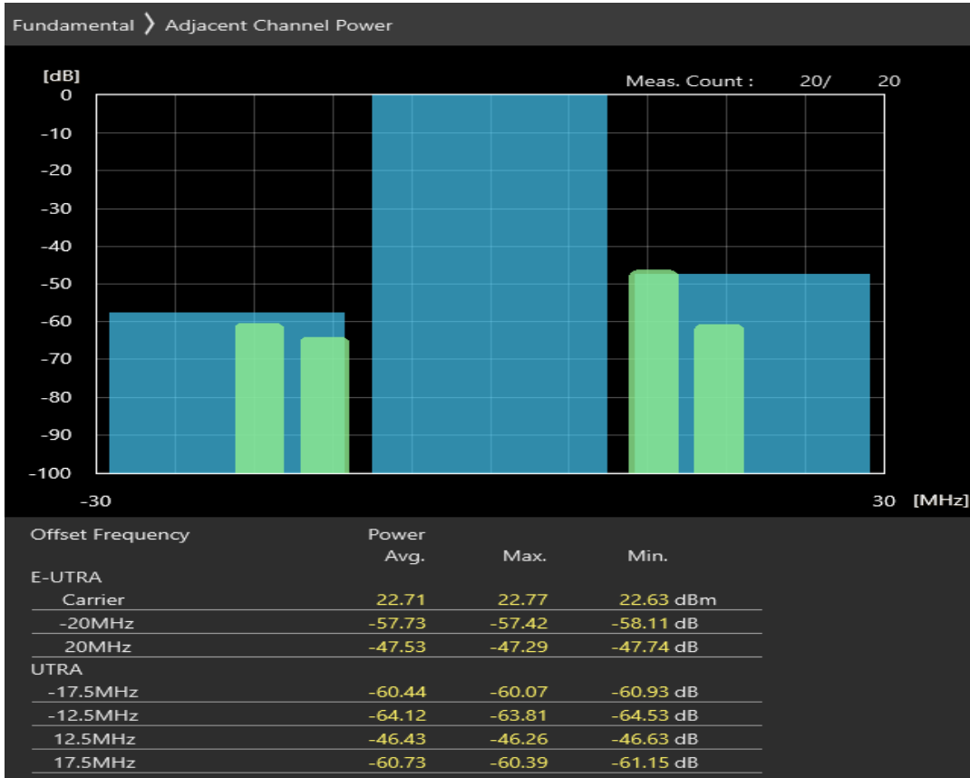
Band20 16QAM BW=20MHz Channel=24300 RB Size=100 Position=#0
