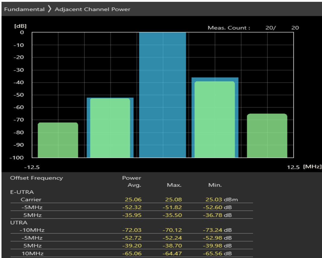
Band1 QPSK BW=5MHz Channel=18025 RB Size=25 Position=#0
