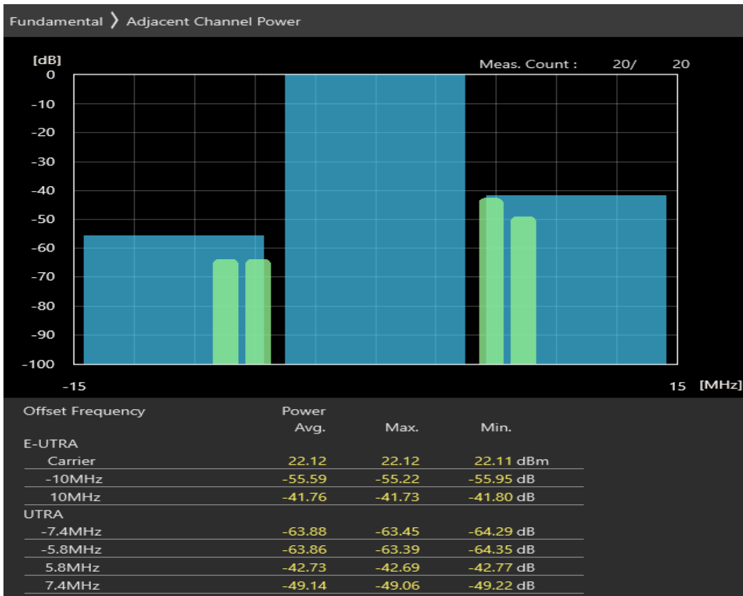
Band40 QPSK BW=10MHz Channel=39600 RB Size=50 Position=#0
