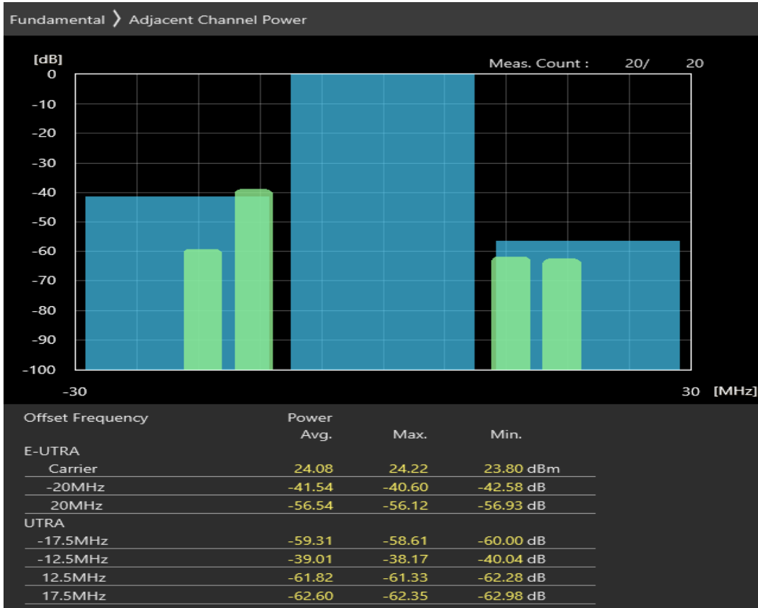
Band7 16QAM BW=20MHz Channel=20850 RB Size=18 Position=#Max
