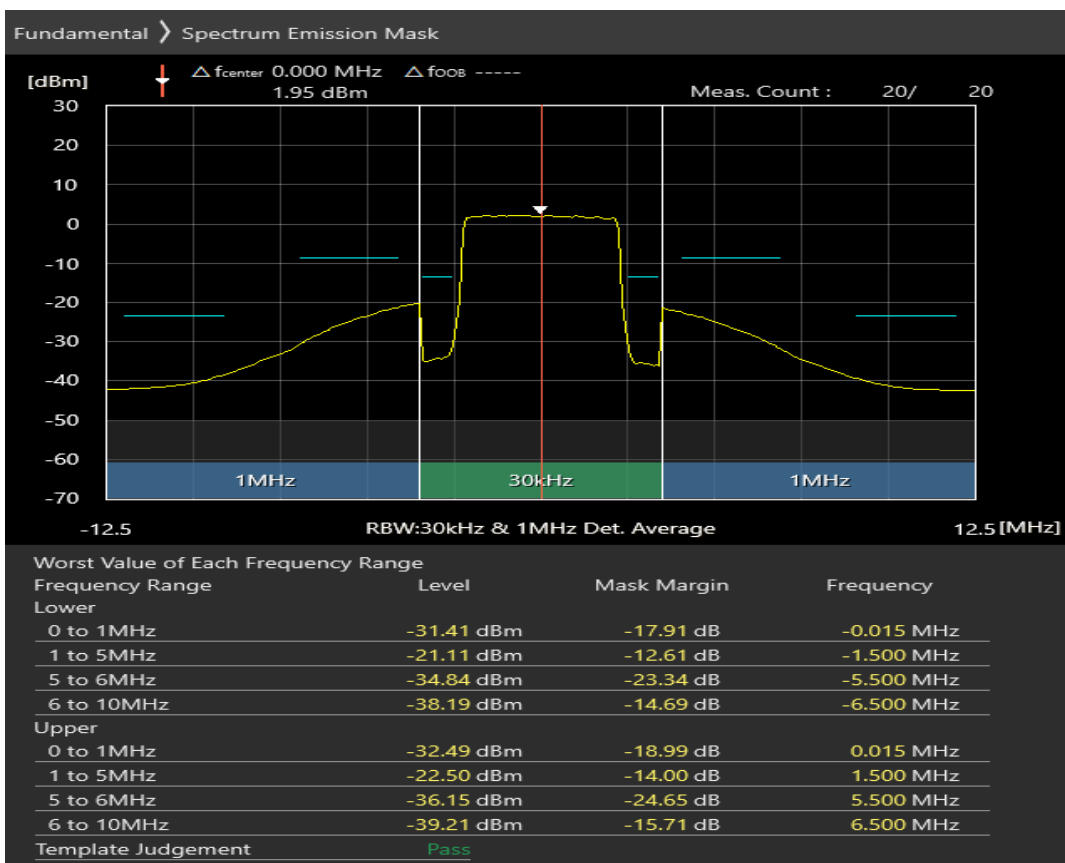
Band1 QPSK BW=10MHz Channel=18050 RB Size=12 Position=#0
