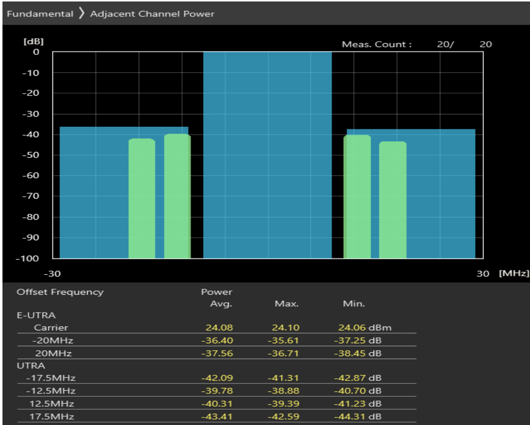
Band1 16QAM BW=20MHz Channel=18500 RB Size=18 Position=#0
