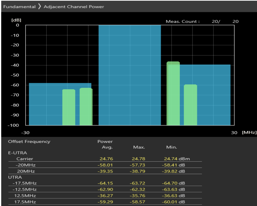
Band7 QPSK BW=20MHz Channel=21350 RB Size=100 Position=#0
