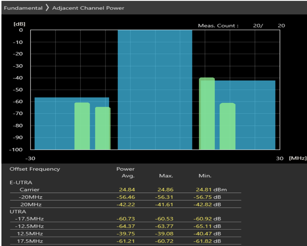
Band7 QPSK BW=20MHz Channel=21100 RB Size=100 Position=#0
