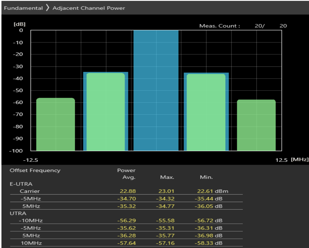
Band7 QPSK BW=10MHz Channel=20800 RB Size=12 Position=#0
