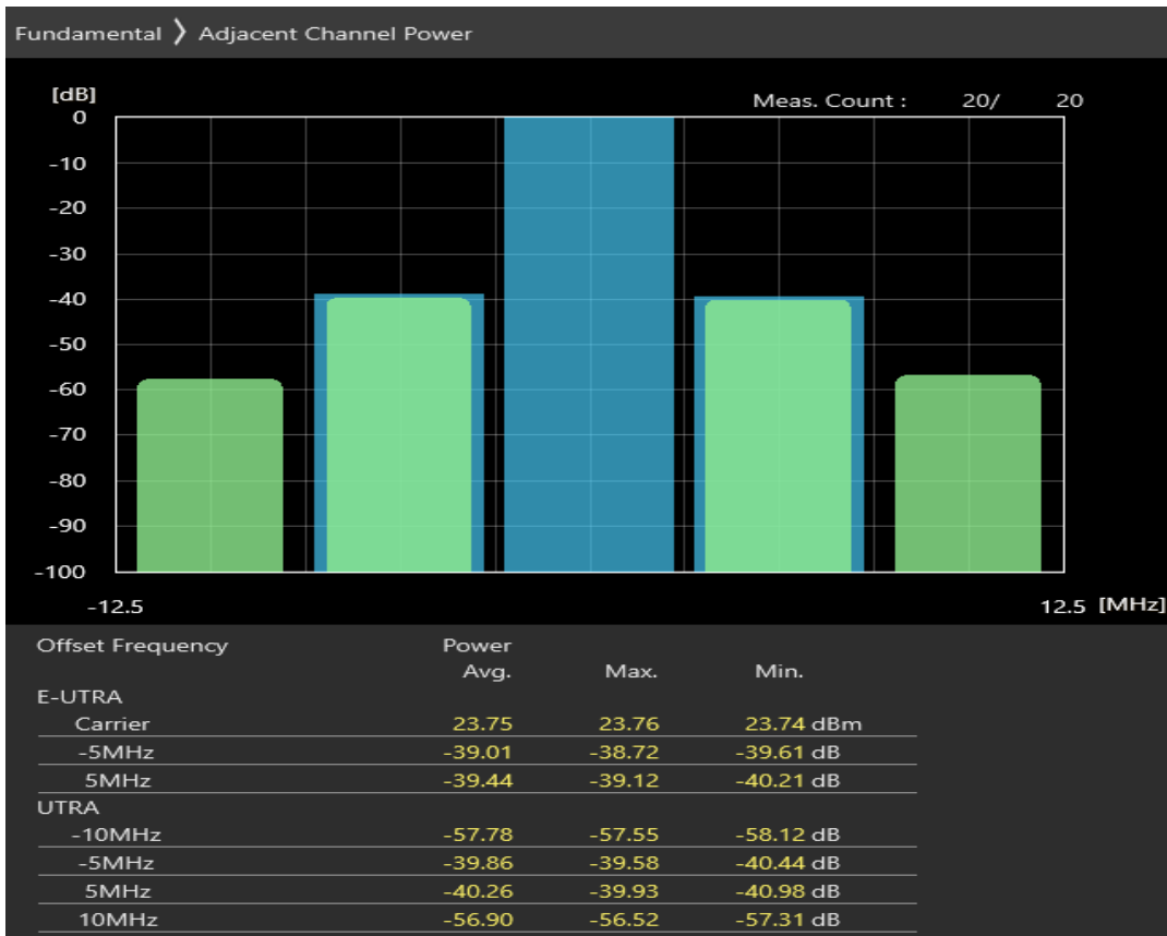
Band7 16QAM BW=5MHz Channel=21100 RB Size=8 Position=#0
