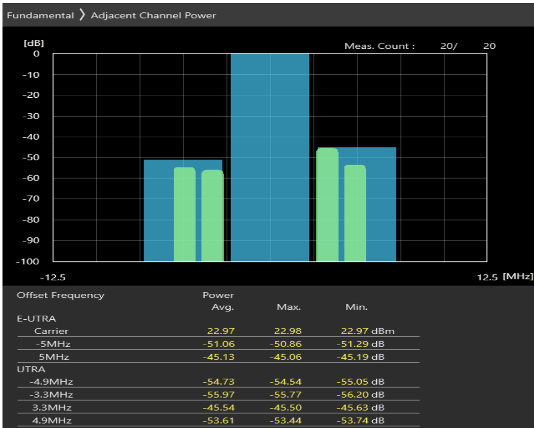
Band40 QAM16 BW=5MHz Channel=39625 RB Size=25 Position=#0
