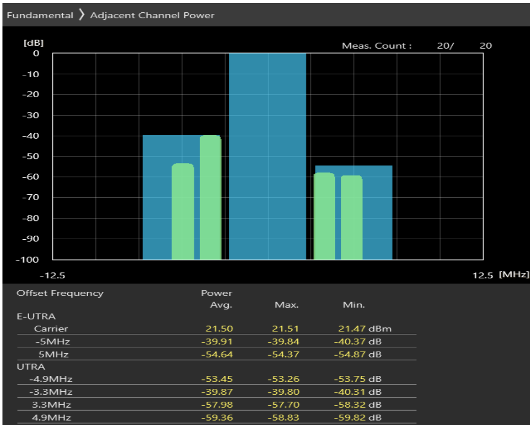
Band40 16QAM BW=5MHz Channel=39150 RB Size=8 Position=#Max
