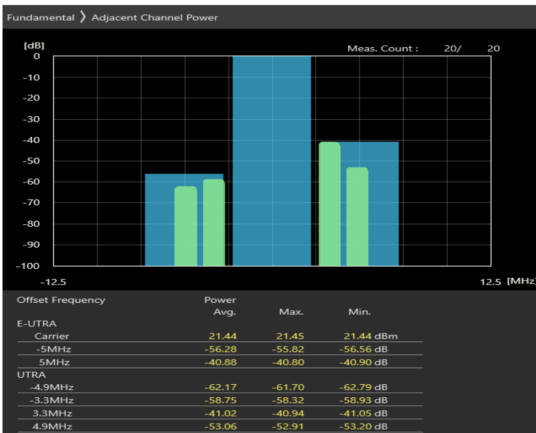
Band40 16QAM BW=5MHz Channel=39150 RB Size=25 Position=#0
