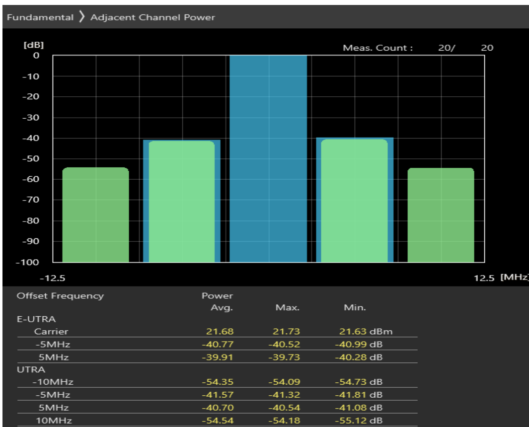
Band20 QPSK BW=5MHz Channel=24425 RB Size=8 Position=#0
