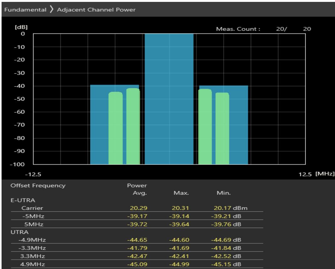
Band40 QPSK BW=5MHz Channel=39150 RB Size=8 Position=#0
