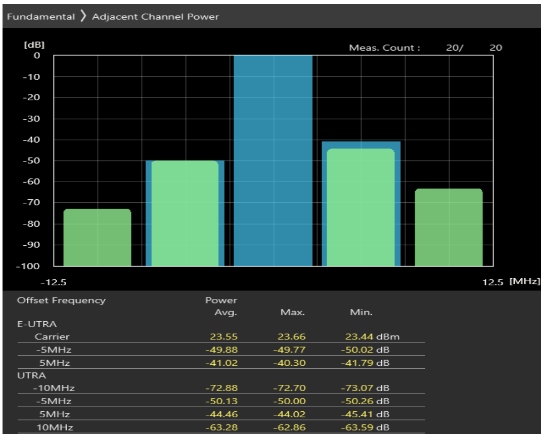
Band8 16QAM BW=5MHz Channel=21475 RB Size=25 Position=#0
