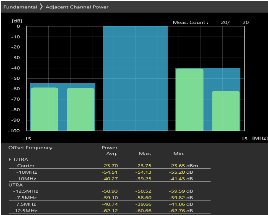
Band3 16QAM BW=10MHz Channel=19575 RB Size=50 Position=#0
