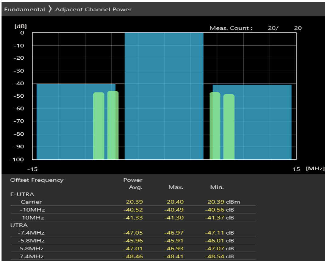
Band40 QPSK BW=20MHz Channel=38750 RB Size=18 Position=#0
