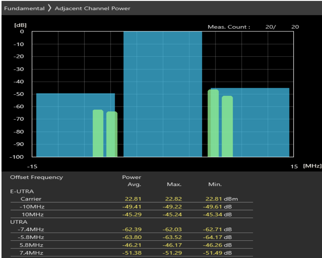
Band40 QAM16 BW=10MHz Channel=39150 RB Size=50 Position=#0
