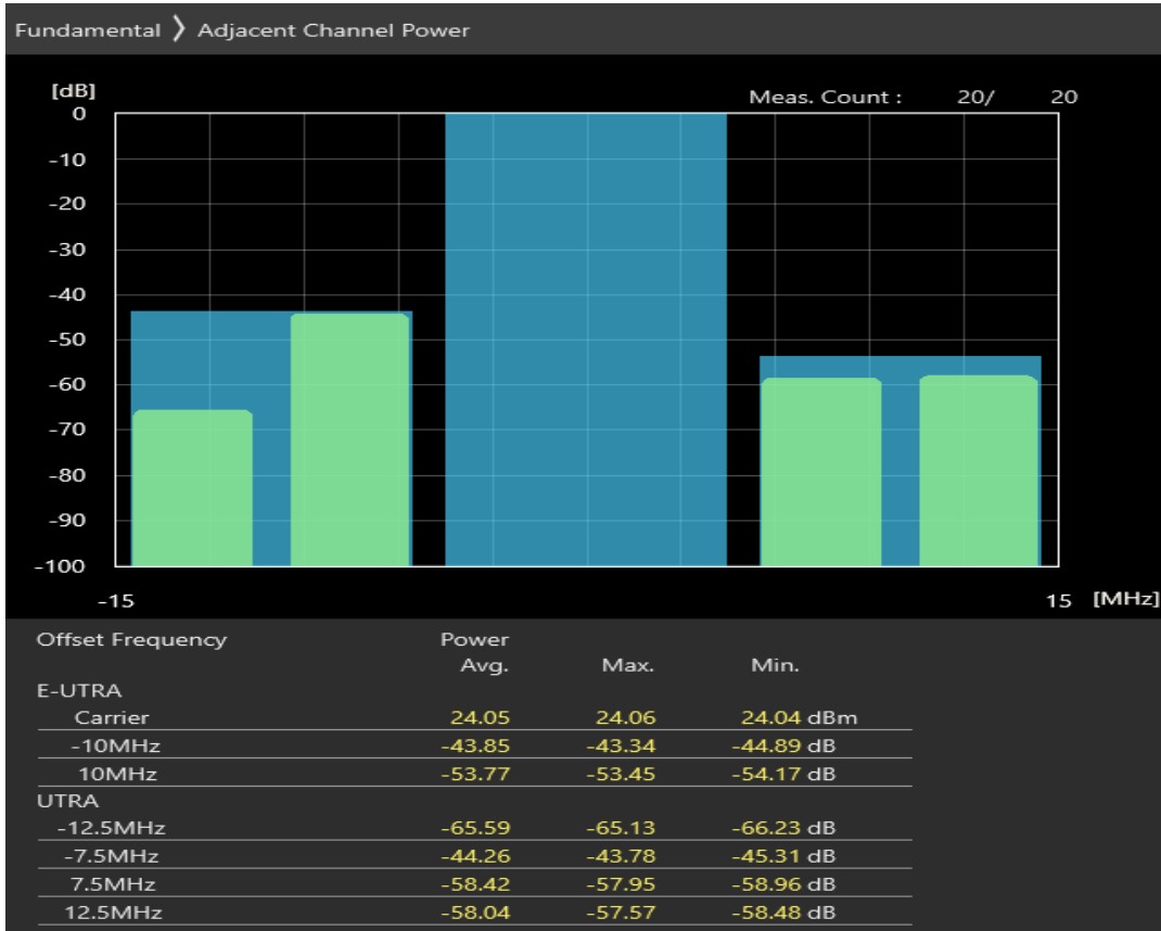
Band3 QPSK BW=10MHz Channel=19250 RB Size=12 Position=#Max
