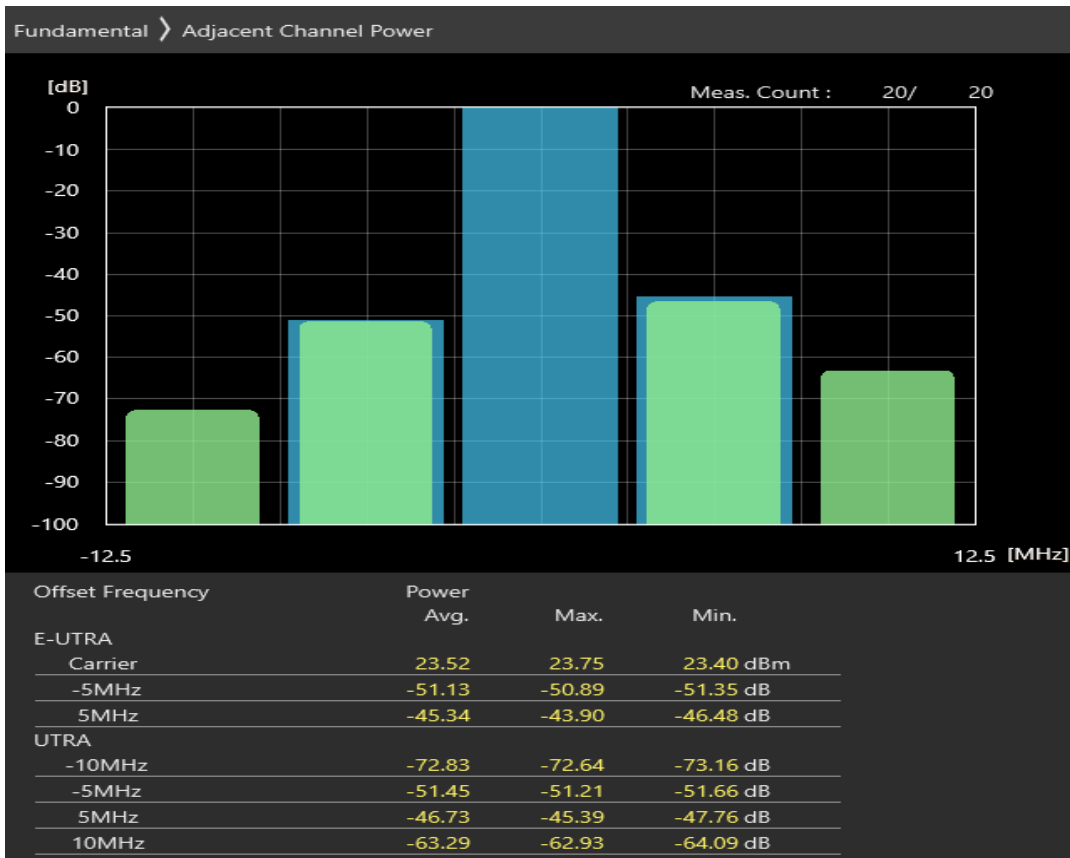
Band20 QPSK BW=5MHz Channel=24175 RB Size=25 Position=#0
