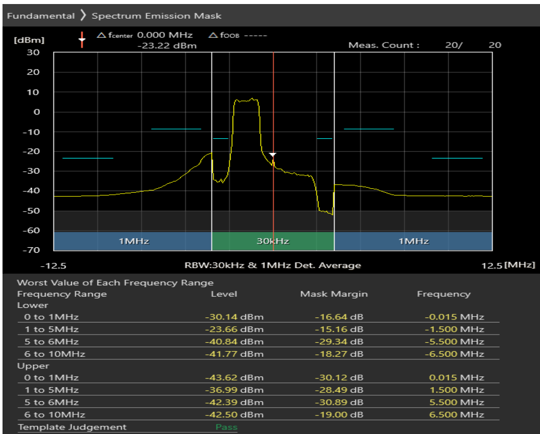
Band40 QPSK BW=5MHz Channel=39625 RB Size=8 Position=#Max
