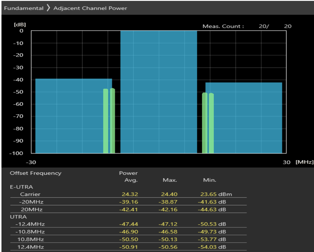
Band40 QAM16 BW=20MHz Channel=39150 RB Size=18 Position=#0
