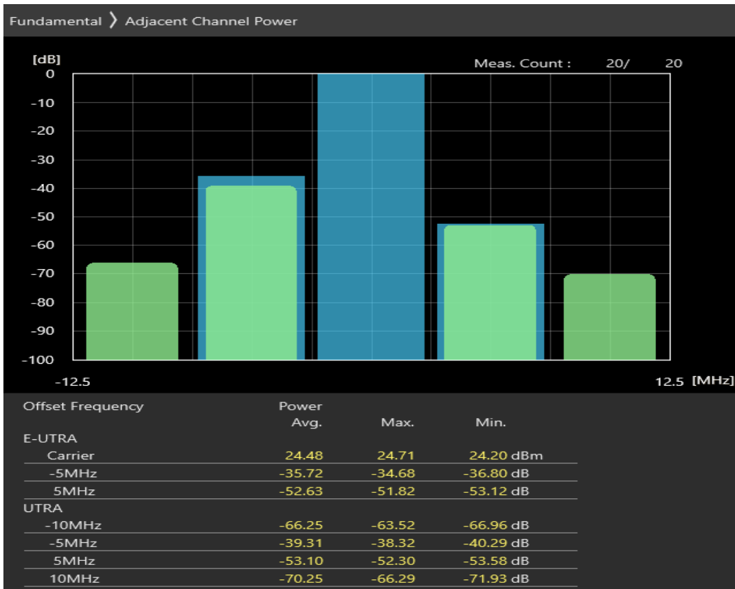
Band1 16QAM BW=5MHz Channel=18025 RB Size=8 Position=#Max
