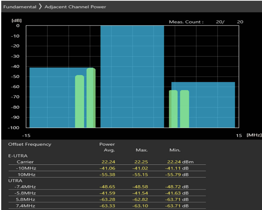
Band40 QPSK BW=10MHz Channel=39150 RB Size=12 Position=#Max
