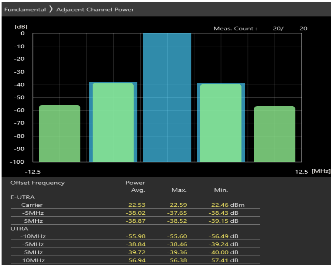
Band3 QPSK BW=5MHz Channel=19925 RB Size=8 Position=#0
