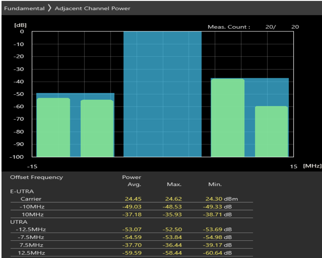
Band1 16QAM BW=10MHz Channel=18300 RB Size=50 Position=#0
