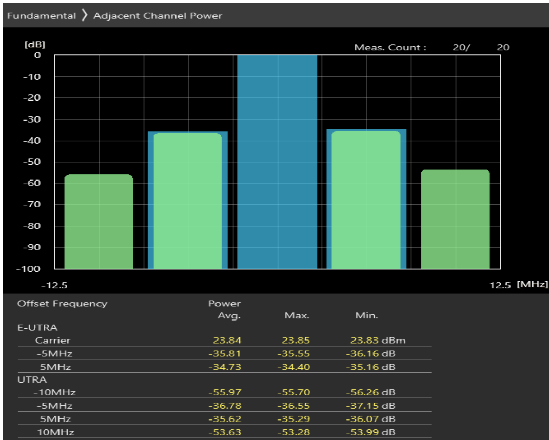
Band7 16QAM BW=5MHz Channel=20775 RB Size=8 Position=#0
