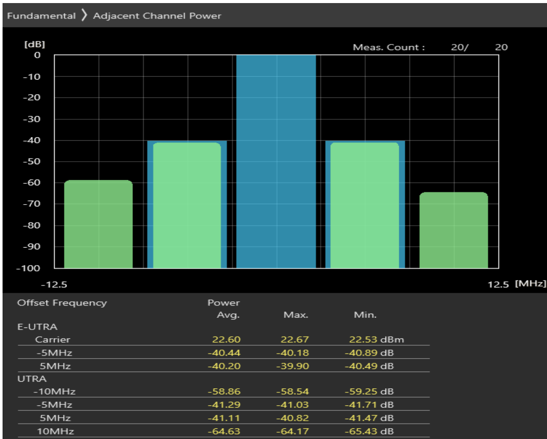
Band3 QPSK BW=10MHz Channel=19250 RB Size=12 Position=#0
