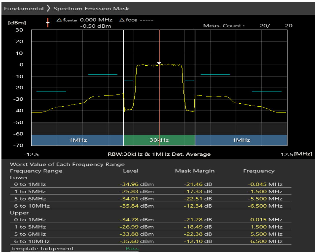
Band40 16QAM BW=5MHz Channel=39625 RB Size=8 Position=#0
