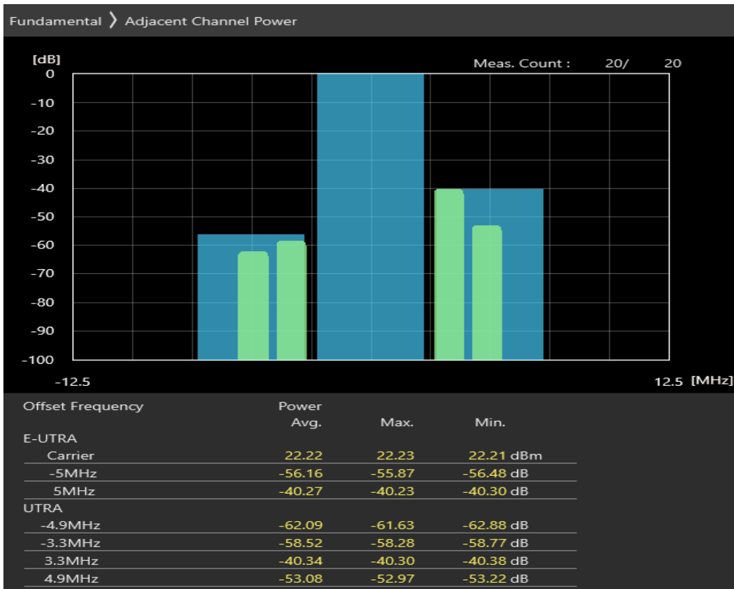
Band40 QPSK BW=5MHz Channel=38675 RB Size=25 Position=#0
