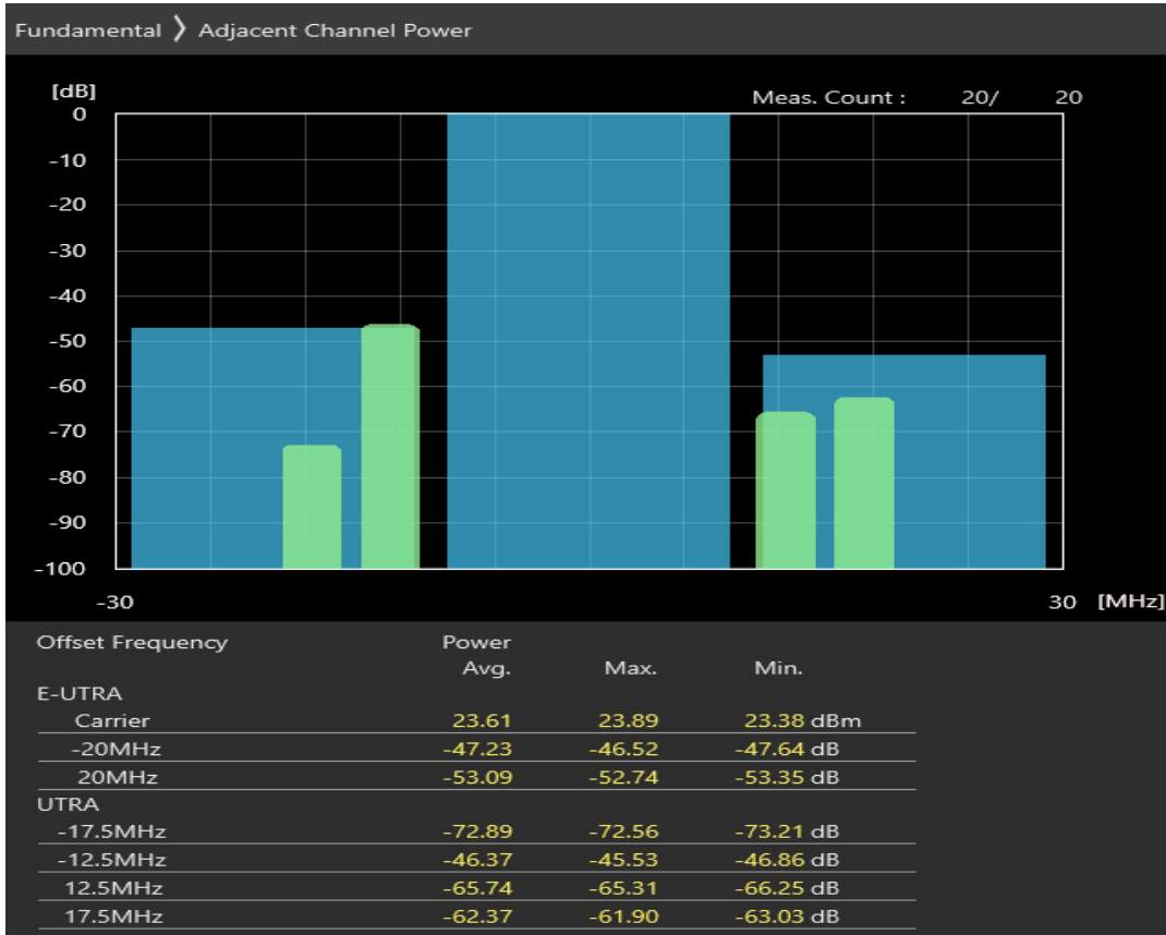
Band20 QPSK BW=20MHz Channel=24250 RB Size=18 Position=#Max
