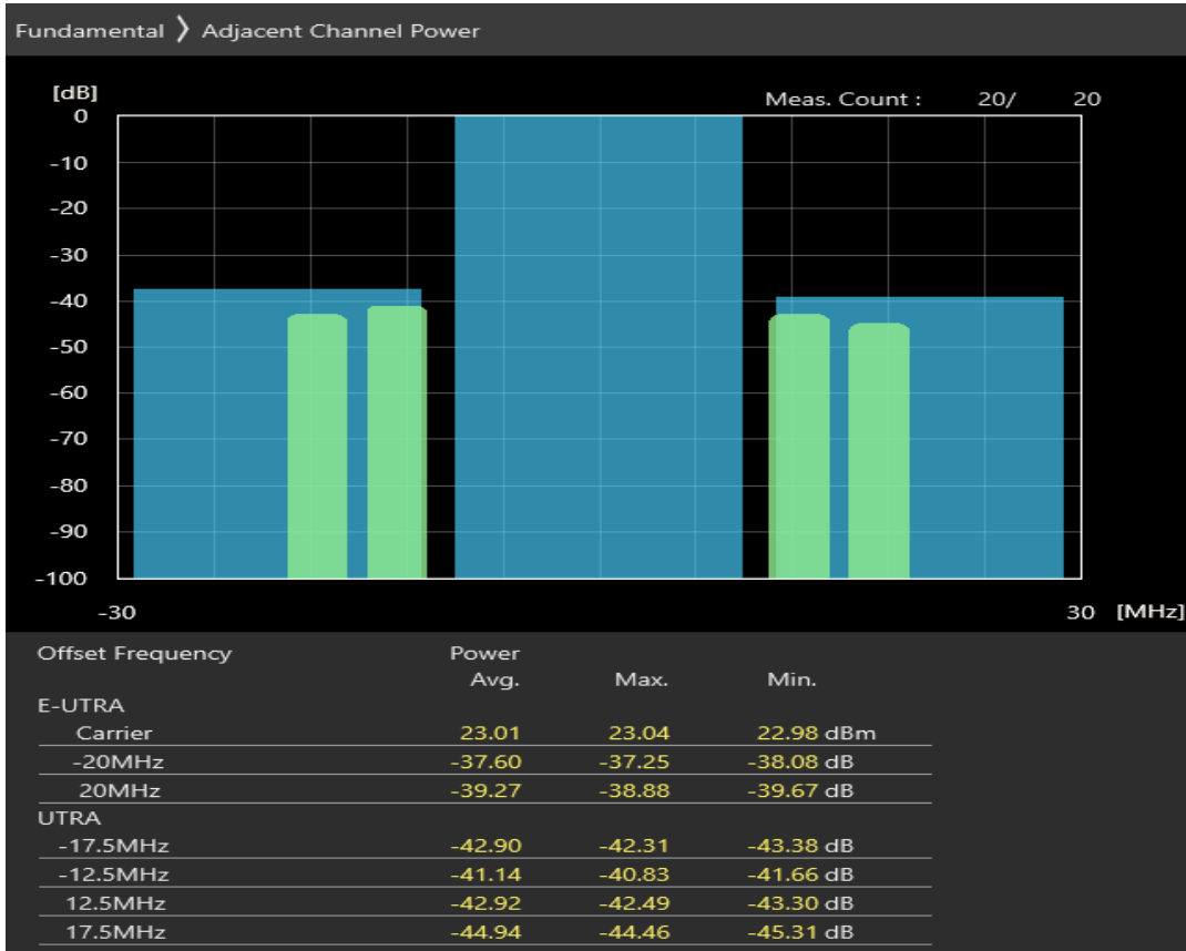
Band7 QPSK BW=20MHz Channel=21350 RB Size=18 Position=#0
