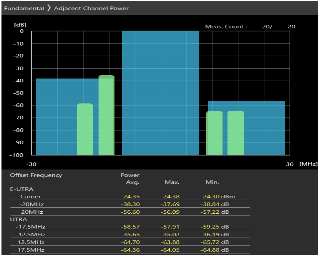
Band3 QPSK BW=20MHz Channel=19575 RB Size=18 Position=#Max
