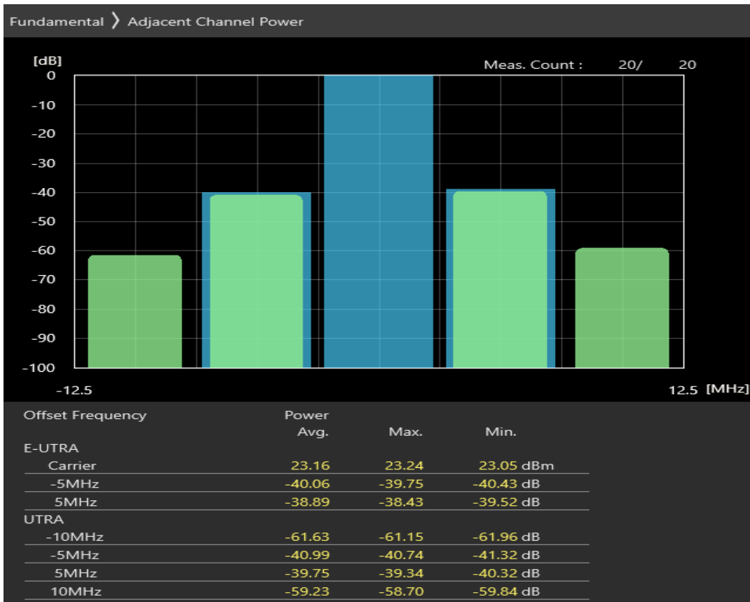
Band1 QPSK BW=5MHz Channel=18575 RB Size=8 Position=#0
