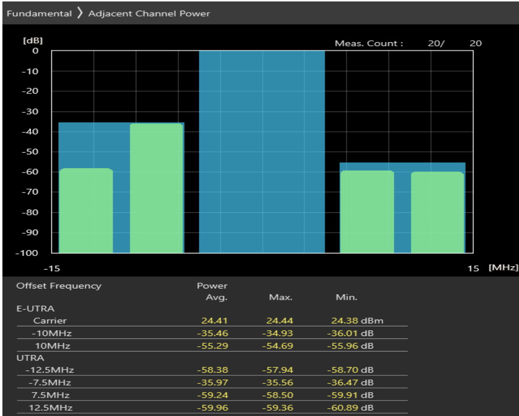
Band3 QPSK BW=10MHz Channel=19575 RB Size=12 Position=#Max
