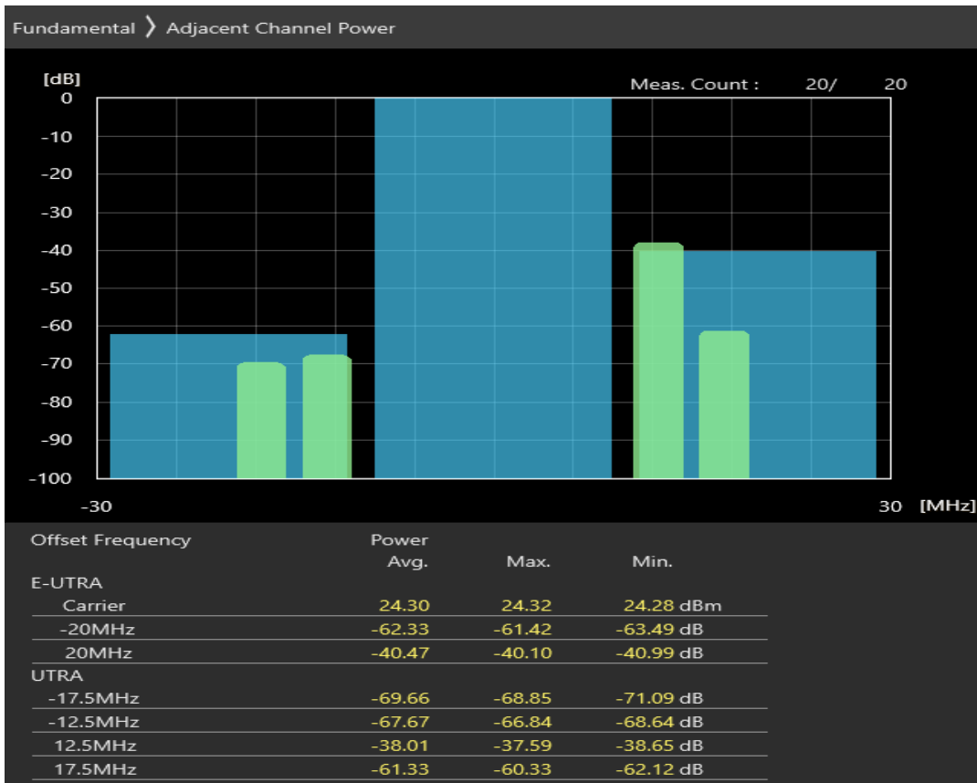
Band3 QPSK BW=20MHz Channel=19300 RB Size=100 Position=#0
