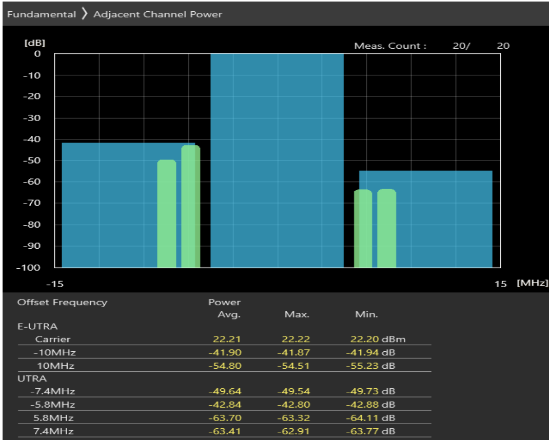
Band40 QPSK BW=10MHz Channel=39600 RB Size=12 Position=#Max
