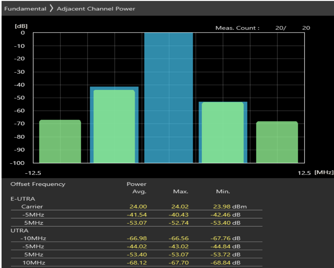
Band3 QPSK BW=5MHz Channel=19225 RB Size=8 Position=#Max
