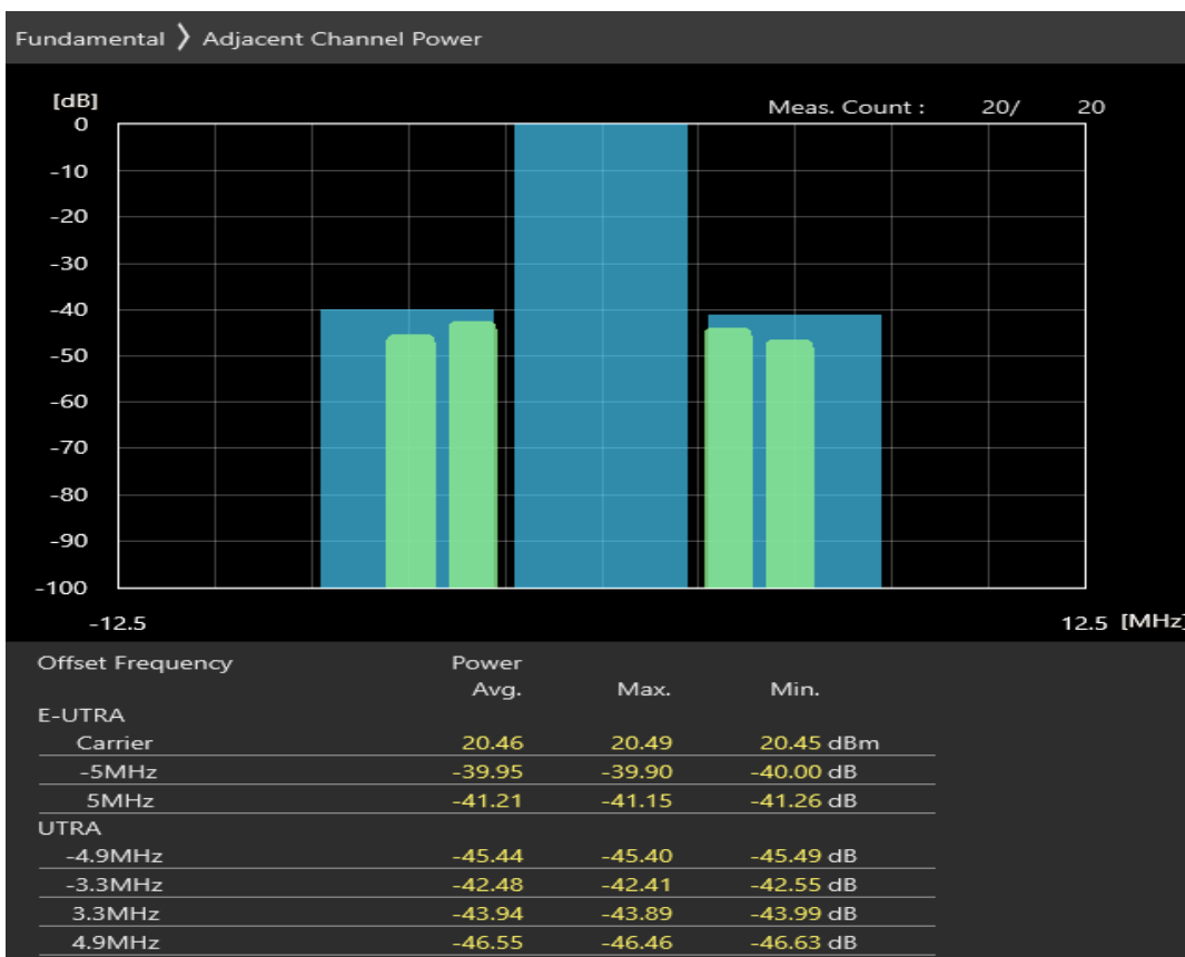
Band40 QPSK BW=5MHz Channel=39625 RB Size=8 Position=#0
