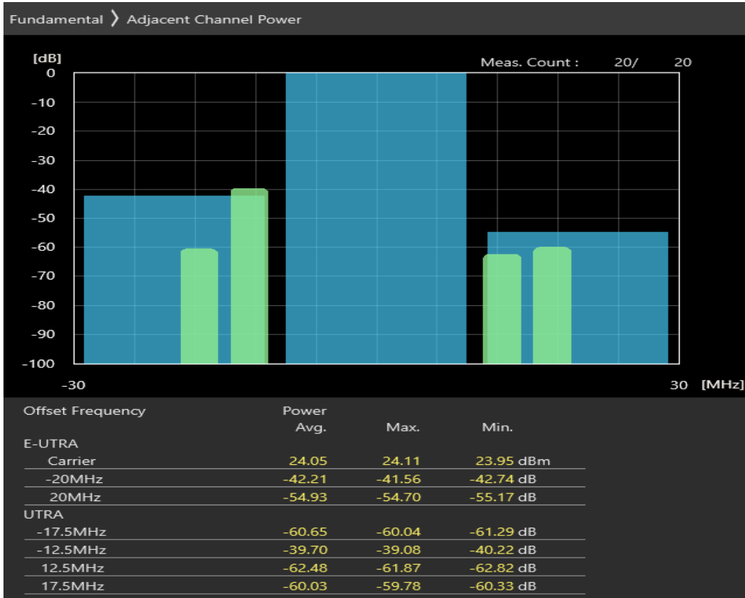
Band7 16QAM BW=20MHz Channel=21100 RB Size=18 Position=#Max
