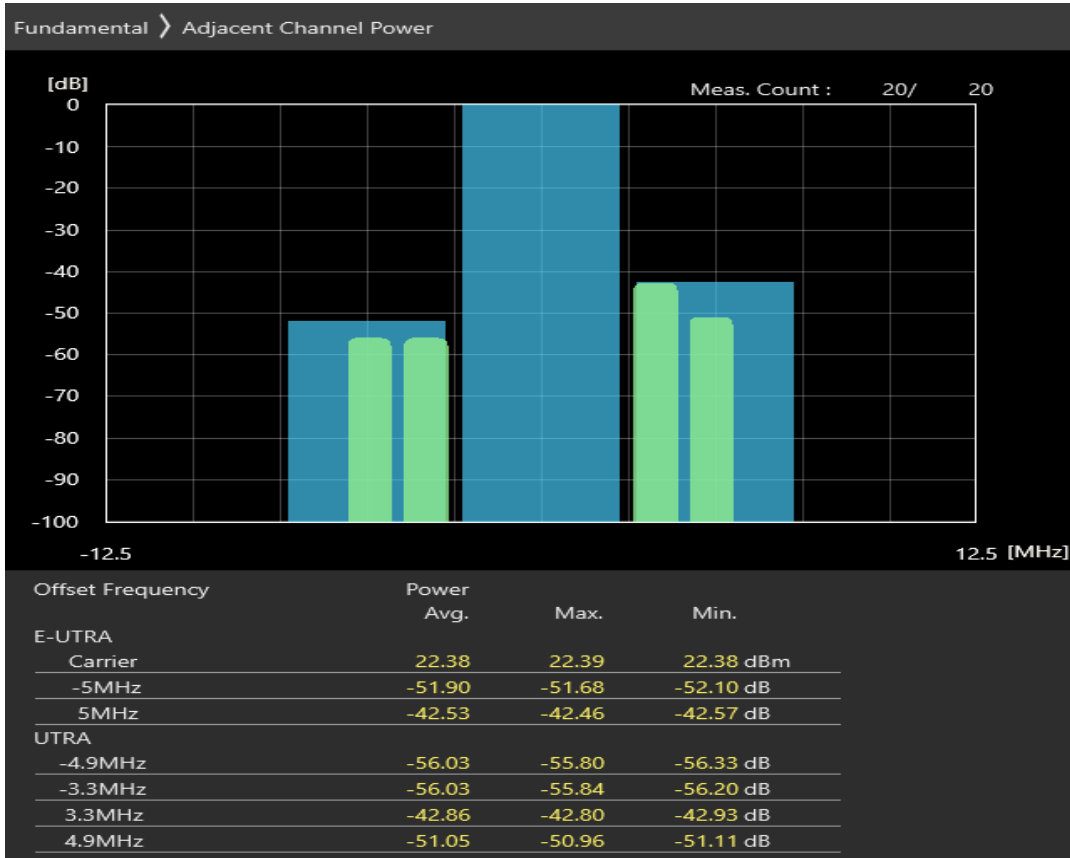
Band40 QAM16 BW=5MHz Channel=39150 RB Size=25 Position=#0
