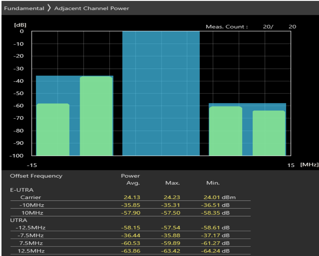
Band7 16QAM BW=10MHz Channel=21400 RB Size=12 Position=#Max
