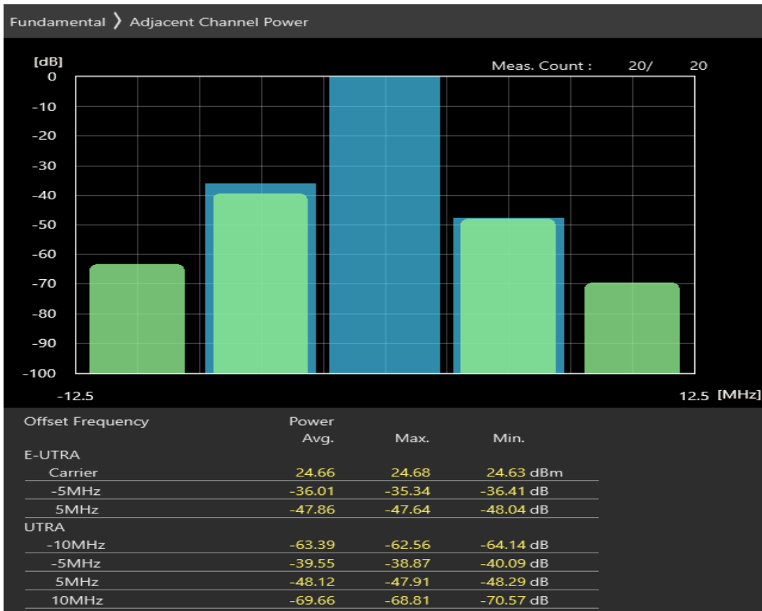
Band8 QPSK BW=5MHz Channel=21625 RB Size=8 Position=#Max
