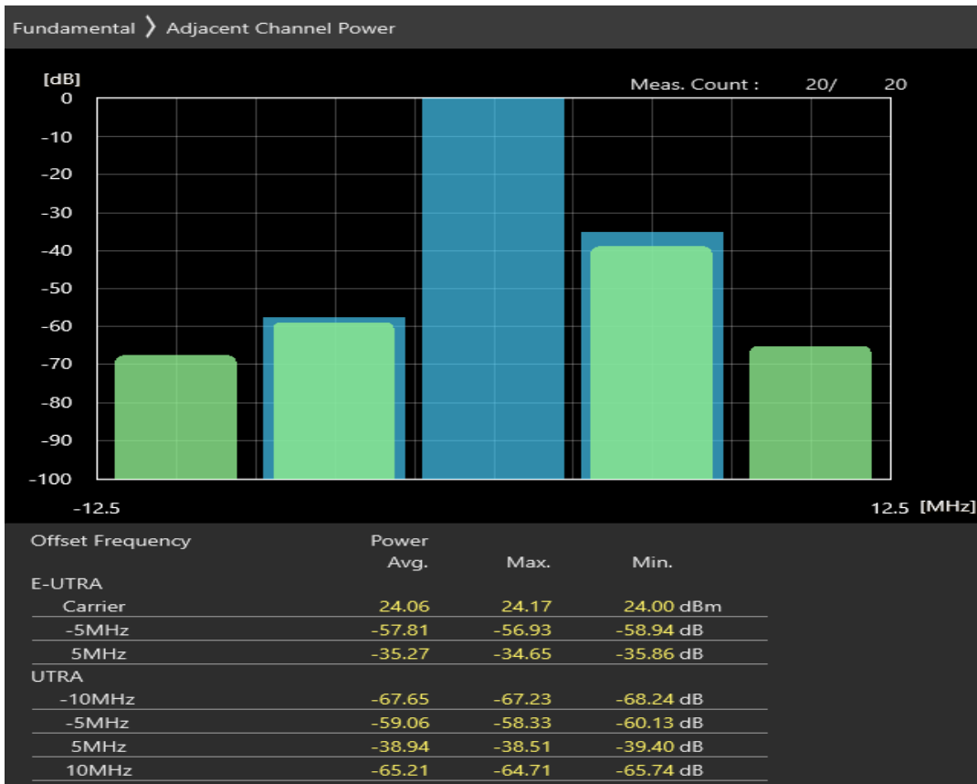
Band7 16QAM BW=5MHz Channel=20775 RB Size=25 Position=#0
