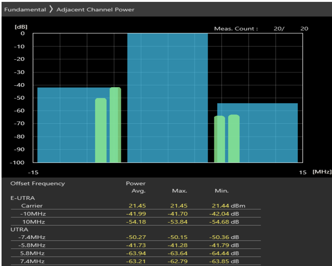
Band40 16QAM BW=10MHz Channel=39150 RB Size=12 Position=#Max
