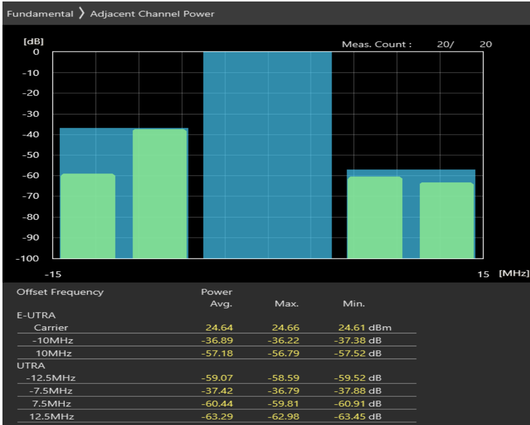
Band3 QPSK BW=10MHz Channel=1990 RB Size=12 Position=#Max
