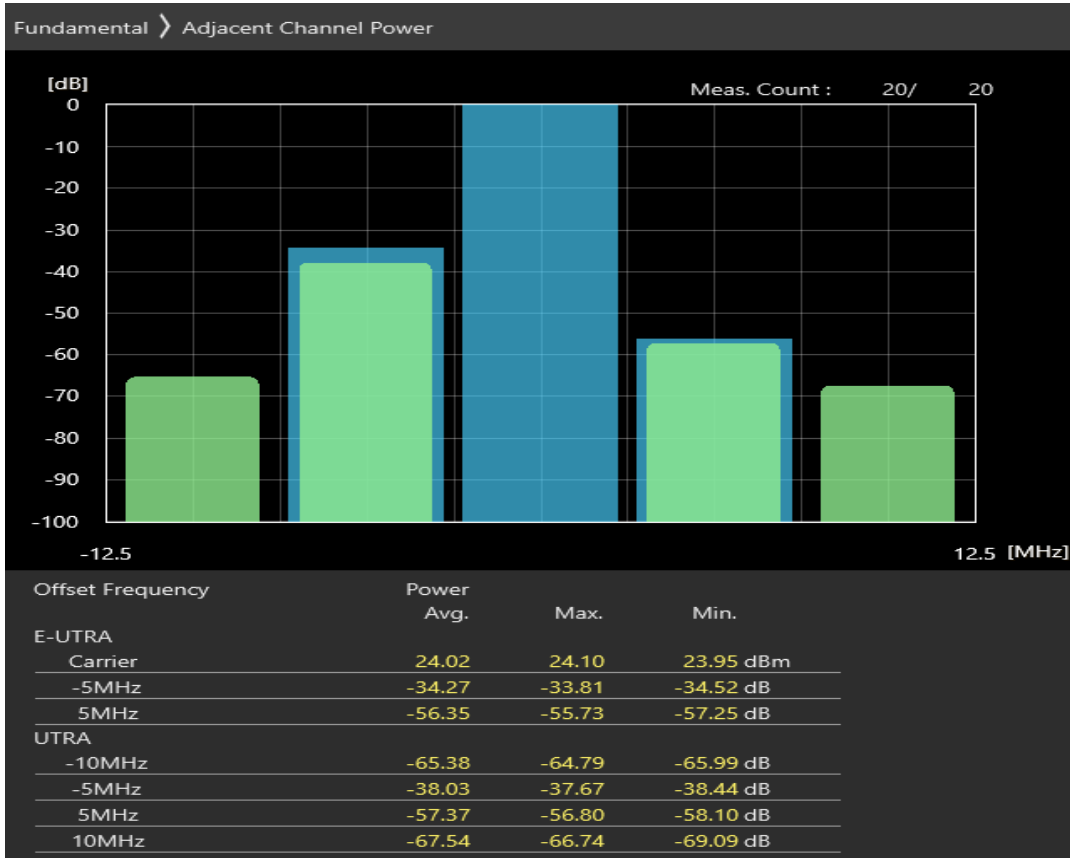
Band7 16QAM BW=5MHz Channel=21425 RB Size=8 Position=#Max
