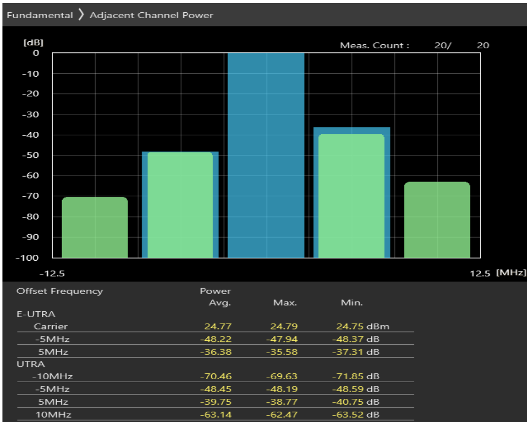
Band1 QPSK BW=5MHz Channel=18300 RB Size=25 Position=#0
