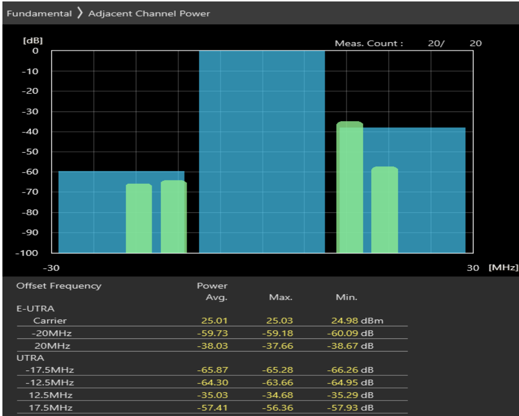
Band7 QPSK BW=20MHz Channel=20850 RB Size=100 Position=#0
