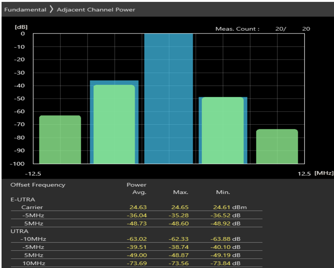
Band8 QPSK BW=5MHz Channel=21775 RB Size=8 Position=#Max
