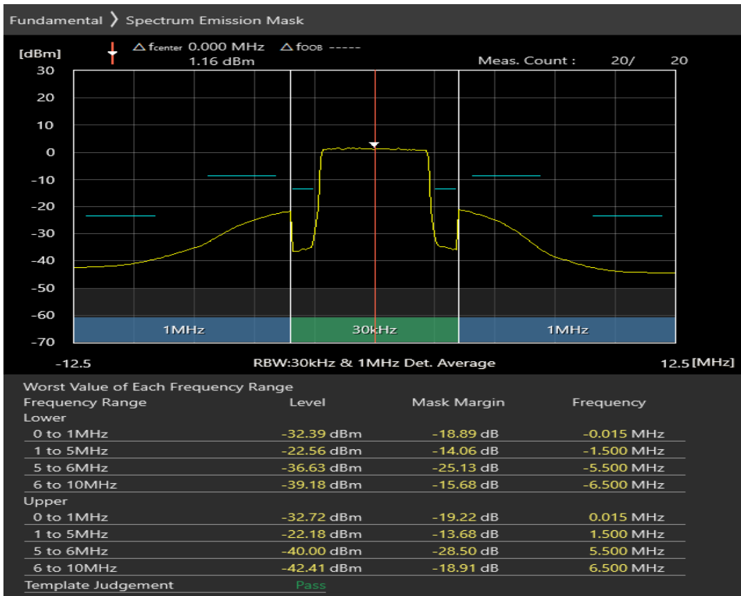
Band3 QPSK BW=10MHz Channel=19250 RB Size=12 Position=#0
