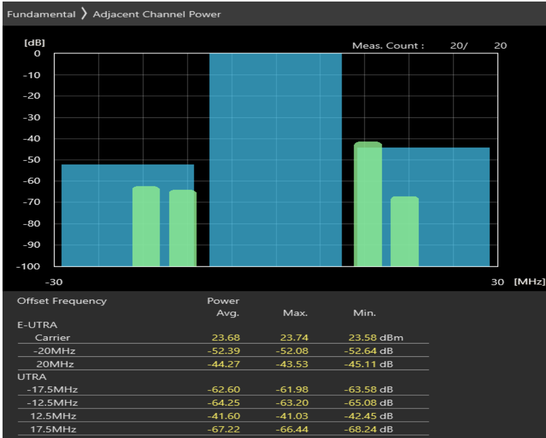
Band3 16QAM BW=20MHz Channel=19850 RB Size=100 Position=#0
