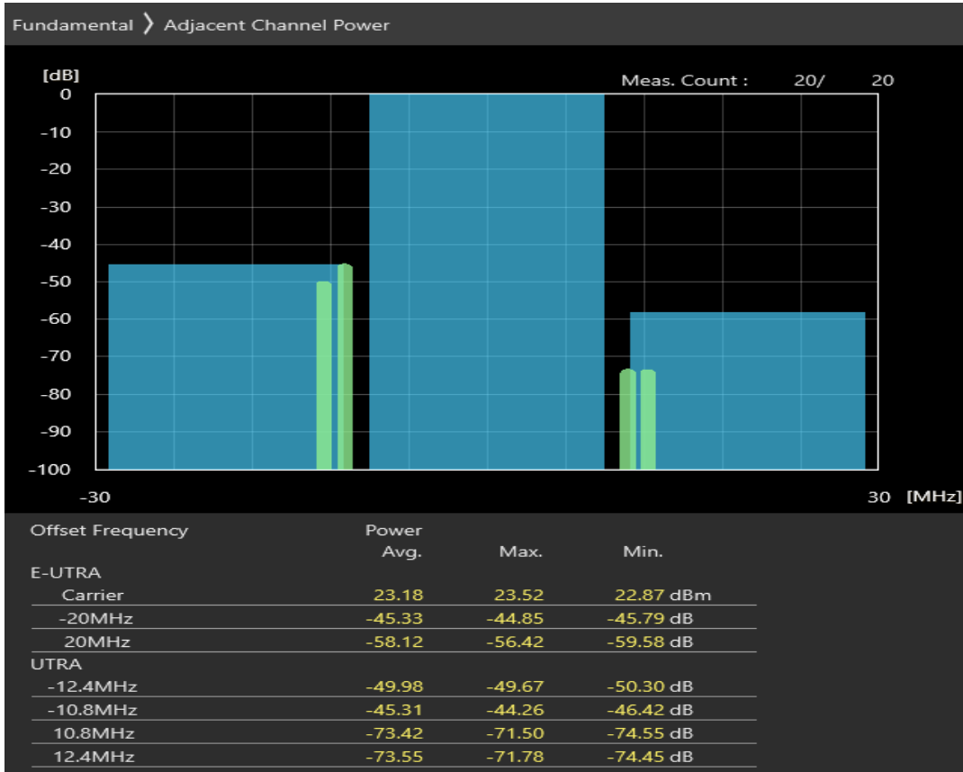
Band40 QAM16 BW=20MHz Channel=39550 RB Size=18 Position=#Max
