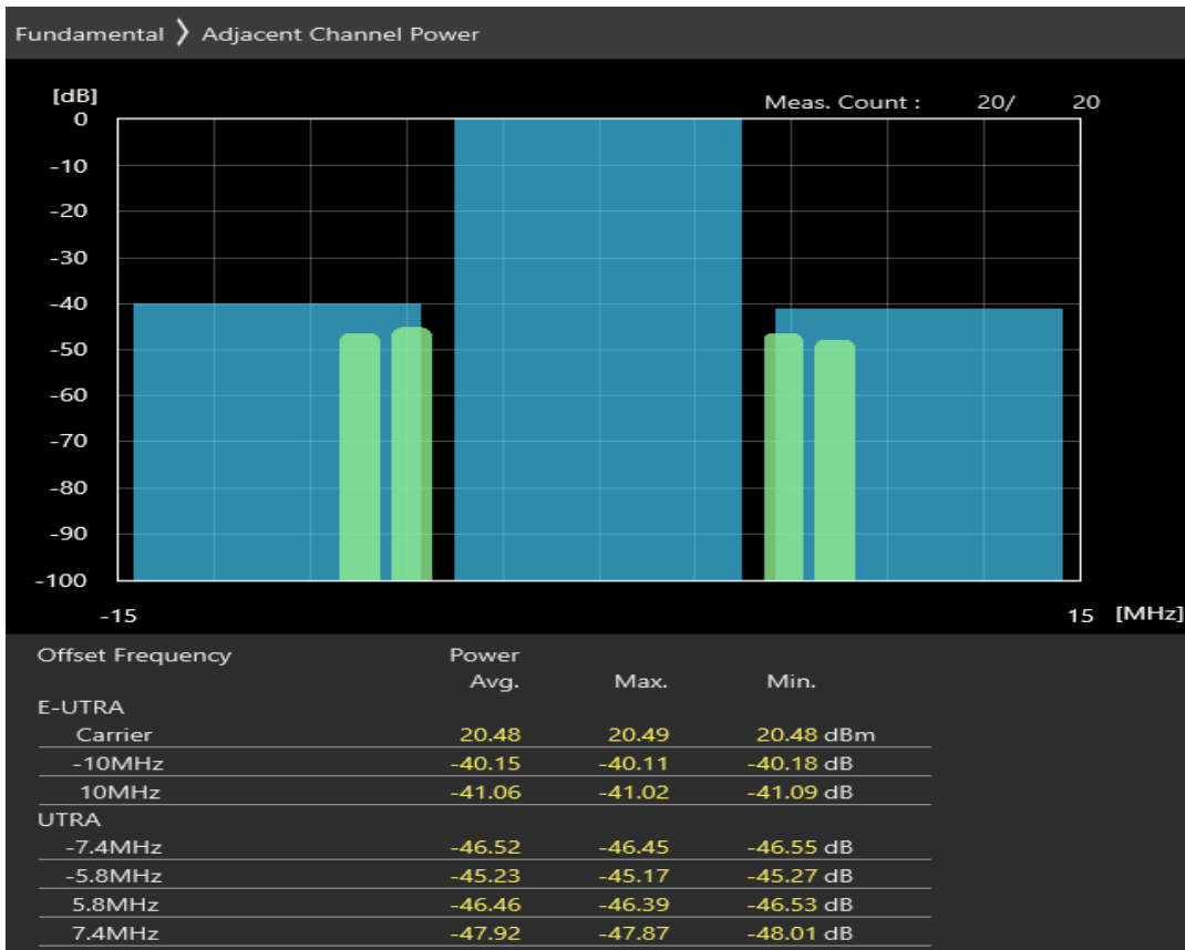
Band40 QPSK BW=10MHz Channel=39600 RB Size=12 Position=#0
