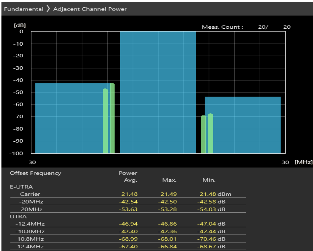
Band40 16QAM BW=20MHz Channel=38750 RB Size=18 Position=#Max
