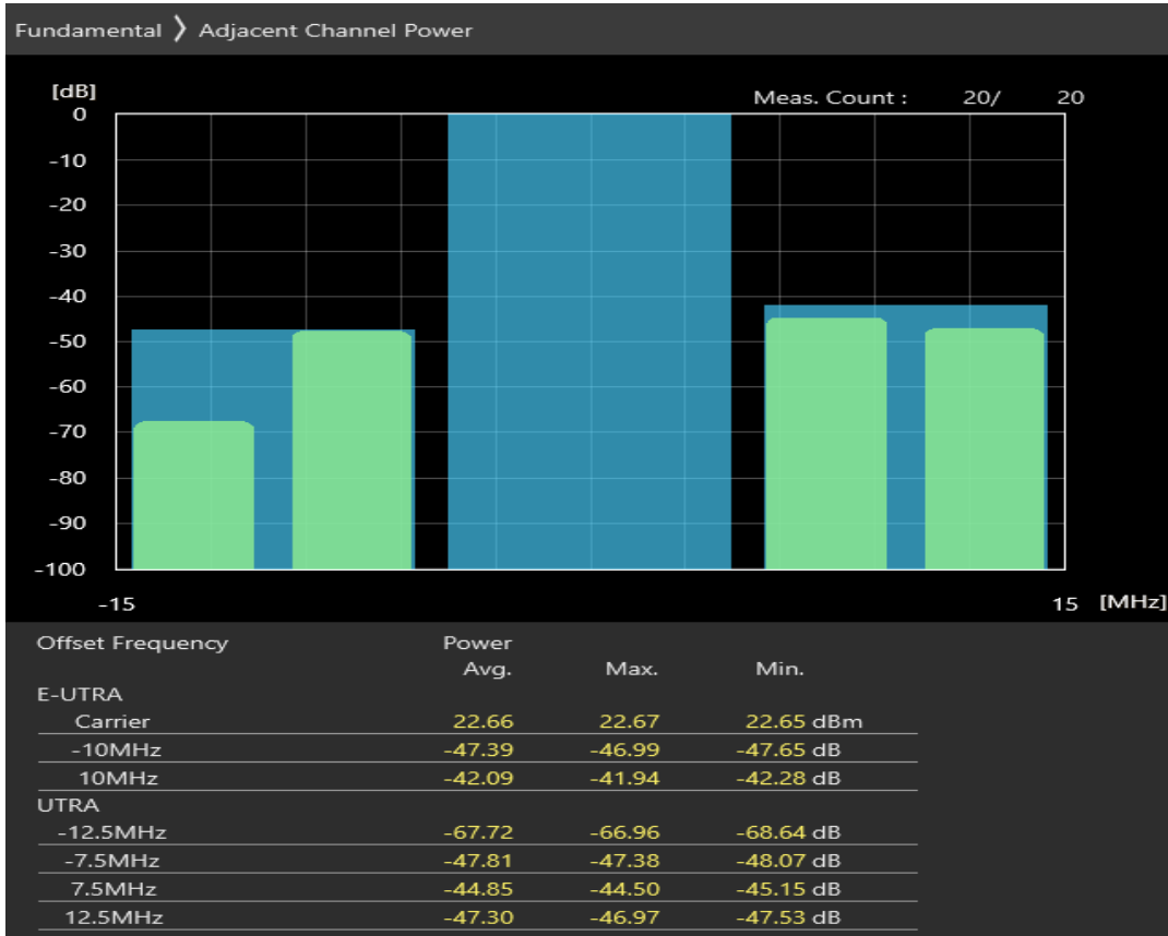
Band20 16QAM BW=10MHz Channel=24200 RB Size=12 Position=#0
