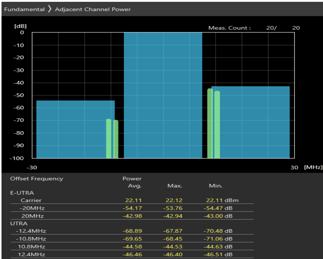
Band40 QPSK BW=20MHz Channel=38750 RB Size=100 Position=#0
