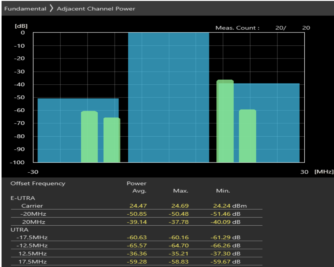
Band1 16QAM BW=20MHz Channel=18300 RB Size=100 Position=#0
