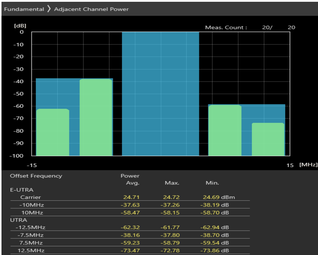
Band8 QPSK BW=10MHz Channel=21750 RB Size=12 Position=#Max
