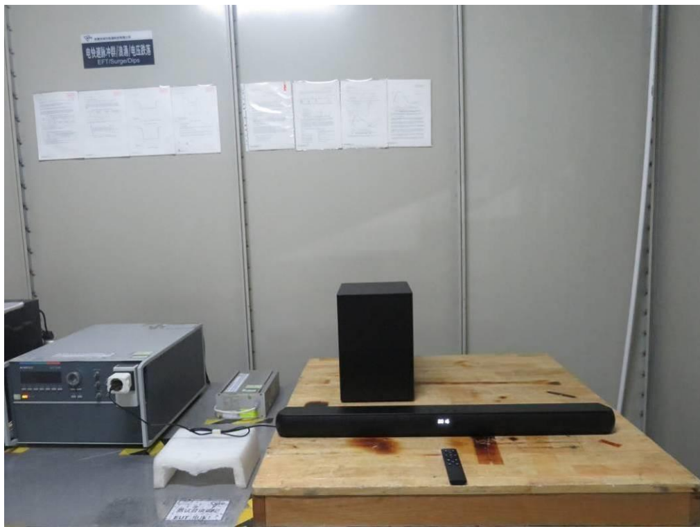
Photo of Electrical Fast Transients / Burst / Surge / Voltage Dips and Interruptions Measurement
