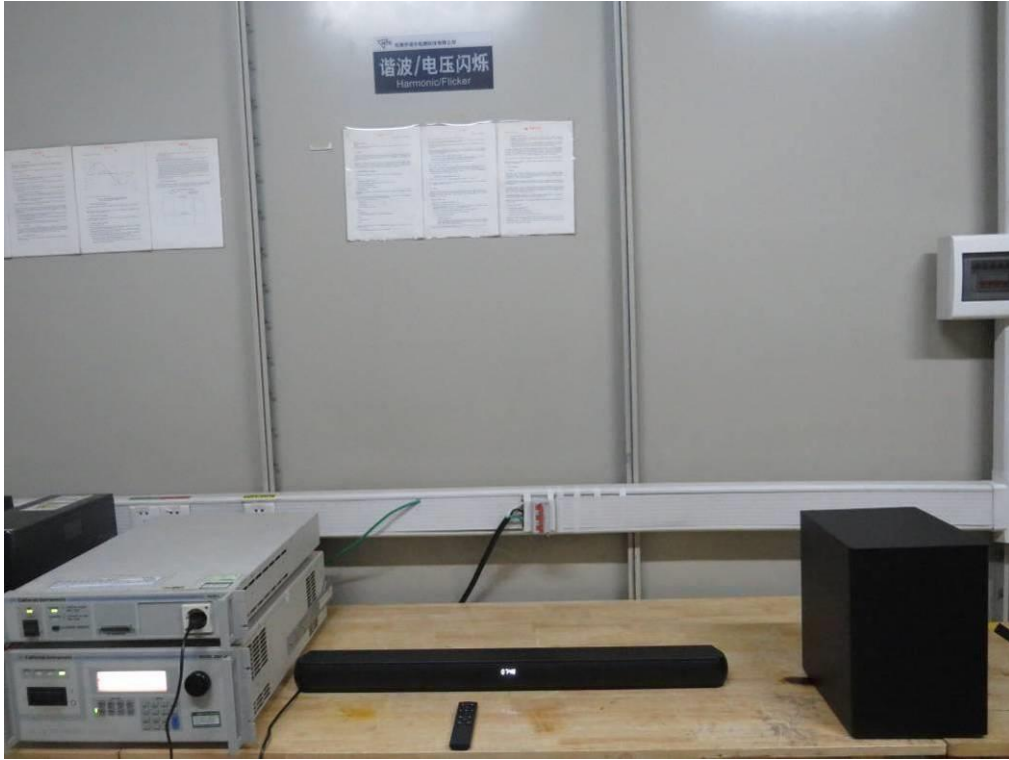
Photo of Harmonic/Flicker Measurement
