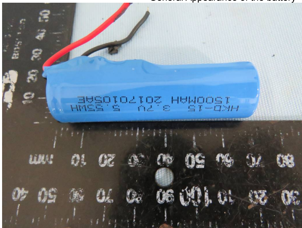
Figure 14 General Appearance of the battery
